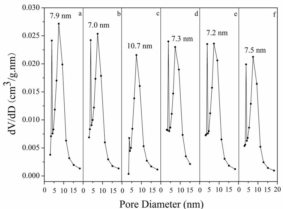
**Fig. S3** Pore size distribution curves as a function of pore diameter. (a) HZSM-5(38); (b) 4.6%Cu/HZSM-5(38) (Fresh); (c) 4.6%Cu/HZSM-5(38) (Used); (d) 4.6%Cu/HZSM-5(38) (Regenerated); (e) 2.3%Cu/HZSM-5(38); (f) 15.3%Cu/HZSM-5(38).
