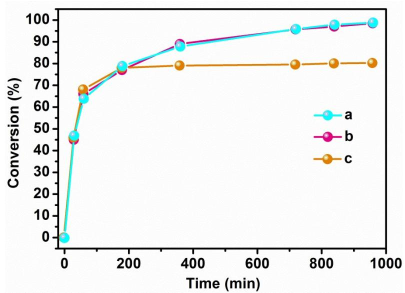
**Fig. S8** Recycle reaction kinetics for the formation of propylene carbonate catalysed by **1** at 100°C and 1 atm (a) cycle 1, (b) cycle 2 and (c) after the reaction was performed for 3 hours, **1** was removed from the mixture and the reaction was continued for another 13 hours.
