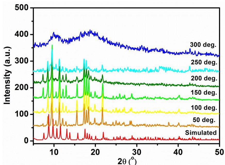
**Fig. S3** The PXRD patterns of **1** recorded at different temperatures.
