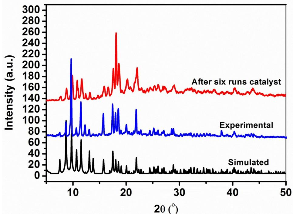
**Fig. S7** The PXRD patterns of **1** after six runs for the cycloaddition of  $\text{CO}_2$  with propylene oxide.
