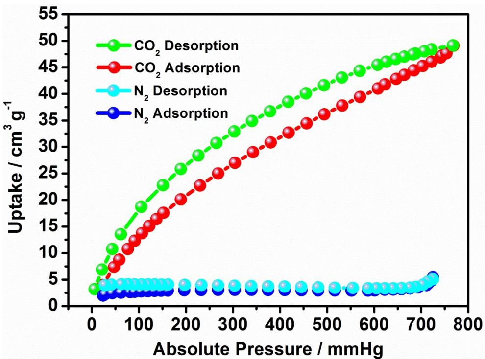
**Fig. S6** The Gas sorption isotherms of **1** for  $\text{CO}_2$  and  $\text{N}_2$  measured at 273 K.
