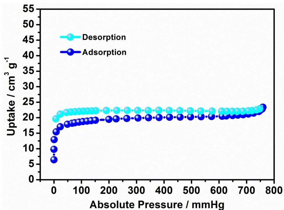
Fig. S5 The Gas sorption isotherm of 1 for N<sub>2</sub> measured at 77 K.
