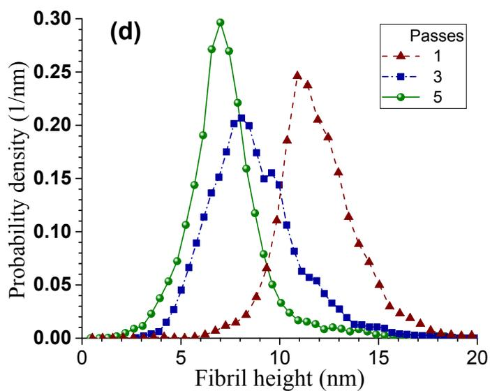
Fig. S1. Effect of the degree of mechanical fibrillation measured by the number of passes through the 87  $\mu\text{m}$  chamber of the microfluidizer on CNF morphology. The FCSR was produced from hydrolysis of BEP under (A70, 100, 30). (a), (b) and (c) are AFM images of the CNFs. (d) is the AFM measured CNF height (equivalent to diameter) distribution.
