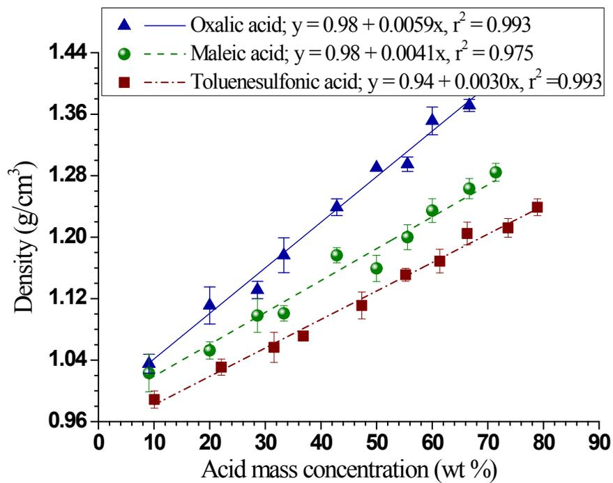
Fig. S3 Densities of concentrated organic acid aqueous solutions at different concentrations at 100 °C.
