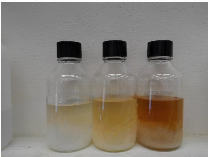
Fig. S2. Crystallization of oxalic acid at ambient temperature in hydrolysates (diluted 3 times at 80°C) after reacting with BEP fibers at different acids concentrations. From left to right: (O50, 100, 45); (O60, 100, 45); and (O70, 100, 45).
