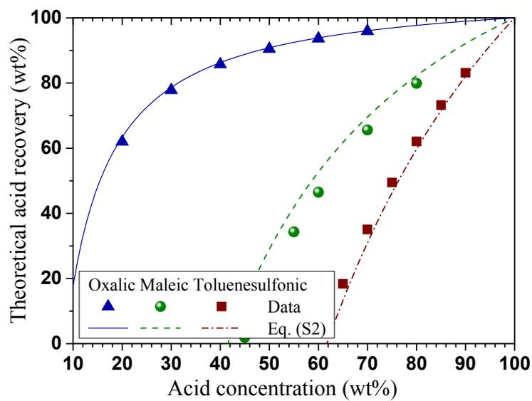
Fig. S6 Acid recoveries at different acid concentrations estimated based on UV absorption measured acid concentrations and solubility limit.
