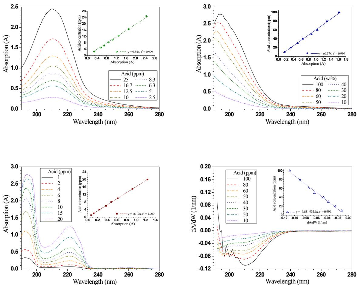
Fig. S4. Absorption spectra and wavelength derivative spectra of three organic acids at various concentrations in aqueous solutions. (a) Maleic acid; (b) p-Toluenesulfonic acid; (c) Oxalic acid; (d) Oxalic acid wavelength derivative spectra. Inserts show acid concentration calibration lines.
