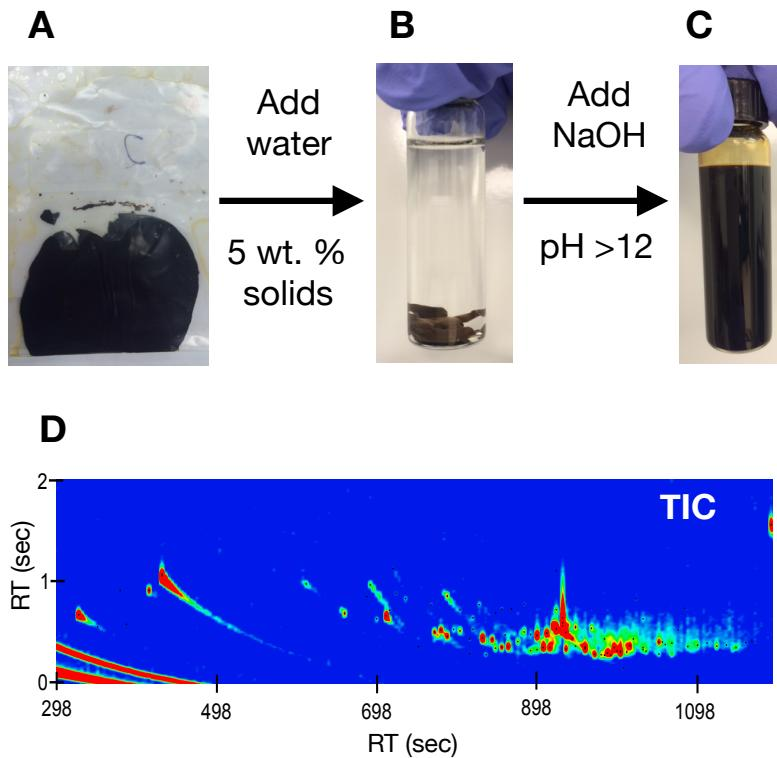
**Figure S5:** (A) Pyrolytic lignin sample at ~20-30 wt.% exhibits a tar like consistency. (B) The sample is diluted in water to ~5 wt.% solids. Here the pyrolytic lignin is completely insoluble. (C) Solid sodium hydroxide is added to the solution until the pH is > 12 solubilizing the material. Then the sample is derivatized following the same workup protocol as that used for the APL samples. (D) TIC chromatogram from the GCxGC-TOFMS analysis of the derivatized sample.
