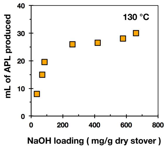
**Figure S6:** Volume of APL produced (in mL) as a function of NaOH loading for corn stover pretreatments at 130 °C in accordance with our previous work presented in Ref. 1
