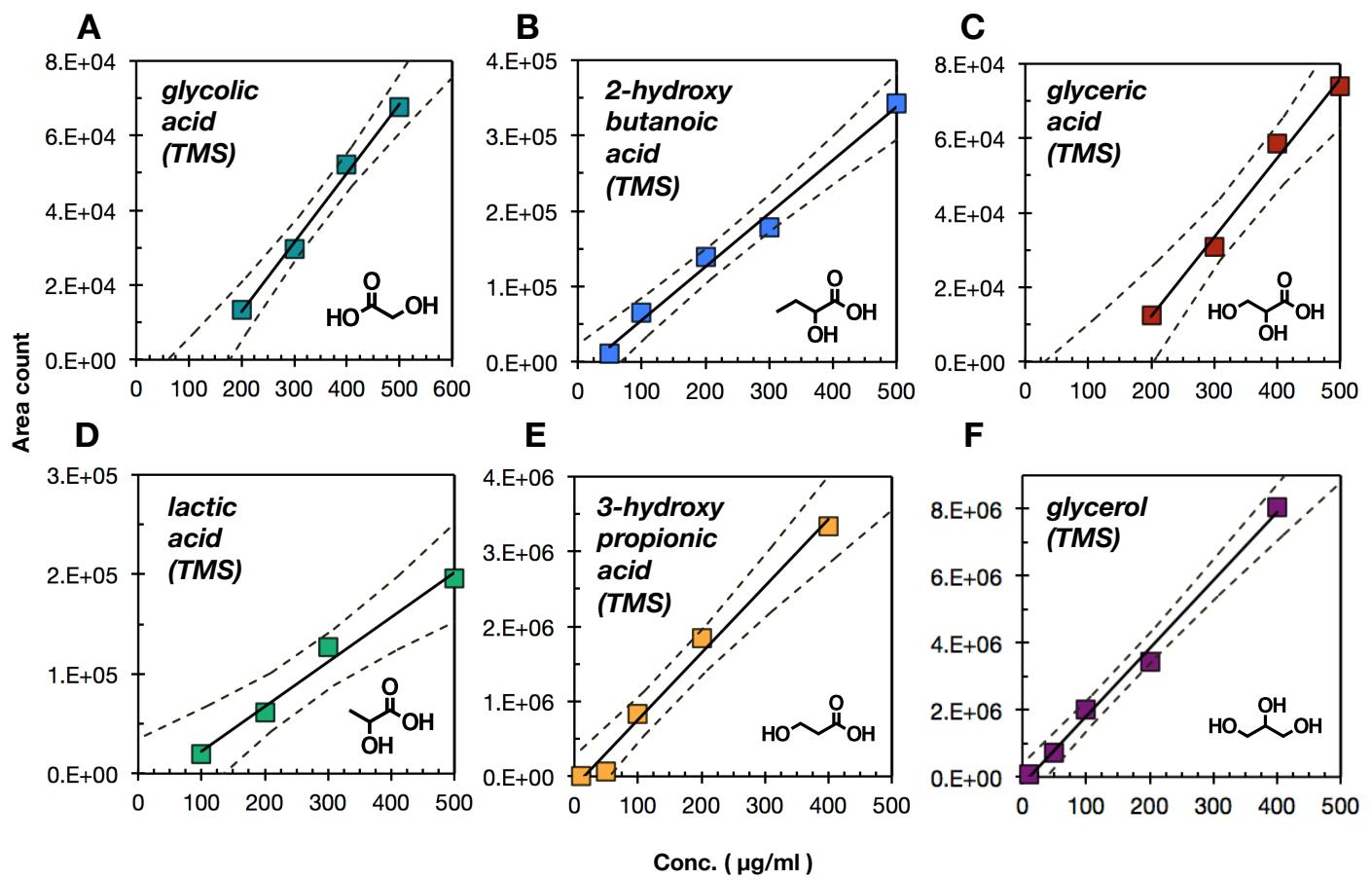
Figure S3: Calibration curves for sugar degradation products.
