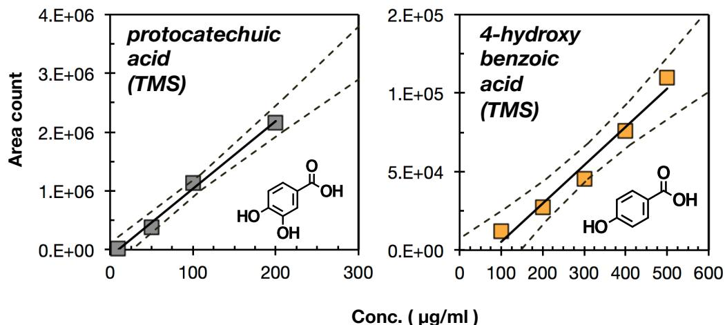
**Figure S4:** Calibration curves for the TMS derivatives of protocatechuic acid and 4-hydroxy benzoic acid. These compounds are produced biologically during fermentation of APL samples.
