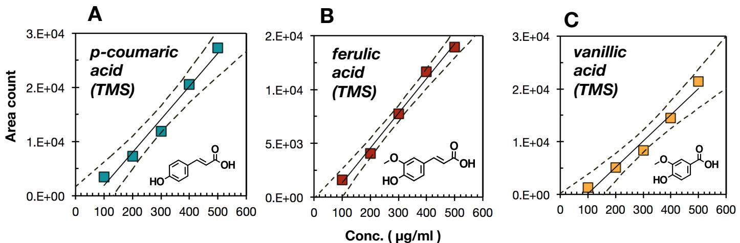
**Figure S2:** calibration curves for lignin derived monomers.
