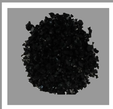
Fig. S1 As synthesized PAF material. Synthesis condition: 3, 3'-diaminobenzidine (1 mmol), (diacetoxyiodo) benzene (4 mmol) and DMSO (10 mL), RT, 24 h.
