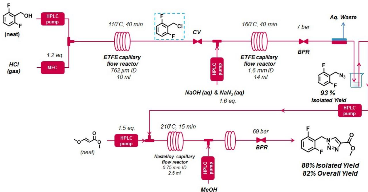
**Scheme S6.** Schematic representation of setup assembled for 3-step continuous synthesis of rufinamide precursor.
