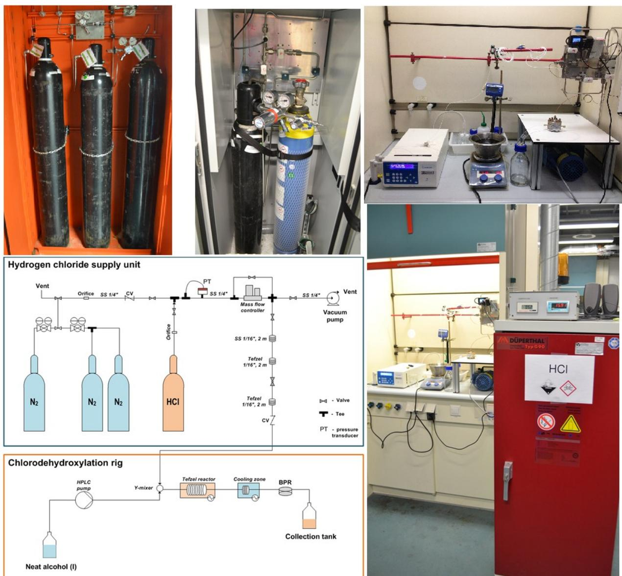
**Scheme S2.** Schematic representation of setup assembled for continuous chlorodehydroxylation
