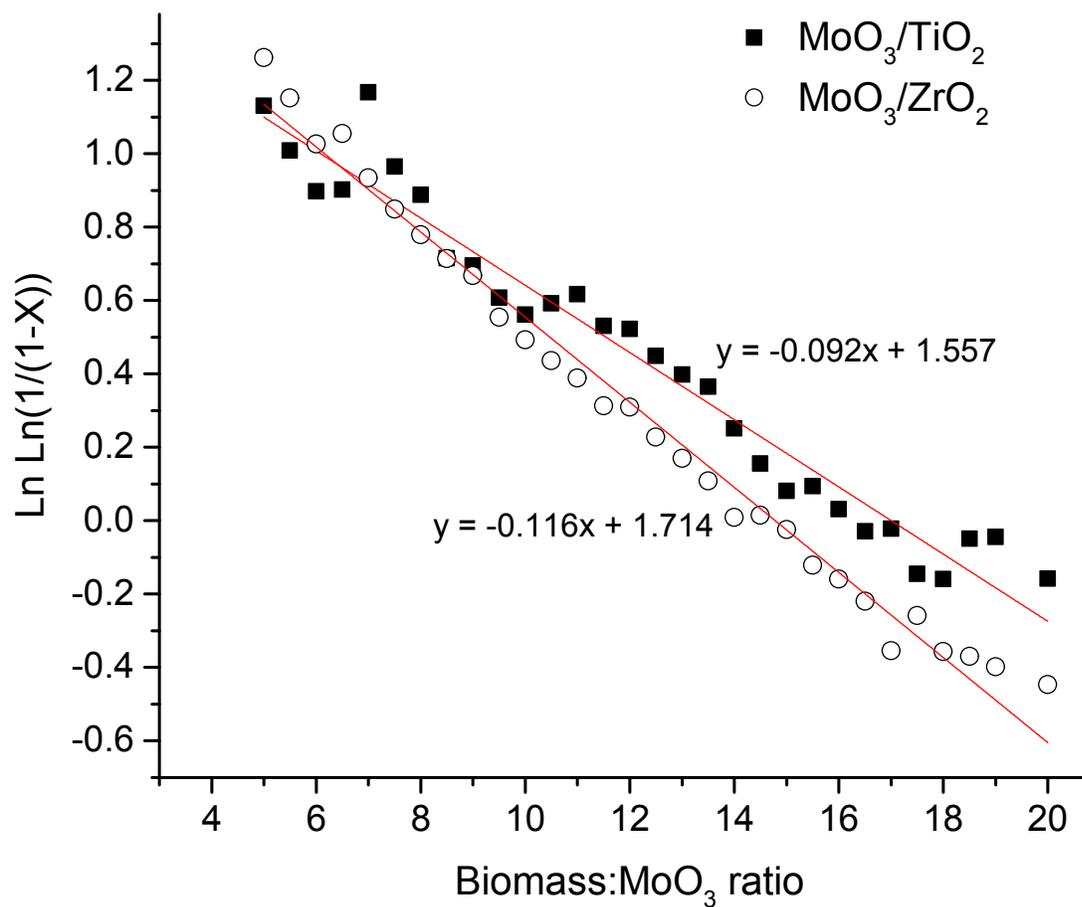
**Fig. S8** Deactivation profiles for MoO<sub>3</sub>/TiO<sub>2</sub> and MoO<sub>3</sub>/ZrO<sub>2</sub> for CFP of pine in the horizontal reactor-MBMS set up fitted to a first-order deactivation model.
