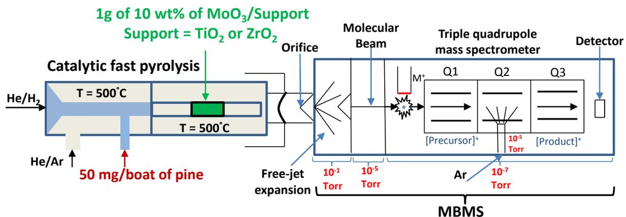
**Fig. S1** Schematic of horizontal reactor-MBMS set up.
