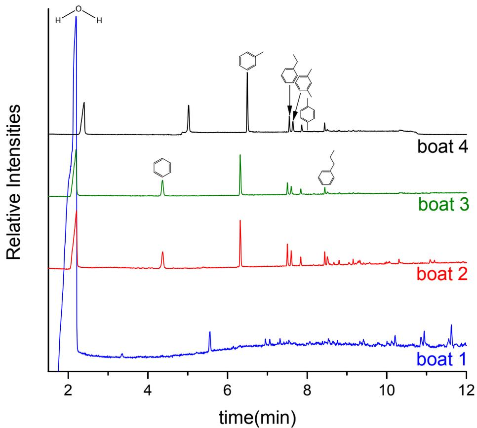
**Fig. S6** Product distribution of CFP of pine over 40 mg of  $\text{MoO}_3$  in the micropyrolyzer-GCMS set up. Reaction conditions: catalyst = 40 mg, biomass = 4 boats of 0.5 mg pine,  $T = 500^\circ\text{C}$ ,  $P_{\text{total}} = 1.013$  bar (71 vol%  $\text{H}_2$ -He). The cryo-trap temperature was set to  $-80^\circ\text{C}$  in this experiment, thereby explaining the absence of alkenes and alkanes.
