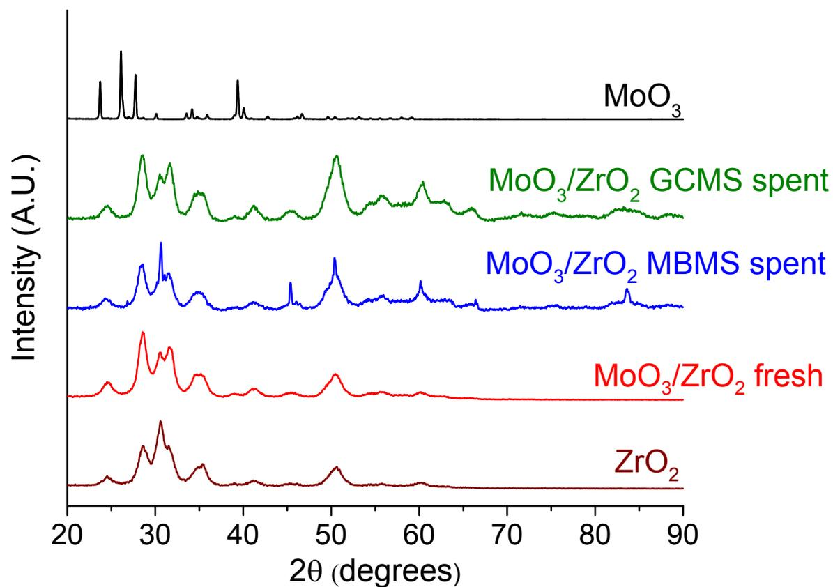
**Fig. S7** Normalised PXRD patterns of the fresh and spent MoO<sub>3</sub>/ZrO<sub>2</sub> catalysts in comparison with fresh ZrO<sub>2</sub> and MoO<sub>3</sub> samples. The spent MoO<sub>3</sub>/ZrO<sub>2</sub> samples from both reactor systems were derived after experiments shown in Fig. 3(b) and S3.
