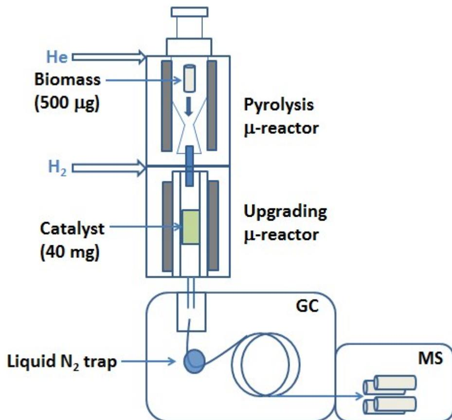
**Fig. S2** Schematic of tandem micropyrolyzer-GCMS set up
