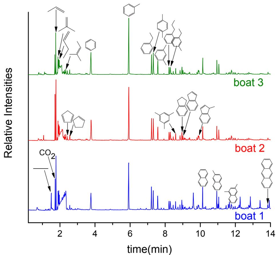
**Fig. S3** Product distribution of CFP of pine over 40 mg of 10 wt% MoO<sub>3</sub>/ZrO<sub>2</sub> in the micropyrolyzer-GCMS set up. Reaction conditions: catalyst = 40 mg, biomass = 3 boats of 0.5 mg pine, T = 500°C, P<sub>total</sub> = 1.013 bar (71 vol% H<sub>2</sub>-He)
