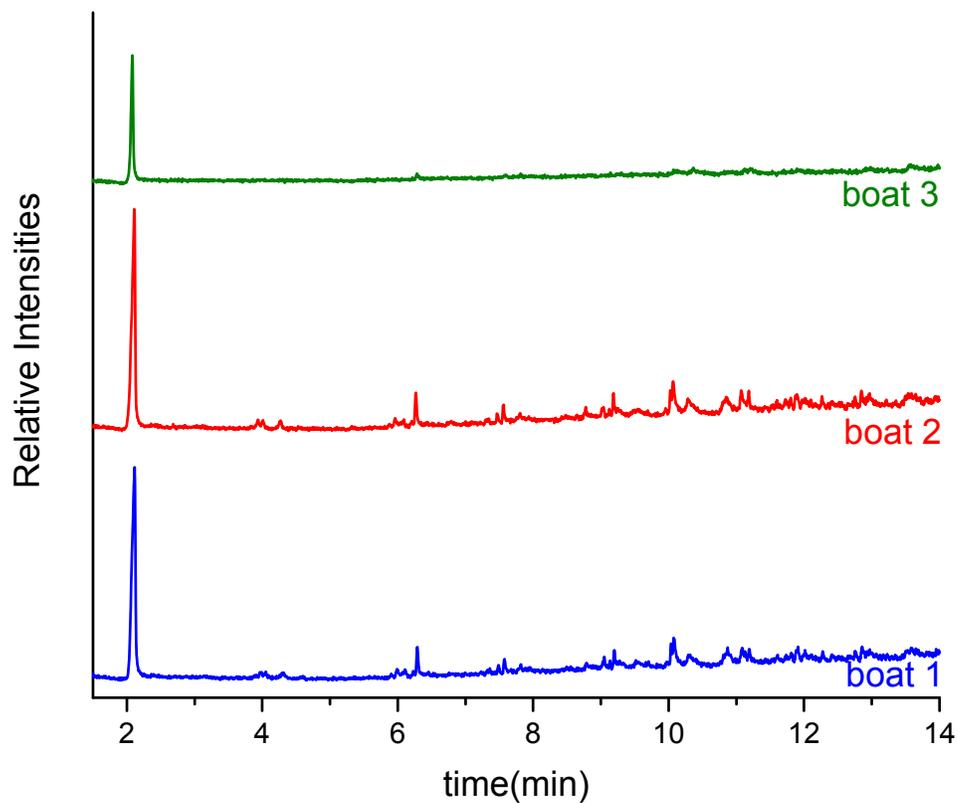
**Fig. S5** GCMS chromatograms of the CFP of 3 pine boats over 40 mg of bare  $\text{ZrO}_2$  support in the microreactor-GCMS set up. The  $\text{ZrO}_2$  support shows negligible catalytic activity under the reaction conditions investigated. Reaction conditions: catalyst = 40 mg of  $\text{ZrO}_2$ , biomass = 3 boats of 0.5 mg pine,  $T = 500^\circ\text{C}$ ,  $P_{\text{total}} = 1.013$  bar (71 vol%  $\text{H}_2$ -He)
