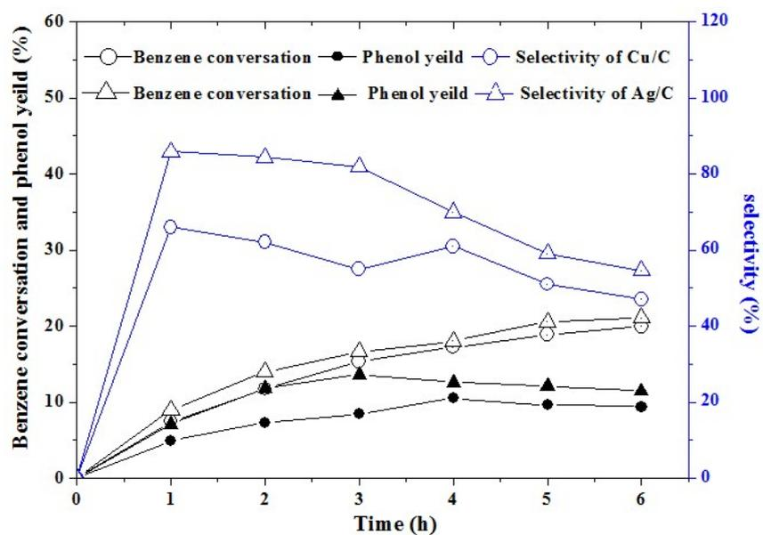
Fig. S7. Catalytic HOB by the carbon support bimetallic Cu-Ag NPs (Catalyst: Cu/C, Ag/C; solvent: CH<sub>3</sub>COOH; temperature: 323 K).
