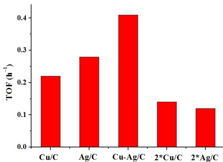
Fig. S9. The TOF value of different catalyst in catalytic HOB (Catalyst: Cu/C, Ag/C, Cu-Ag/C; solvent:  $\text{CH}_3\text{COOH}$ ; temperature: 323K; reaction time: 2h).
