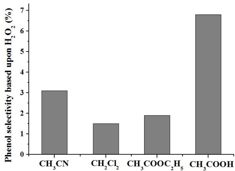
Fig. S6. The phenol selectivity based upon H<sub>2</sub>O<sub>2</sub> for Cu-Ag/C in catalytic HOB at different solvent (Catalyst: Cu-Ag/C; temperature: 323 K; reaction time: 2 h).
