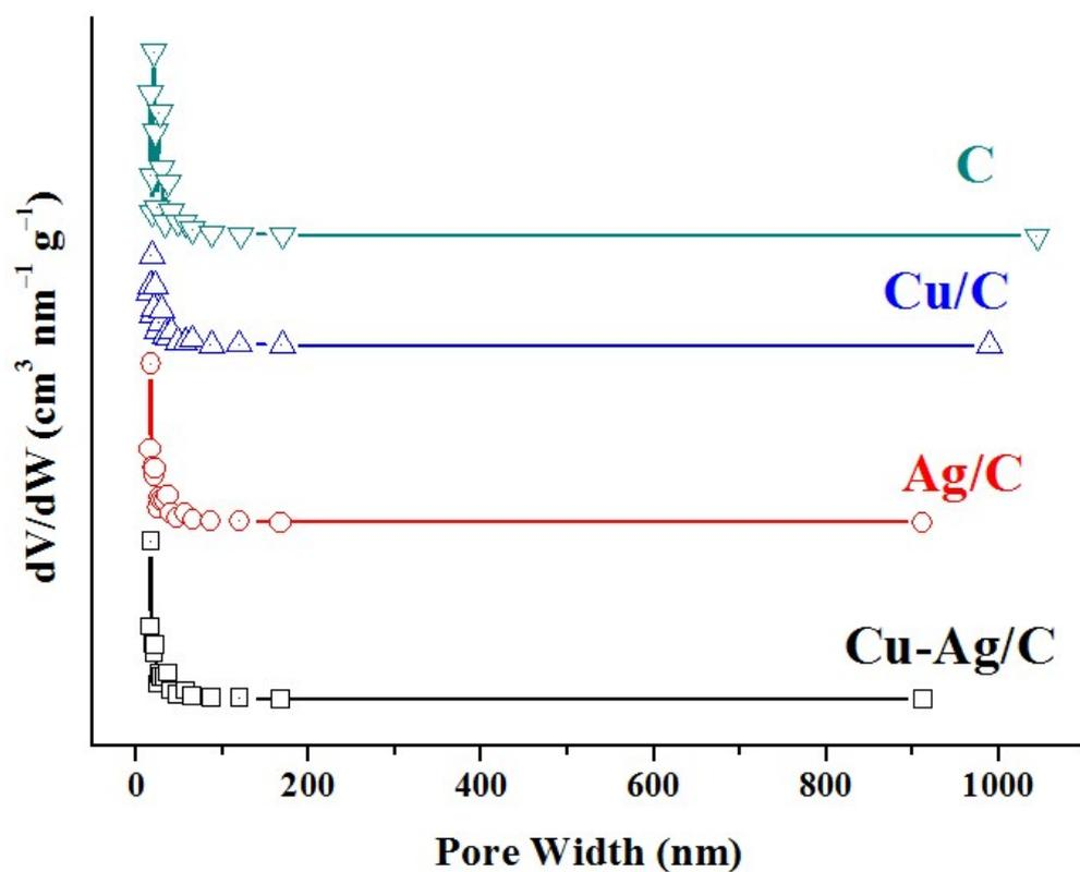
Fig. S1 The adsorption/desorption isotherms and size distribution of Ag-Cu/C, Cu/C, Ag/C and C.
