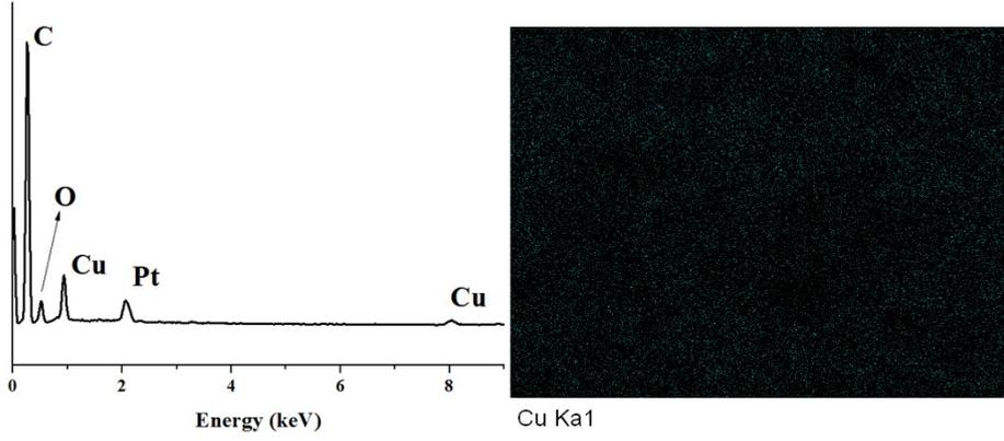
Fig.S3. SEM/EDX/mapping scanning of Cu/C.
