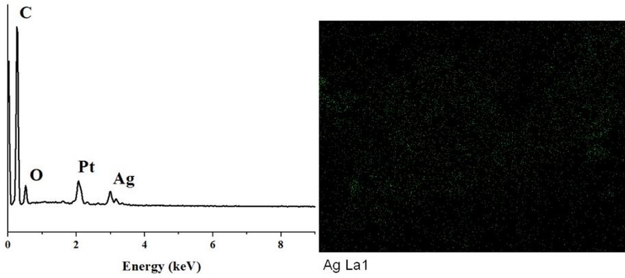
Fig.S4. SEM/EDX/mapping scanning of Ag/C.
