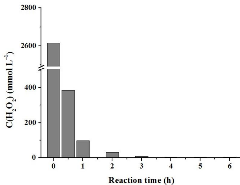
Fig. S8. The amount of H<sub>2</sub>O<sub>2</sub> in catalytic HOB of Cu-Ag/C (Catalyst: Cu-Ag/C; solvent: CH<sub>3</sub>COOH; temperature: 323 K)
