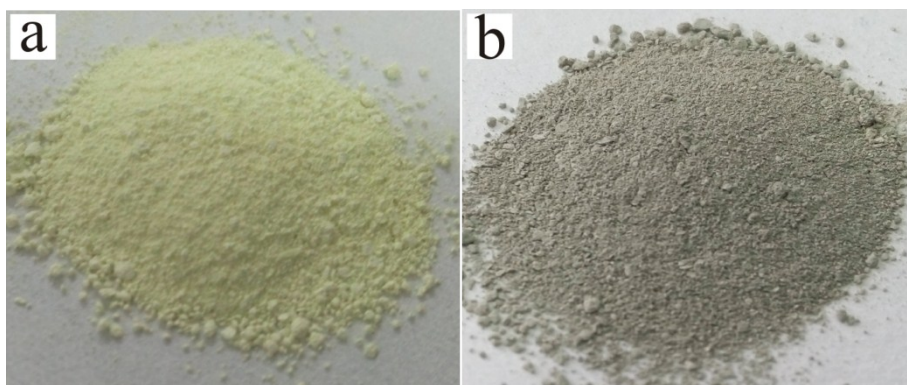
Fig. S7 (a) Photograph of \text{WO}_3 powder, (b) 1 wt.% Ru supported on \text{WO}_3 nanosheets powder.
