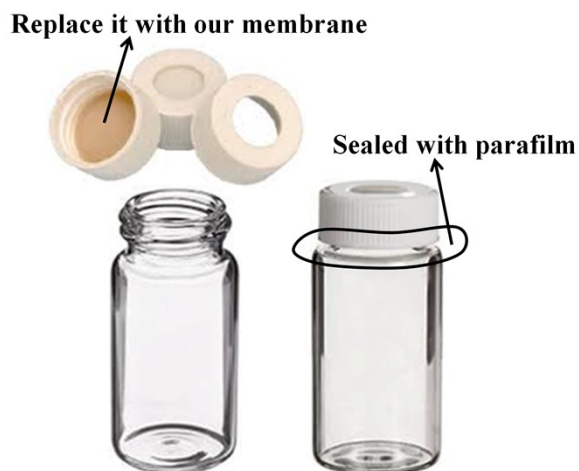
Figure S2. Water vapor transmittance (WVT) test set up.
