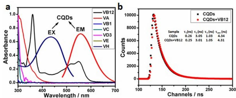
**Fig. S13** Sensing principle of the CQDs-based probe for VB12. (a) The UV-Vis absorption spectra of all vitamins and the fluorescence excitation and emission spectra of CQDs; (b) Time-resolved decay of the CQDs in the presence and absence of VB12 (1  $\mu\text{M}$ ) in BR buffer (pH 6.09). The inset table presents the lifetime value.
