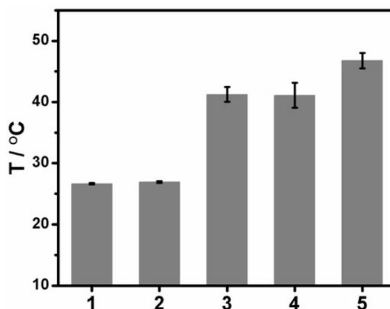
**Fig. S2** Increased temperature of exothermic system. 1, Control (water); 2, Hydroquinone + 10% H<sub>2</sub>O<sub>2</sub>; 3, 15% EDA; 4, Hydroquinone + 15% EDA; 5, *p*-Benzoquinone + 15% EDA. Hydroquinone: 100 mg; *p*-Benzoquinone: 100 mg.
