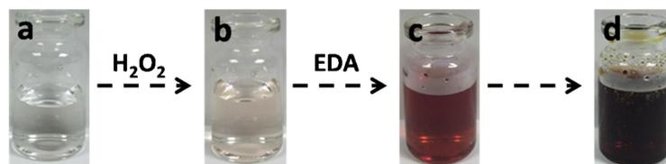
**Fig. S1** Scheme of the green synthesis routine of the CQDs. (a) The hydroquinone solution; (b) the reaction solution after adding H<sub>2</sub>O<sub>2</sub>; (c) the resulting solution after adding EDA; (d) the final CQDs solution.
