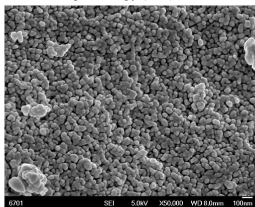
Figure S9. Scanning electron microscope (SEM) characterization of CuO-ZnO-500
