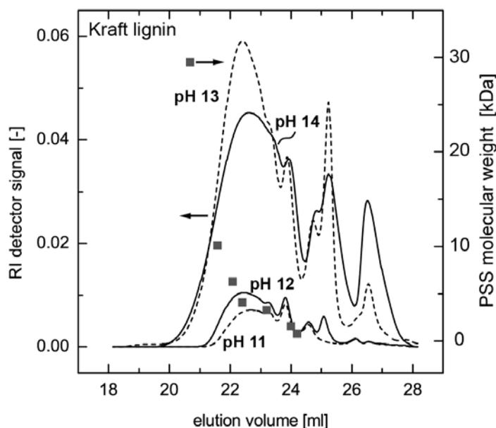
Fig SI 1 SEC Elugrams of extracted Kraft lignin for pH 11 to 14.
