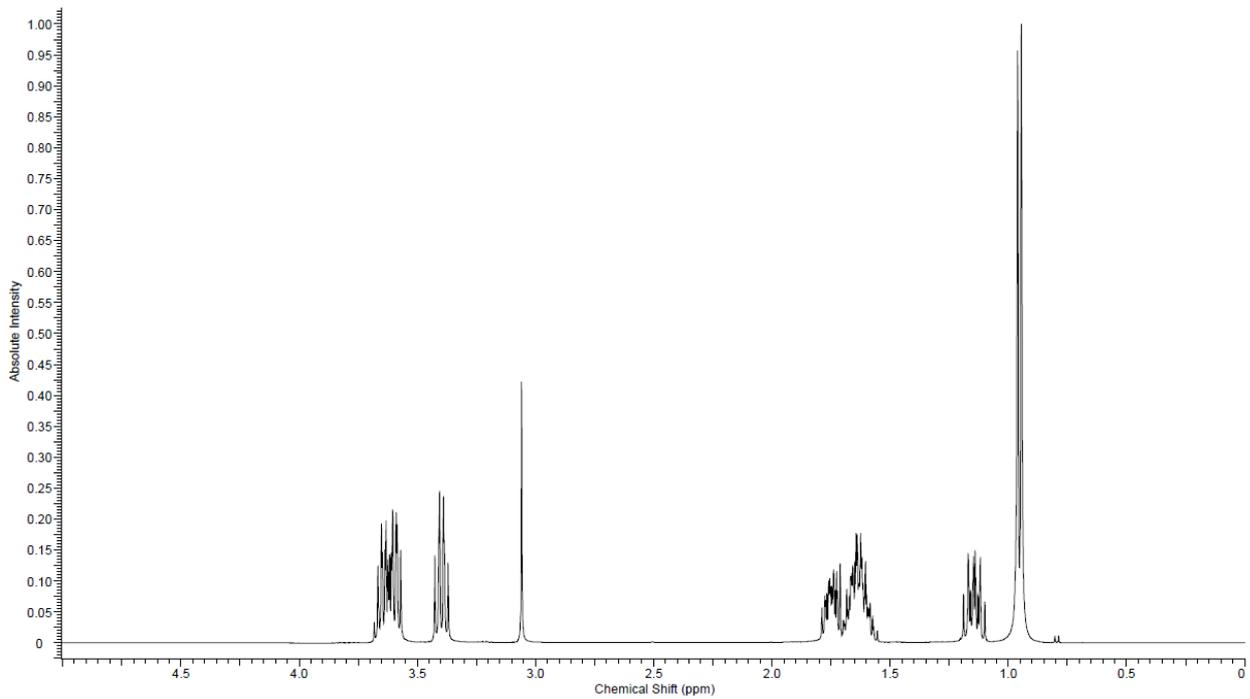
Fig SI 31H-NMR spectrum for 2-MTHF spiked with an alkaline solution
