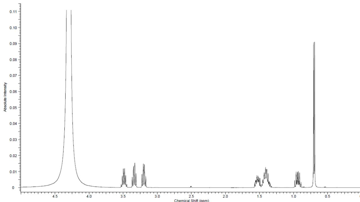
Fig SI 2 <sup>1</sup>H-NMR spectrum for an alkaline solution spiked with 2-MTHF
