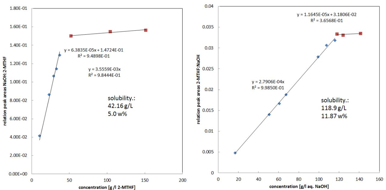
Fig SI 4 Relation of the characteristic integrated peak areas of 2-MTHF and aqueous sodium hydroxide plotted against respective concentration of the two phases. The left graph shows dissolved aqueous sodium hydroxide in 2-MTHF, the right graph 2-MTHF in aqueous sodium hydroxide. Linear regression lines with their equations are noted next to the lines.
