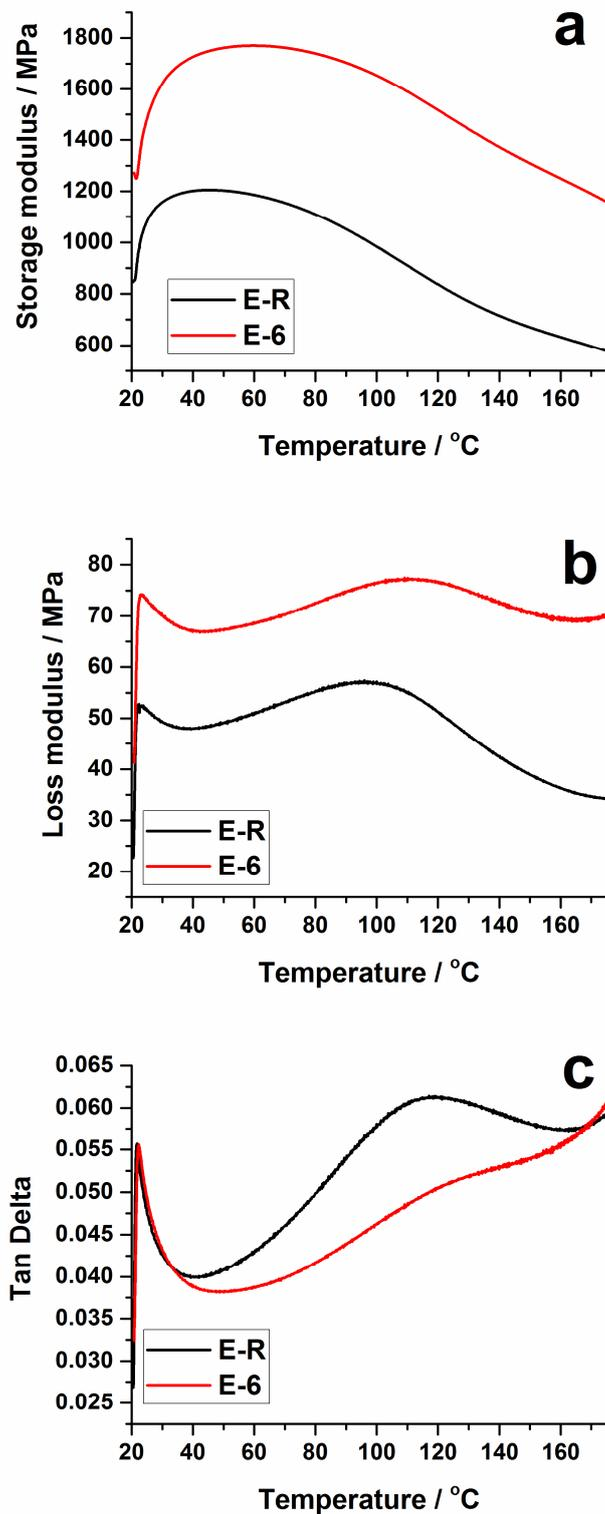
**Figure S4** (a) Storage modulus, (b) Loss modulus, and (c) Tan  $\delta$  Dynamic Mechanical Analysis (DMA) data for E-R & E-6. Measured at 1 Hz from 20 to 175°C with a heating rate of 5°C min<sup>-1</sup> on a TA Dynamic Mechanical Analysis Q800.
