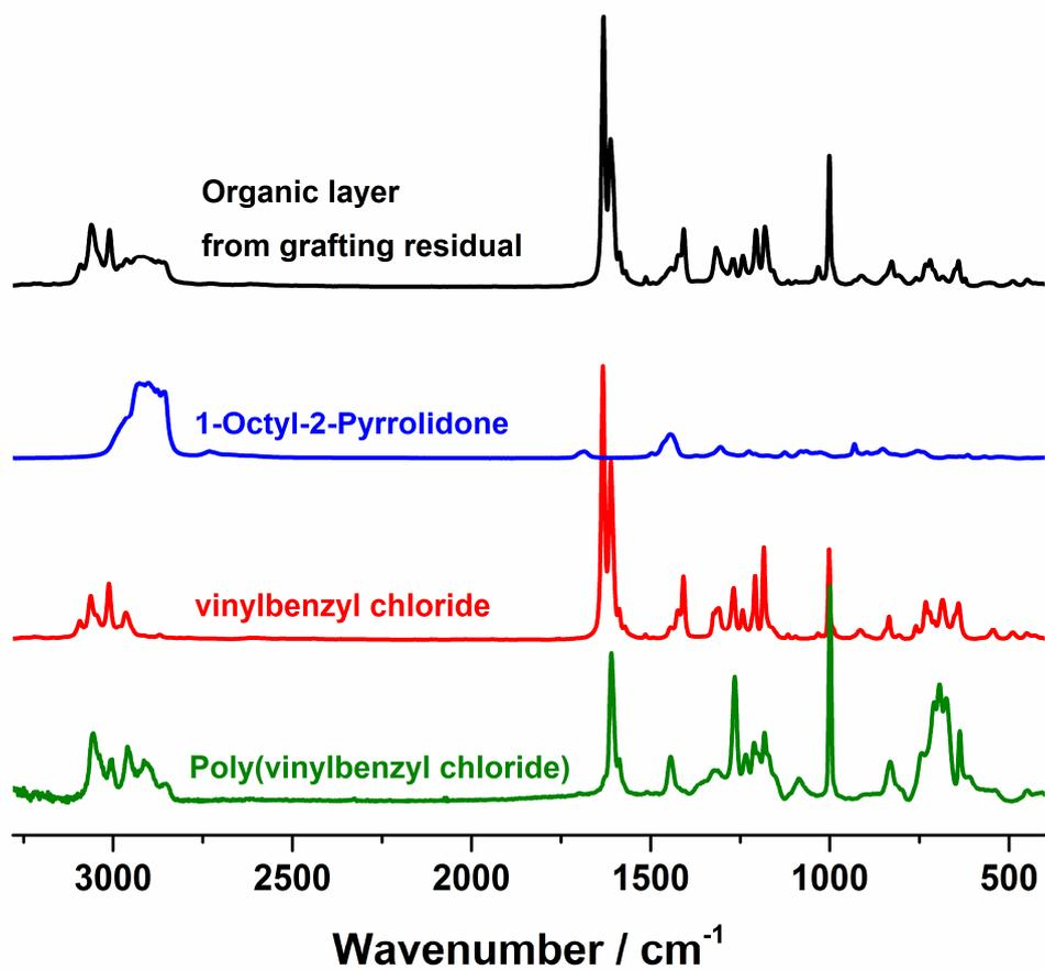
**Figure S7** The Raman spectrum ( $\lambda = 532$  nm laser) of organic layer recovered from the grafting mixture after the synthesis of AEM E-6A. The Raman spectra of vinylbenzyl chloride (VBC), poly(vinylbenzyl chloride), and 1-octyl-2-pyrrolidone are also shown.
