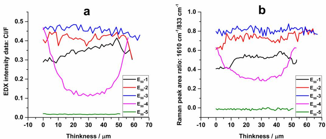
**Figure S3** (a) EDX & (b) Raman line data of the ETFE-*g*-poly(VBC) intermediate membranes for all the thicker RG-AEMs synthesised from the 50  $\mu\text{m}$  ETFE. The through-plane direction is from left to right in these line maps.
