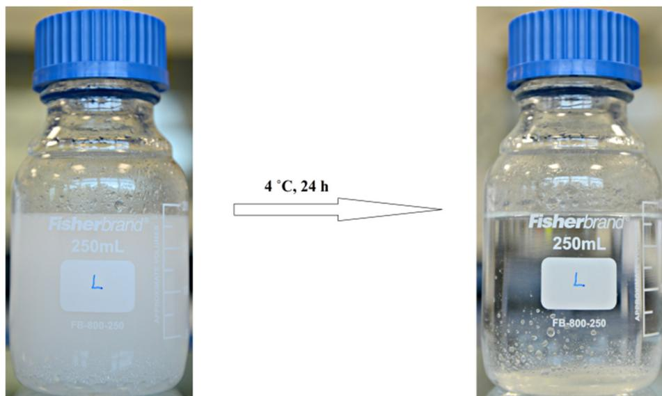
**Figure S5** The residual grafting mixture used to make AEM E-6A before (left) and after (right) storage at 4°C for 24 h.
