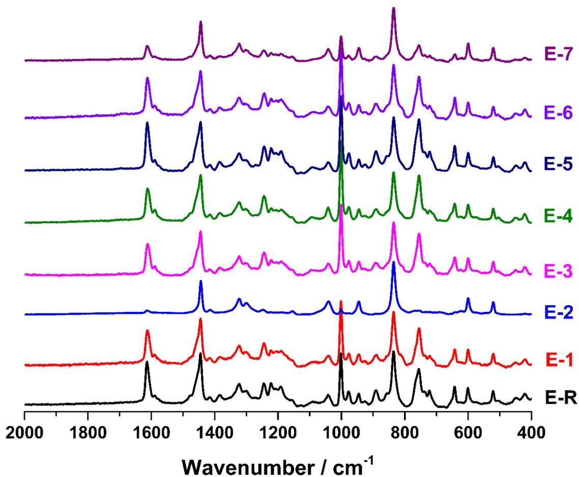
**Figure S1** The Raman spectra ( $\lambda = 780$  nm laser) of all the RG-AEMs synthesised from 25  $\mu\text{m}$  ETFE (discussed in the main article). The spectra were normalised to the intensity of the ETFE-derived peak at  $835\text{ cm}^{-1}$  for ease of visual comparison.
