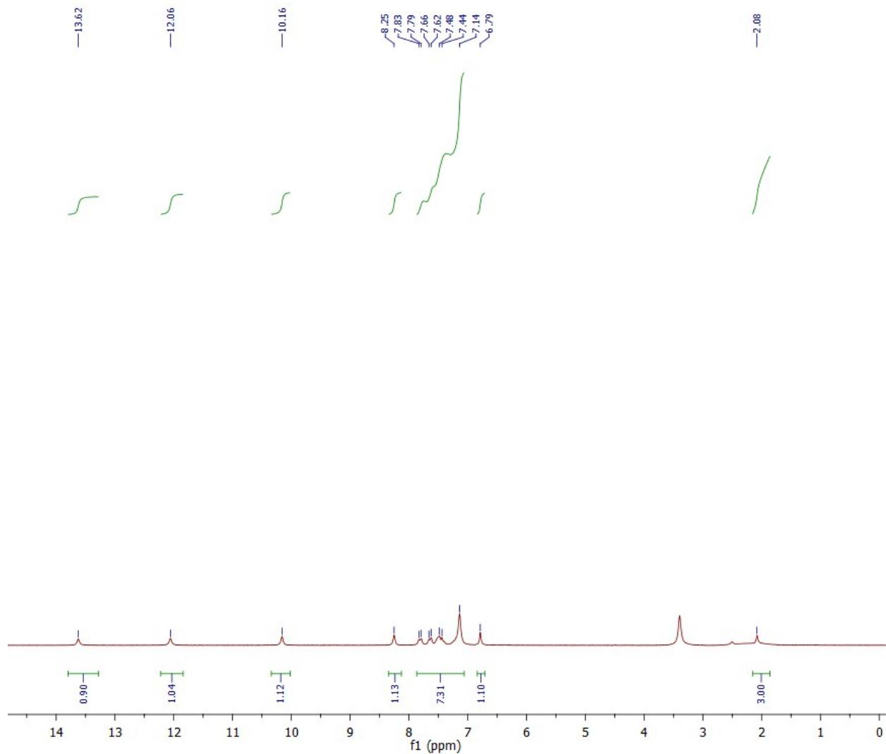
Fig. S24 <sup>1</sup>H NMR spectrum of 4l
