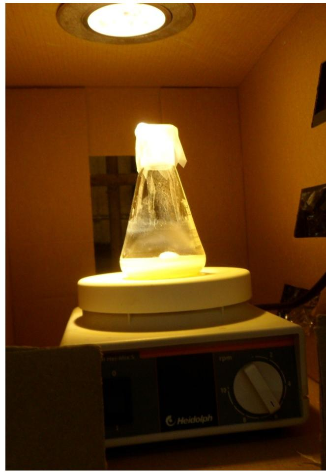
**Figure S2 :** Reaction Setup under Visible light (LED Lamp).
