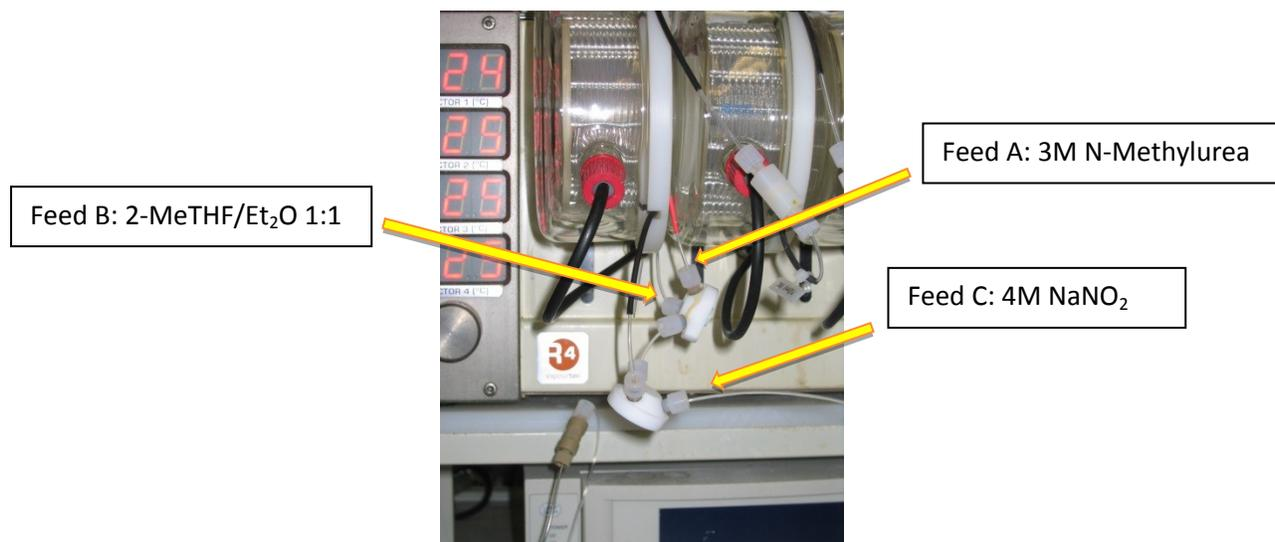
**Figure 6a: Photo of combined setup, part 2, flow synthesis of diazomethane**
