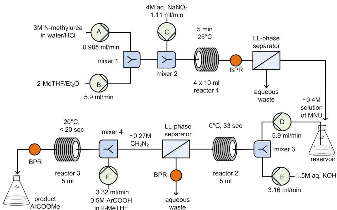
Figure 4: Photo of combined setup, part 1, flow synthesis of MNU
