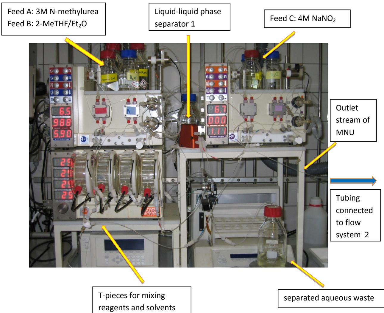
**Figure 5: T-pieces for mixing of reagents and solvent**
