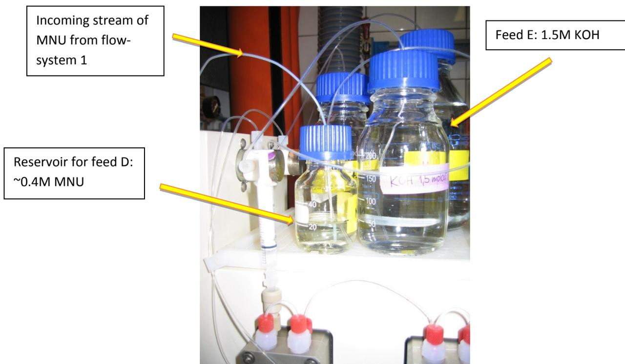
**Figure 6b: Photo of combined setup, part 2, flow synthesis of diazomethane**
