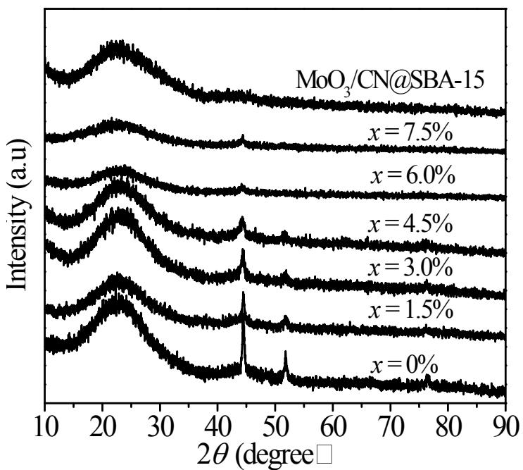
**Figure S3.** Wide-angle XRD patterns of the  $\text{Ni}-x\text{MoO}_3/\text{CN}@\text{SBA-15}$  and  $\text{MoO}_3/\text{CN}@\text{SBA-15}$  catalysts.
