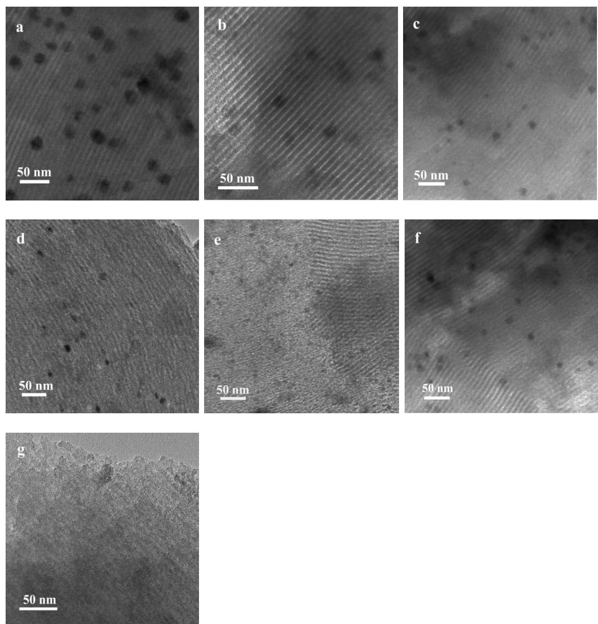
**Figure 4.** TEM images of the  $\text{Ni-}x\text{MoO}_3/\text{CN@SBA-15}$  and  $\text{MoO}_3/\text{CN@SBA-15}$  catalysts. (a)  $x = 0\%$ , (b)  $x = 1.5\%$ , (c)  $x = 3.0\%$ , (d)  $x = 4.5\%$ , (e)  $x = 6.0\%$ , (f)  $x = 7.5\%$ , and (g)  $\text{MoO}_3/\text{CN@SBA-15}$ .
