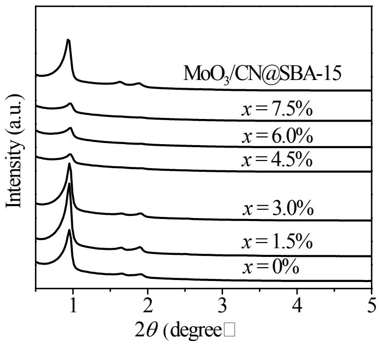
**Figure S2.** Low-angle XRD patterns of the  $\text{Ni}-x\text{MoO}_3/\text{CN}@\text{SBA-15}$  and  $\text{MoO}_3/\text{CN}@\text{SBA-15}$  catalysts.
