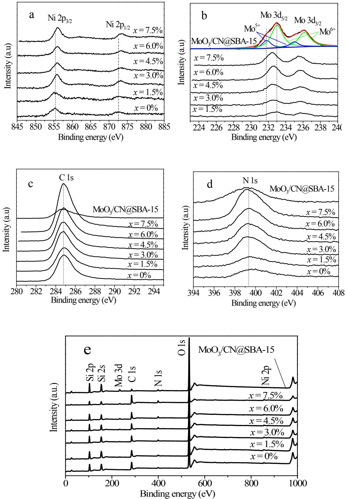
**Figure 5.** XPS spectra of the Ni- $x$ MoO<sub>3</sub>/CN@SBA-15 and MoO<sub>3</sub>/CN@SBA-15 catalysts: (a) Ni 2p, (b) Mo 3d, (c) C 1s, (d) N 1s, and (e) the survey scan.
