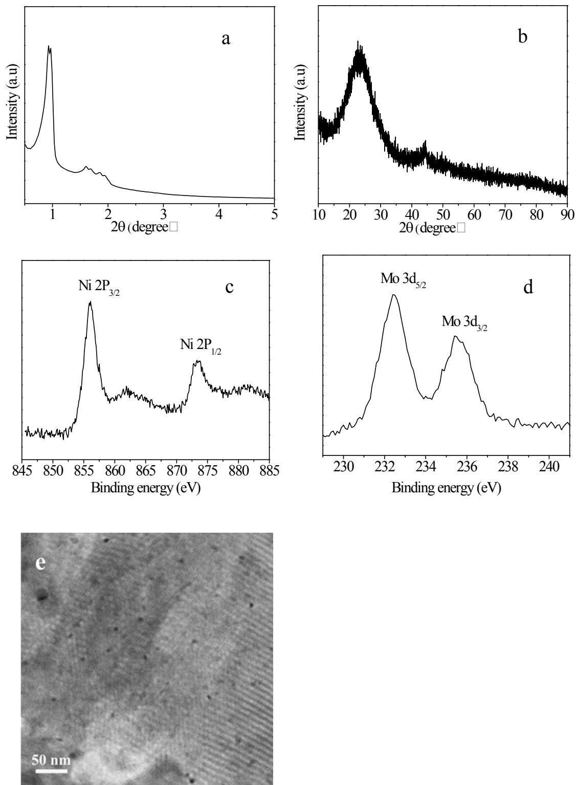
**Figure S6.** (a,b), XRD, (c,d), XPS and (e), TEM results of the spent Ni-6.0%MoO<sub>3</sub>/CN@SBA-15 catalyst for the reduction of 2,4-dichloronitrobenzene after the tenth run.
