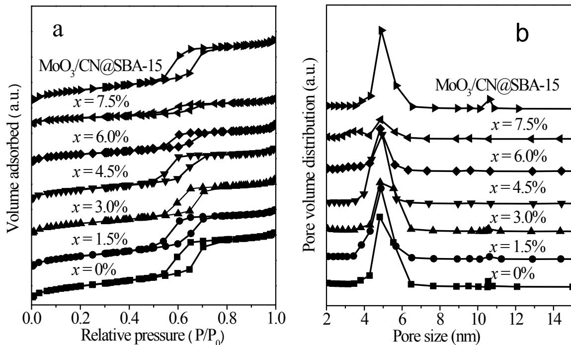
**Figure S1.** (a) N<sub>2</sub> sorption isotherms, and (b) BJH pore size distributions of the Ni- $x$ MoO<sub>3</sub>/CN@SBA-15 and MoO<sub>3</sub>/CN@SBA-15 catalysts.
