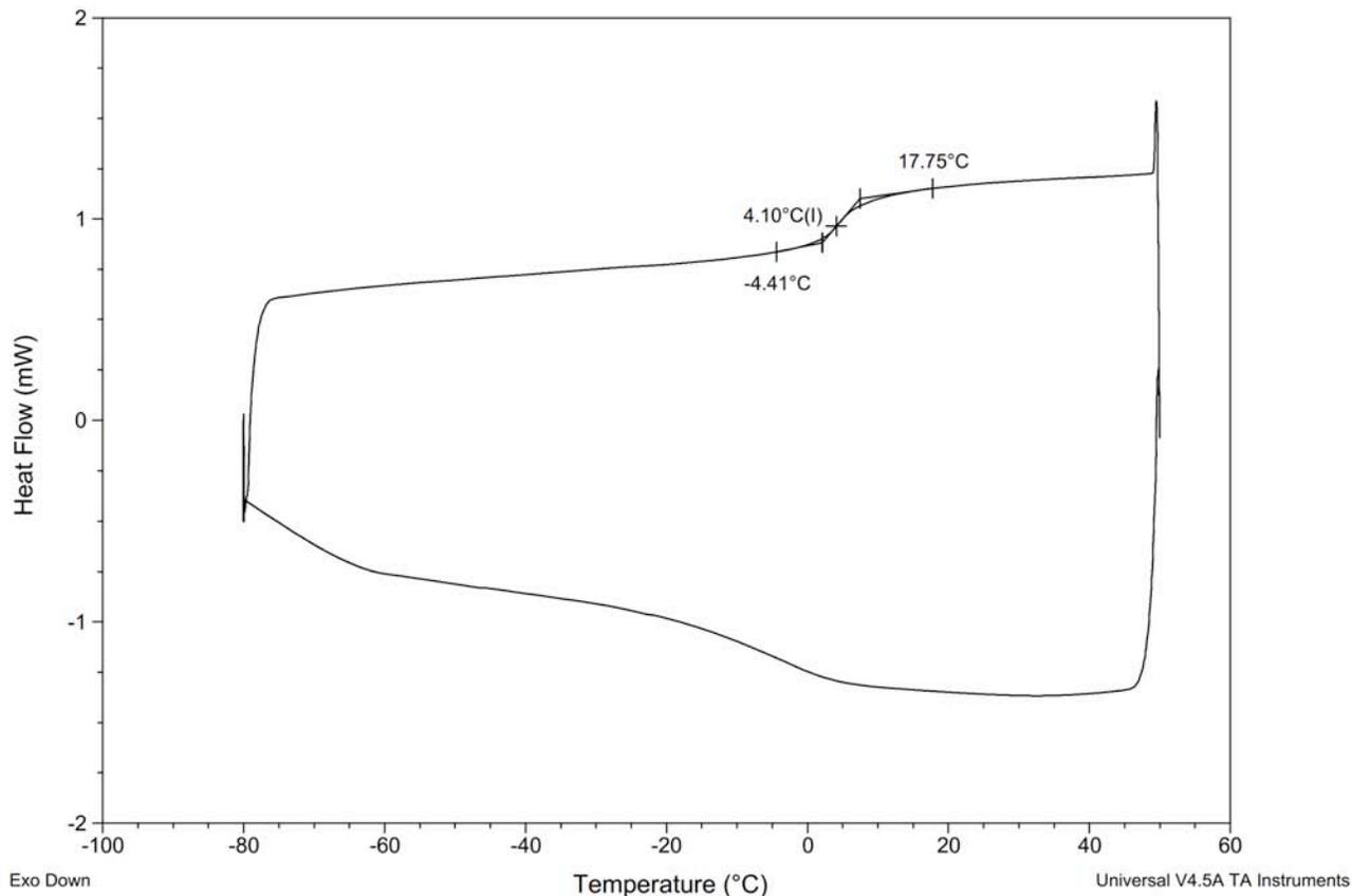
**Figure S149.** DSC Thermogram of copoly(caprolactone/ hydroxyethylsyngic acid) [50:50] at 4 hours (Table S4, entry 10).
