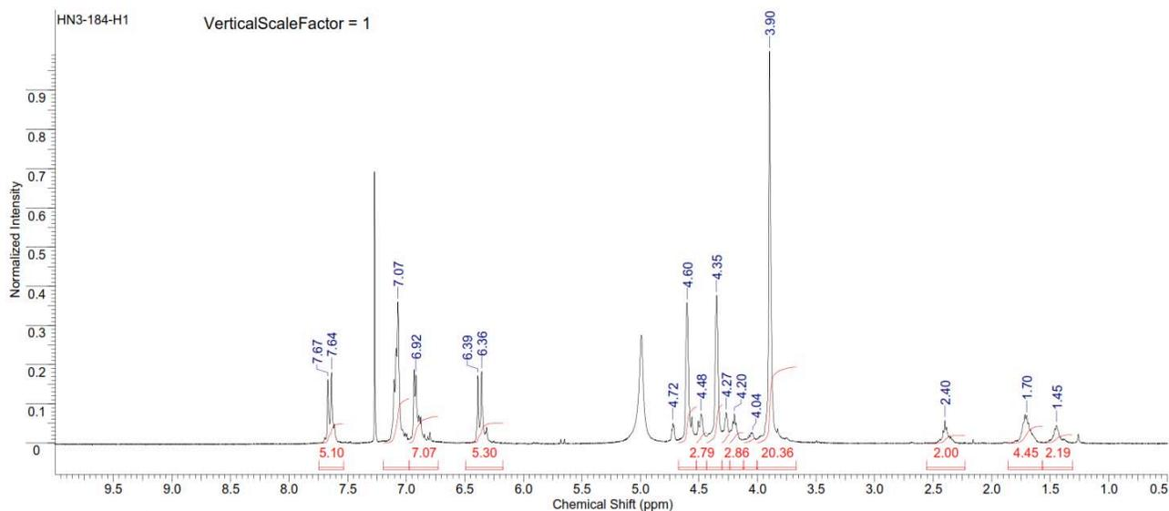
Figure S261. <sup>1</sup>H NMR spectrum of copoly(caprolactone/ hydroxyethylferulic acid) [20:80] (Table S2, entry 29).
