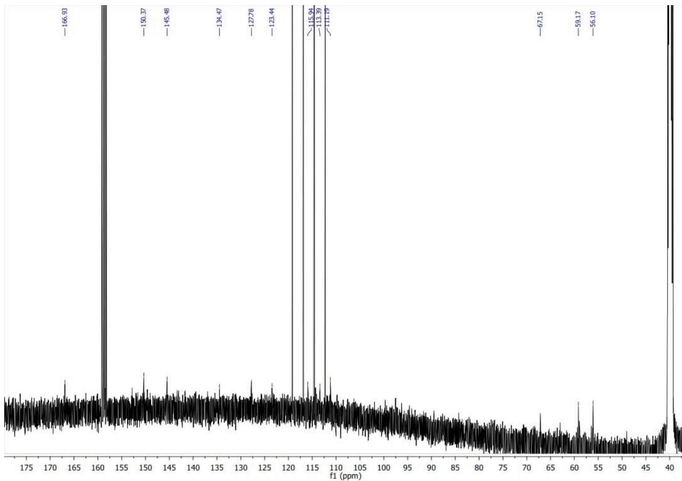
Figure S334.  $^{13}\text{C}$  NMR spectrum of polyethylene ferulate (Table S2, entry 31).
