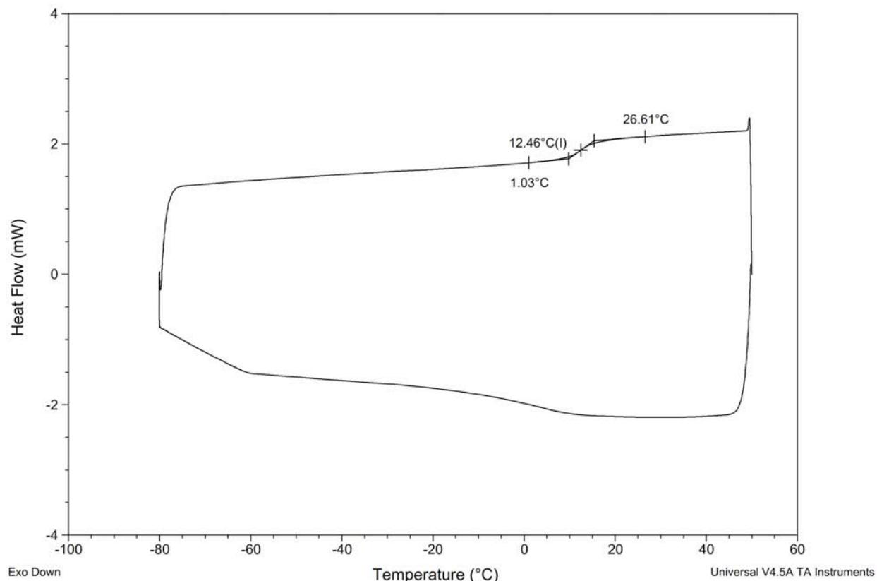
**Figure S152.** DSC Thermogram of copoly(caprolactone/ hydroxyethylsyngic acid) [50:50] at 6 hours (Table S4, entry 13).
