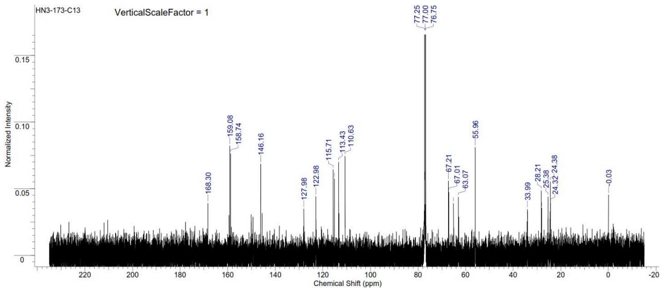
Figure S331.  $^{13}\text{C}$  NMR spectrum of copoly(caprolactone/ hydroxyethylferulic acid) [50:50] (Table S2, entry 26).
