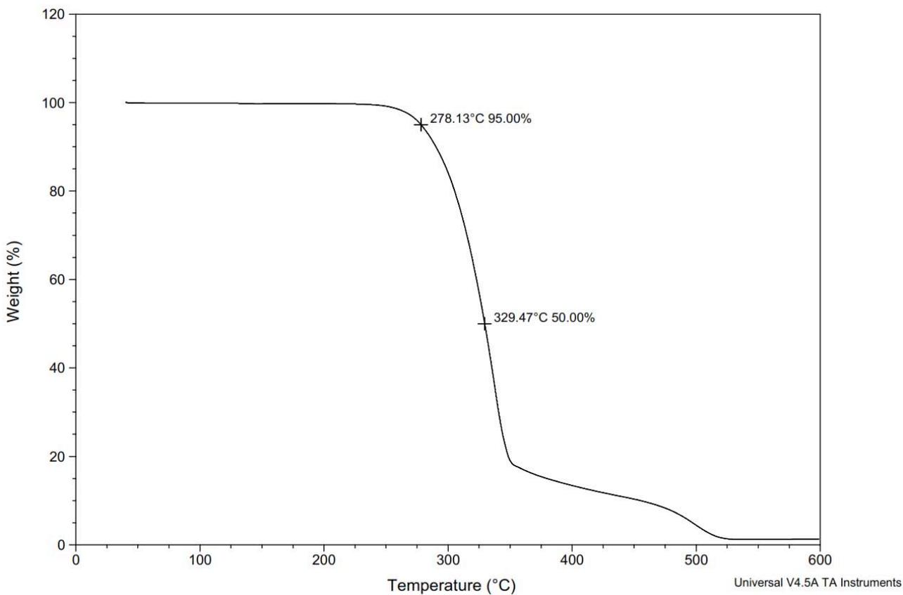
Figure S159. TGA Thermogram of copoly(caprolactone/ hydroxyethylsyngic acid) [90:10] (Table S2, entry 2).
