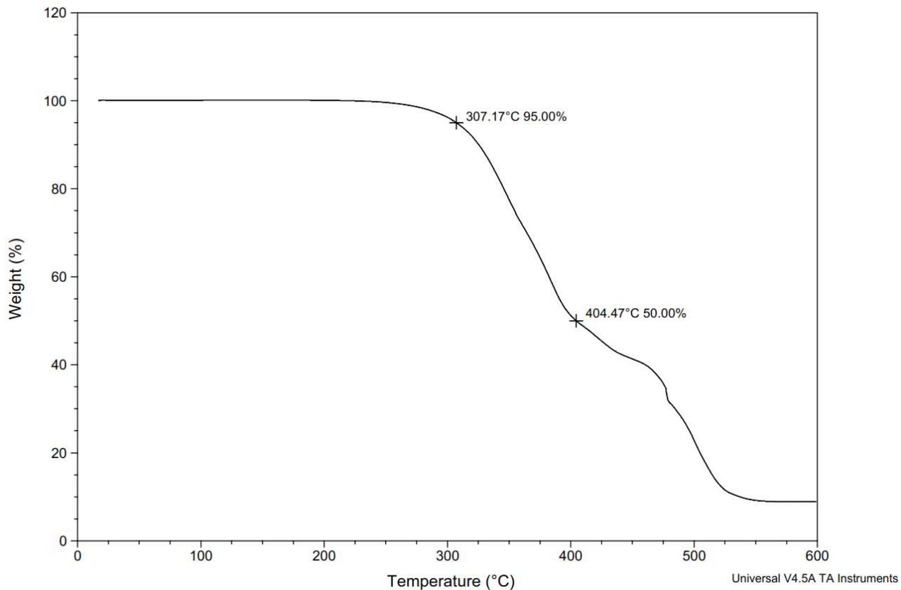
**Figure S185.** TGA Thermogram of copoly(caprolactone/ hydroxyethylferulic acid) [30:70] (Table S2, entry 28).
