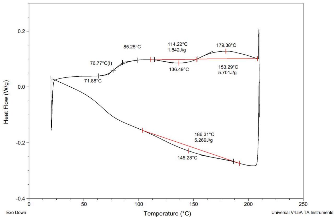
**Figure S128.** DSC Thermogram of copoly(L-lactide/ hydroxyethylvanillic acid) [40:60] (Table S3, entry 9).
