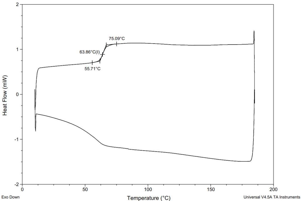
**Figure S130.** DSC Thermogram of copoly(L-lactide/ hydroxyethylferulic acid) [90:10] (Table S3, entry 12).
