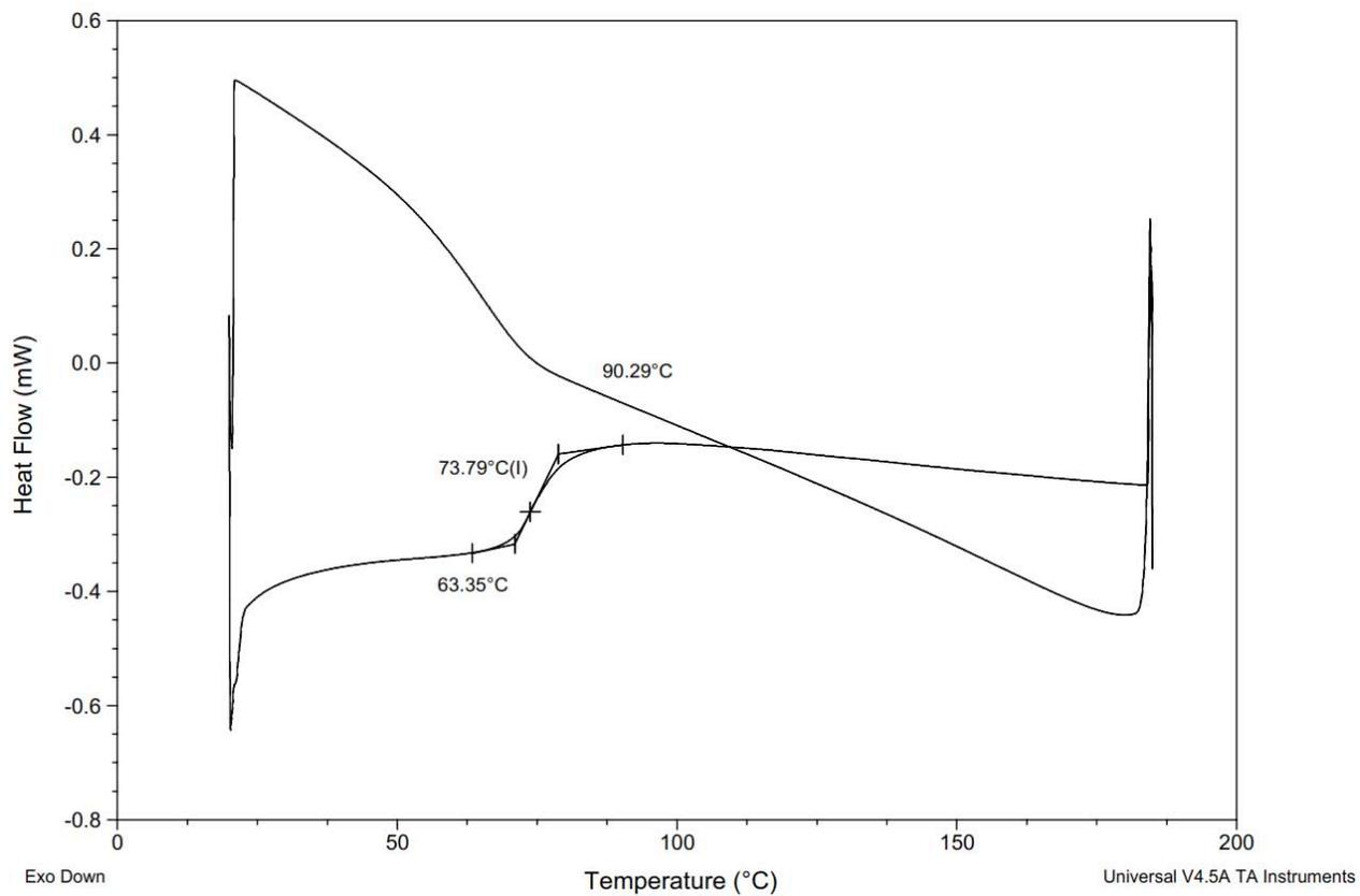
**Figure S138.** DSC Thermogram of copoly(L-lactide/ hydroxyethylcoumaric acid) [60:40] (Table S3, entry 21).
