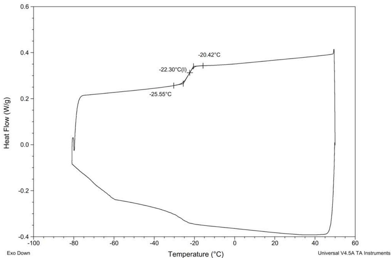
**Figure S144.** DSC Thermogram of copoly(caprolactone/ hydroxyethylsyngic acid) [50:50] at 1.5 hours (Table S4, entry 5).
