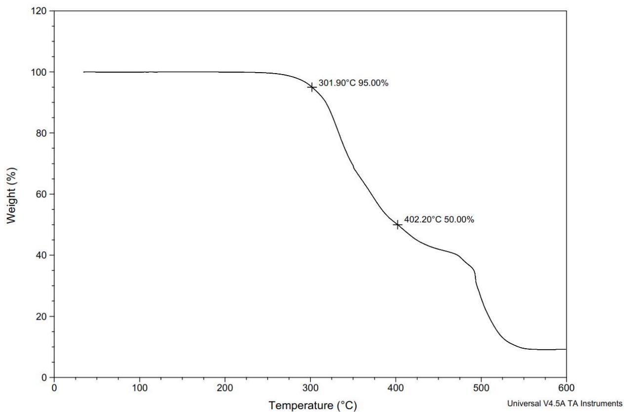
**Figure S183.** TGA Thermogram of copoly(caprolactone/ hydroxyethylferulic acid) [50:50] (Table S2, entry 26).
