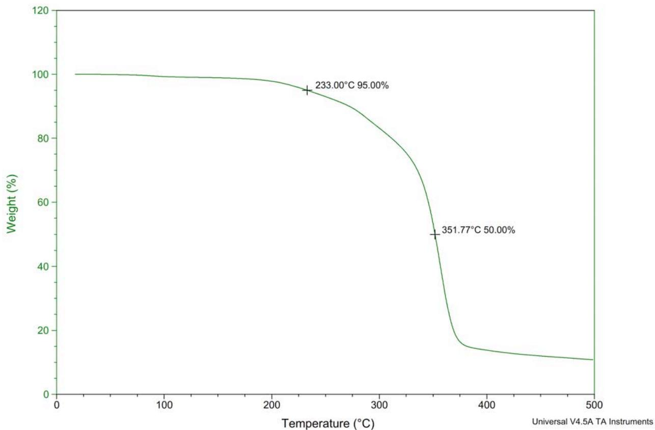
Figure S219. TGA Thermogram of copoly(caprolactone/ hydroxyethylsyngic acid) [50:50] at 3 hours (Table S4, entry 8).
