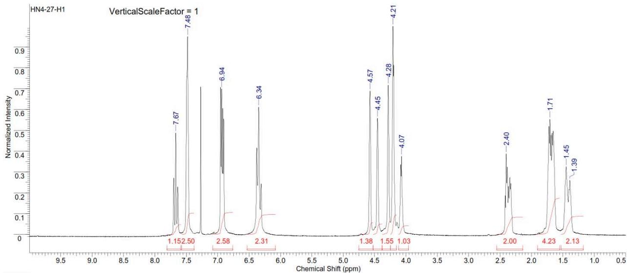
**Figure S265.**  $^1\text{H}$  NMR spectrum of copoly(caprolactone/ hydroxyethylcoumaric acid) [50:50] (Table S2, entry 33).
