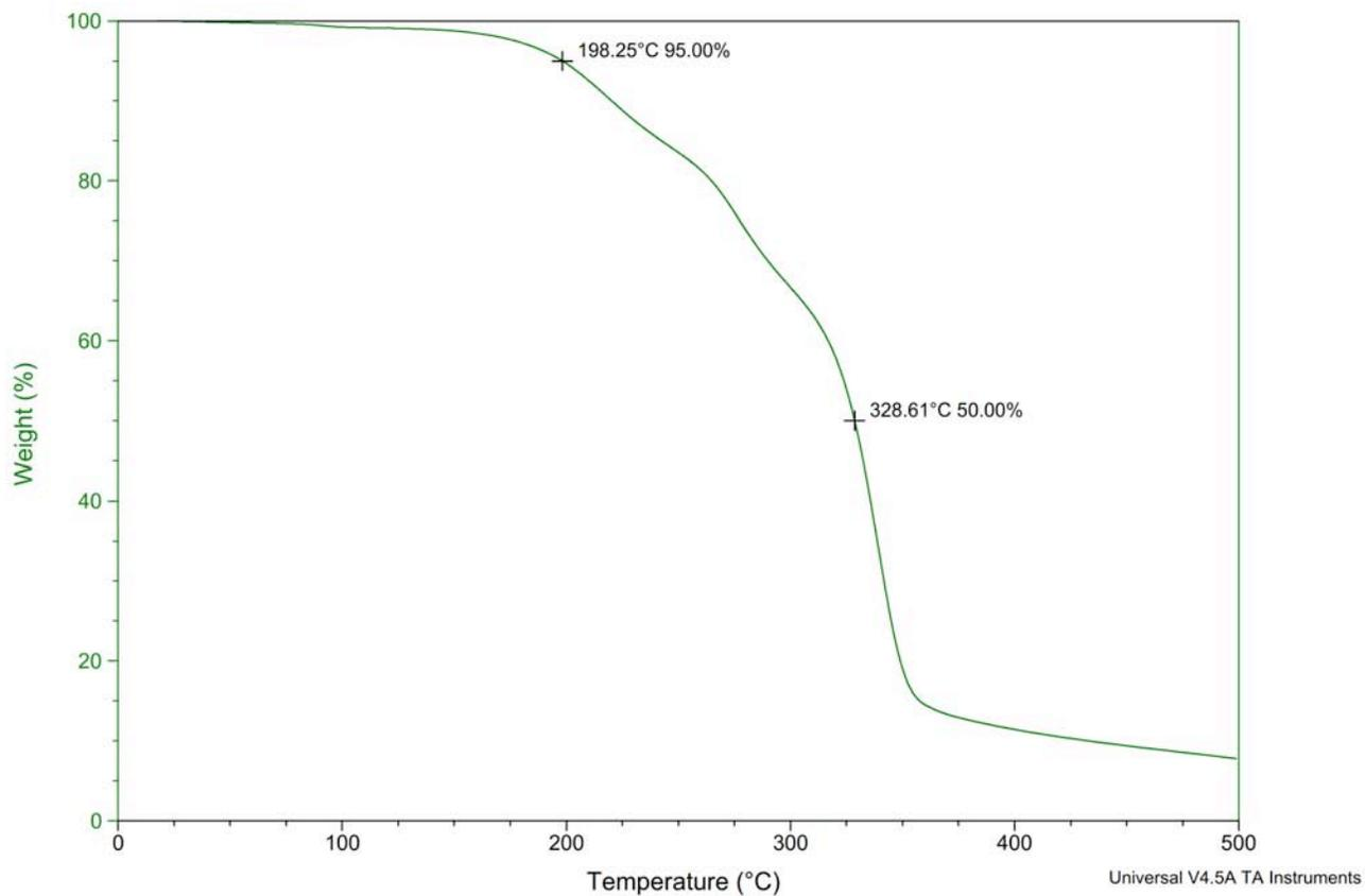
Figure S216. TGA Thermogram of copoly(caprolactone/ hydroxyethylsyngic acid) [50:50] at 1.5 hours (Table S4, entry 5).
