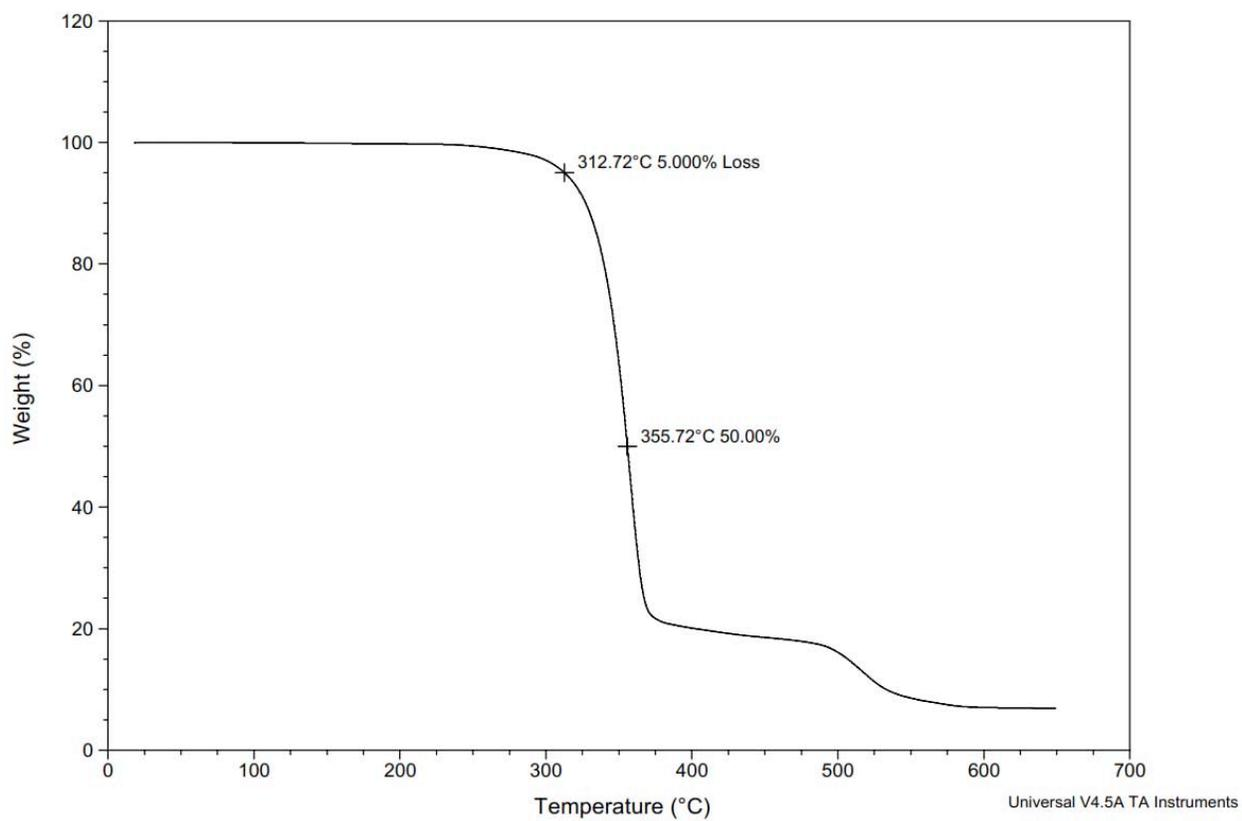
**Figure S175.** TGA Thermogram of copoly(caprolactone/ hydroxyethylvanillic acid) [30:70] (Table S2, entry 18).
