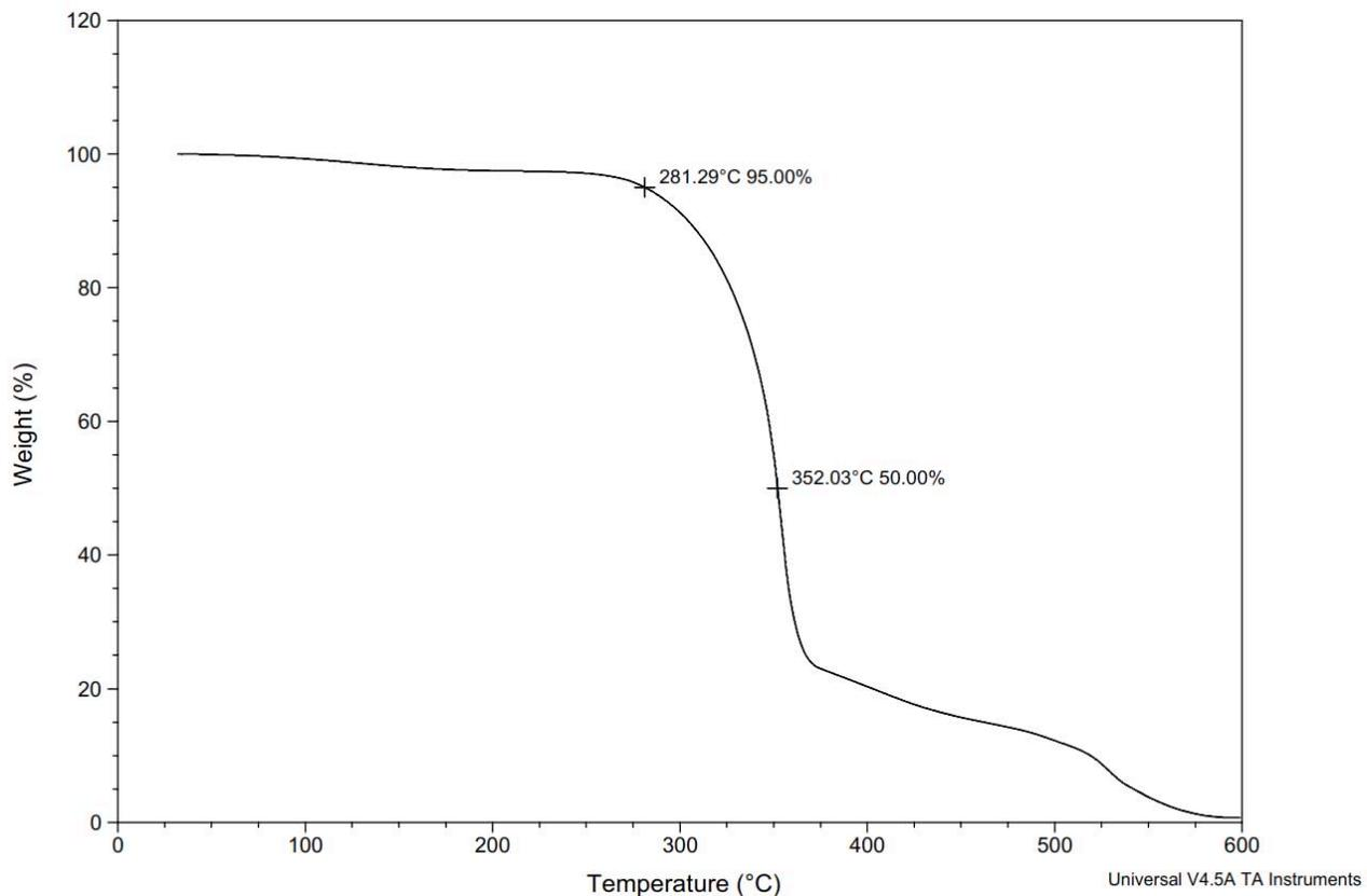
**Figure S161.** TGA Thermogram of copoly(caprolactone/ hydroxyethylsyngic acid) [70:30] (Table S2, entry 4).
