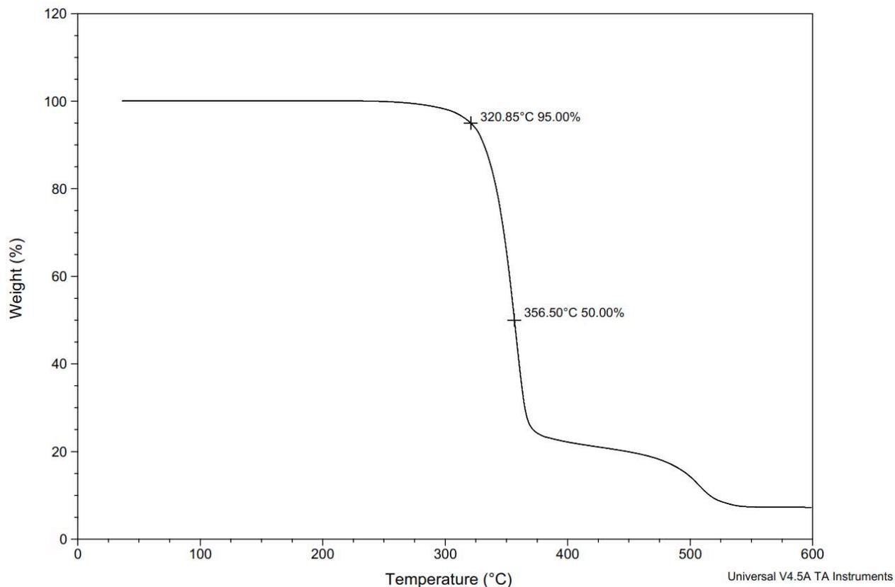
**Figure S176.** TGA Thermogram of copoly(caprolactone/ hydroxyethylvanillic acid) [20:80] (Table S2, entry 19).
