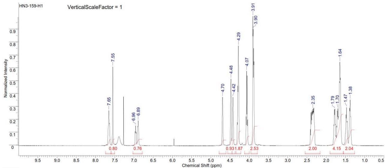
Figure S248. <sup>1</sup>H NMR spectrum of copoly(caprolactone/ hydroxyethylvanillic acid) [60:40] (Table S2, entry 15).
