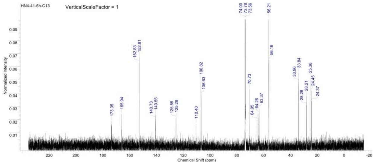
Figure S366.  $^{13}\text{C}$  NMR spectrum of copoly(caprolactone/ hydroxyethylsyringic acid) [50:50] at 6 hours (Table S4, entry 13).
