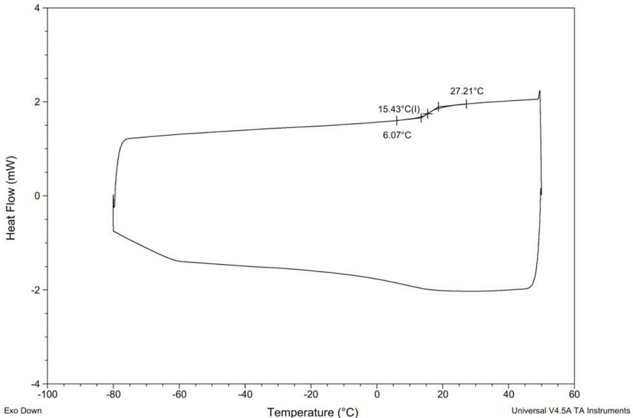
**Figure S153.** DSC Thermogram of copoly(caprolactone/ hydroxyethylsyngic acid) [50:50] at 7 hours (Table S4, entry 14).
