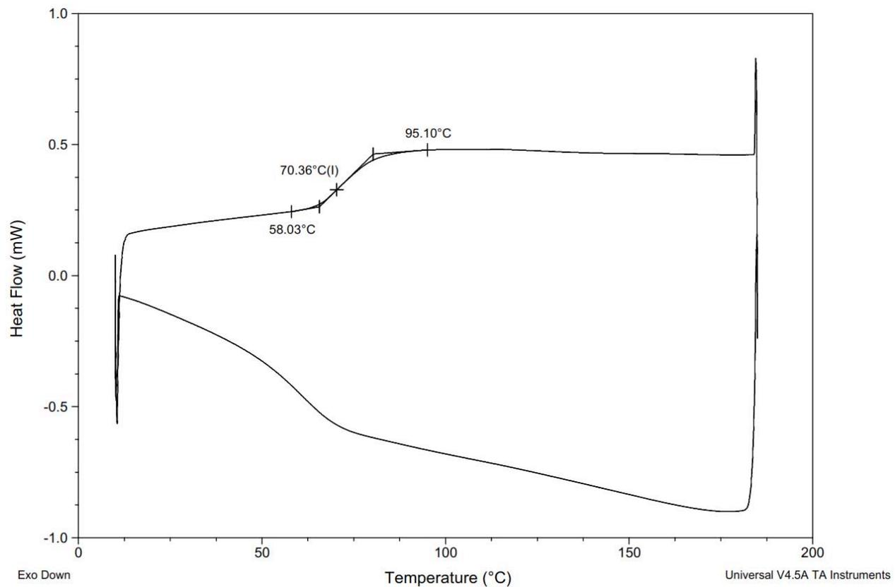
**Figure S136.** DSC Thermogram of copoly(L-lactide/ hydroxyethylcoumaric acid) [80:20] (Table S3, entry 19).
