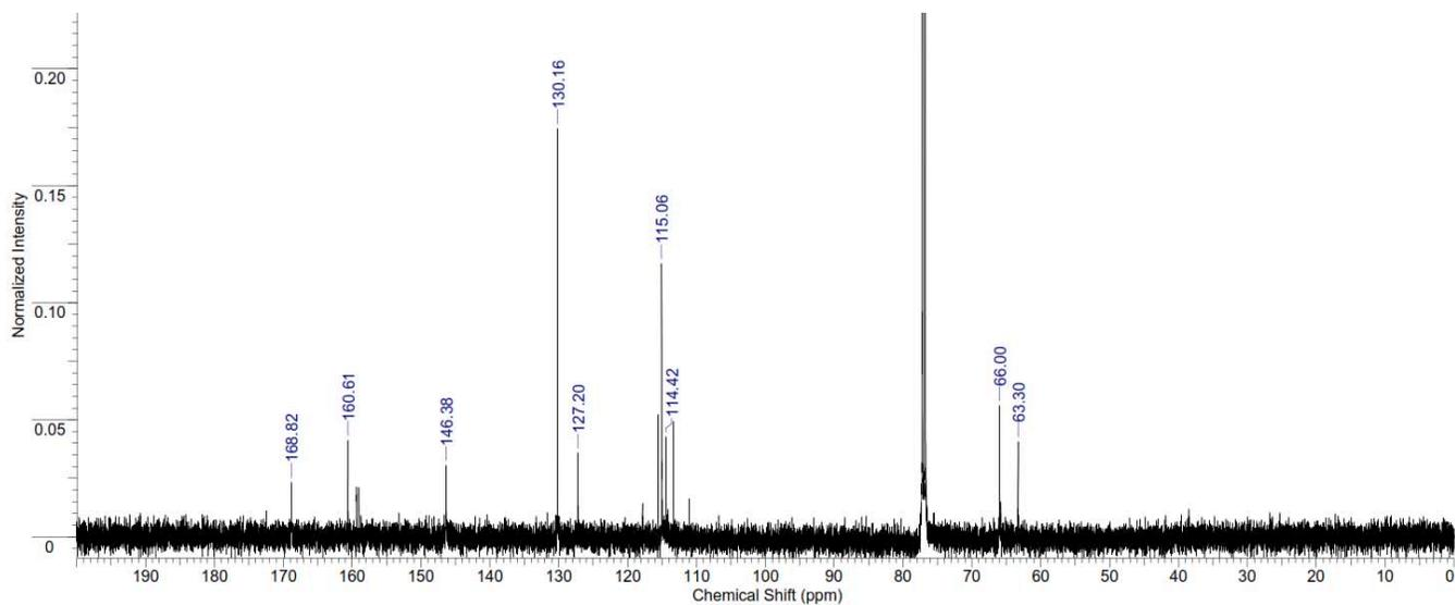
Figure S337.  $^{13}\text{C}$  NMR spectrum of polyethylene coumarate (Table S2, entry 35).
