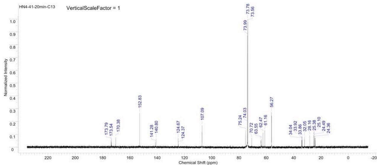
Figure S355.  $^{13}\text{C}$  NMR spectrum of copoly(caprolactone/ hydroxyethylsyringic acid) [50:50] at 20 min. (Table S4, entry 2).
