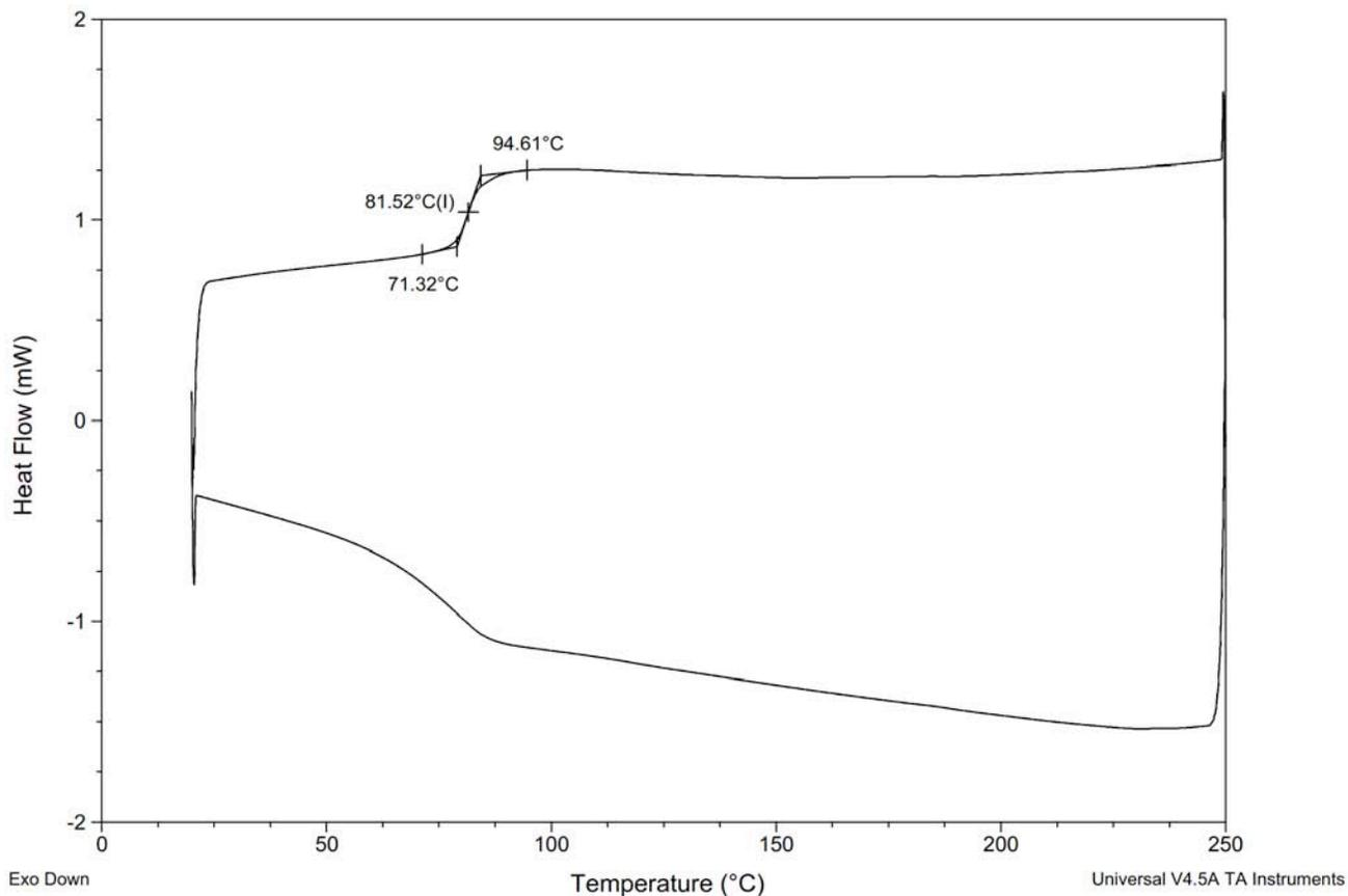
**Figure S133.** DSC Thermogram of copoly(L-lactide/ hydroxyethylferulic acid) [60:40] (Table S3, entry 15).
