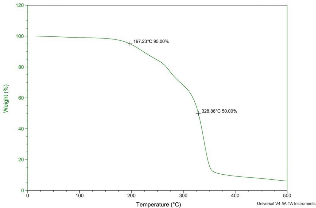
Figure S217. TGA Thermogram of copoly(caprolactone/ hydroxyethylsyngic acid) [50:50] at 2 hours (Table S4, entry 6).
