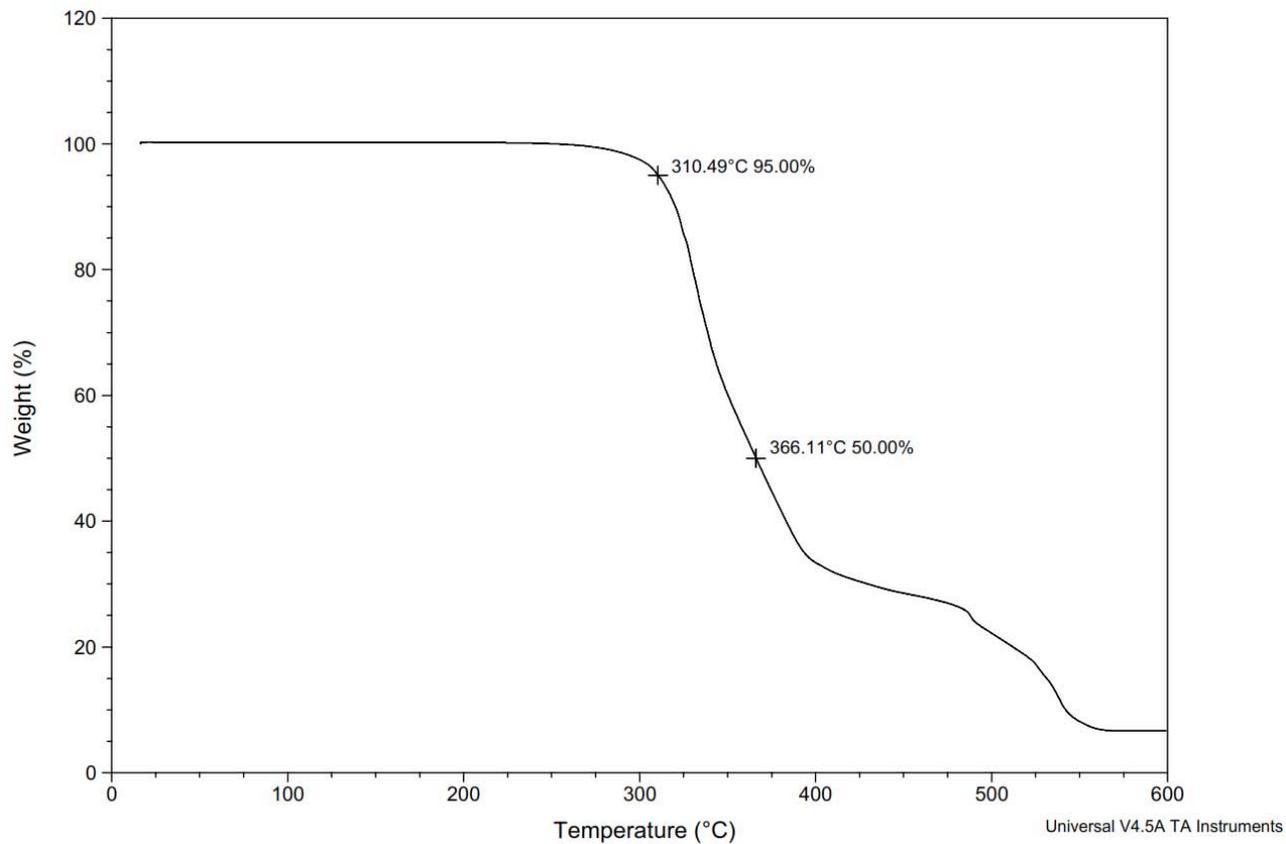
Figure S181. TGA Thermogram of copoly(caprolactone/ hydroxyethylferulic acid) [70:30] (Table S2, entry 24).
