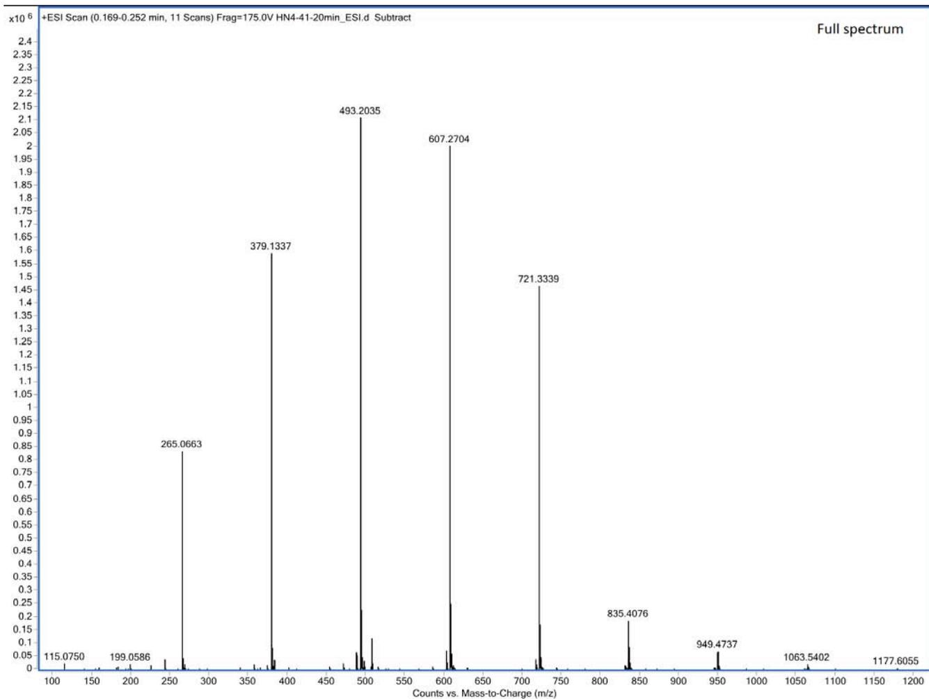
**Figure S381.** ESI spectra of copoly(caprolactone/hydroxyethylsyngic acid) [50:50] at 20 min. (Table S4, entry 2)
