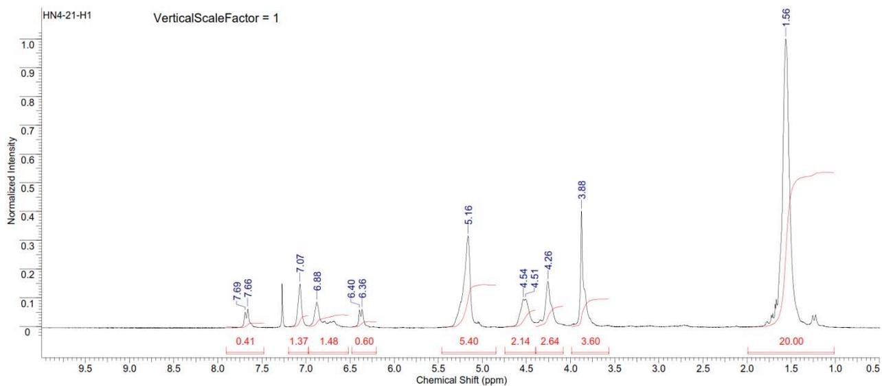
**Figure S277.**  $^1\text{H}$  NMR spectrum of copoly(L-lactide/ hydroxyethylferulic acid) [90:10] (Table S3, entry 12).
