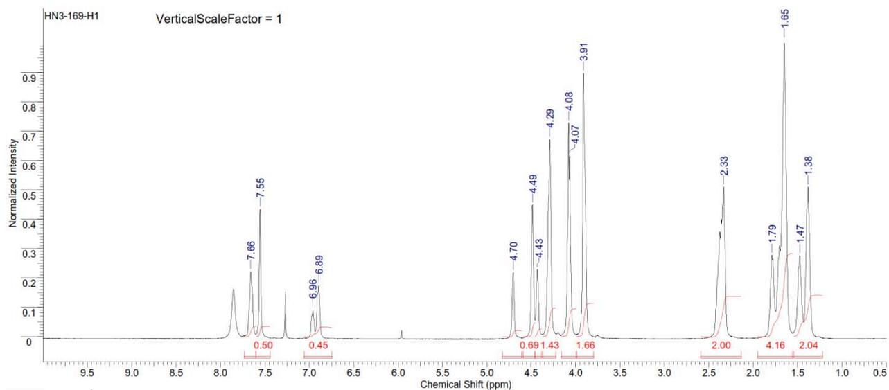
Figure S247. <sup>1</sup>H NMR spectrum of copoly(caprolactone/ hydroxyethylvanillic acid) [70:30] (Table S2, entry 14).
