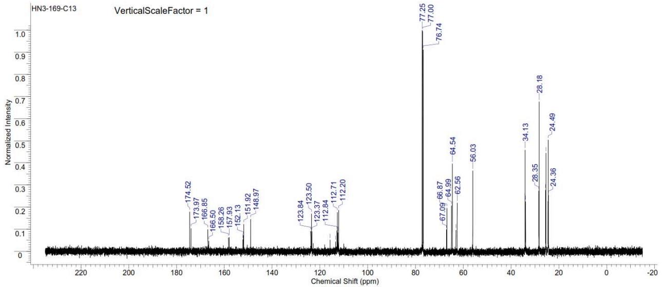
Figure S322.  $^{13}\text{C}$  NMR spectrum of copoly(caprolactone/ hydroxyethylvanillic acid) [70:30] (Table S2, entry 14).
