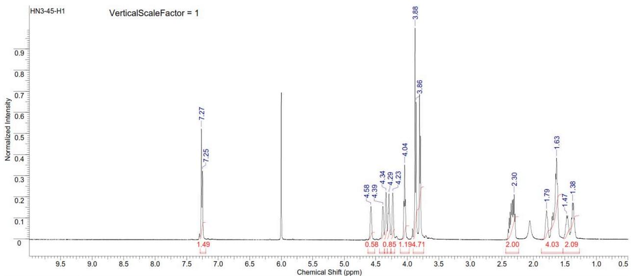
**Figure S238.**  $^1\text{H}$  NMR spectrum of copoly(caprolactone/ hydroxyethylsyngic acid) [60:40] (Table S2, entry 5).
