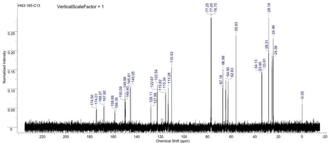
Figure S330. <sup>13</sup>C NMR spectrum of copoly(caprolactone/ hydroxyethylferulic acid) [60:40] (Table S2, entry 25).
