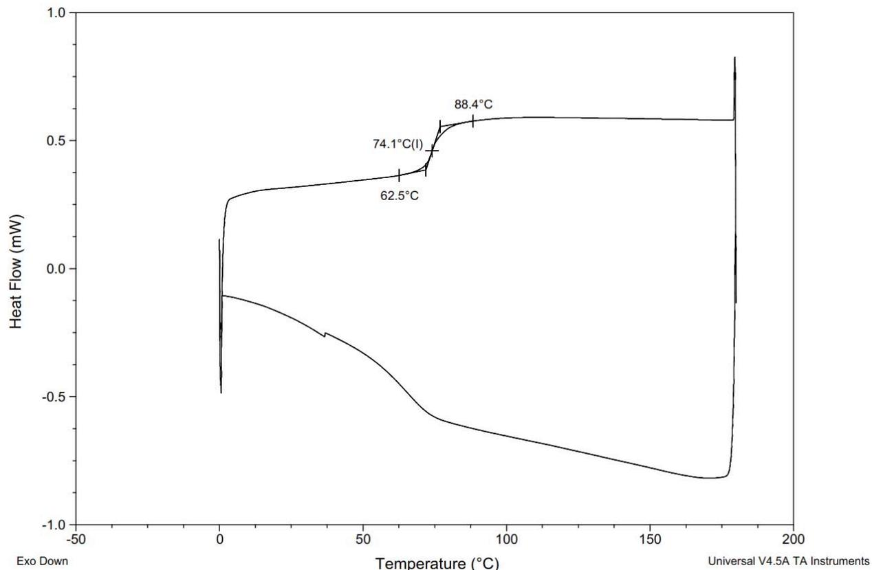
**Figure S125.** DSC Thermogram of copoly(L-lactide/ hydroxyethylsyringic acid) [20:80] (Table S3, entry 5).
