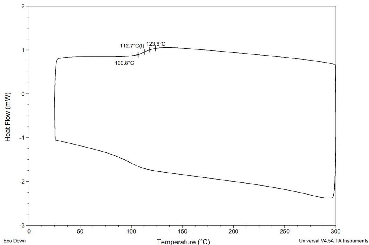
**Figure S116.** DSC Thermogram of polyethylene ferulate (Table S2, entry 31).
