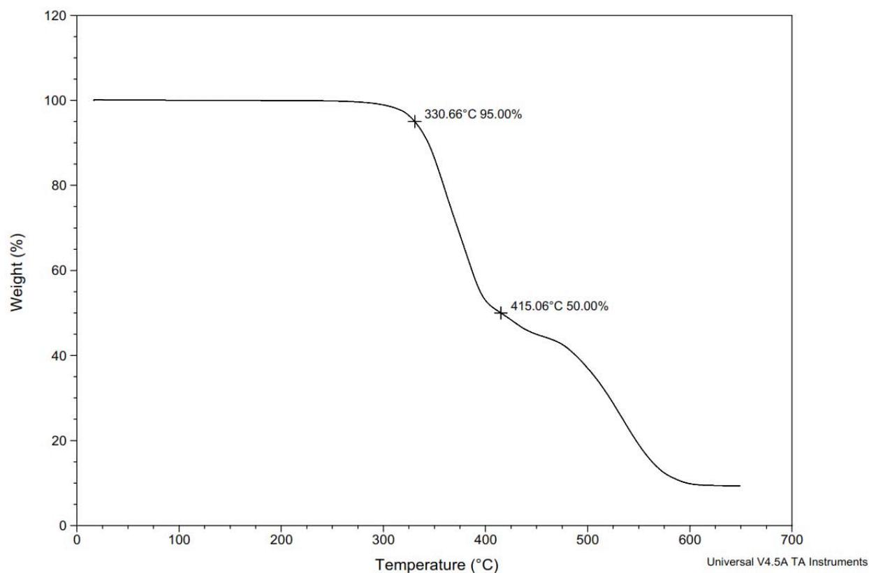
**Figure S187.** TGA Thermogram of copoly(caprolactone/ hydroxyethylferulic acid) [10:90] (Table S2, entry 30).
