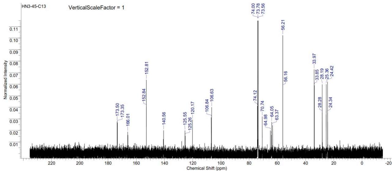
Figure S313.  $^{13}\text{C}$  NMR spectrum of copoly(caprolactone/ hydroxyethylsyringic acid) [60:40] (Table S2, entry 5).
