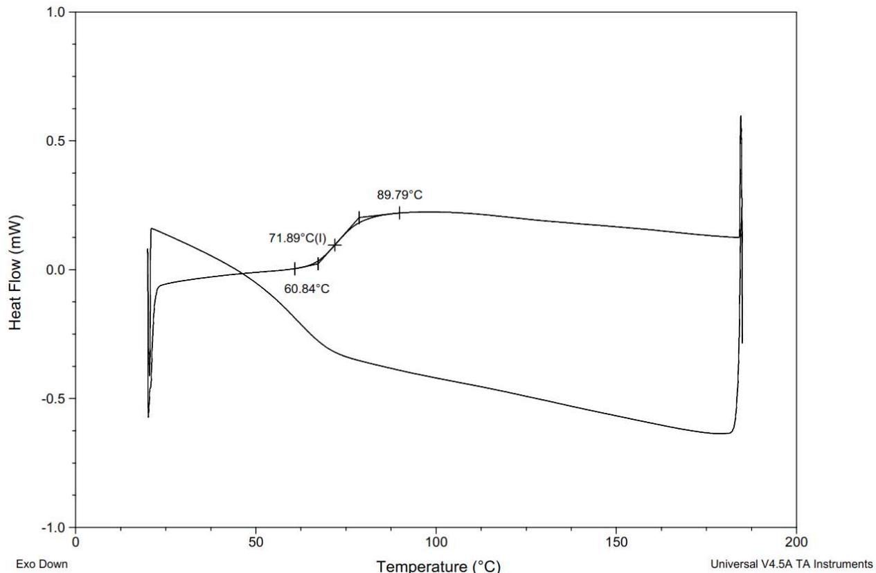
**Figure S137.** DSC Thermogram of copoly(L-lactide/ hydroxyethylcoumaric acid) [70:30] (Table S3, entry 20).
