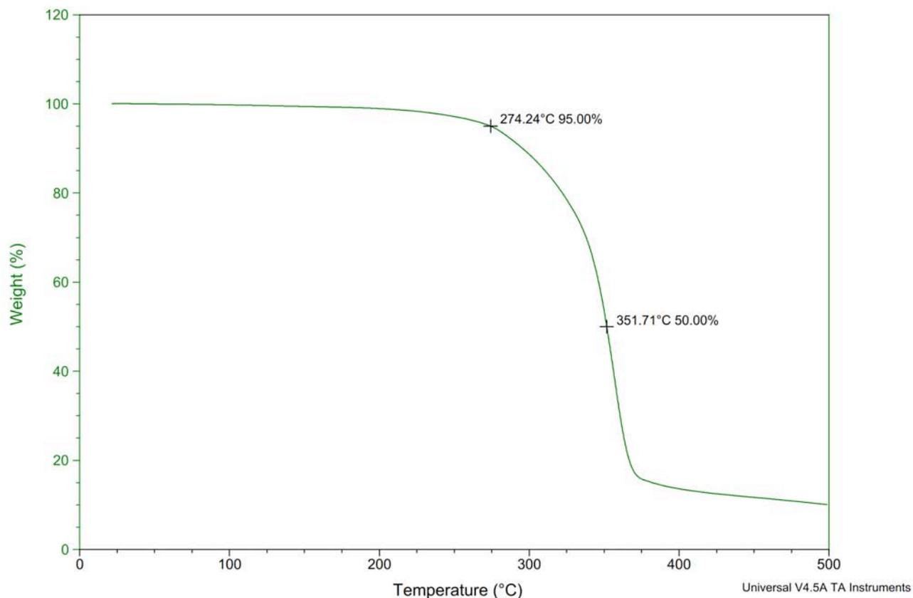
**Figure S222.** TGA Thermogram of copoly(caprolactone/ hydroxyethylsyringic acid) [50:50] at 4.5 hours (Table S4, entry 11).
