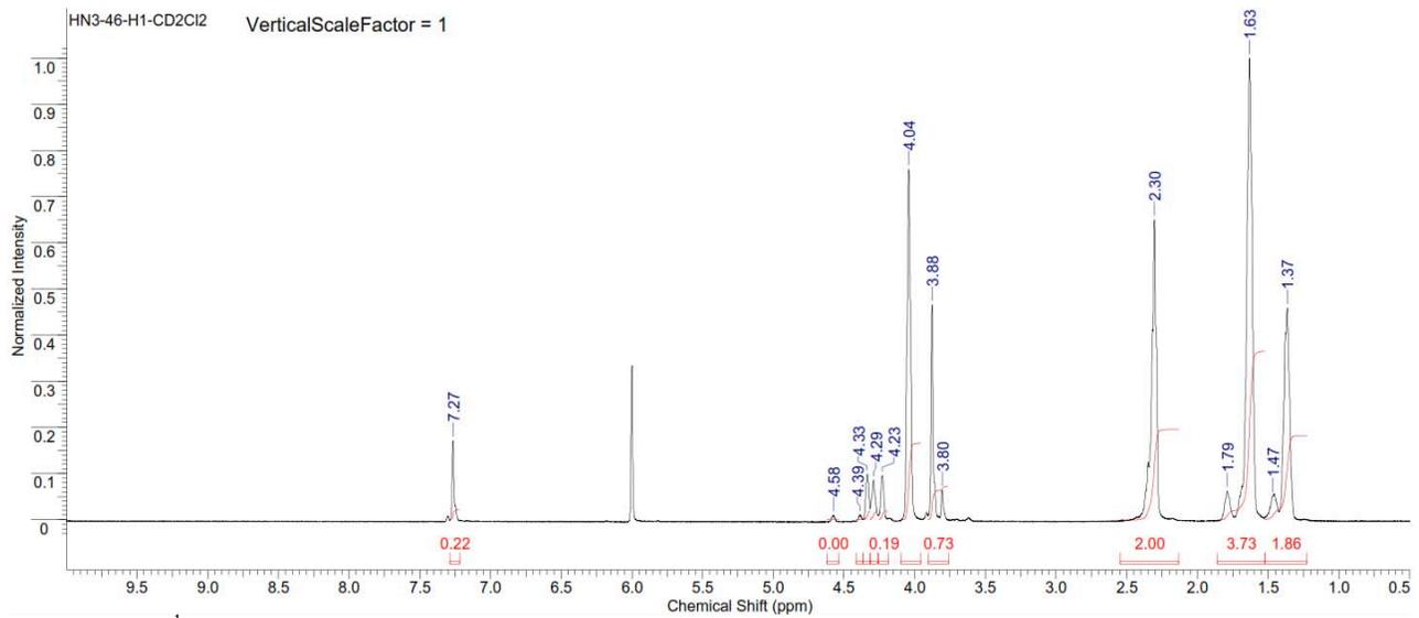
Figure S235. <sup>1</sup>H NMR spectrum of copoly(caprolactone/ hydroxyethylsyngic acid) [90:10] (Table S2, entry 2).
