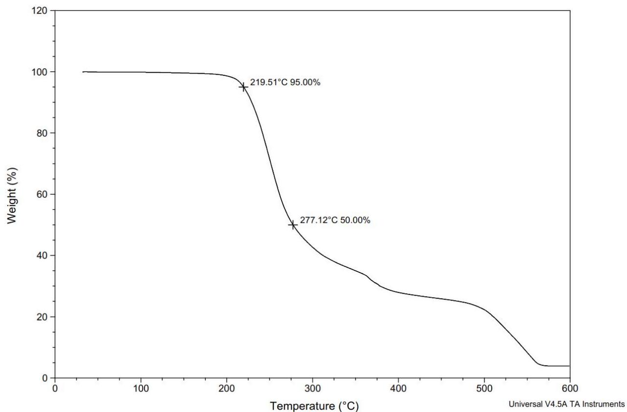
**Figure S202.** TGA Thermogram of copoly(L-lactide/ hydroxyethylferulic acid) [90:10] (Table S3, entry 12).
