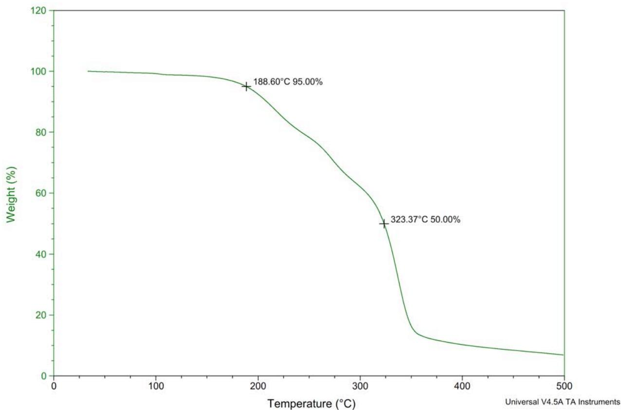
Figure S215. TGA Thermogram of copoly(caprolactone/ hydroxyethylsyngic acid) [50:50] at 1 hour (Table S4, entry 4).
