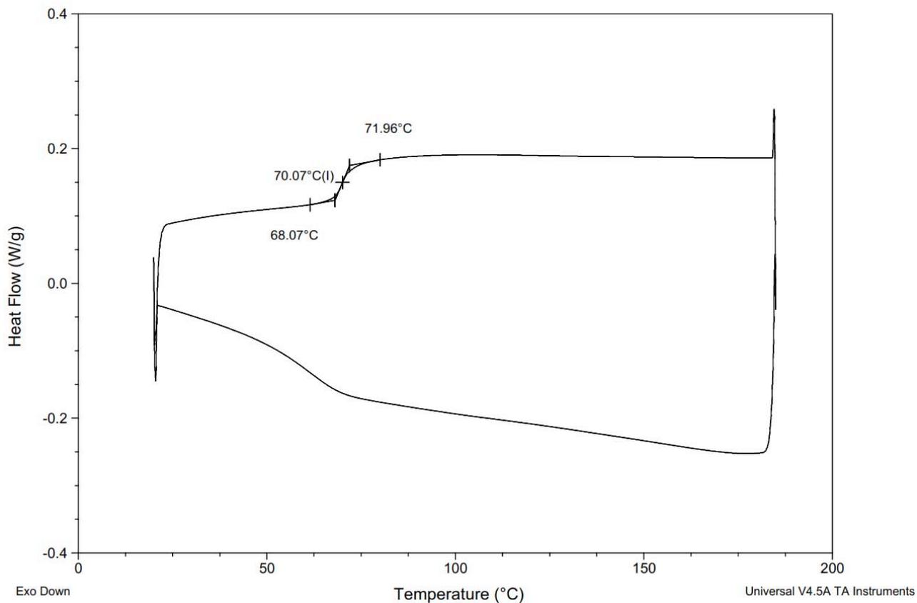
**Figure S124.** DSC Thermogram of copoly(L-lactide/ hydroxyethylsyringic acid) [40:60] (Table S3, entry 4).
