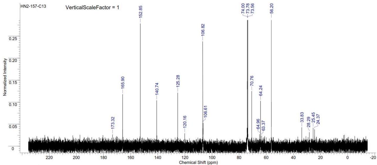
Figure S317.  $^{13}\text{C}$  NMR spectrum of copoly(caprolactone/ hydroxyethylsyringic acid) [20:80] (Table S2, entry 9).
