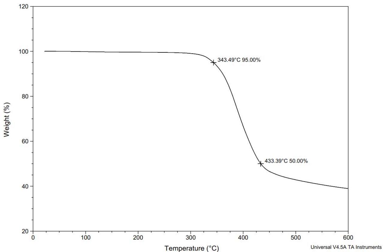
Figure S192. TGA Thermogram of polyethylene coumarate (Table S2, entry 35).
