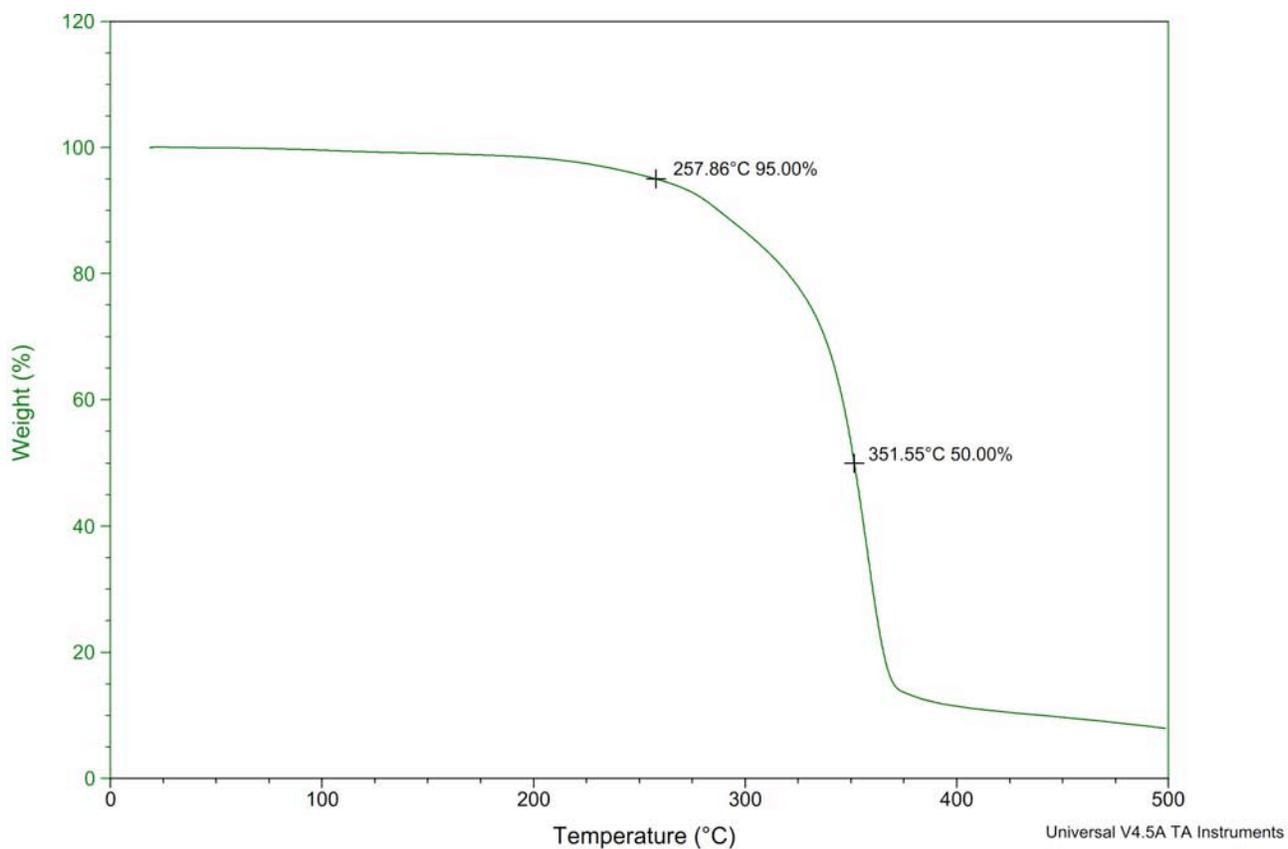
**Figure S221.** TGA Thermogram of copoly(caprolactone/ hydroxyethylsyngic acid) [50:50] at 4 hours (Table S4, entry 10).
