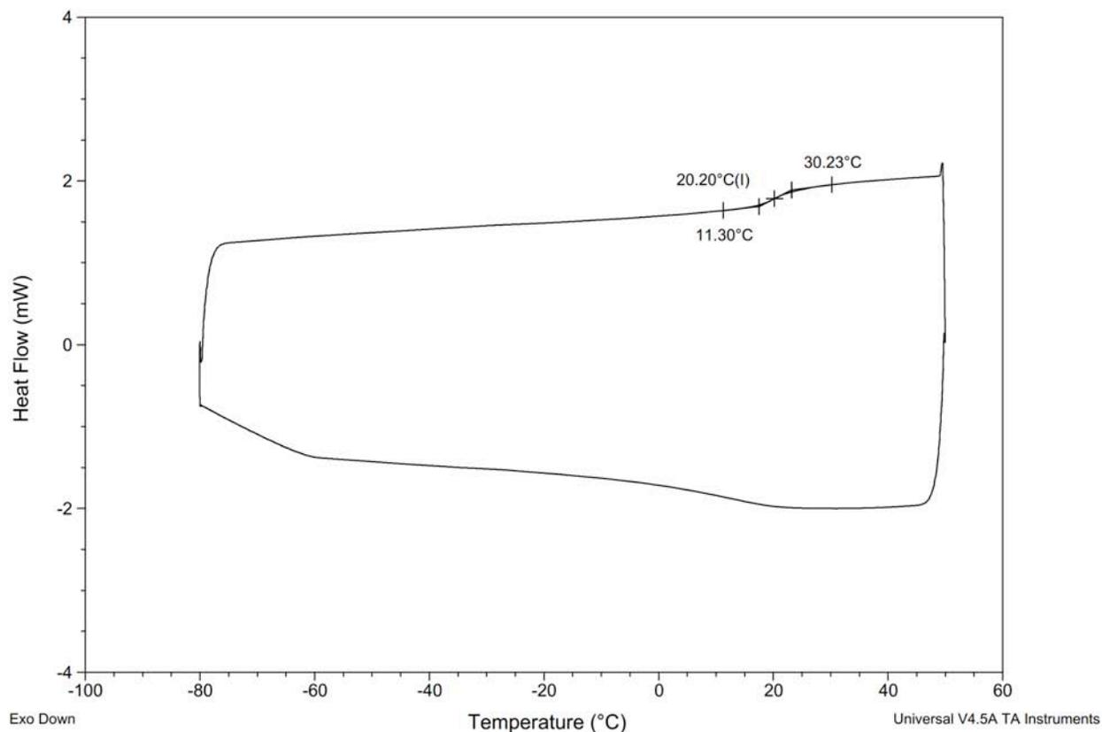
**Figure S156.** DSC Thermogram of copoly(caprolactone/ hydroxyethylsyngic acid) [50:50] at 10 hours (Table S4, entry 17).
