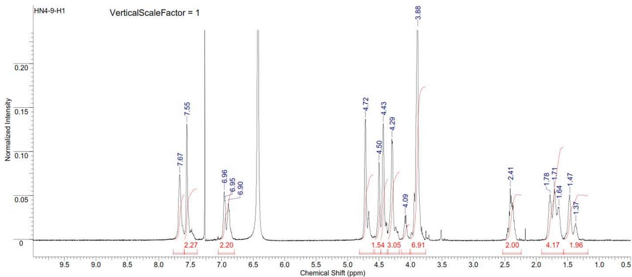
Figure S251. <sup>1</sup>H NMR spectrum of copoly(caprolactone/ hydroxyethylvanillic acid) [30:70] (Table S2, entry 18).
