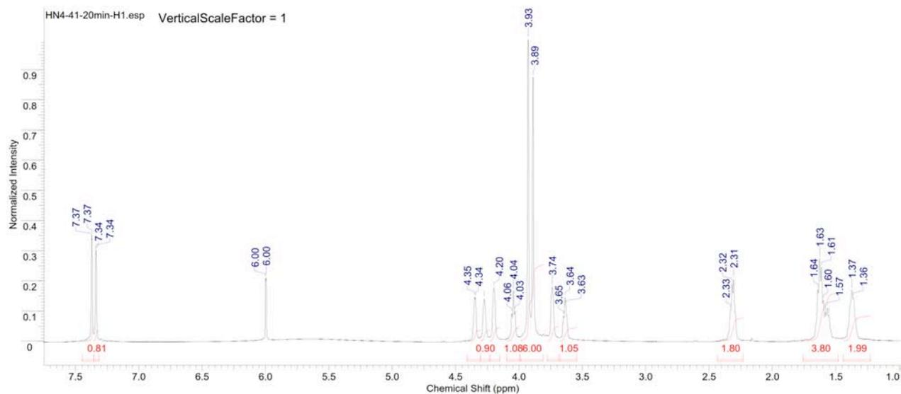
**Figure S288.**  $^1\text{H}$  NMR spectrum of copoly(caprolactone/ hydroxyethylsyngic acid) [50:50] at 20 min. (Table S4, entry 2).
