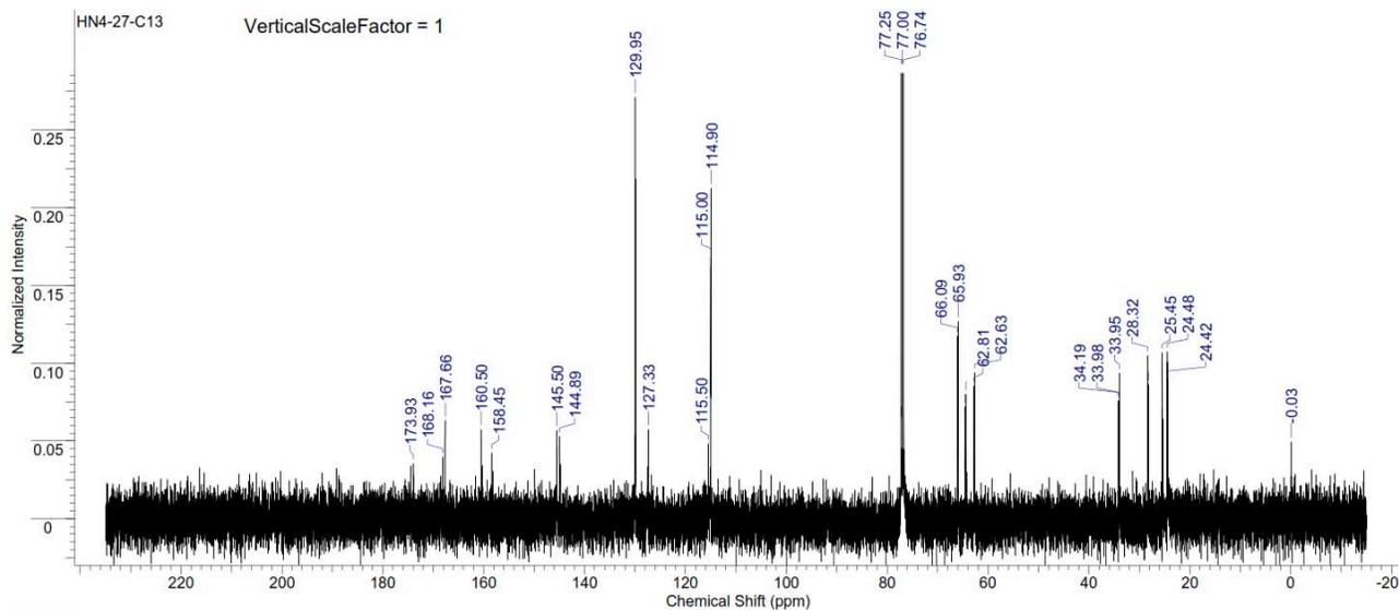
Figure S336.  $^{13}\text{C}$  NMR spectrum of copoly(caprolactone/ hydroxyethylcoumaric acid) [50:50] (Table S2, entry 33).
