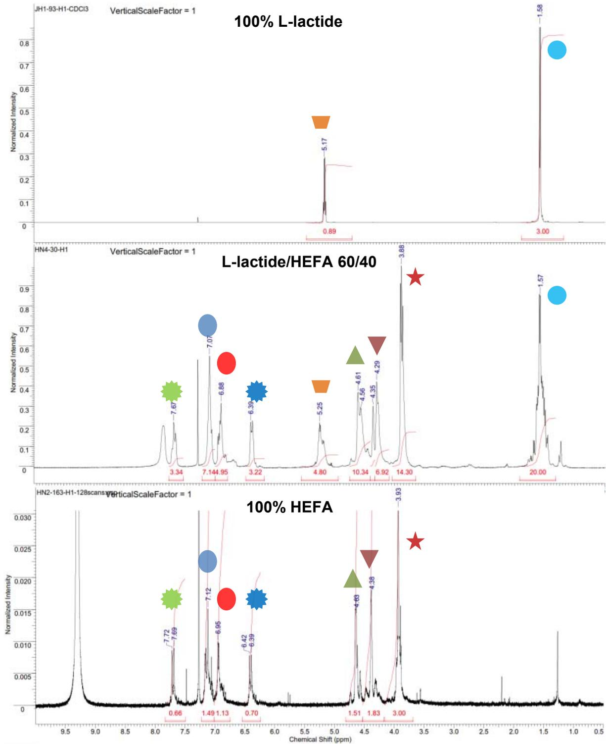
**Figure S378.**  $^1\text{H}$  NMR spectra of copoly(L-lactide/hydroxyethylferulic acid) with hydroxyethylferulic acid (HEFA) feed fractions of 0%, 40%, and 100%.
