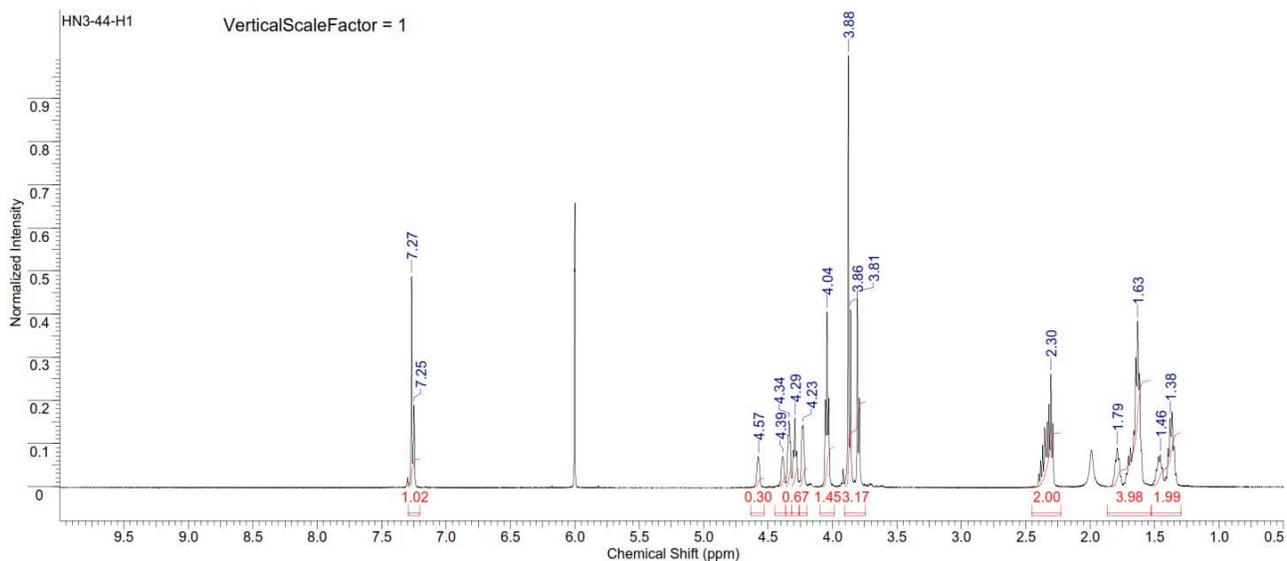
**Figure S237.**  $^1\text{H}$  NMR spectrum of copoly(caprolactone/ hydroxyethylsyngic acid) [70:30] (Table S2, entry 4).
