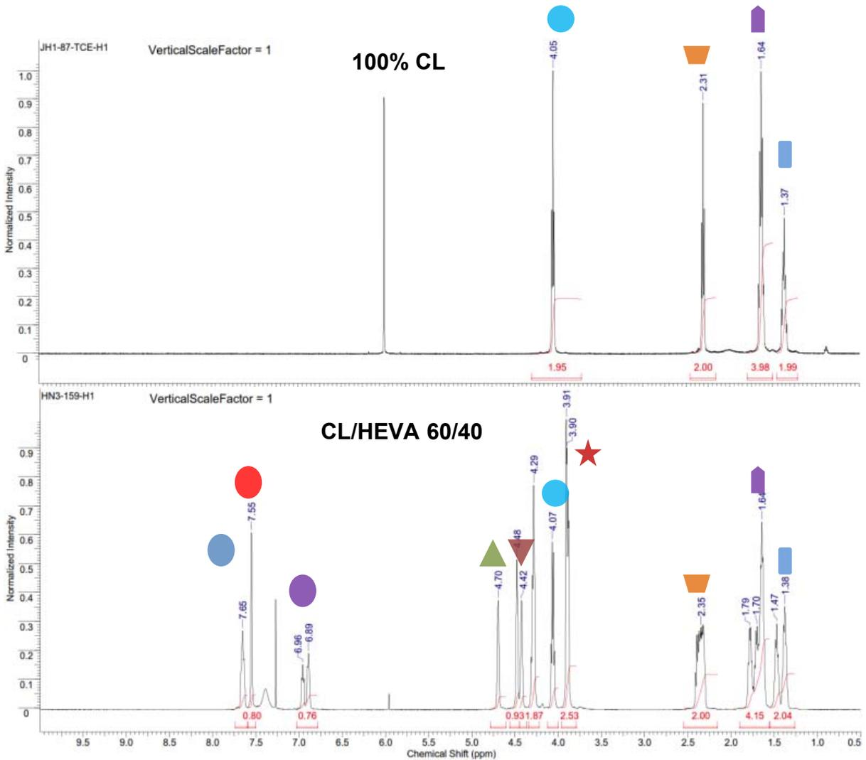
**Figure S373.**  $^1\text{H}$  NMR spectra of copoly(caprolactone/hydroxyethylvanillic acid) with hydroxyethylvanillic acid (HEVA) feed fractions of 0% and 40%.
