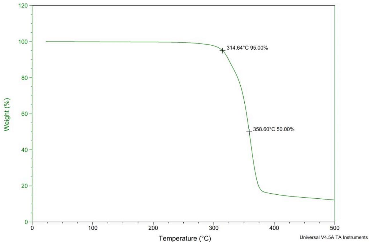
**Figure S229.** TGA Thermogram of copoly(caprolactone/ hydroxyethylsyngic acid) [50:50] at 13 hours (Table S4, entry 18).
