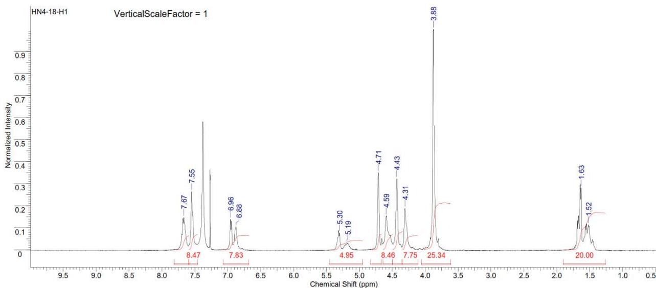
**Figure S275.**  $^1\text{H}$  NMR spectrum of copoly(L-lactide/ hydroxyethylvanillic acid) [40:60] (Table S3, entry 9).
