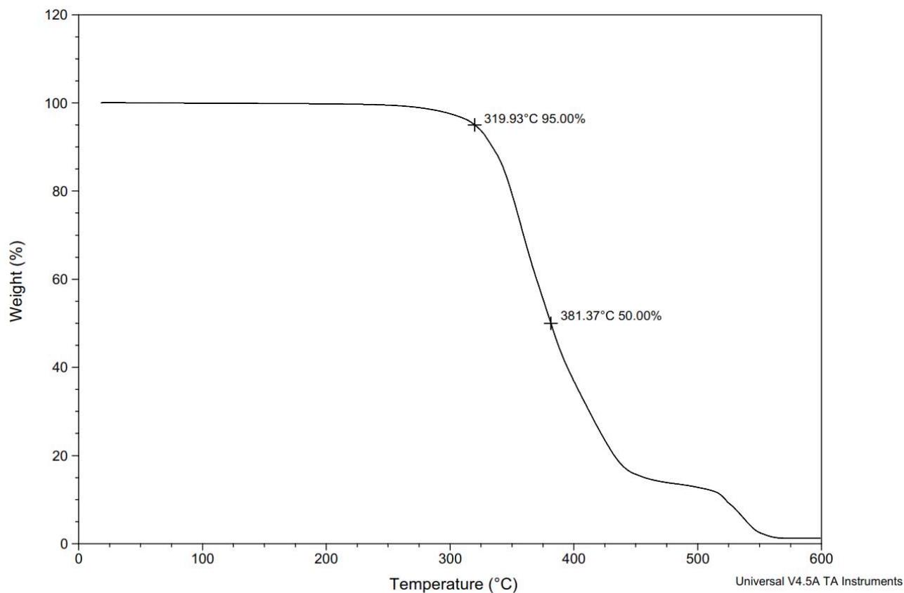
**Figure S189.** TGA Thermogram of copoly(caprolactone/ hydroxyethylcoumaric acid) [80:20] (Table S2, entry 32).
