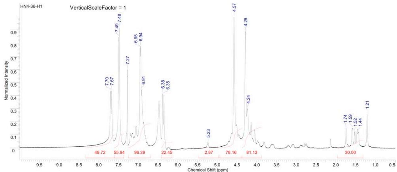
Figure S286. <sup>1</sup>H NMR spectrum of copoly(L-lactide/ hydroxyethylcoumaric acid) [20:80] (Table S3, entry 22).
