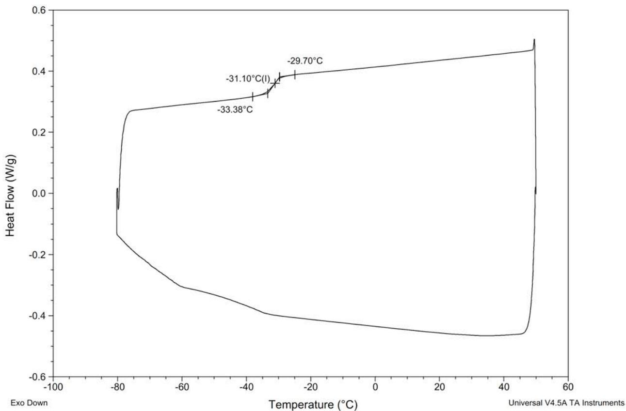
**Figure S143.** DSC Thermogram of copoly(caprolactone/ hydroxyethylsyngic acid) [50:50] at 1 hour (Table S4, entry 4).
