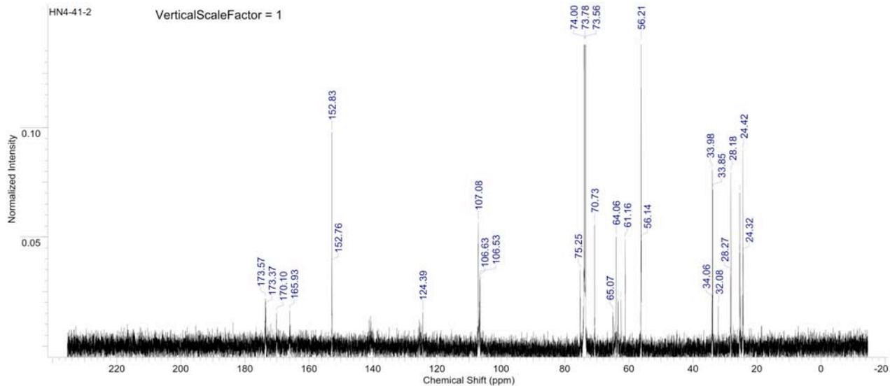
**Figure S360.**  $^{13}\text{C}$  NMR spectrum of copoly(caprolactone/ hydroxyethylsyringic acid) [50:50] at 2.5 hours (Table S4, entry 7).
