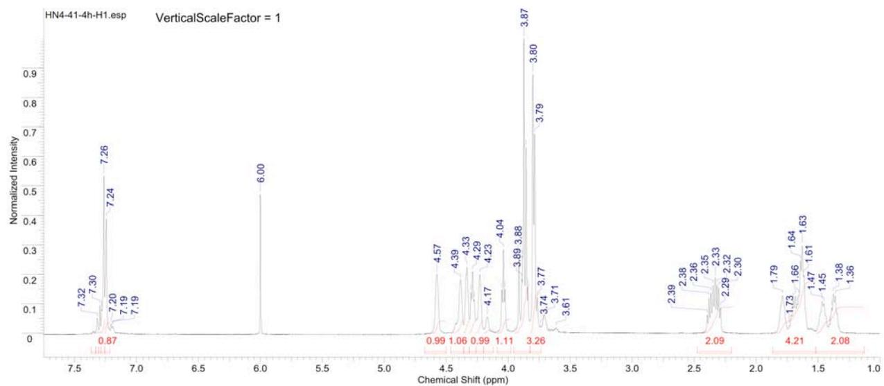
Figure S296. <sup>1</sup>H NMR spectrum of copoly(caprolactone/ hydroxyethylsyngic acid) [50:50] at 4 hours (Table S4, entry 10).
