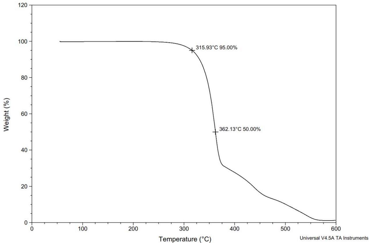
**Figure S166.** TGA Thermogram of copoly(caprolactone/ hydroxyethylsyngic acid) [20:80] (Table S2, entry 9).
