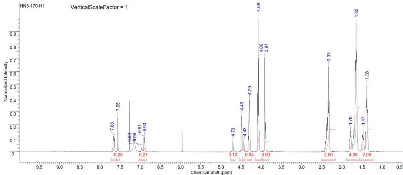
Figure S246. <sup>1</sup>H NMR spectrum of copoly(caprolactone/ hydroxyethylvanillic acid) [80:20] (Table S2, entry 13).
