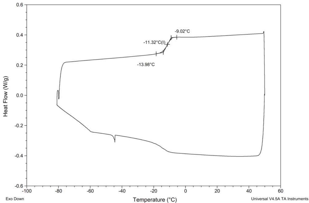
**Figure S146.** DSC Thermogram of copoly(caprolactone/ hydroxyethylsyngic acid) [50:50] at 2.5 hours (Table S4, entry 7).
