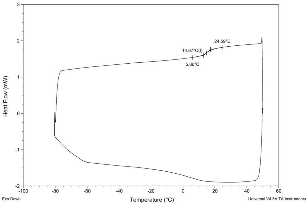
**Figure S154.** DSC Thermogram of copoly(caprolactone/ hydroxyethylsyngic acid) [50:50] at 8 hours (Table S4, entry 15).
