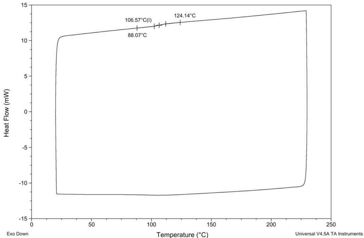
**Figure S134.** DSC Thermogram of copoly(L-lactide/ hydroxyethylferulic acid) [20:80] (Table S3, entry 16).
