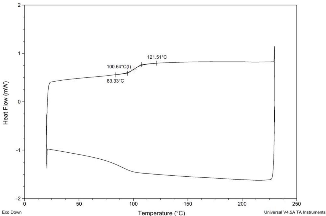
**Figure S139.** DSC Thermogram of copoly(L-lactide/ hydroxyethylcoumaric acid) [20:80] (Table S3, entry 22).
