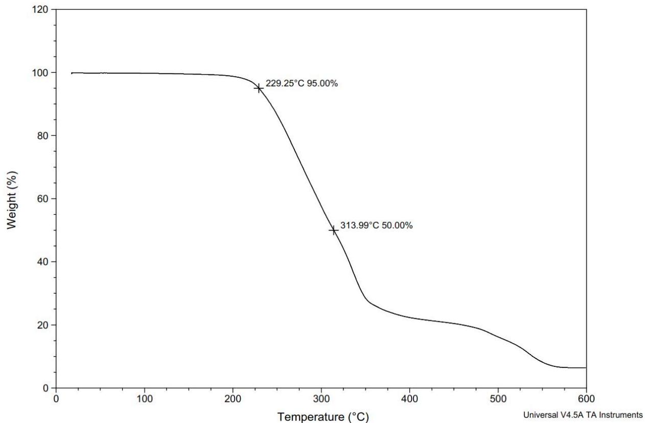
**Figure S198.** TGA Thermogram of copoly(L-lactide/ hydroxyethylvanillic acid) [80:20] (Table S3, entry 7).
