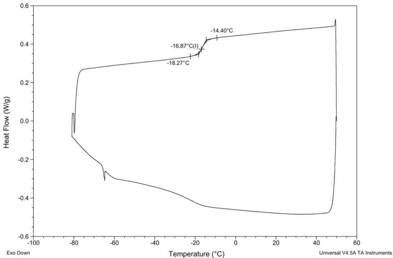
**Figure S145.** DSC Thermogram of copoly(caprolactone/ hydroxyethylsyngic acid) [50:50] at 2 hours (Table S4, entry 6).
