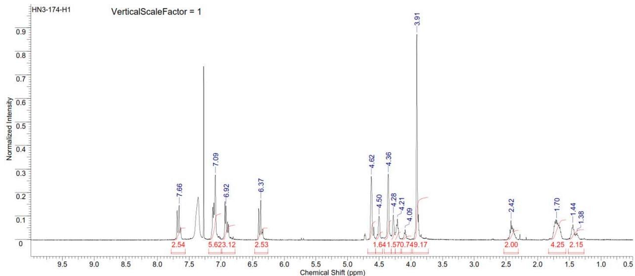
Figure S259.  $^1\text{H}$  NMR spectrum of copoly(caprolactone/ hydroxyethylferulic acid) [40:60] (Table S2, entry 27).
