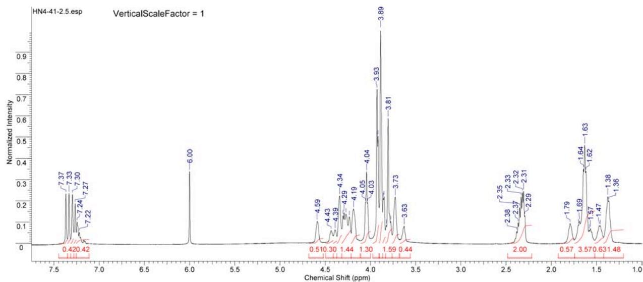
Figure S295. <sup>1</sup>H NMR spectrum of copoly(caprolactone/ hydroxyethylsyngic acid) [50:50] at 3.5 hours (Table S4, entry 9).
