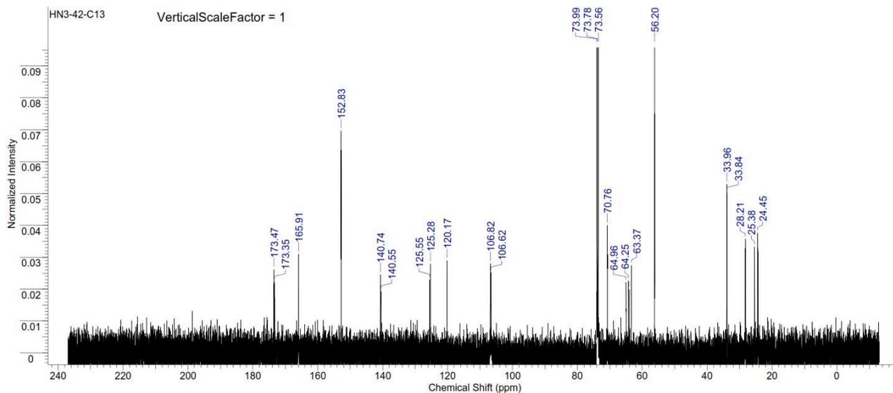
Figure S314.  $^{13}\text{C}$  NMR spectrum of copoly(caprolactone/ hydroxyethylsyringic acid) [50:50] (Table S2, entry 6).
