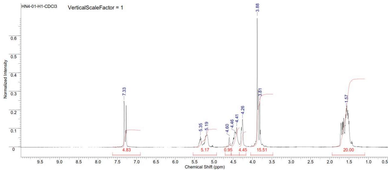
Figure S269.  $^1\text{H}$  NMR spectrum of copoly(L-lactide/ hydroxyethylsyringic acid) [80:20] (Table S3, entry 2).
