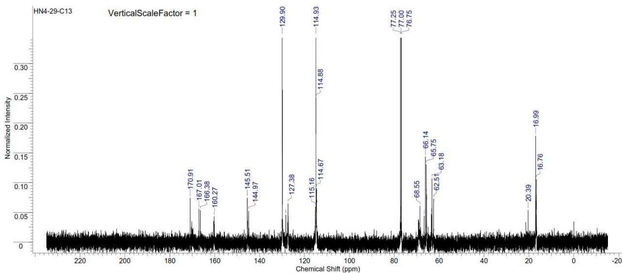
Figure S353.  $^{13}\text{C}$  NMR spectrum of copoly(L-lactide/ hydroxyethylcoumaric acid) [60:40] (Table S3, entry 21).
