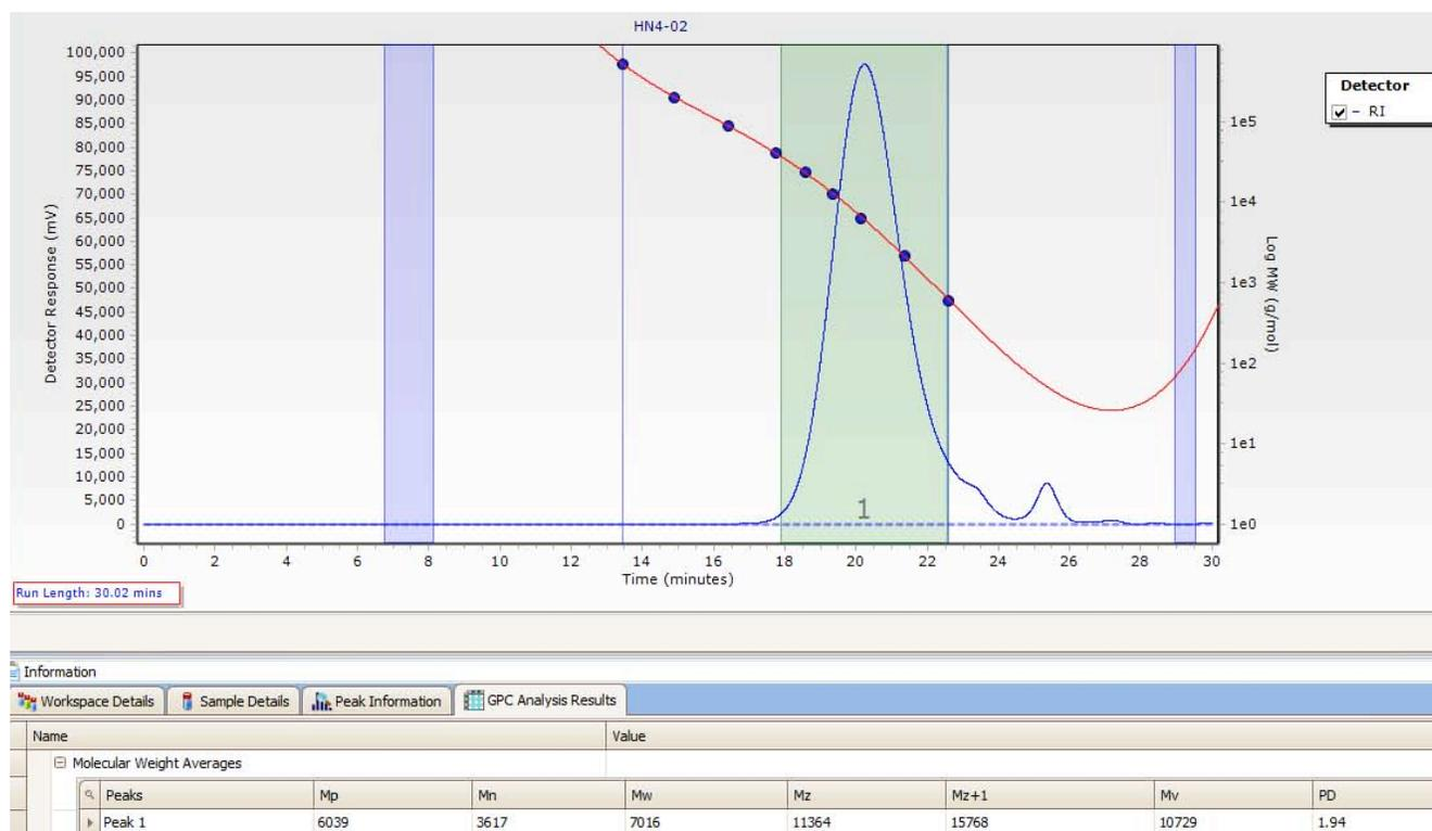
Figure S46. GPC Chromatogram of copoly(L-lactide/ hydroxyethylsyngic acid) [20:80] (Table S3, entry 5).
