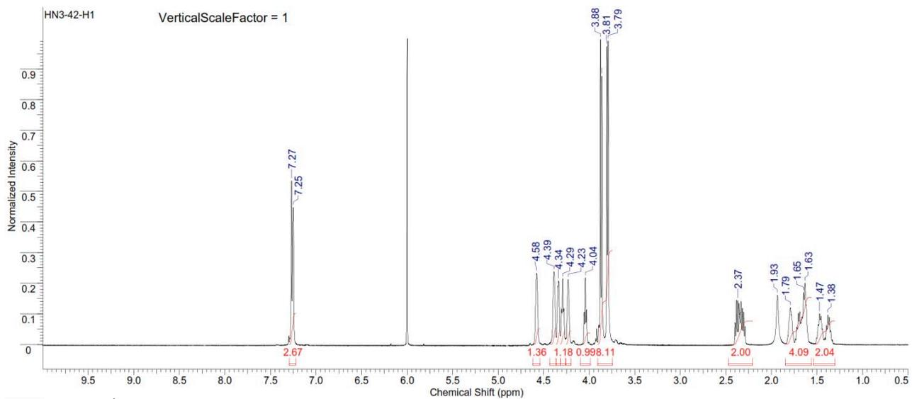
**Figure S239.**  $^1\text{H}$  NMR spectrum of copoly(caprolactone/ hydroxyethylsyngic acid) [50:50] (Table S2, entry 6).
