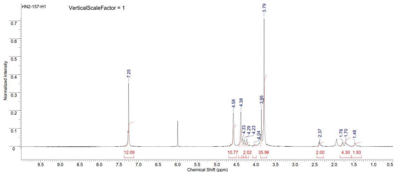
Figure S242. <sup>1</sup>H NMR spectrum of copoly(caprolactone/ hydroxyethylsyngic acid) [20:80] (Table S2, entry 9).
