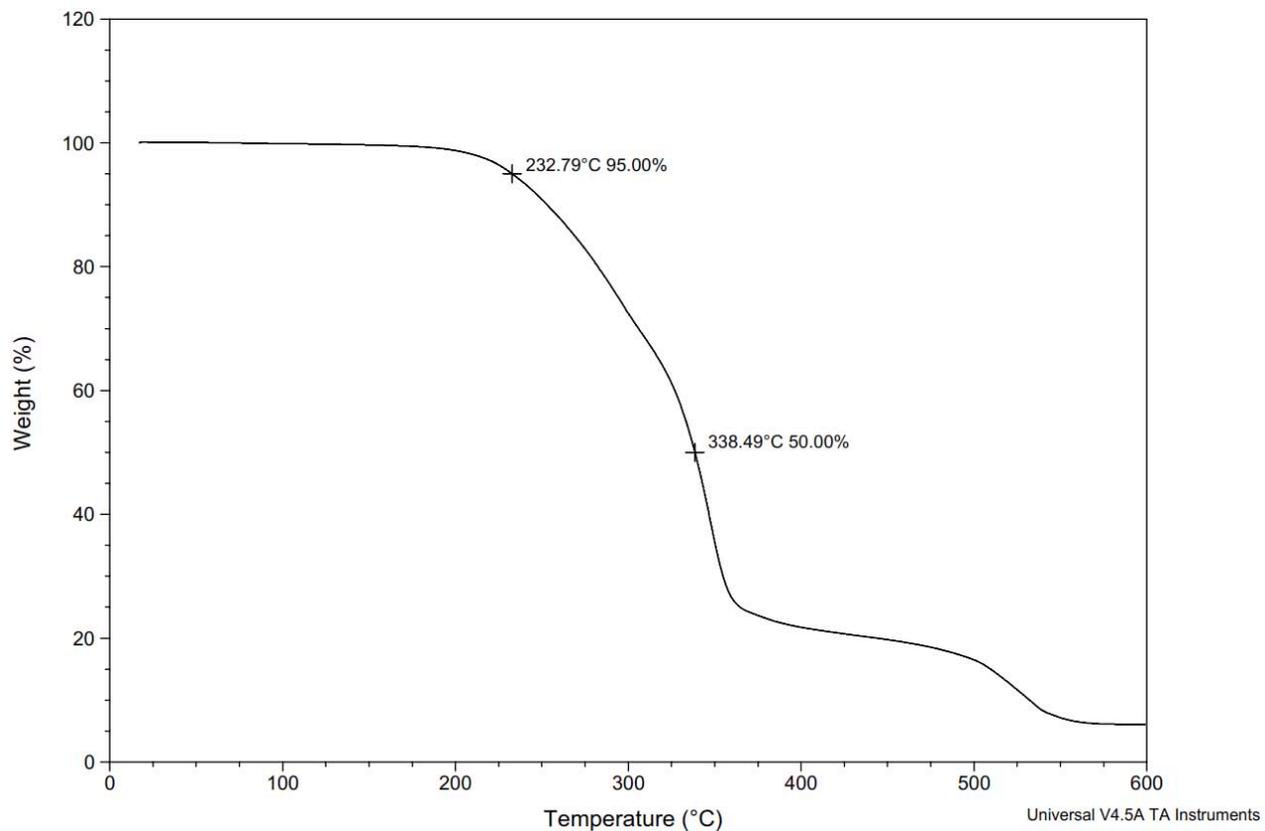
**Figure S199.** TGA Thermogram of copoly(L-lactide/ hydroxyethylvanillic acid) [60:40] (Table S3, entry 8).
