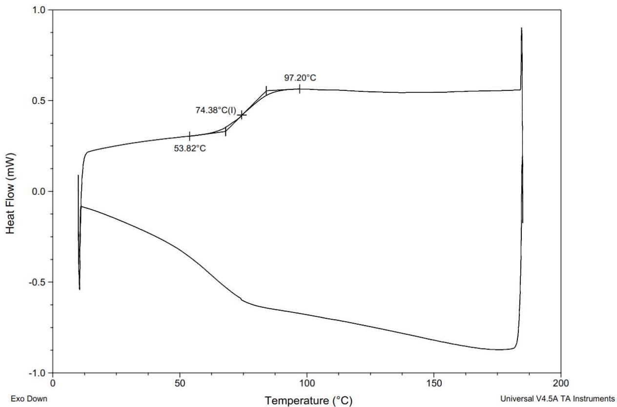
**Figure S132.** DSC Thermogram of copoly(L-lactide/ hydroxyethylferulic acid) [70:30] (Table S3, entry 14).
