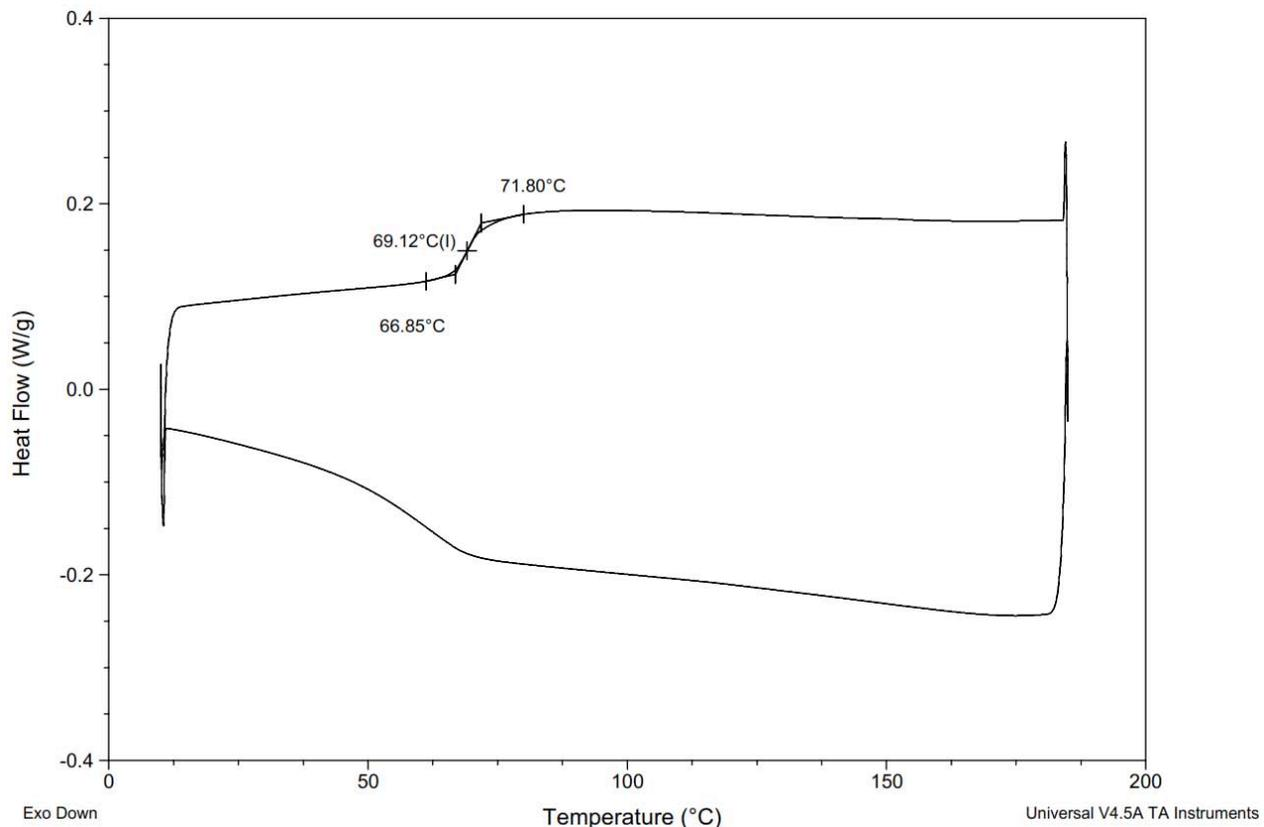
**Figure S131.** DSC Thermogram of copoly(L-lactide/ hydroxyethylferulic acid) [80:20] (Table S3, entry 13).
