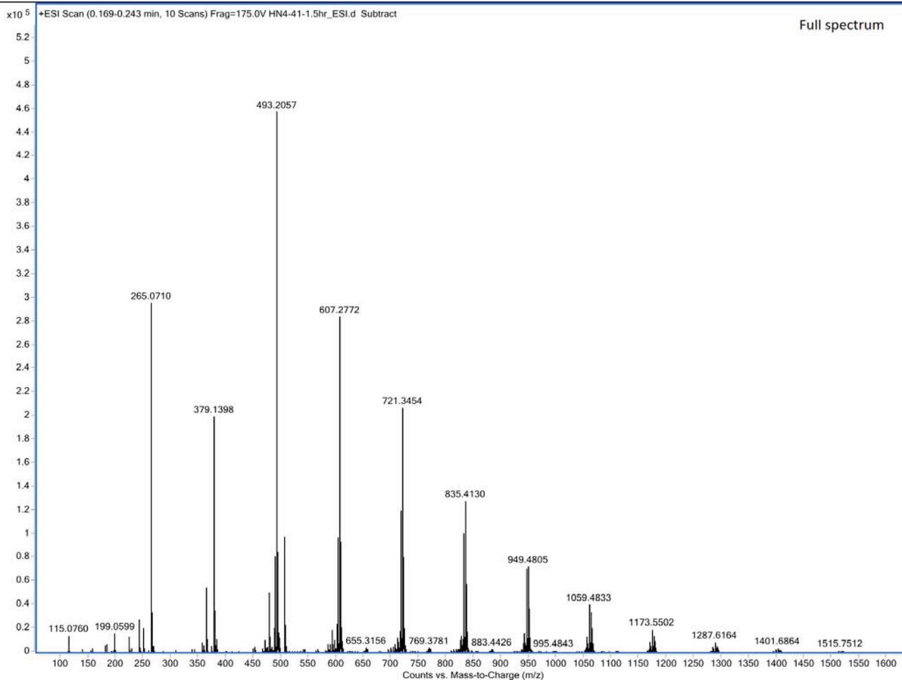
Figure S384. ESI spectra of copoly(caprolactone/hydroxyethylsyngic acid) [50:50] at 1.5 hours (Table S4, entry 5)
