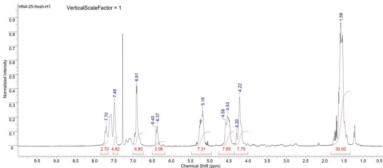
Figure S283. <sup>1</sup>H NMR spectrum of copoly(L-lactide/ hydroxyethylcoumaric acid) [80:20] (Table S3, entry 19).
