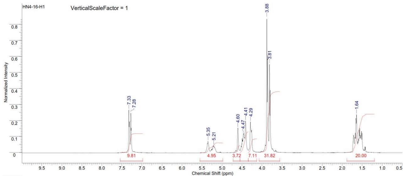
Figure S270. <sup>1</sup>H NMR spectrum of copoly(L-lactide/ hydroxyethylsyngic acid) [60:40] (Table S3, entry 3).
