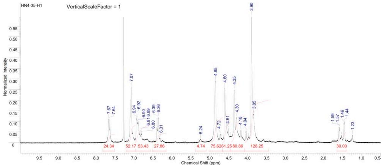
Figure S281. <sup>1</sup>H NMR spectrum of copoly(L-lactide/ hydroxyethylferulic acid) [20:80] (Table S3, entry 16).
