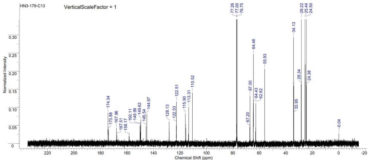
Figure S329. <sup>13</sup>C NMR spectrum of copoly(caprolactone/ hydroxyethylferulic acid) [70:30] (Table S2, entry 24).
