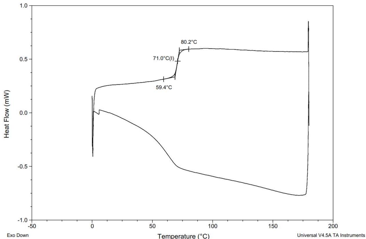
**Figure S127.** DSC Thermogram of copoly(L-lactide/ hydroxyethylvanillic acid) [60:40] (Table S3, entry 8).
