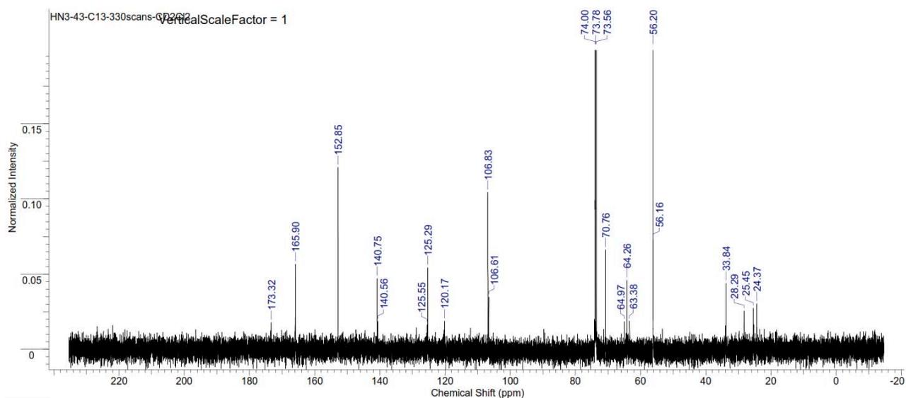
Figure S315.  $^{13}\text{C}$  NMR spectrum of copoly(caprolactone/ hydroxyethylsyringic acid) [40:60] (Table S2, entry 7).
