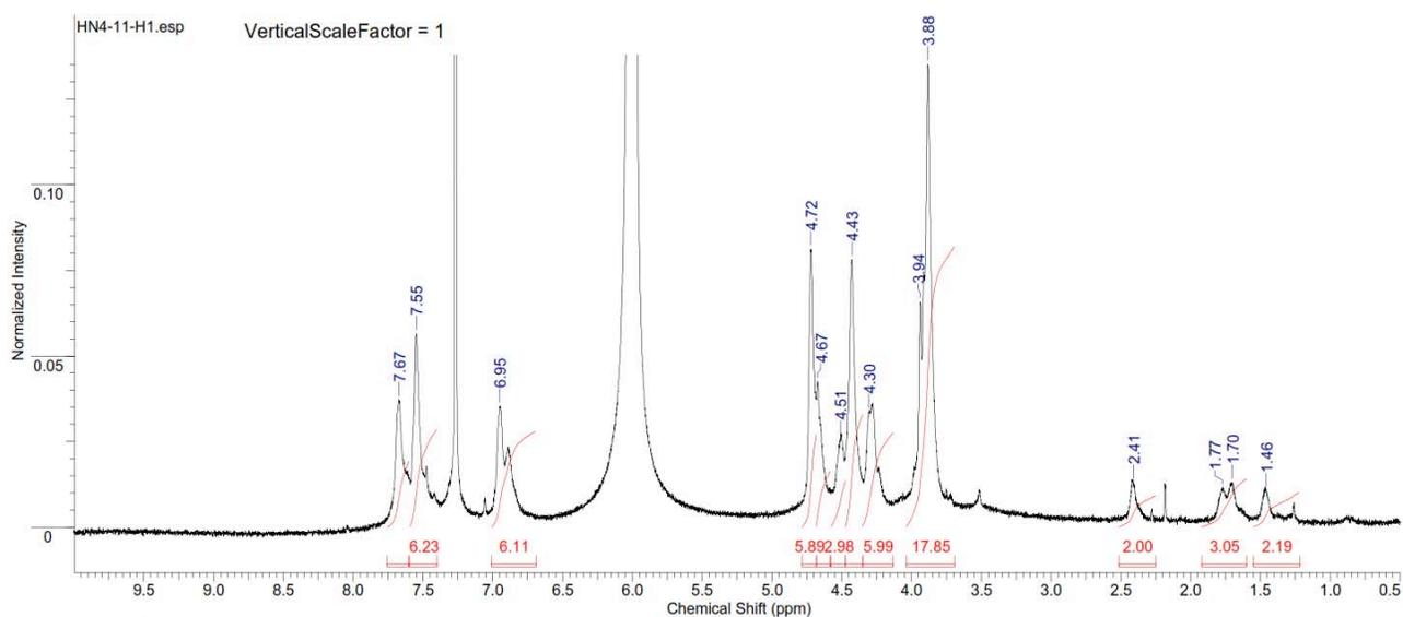
Figure S253. <sup>1</sup>H NMR spectrum of copoly(caprolactone/ hydroxyethylvanillic acid) [10:90] (Table S2, entry 20).
