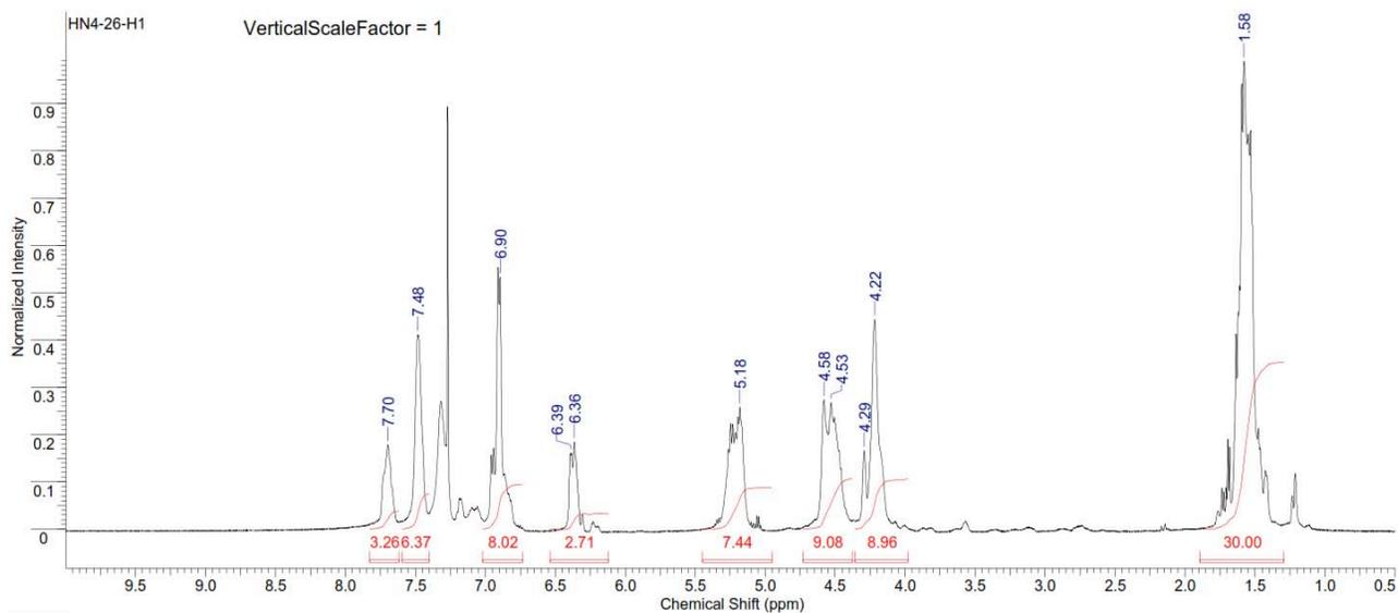
Figure S284. <sup>1</sup>H NMR spectrum of copoly(L-lactide/ hydroxyethylcoumaric acid) [70:30] (Table S3, entry 20).
