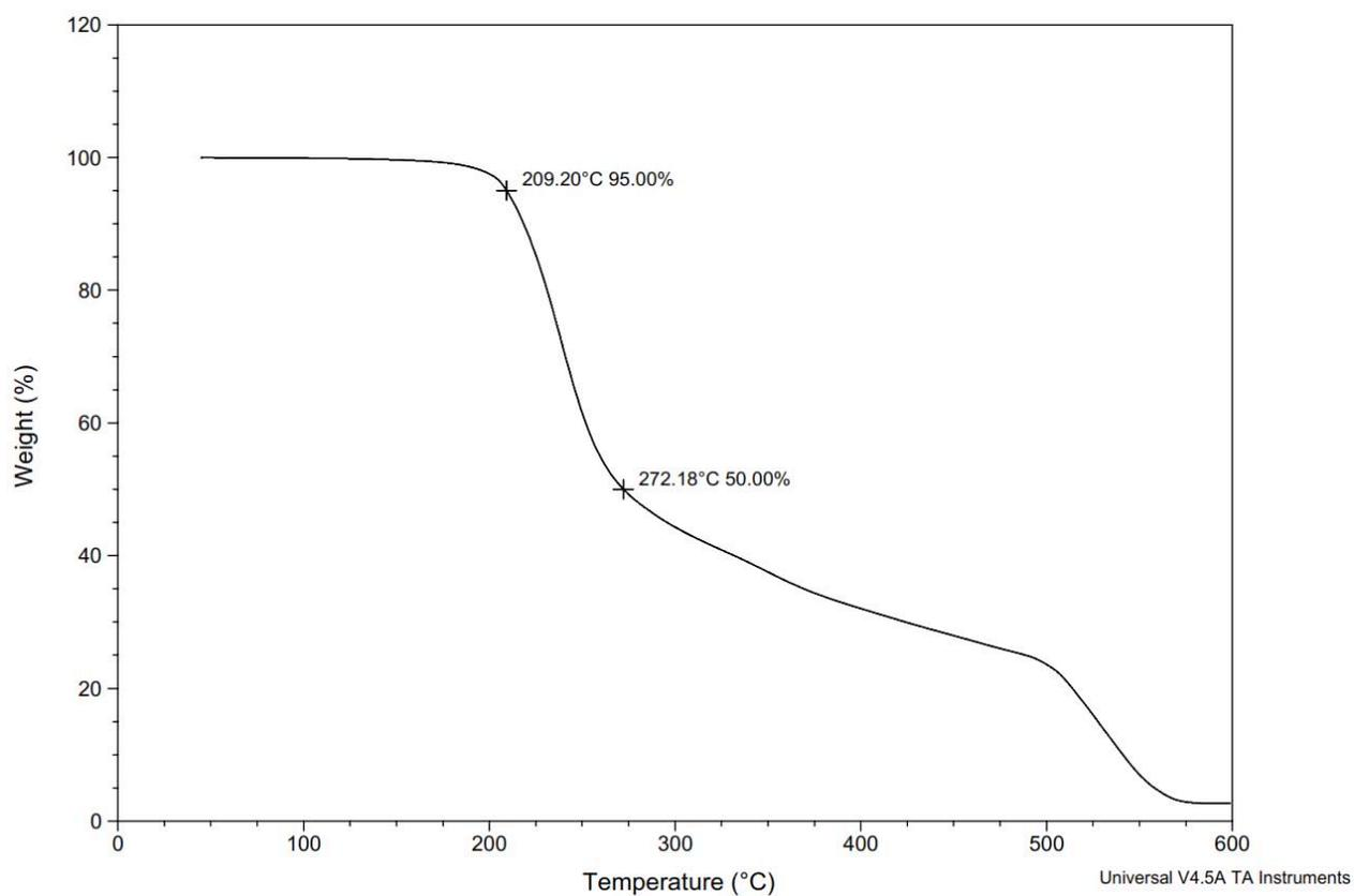
**Figure S207.** TGA Thermogram of copoly(L-lactide/ hydroxyethylcoumaric acid) [90:10] (Table S3, entry 18).
