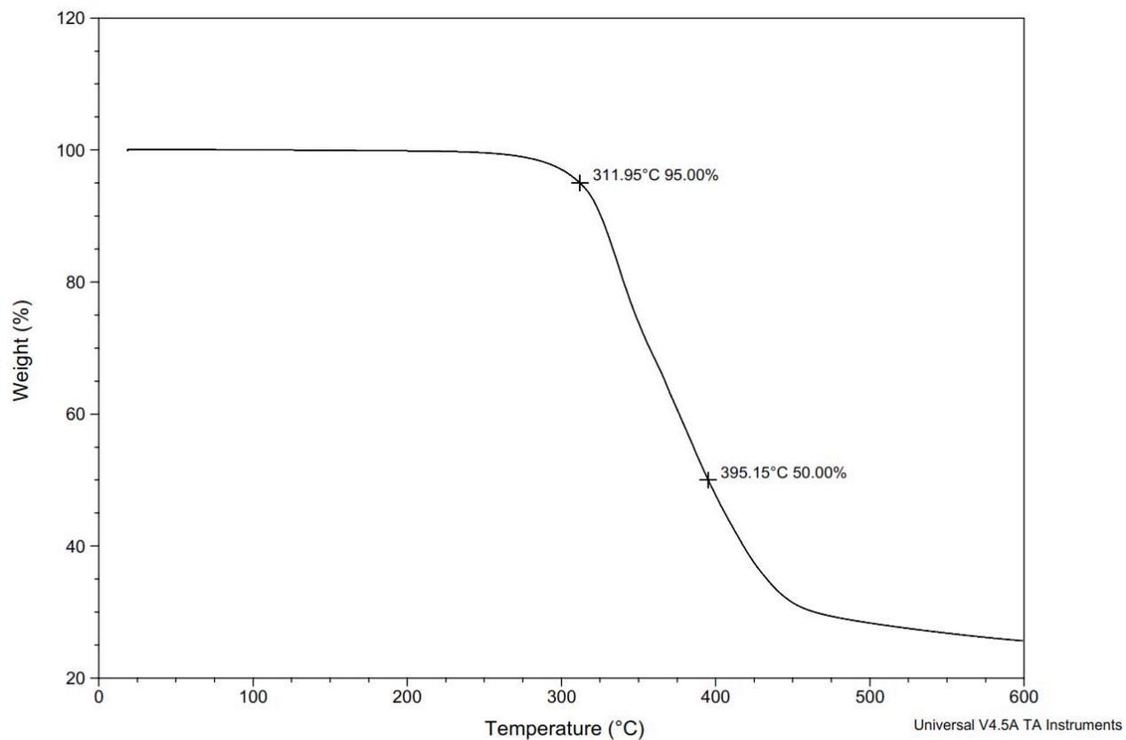
**Figure S190.** TGA Thermogram of copoly(caprolactone/ hydroxyethylcoumaric acid) [50:50] (Table S2, entry 33).
