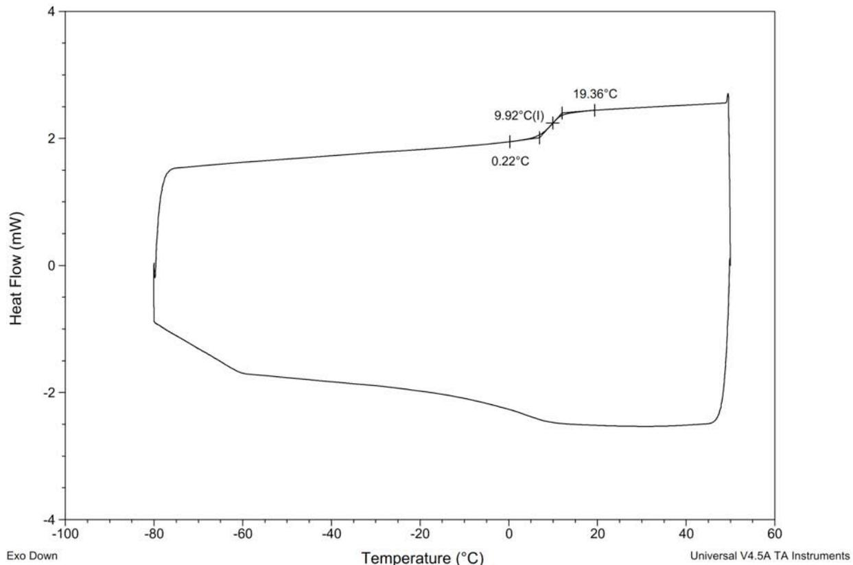
**Figure S151.** DSC Thermogram of copoly(caprolactone/ hydroxyethylsyngic acid) [50:50] at 5 hours (Table S4, entry 12).
