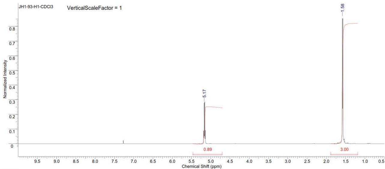
Figure S268.  $^1\text{H}$  NMR spectrum of polylactic acid (Table S3, entry 1).
