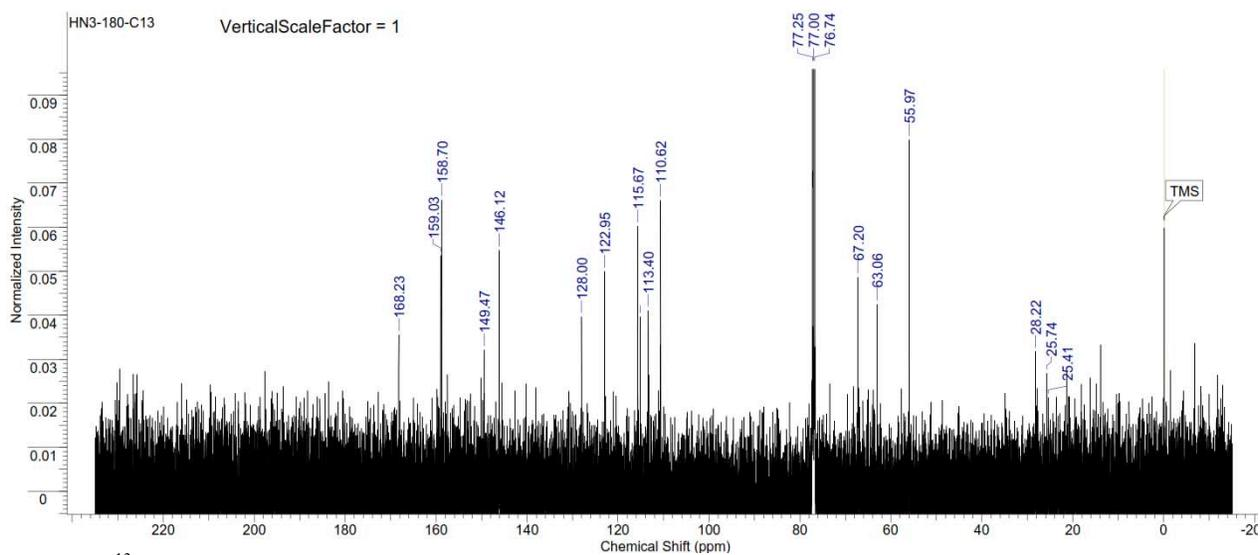
Figure S333.  $^{13}\text{C}$  NMR spectrum of copoly(caprolactone/ hydroxyethylferulic acid) [30:70] (Table S2, entry 28).
