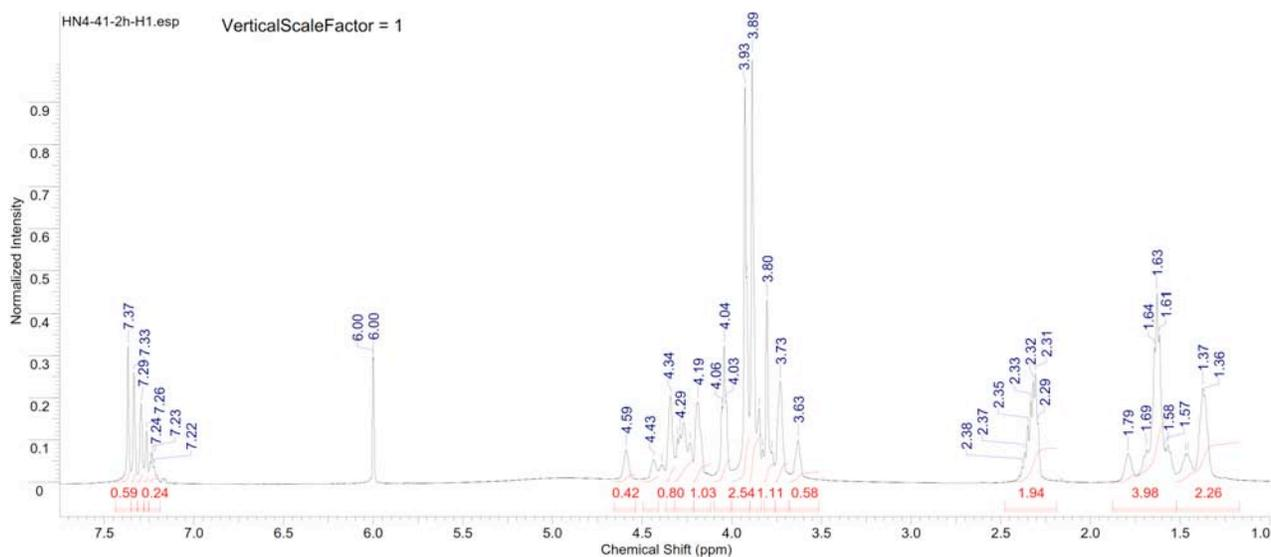
Figure S292. <sup>1</sup>H NMR spectrum of copoly(caprolactone/ hydroxyethylsyngic acid) [50:50] at 2 hours (Table S4, entry 6).
