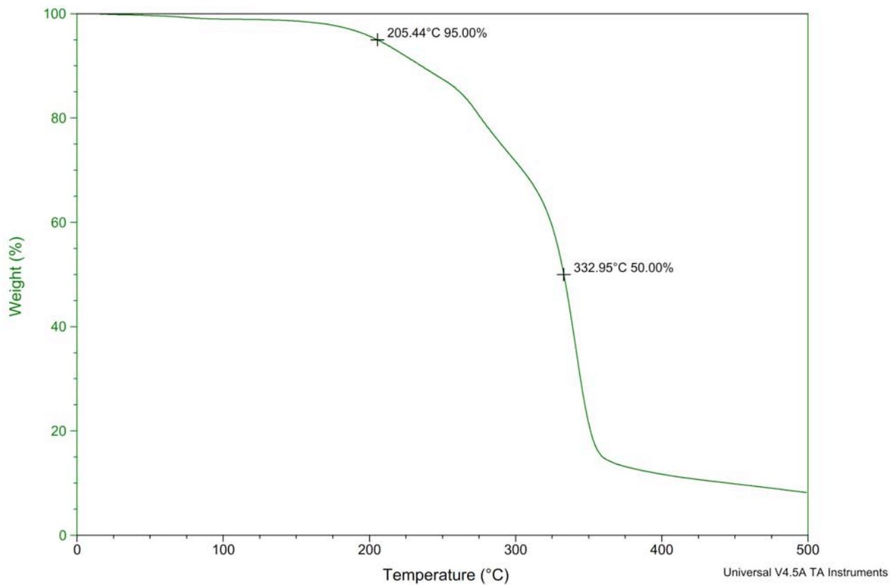
Figure S218. TGA Thermogram of copoly(caprolactone/ hydroxyethylsyngic acid) [50:50] at 2.5 hours (Table S4, entry 7).
