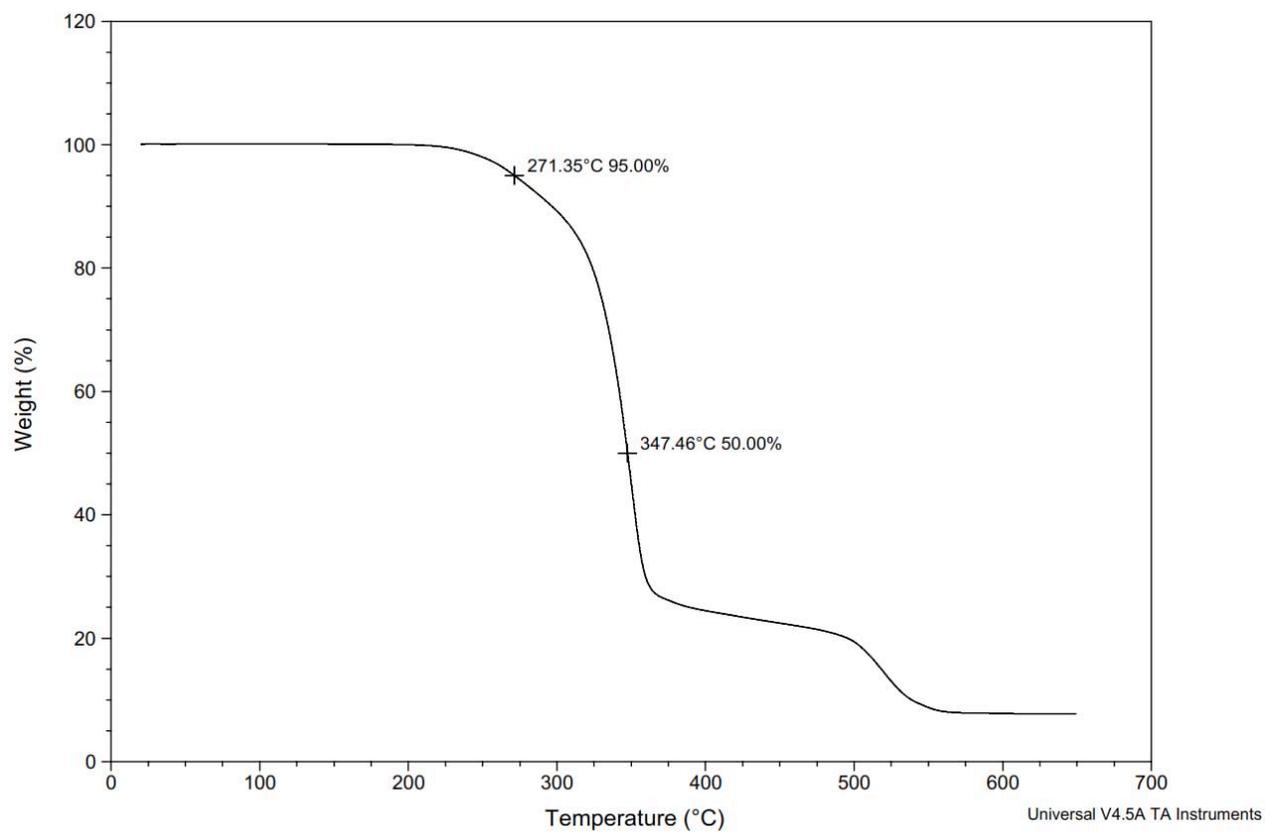
**Figure S200.** TGA Thermogram of copoly(L-lactide/ hydroxyethylvanillic acid) [40:60] (Table S3, entry 9).
