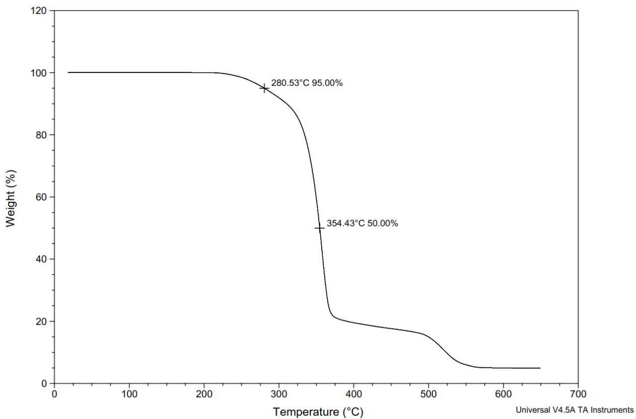
**Figure S201.** TGA Thermogram of copoly(L-lactide/ hydroxyethylvanillic acid) [20:80] (Table S3, entry 10).
