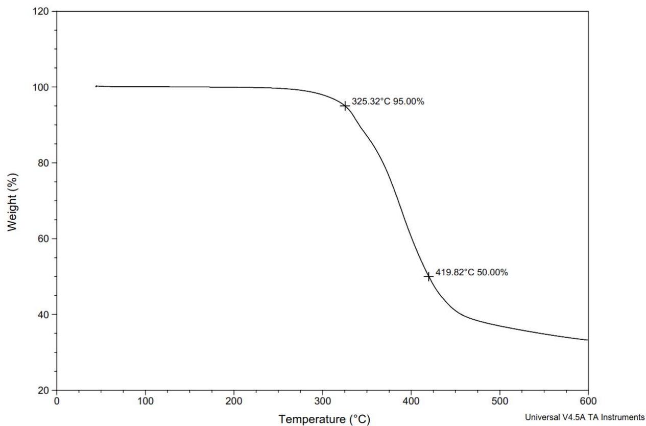
**Figure S191.** TGA Thermogram of copoly(caprolactone/ hydroxyethylcoumaric acid) [20:80] (Table S2, entry 34).
