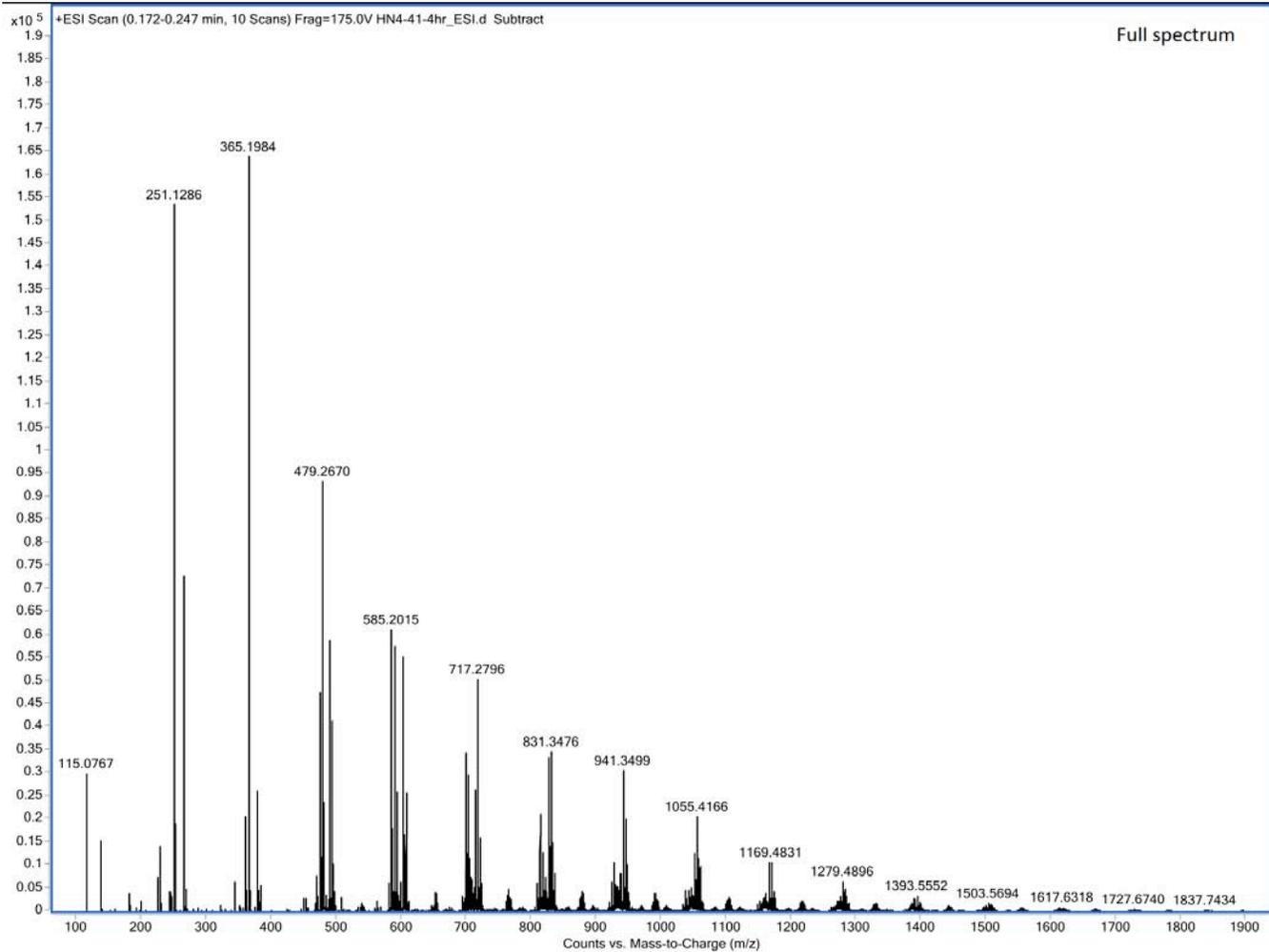
**Figure S389.** ESI spectra of copoly(caprolactone/hydroxyethylsyringic acid) [50:50] at 4 hours (Table S4, entry 10)
