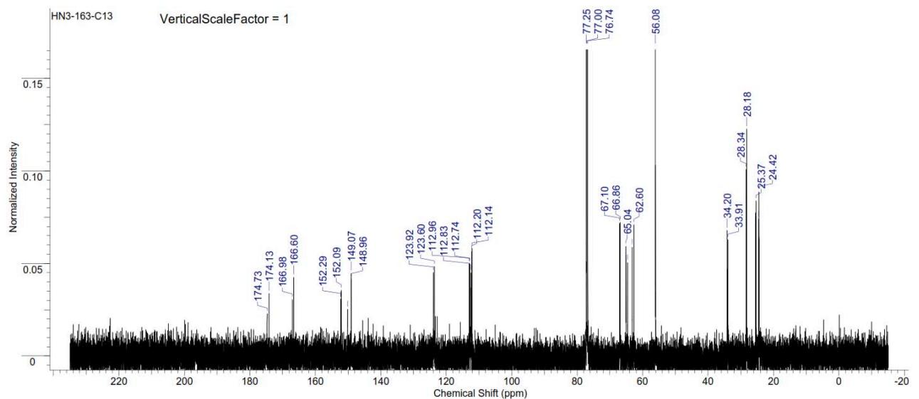
Figure S324.  $^{13}\text{C}$  NMR spectrum of copoly(caprolactone/ hydroxyethylvanillic acid) [50:50] (Table S2, entry 16).
