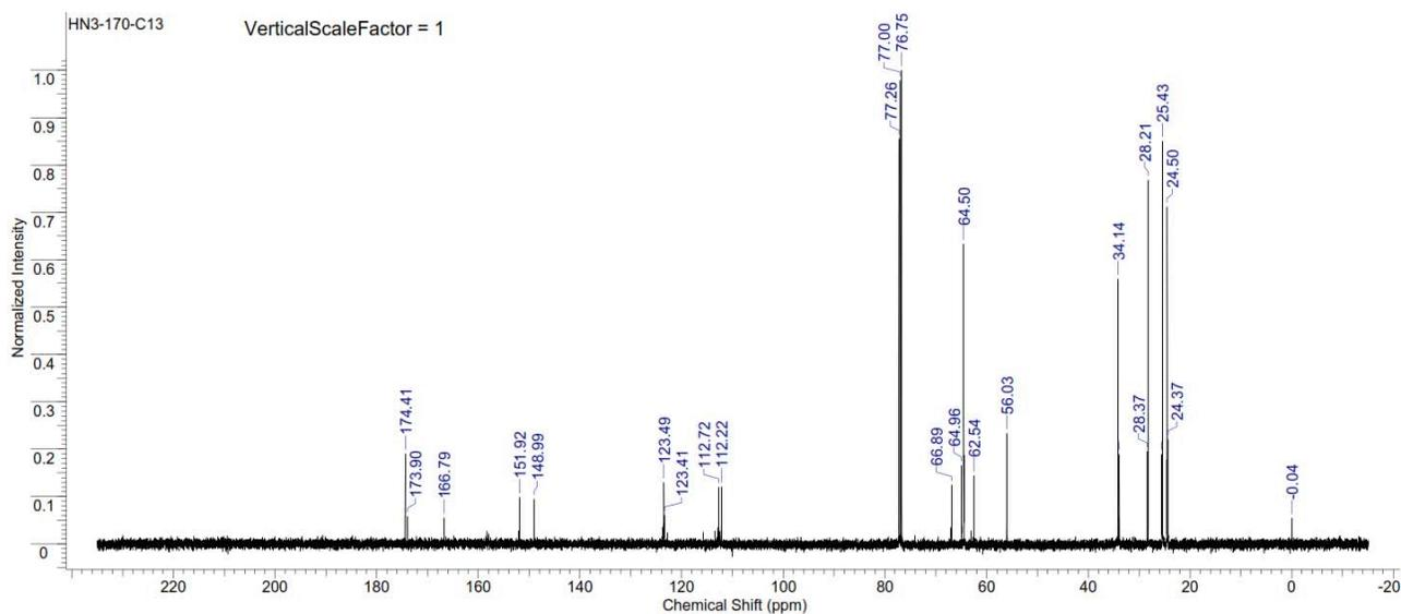
Figure S321.  $^{13}\text{C}$  NMR spectrum of copoly(caprolactone/ hydroxyethylvanillic acid) [80:20] (Table S2, entry 13).
