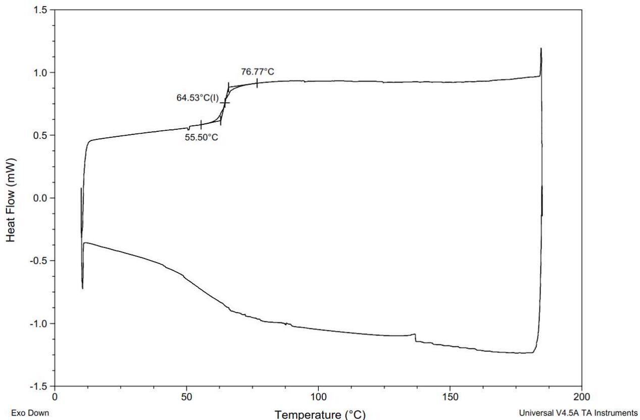
**Figure S135.** DSC Thermogram of copoly(L-lactide/ hydroxyethylcoumaric acid) [90:10] (Table S3, entry 18).
