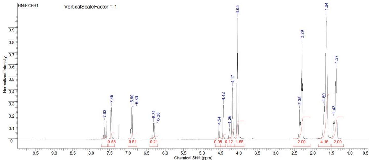
**Figure S264.**  $^1\text{H}$  NMR spectrum of copoly(caprolactone/ hydroxyethylcoumaric acid) [80:20] (Table S2, entry 32).
