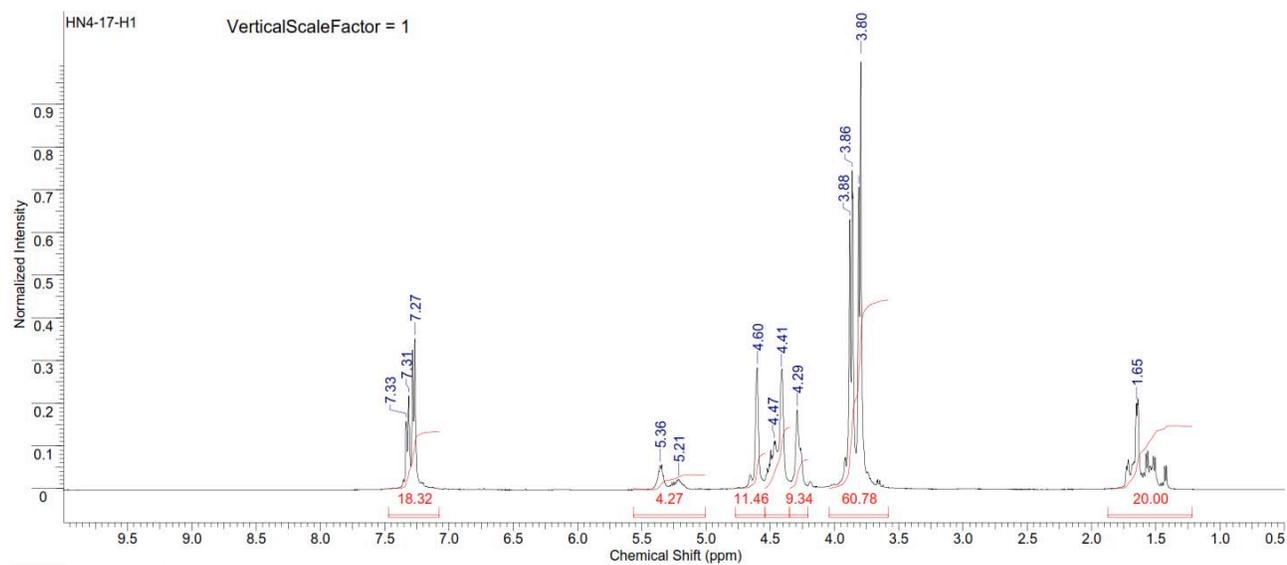
Figure S271. <sup>1</sup>H NMR spectrum of copoly(L-lactide/ hydroxyethylsyngic acid) [40:60] (Table S3, entry 4).
