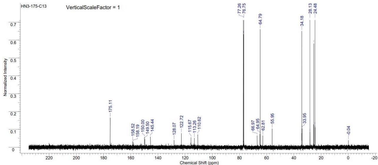
Figure S327.  $^{13}\text{C}$  NMR spectrum of copoly(caprolactone/ hydroxyethylferulic acid) [90:10] (Table S2, entry 22).
