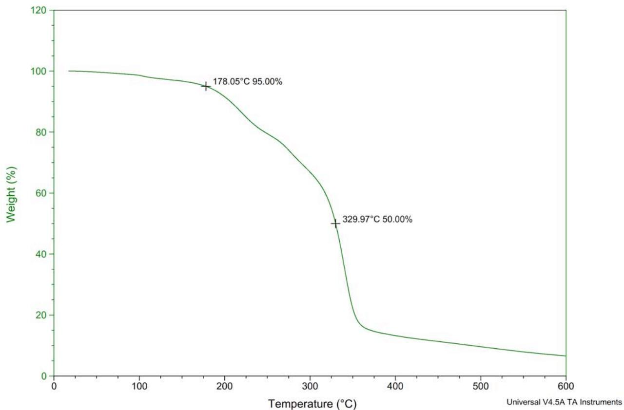
Figure S212. TGA Thermogram of copoly(caprolactone/ hydroxyethylsyngic acid) [50:50] at 10 min. (Table S4, entry 1).
