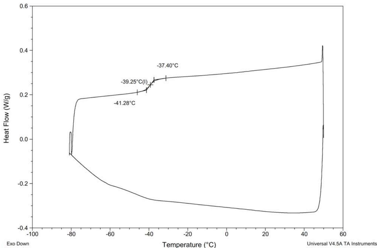
**Figure S140.** DSC Thermogram of copoly(caprolactone/ hydroxyethylsyngic acid) [50:50] at 10 min. (Table S4, entry 1).
