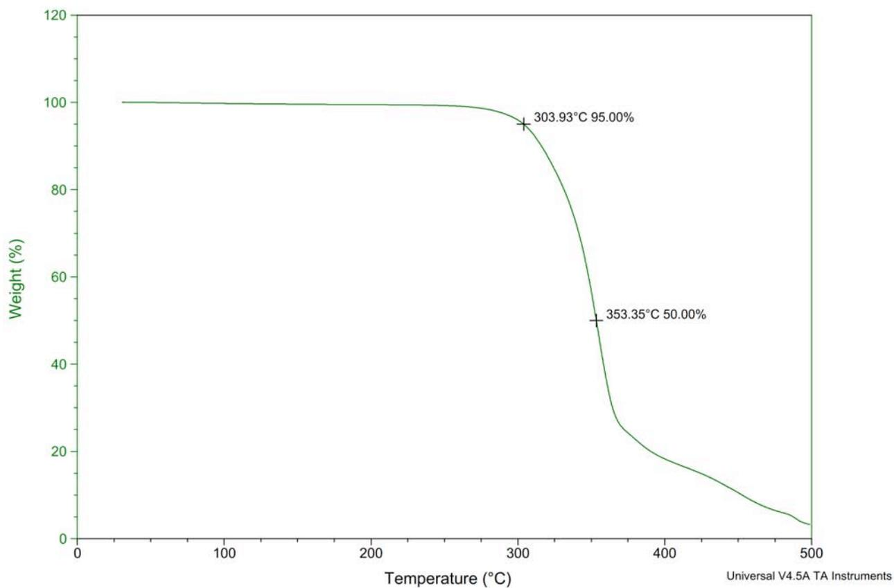
**Figure S226.** TGA Thermogram of copoly(caprolactone/ hydroxyethylsyngic acid) [50:50] at 8 hours (Table S4, entry 15).
