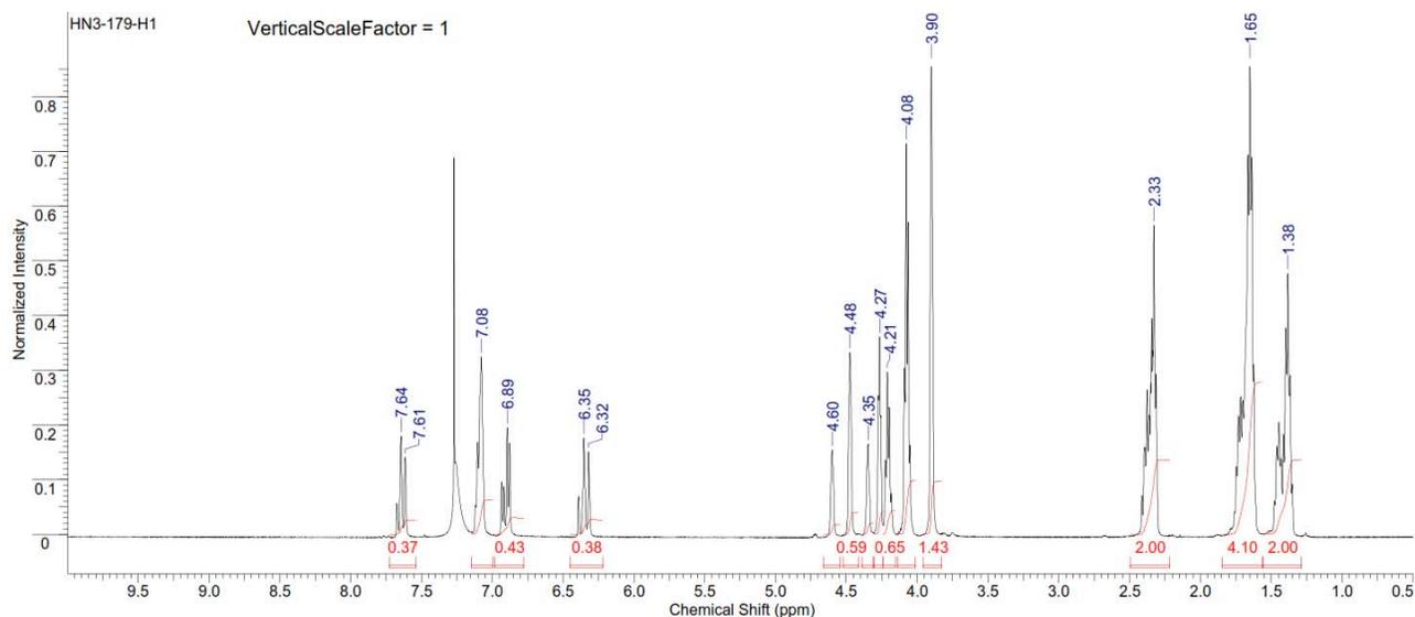
Figure S256. <sup>1</sup>H NMR spectrum of copoly(caprolactone/ hydroxyethylferulic acid) [70:30] (Table S2, entry 24).
