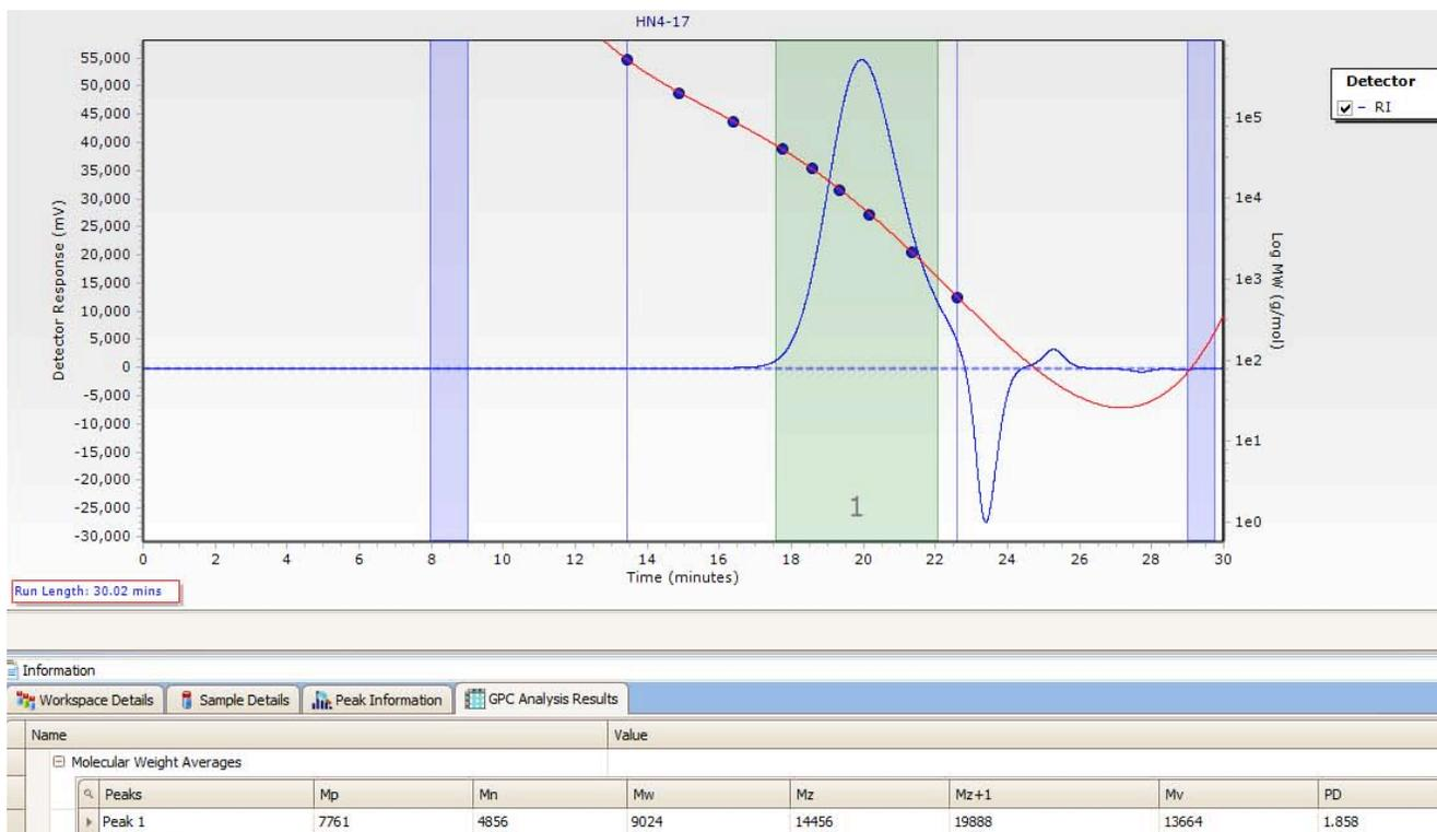
Figure S45. GPC Chromatogram of copoly(L-lactide/ hydroxyethylsyngic acid) [40:60] (Table S3, entry 4).
