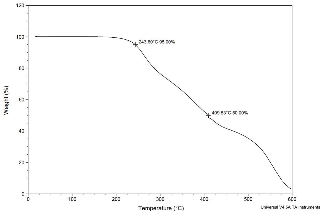
**Figure S210.** TGA Thermogram of copoly(L-lactide/ hydroxyethylcoumaric acid) [60:40] (Table S3, entry 21).
