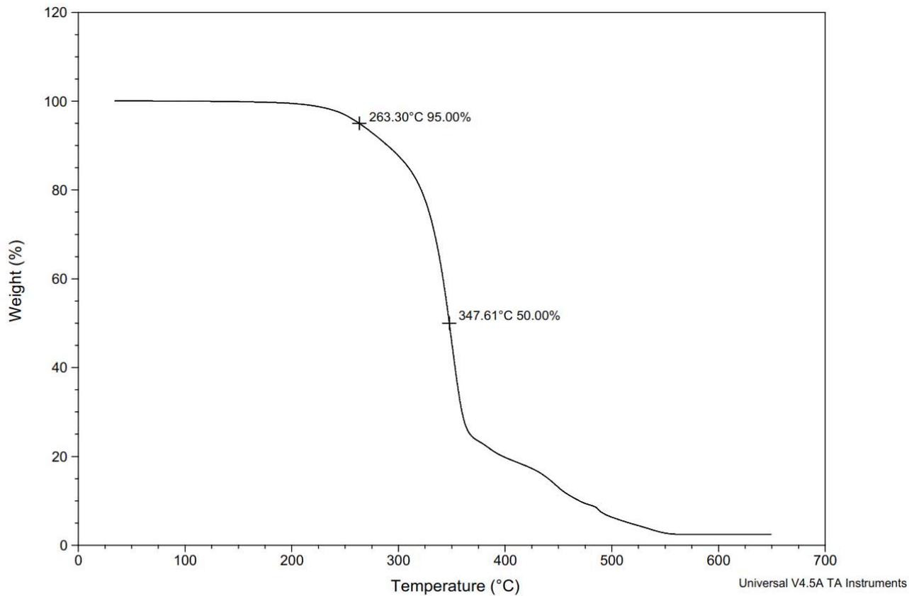
Figure S196. TGA Thermogram of copoly(L-lactide/ hydroxyethylsyngic acid) [40:60] (Table S3, entry 4).
