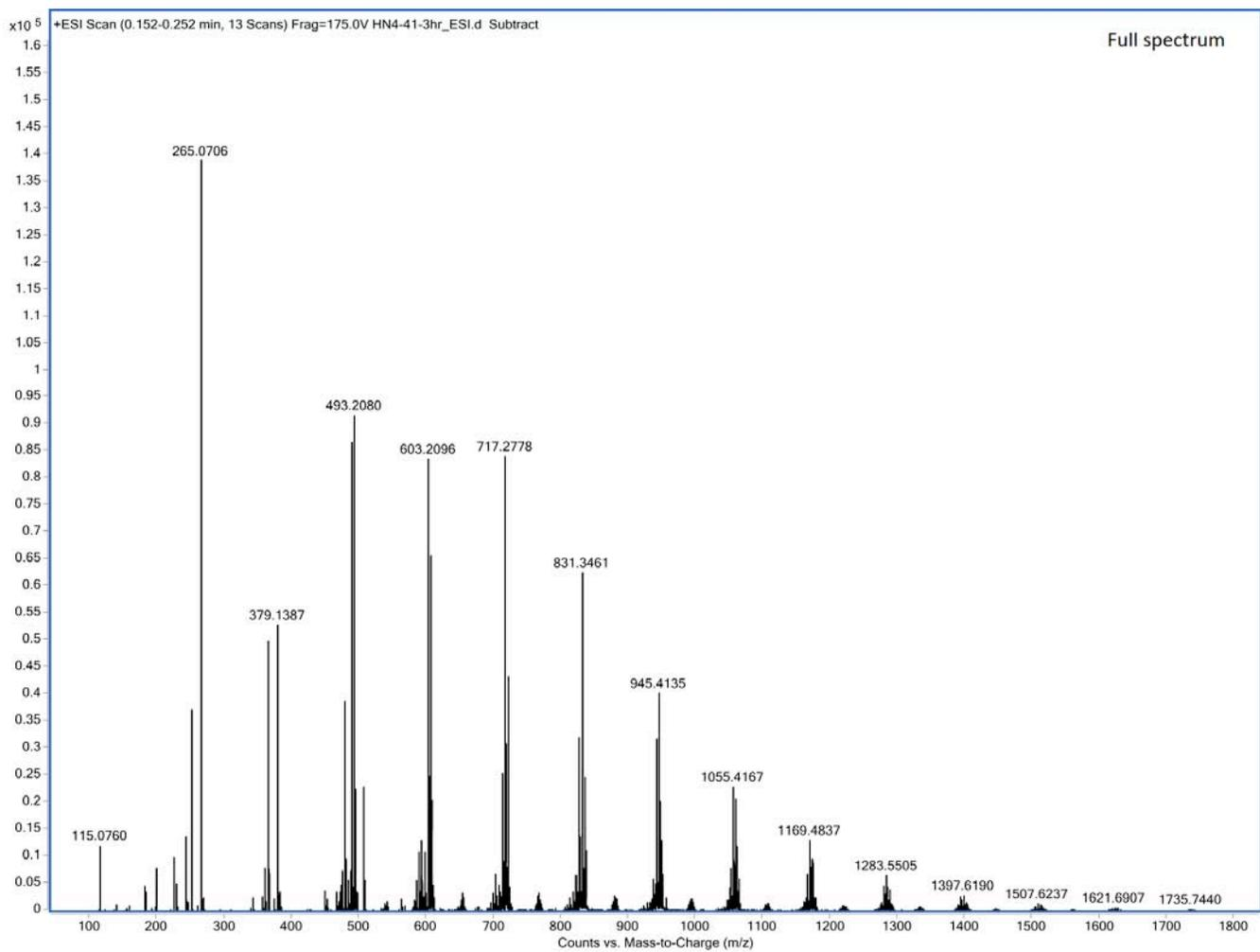
Figure S387. ESI spectra of copoly(caprolactone/hydroxyethylsyngic acid) [50:50] at 3 hours (Table S4, entry 8)
