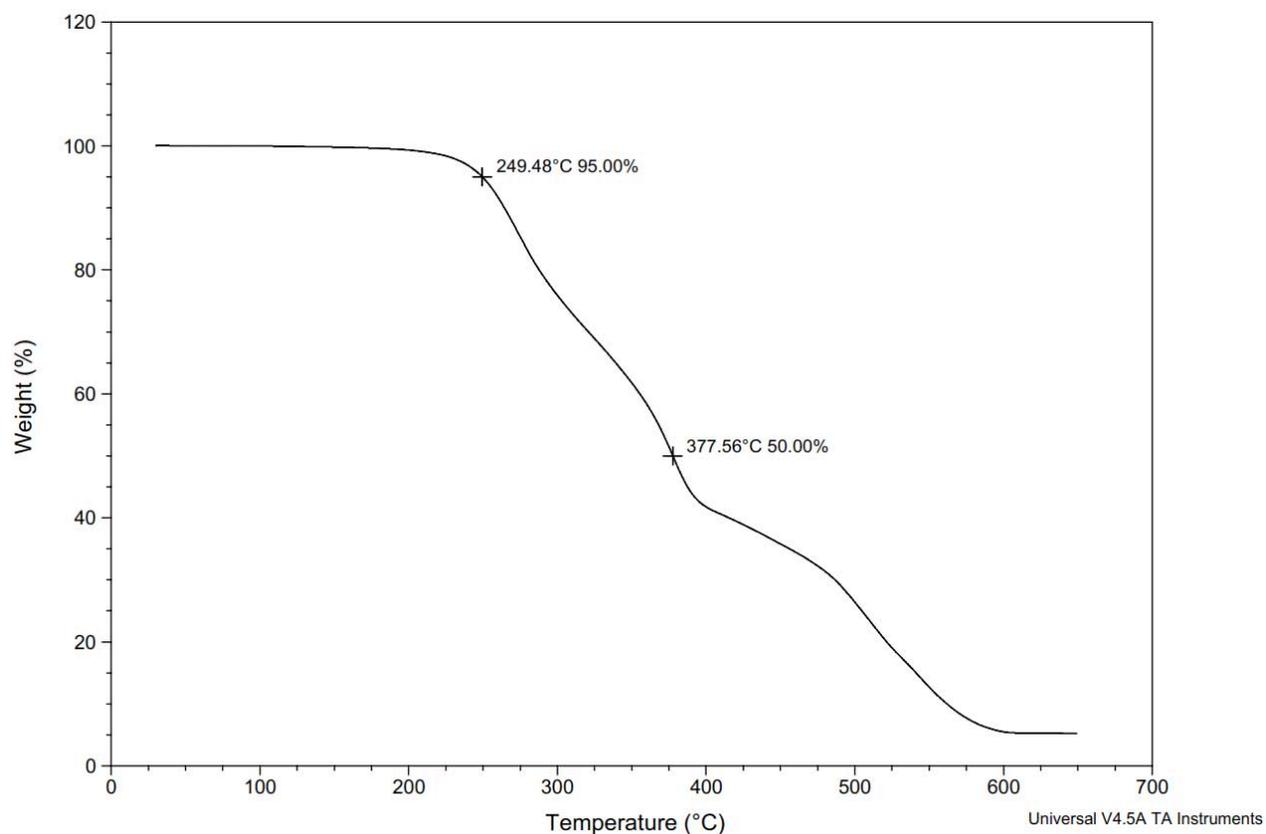
**Figure S205.** TGA Thermogram of copoly(L-lactide/ hydroxyethylferulic acid) [60:40] (Table S3, entry 15).
