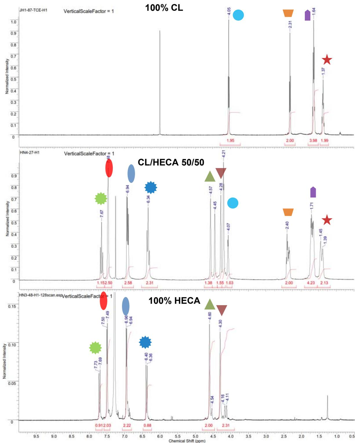
**Figure S375.** <sup>1</sup>H NMR spectra of copoly(caprolactone/hydroxyethylcoumaric acid) with hydroxyethylcoumaric acid (HECA) feed fractions of 0%, 50%, and 100%.
