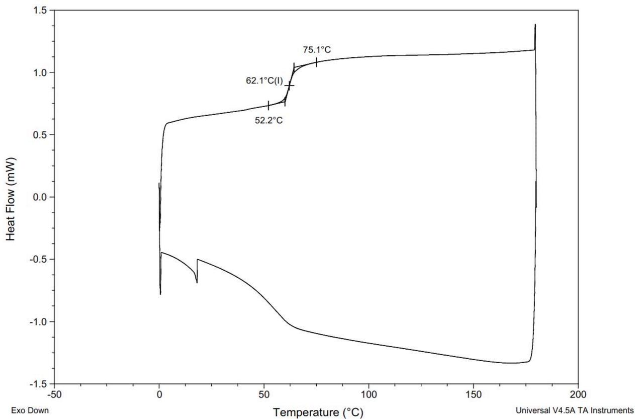
**Figure S122.** DSC Thermogram of copoly(L-lactide/ hydroxyethylsyngic acid) [80:20] (Table S3, entry 2).
