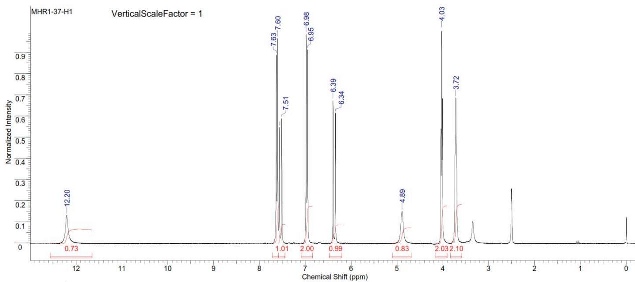
Figure S231. <sup>1</sup>H NMR spectrum of hydroxyethylcoumaric acid.
