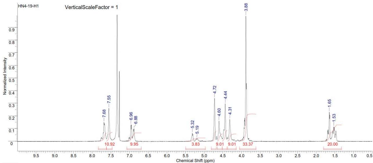
**Figure S276.**  $^1\text{H}$  NMR spectrum of copoly(L-lactide/ hydroxyethylvanillic acid) [20:80] (Table S3, entry 10).
