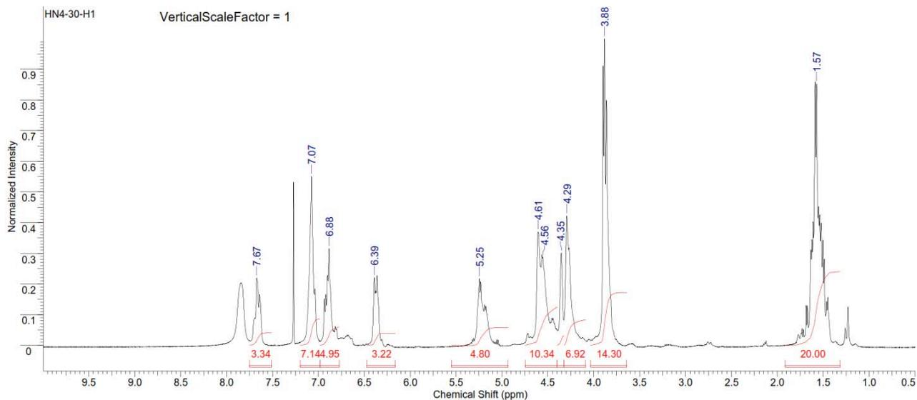
Figure S280. <sup>1</sup>H NMR spectrum of copoly(L-lactide/ hydroxyethylferulic acid) [60:40] (Table S3, entry 15).
