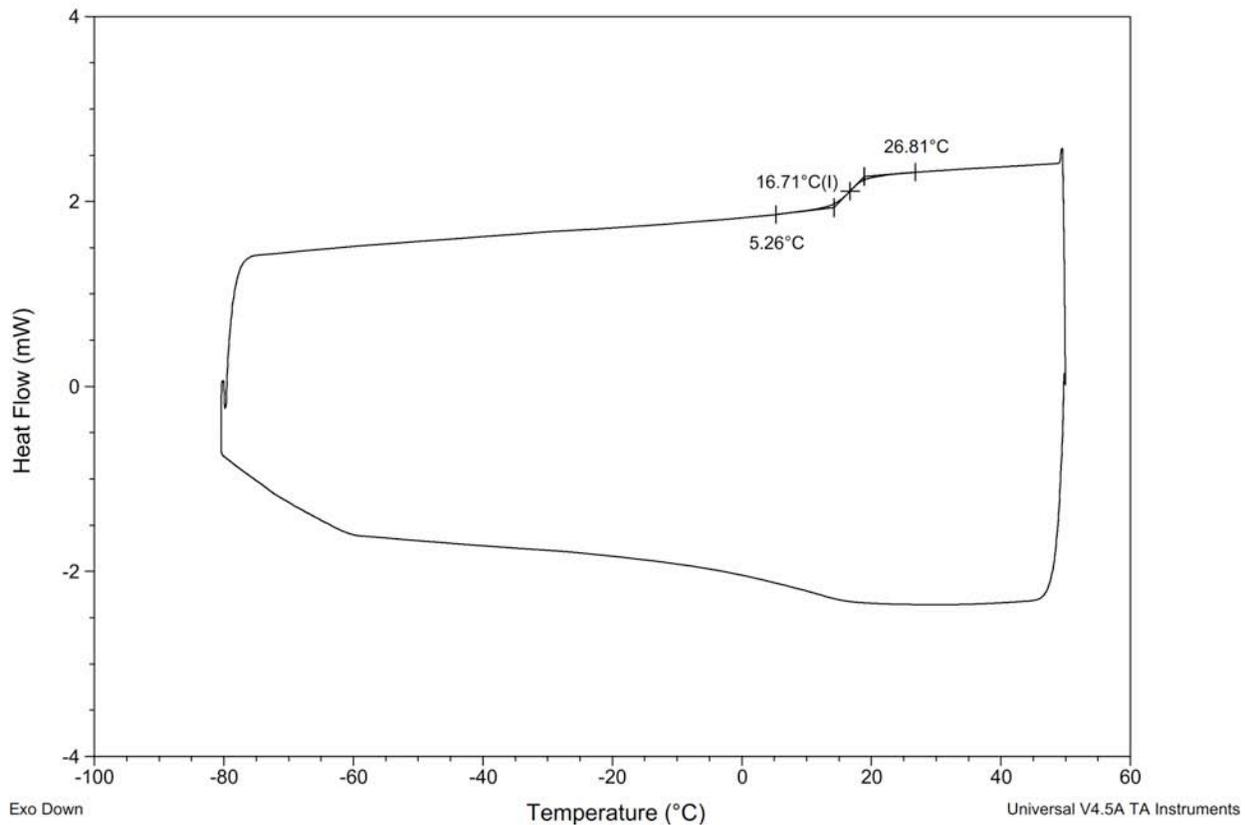
**Figure S155.** DSC Thermogram of copoly(caprolactone/ hydroxyethylsyngic acid) [50:50] at 9 hours (Table S4, entry 16).
