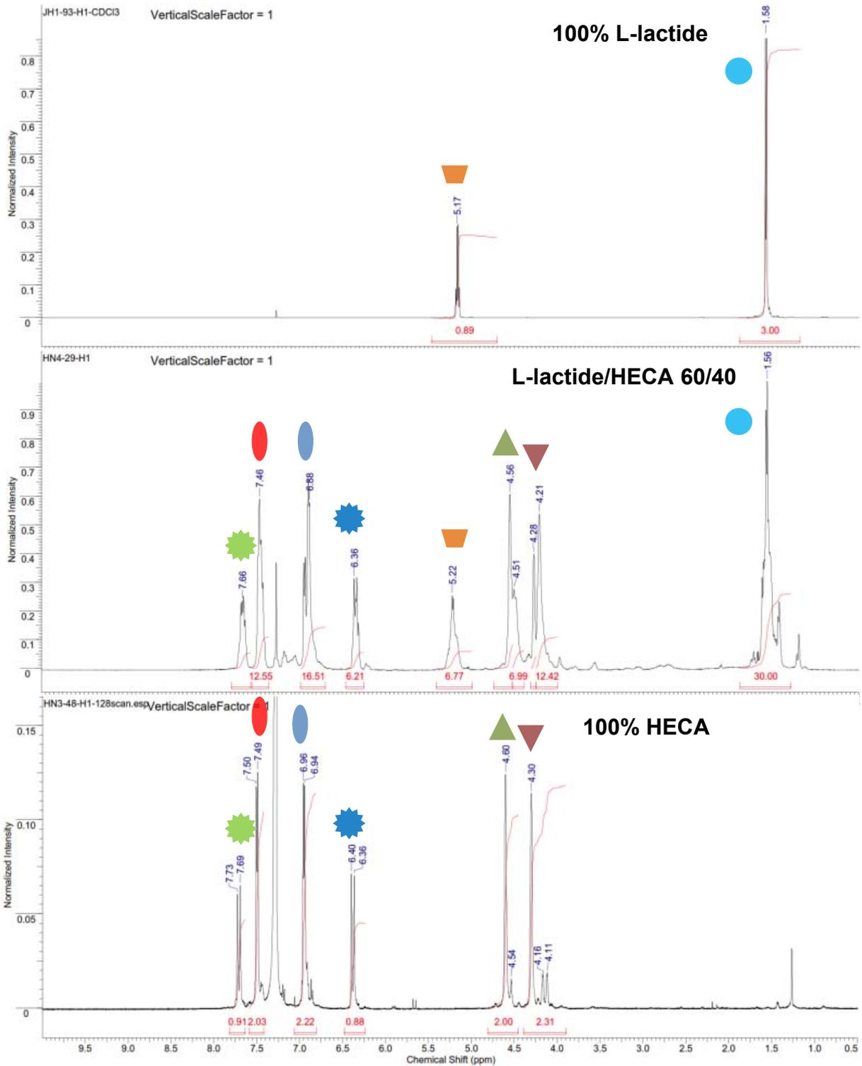
**Figure S379.**  $^1\text{H}$  NMR spectra of copoly(L-lactide/hydroxyethylcoumaric acid) with hydroxyethylcoumaric acid (HECA) feed fractions of 0%, 40%, and 100%.
