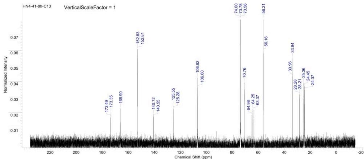
Figure S368.  $^{13}\text{C}$  NMR spectrum of copoly(caprolactone/ hydroxyethylsyringic acid) [50:50] at 8 hours (Table S4, entry 15).
