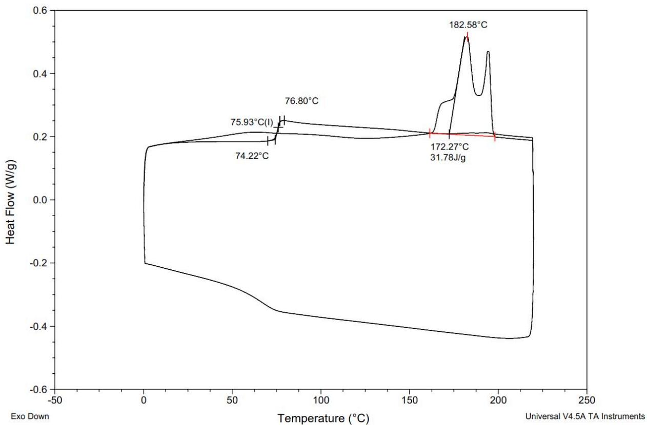
**Figure S96.** DSC Thermogram of polyethylene syringate (Table S2, entry 11).
