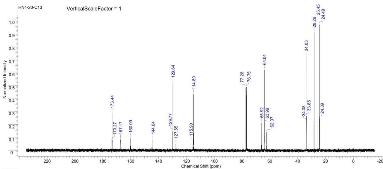
Figure S335.  $^{13}\text{C}$  NMR spectrum of copoly(caprolactone/ hydroxyethylcoumaric acid) [80:20] (Table S2, entry 32).
