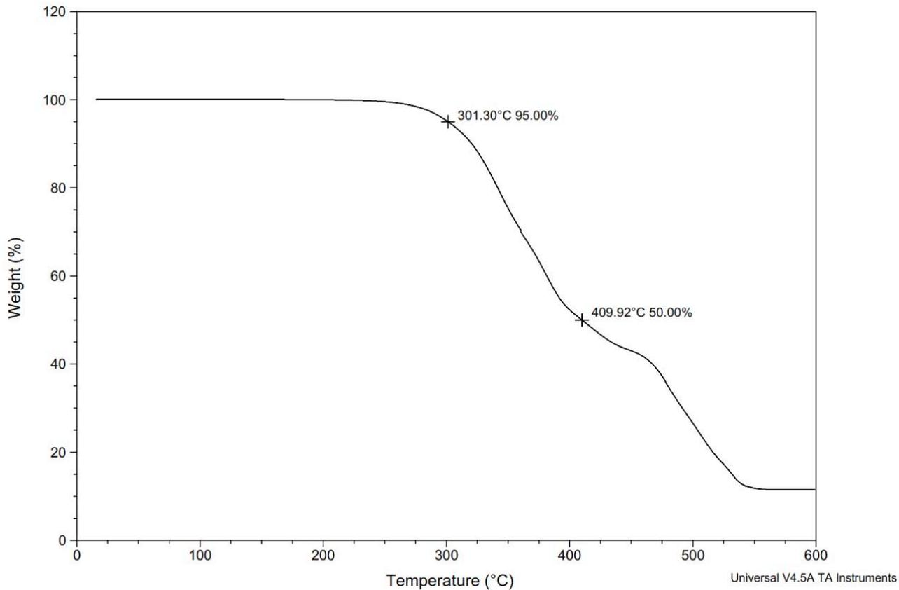
**Figure S184.** TGA Thermogram of copoly(caprolactone/ hydroxyethylferulic acid) [40:60] (Table S3, entry 37).
