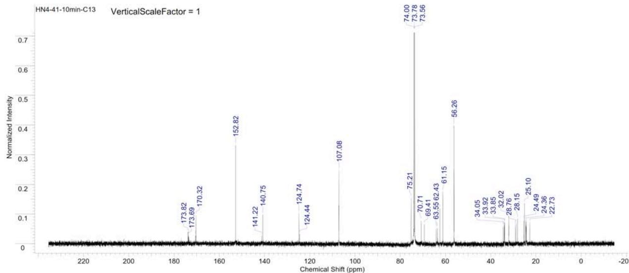
Figure S354.  $^{13}\text{C}$  NMR spectrum of copoly(caprolactone/ hydroxyethylsyringic acid) [50:50] at 10 min. (Table S4, entry 1).
