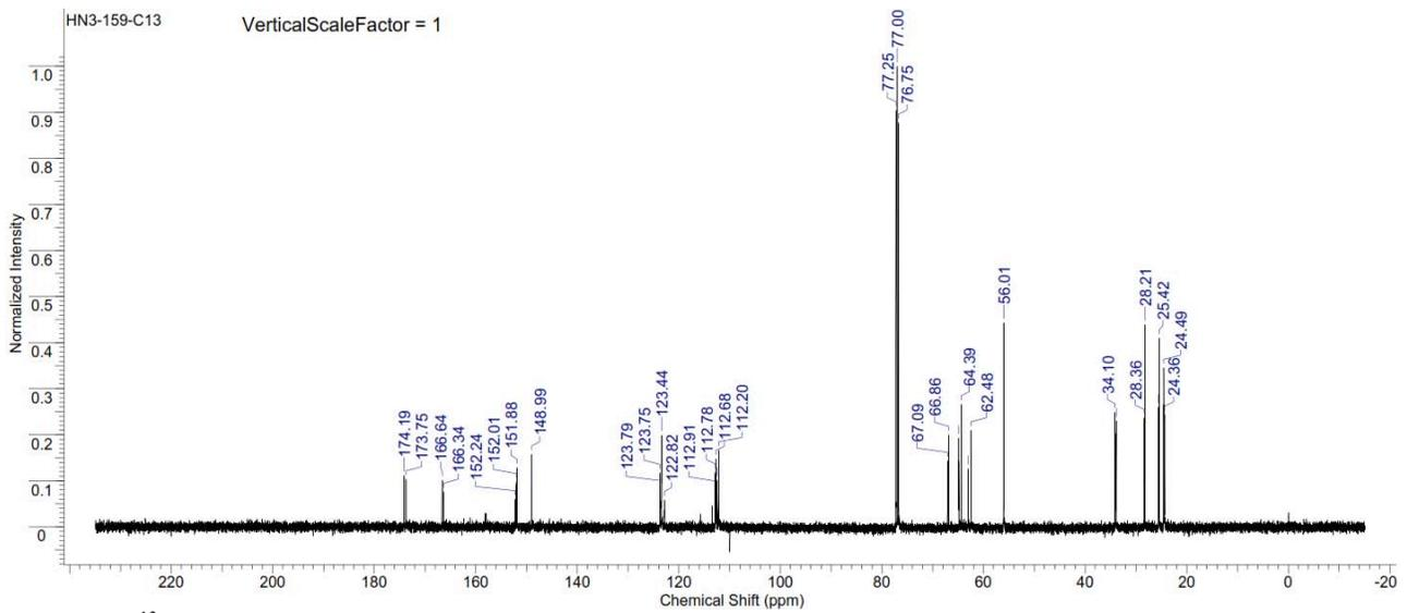
Figure S323.  $^{13}\text{C}$  NMR spectrum of copoly(caprolactone/ hydroxyethylvanillic acid) [60:40] (Table S2, entry 15).
