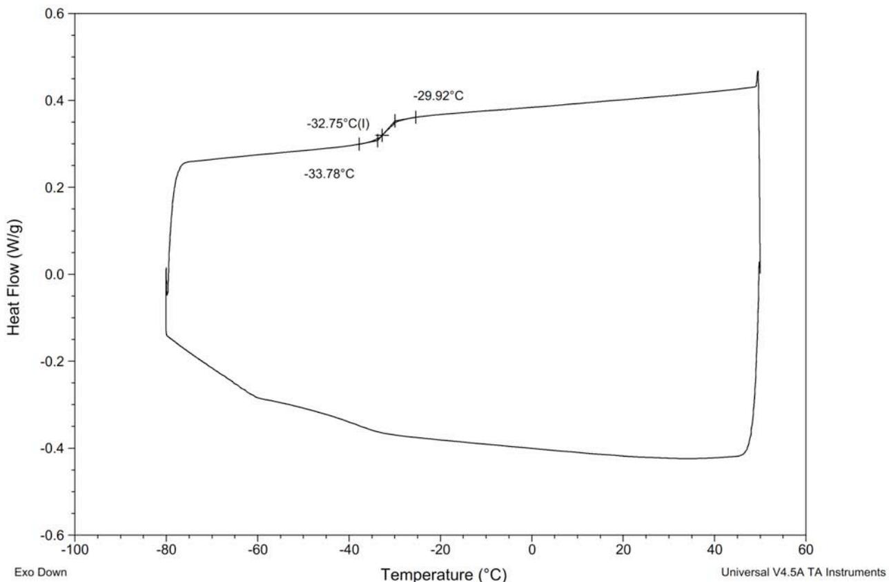
**Figure S142.** DSC Thermogram of copoly(caprolactone/ hydroxyethylsyningic acid) [50:50] at 30 min. (Table S4, entry 3).
