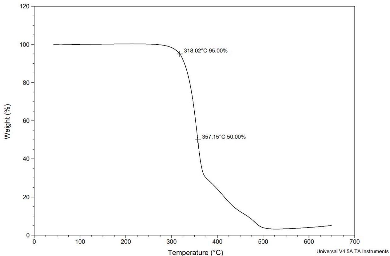
**Figure S168.** TGA Thermogram of polyethylene synringate (Table S2, entry 11).
