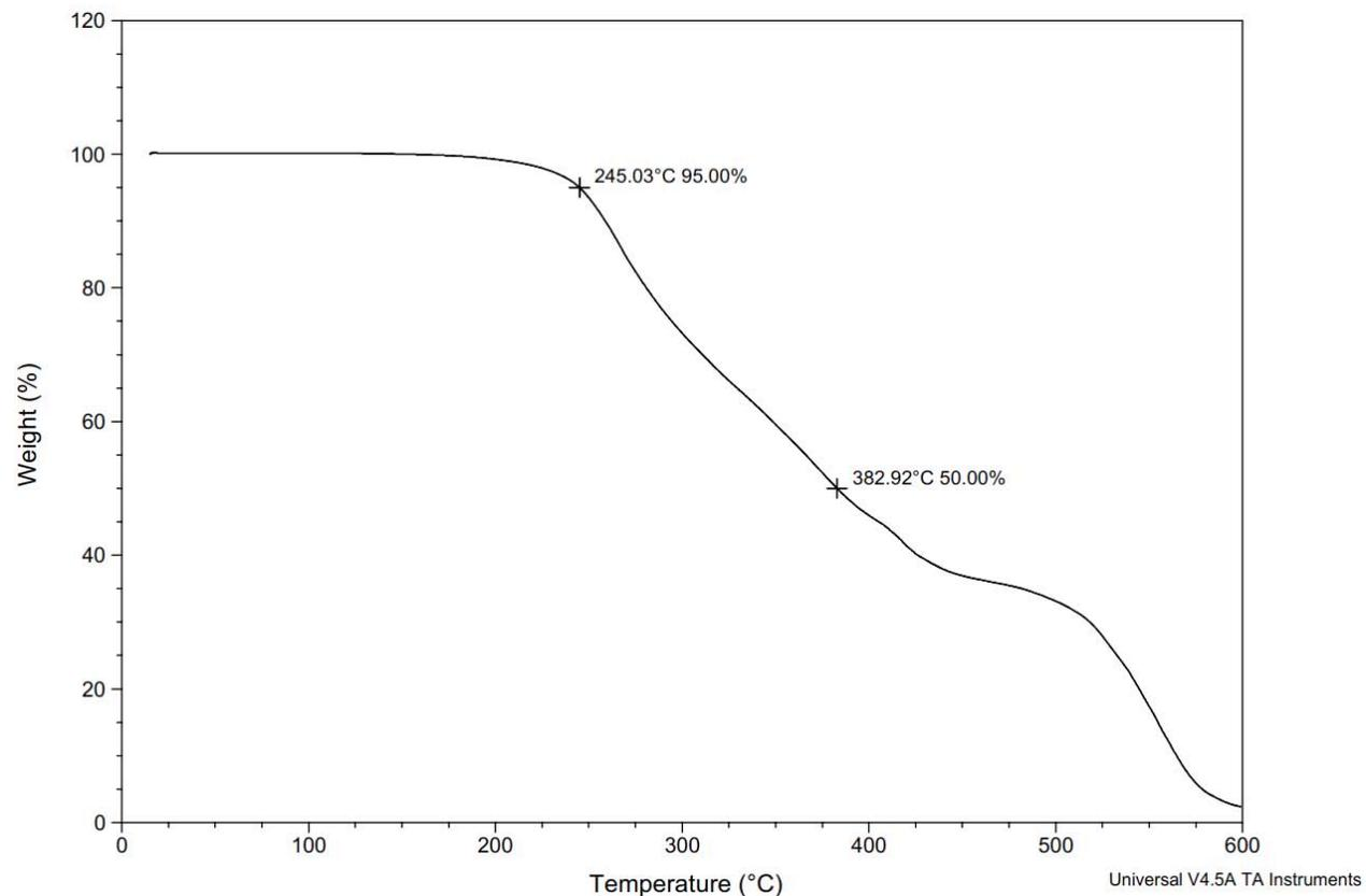
**Figure S209.** TGA Thermogram of copoly(L-lactide/ hydroxyethylcoumaric acid) [70:30] (Table S3, entry 20).
