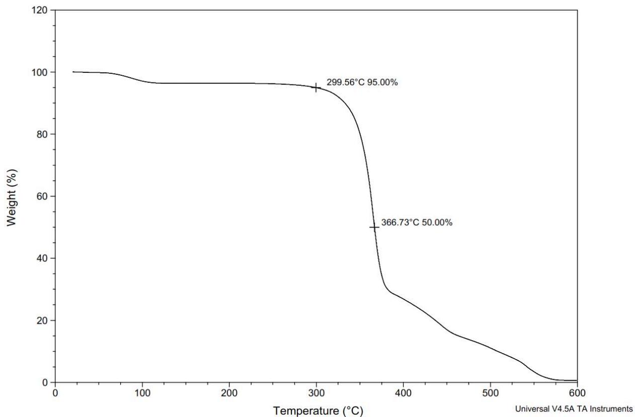
**Figure S167.** TGA Thermogram of copoly(caprolactone/ hydroxyethylsyngic acid) [10:90] (Table S2, entry 10).
