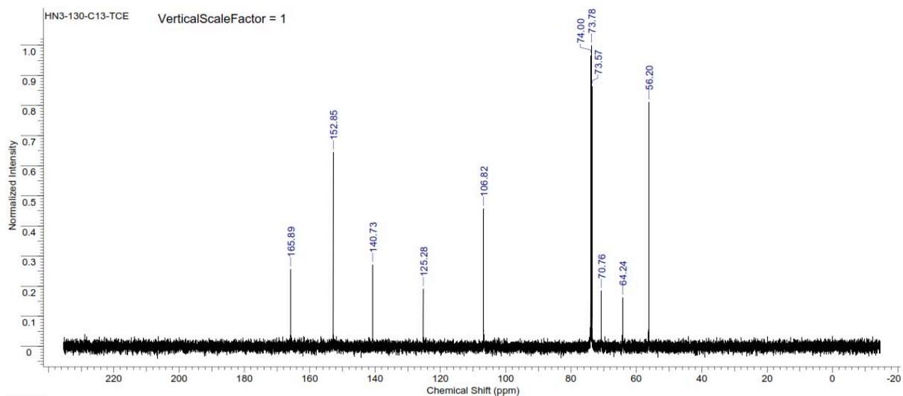
Figure S319.  $^{13}\text{C}$  NMR spectrum of polyethylene syringate (Table S2, entry 11).
