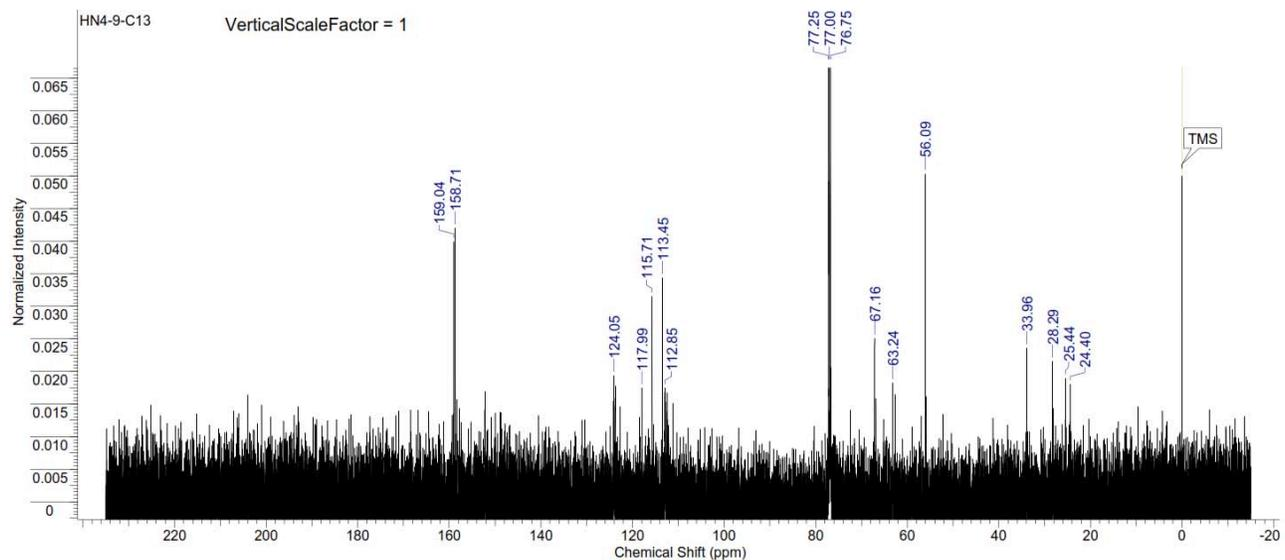
Figure S326.  $^{13}\text{C}$  NMR spectrum of copoly(caprolactone/ hydroxyethylvanillic acid) [30:70] (Table S2, entry 18).
