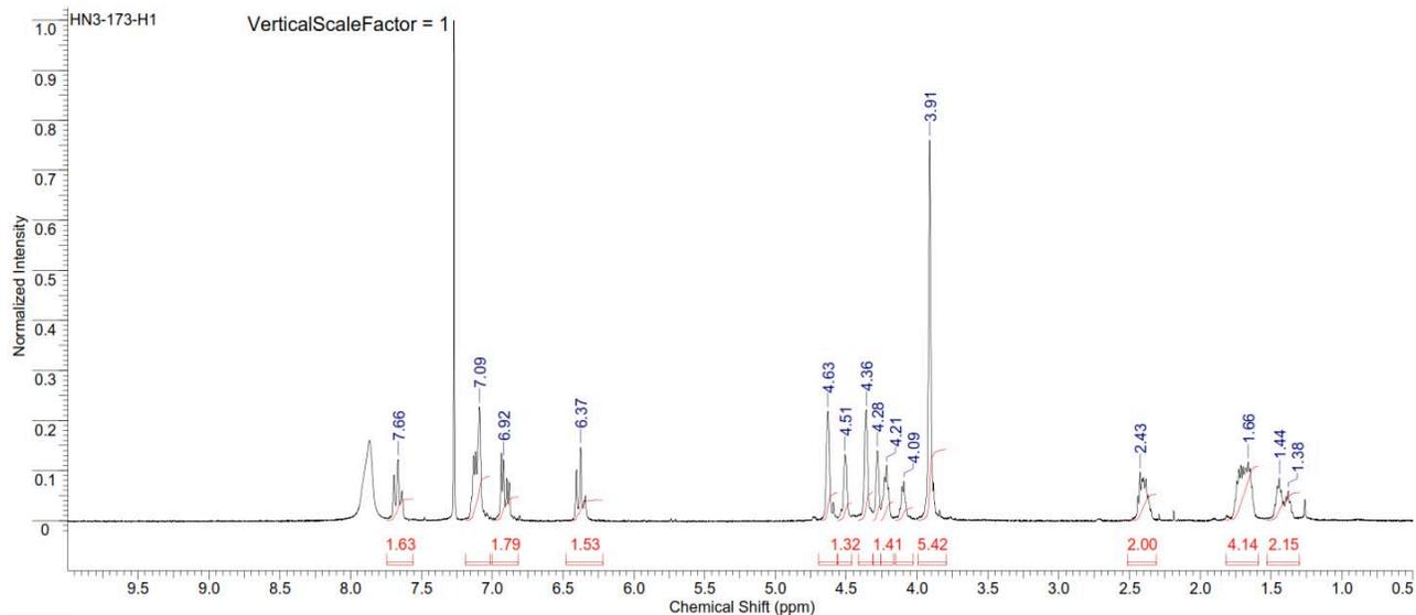
Figure S258.  $^1\text{H}$  NMR spectrum of copoly(caprolactone/ hydroxyethylferulic acid) [50:50] (Table S2, entry 26).
