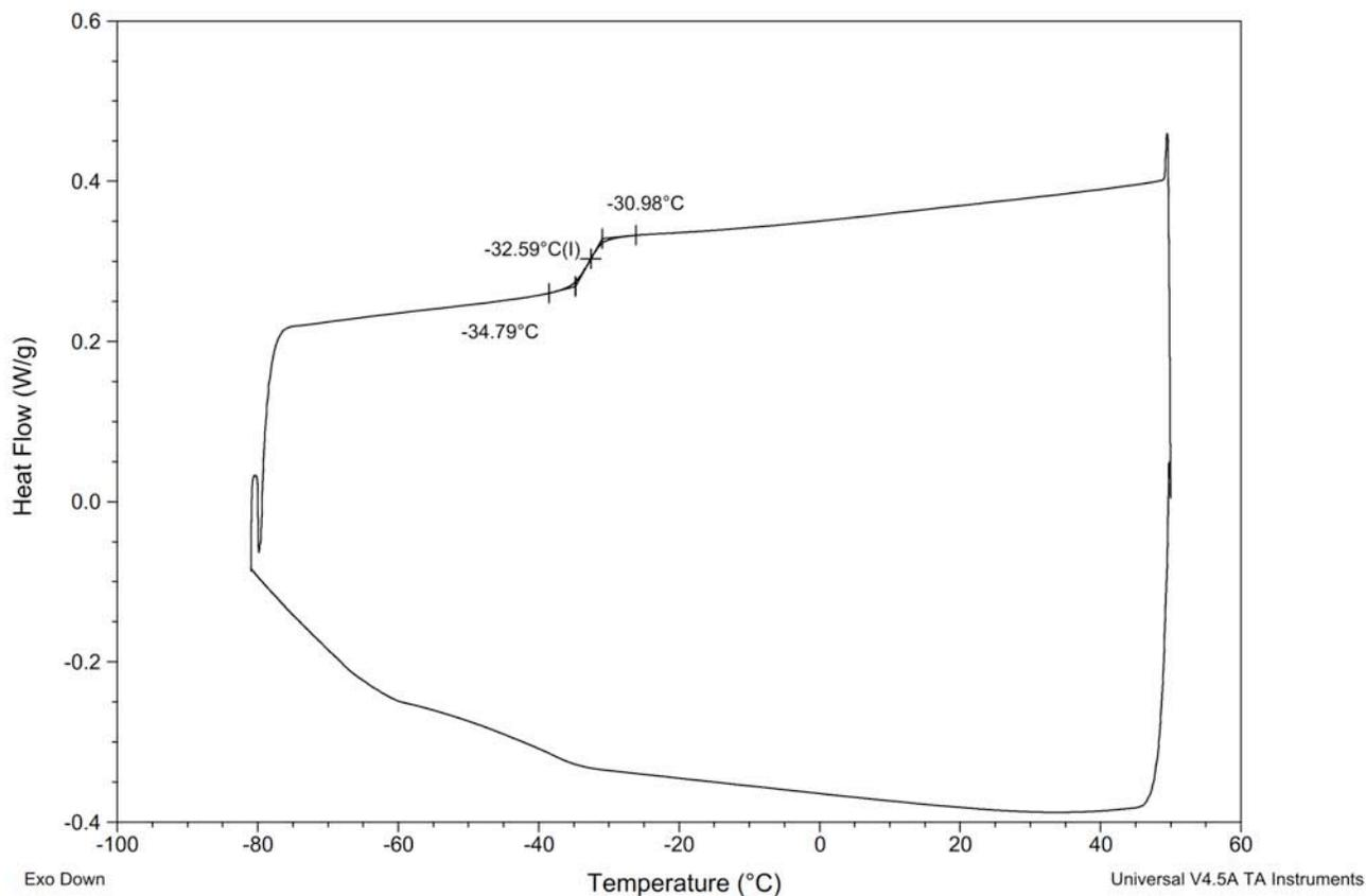
**Figure S141.** DSC Thermogram of copoly(caprolactone/ hydroxyethylsyningic acid) [50:50] at 20 min. (Table S4, entry 2).
