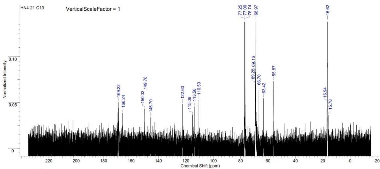
Figure S346. <sup>13</sup>C NMR spectrum of copoly(L-lactide/ hydroxyethylferulic acid) [90:10] (Table S3, entry 12).
