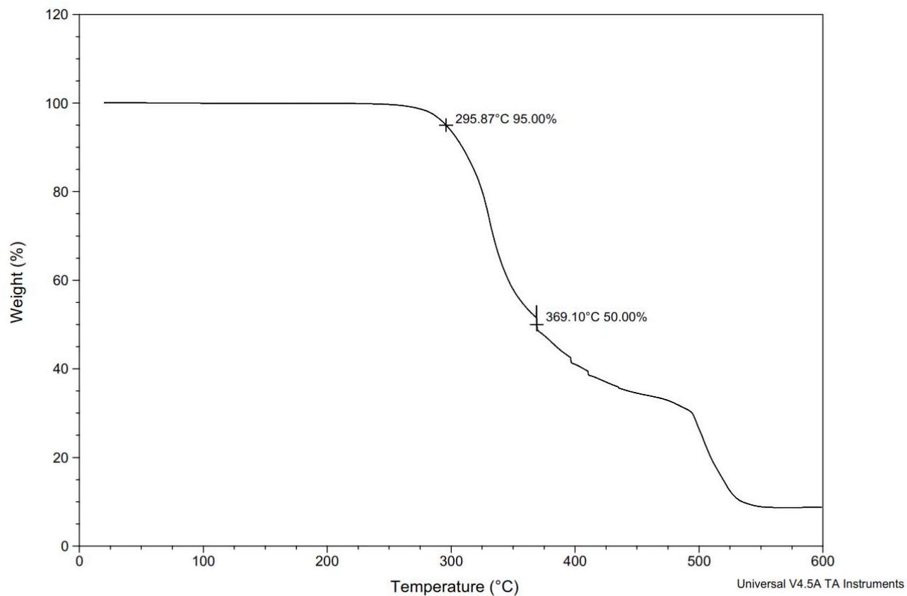
**Figure S182.** TGA Thermogram of copoly(caprolactone/ hydroxyethylferulic acid) [60:40] (Table S2, entry 25).
