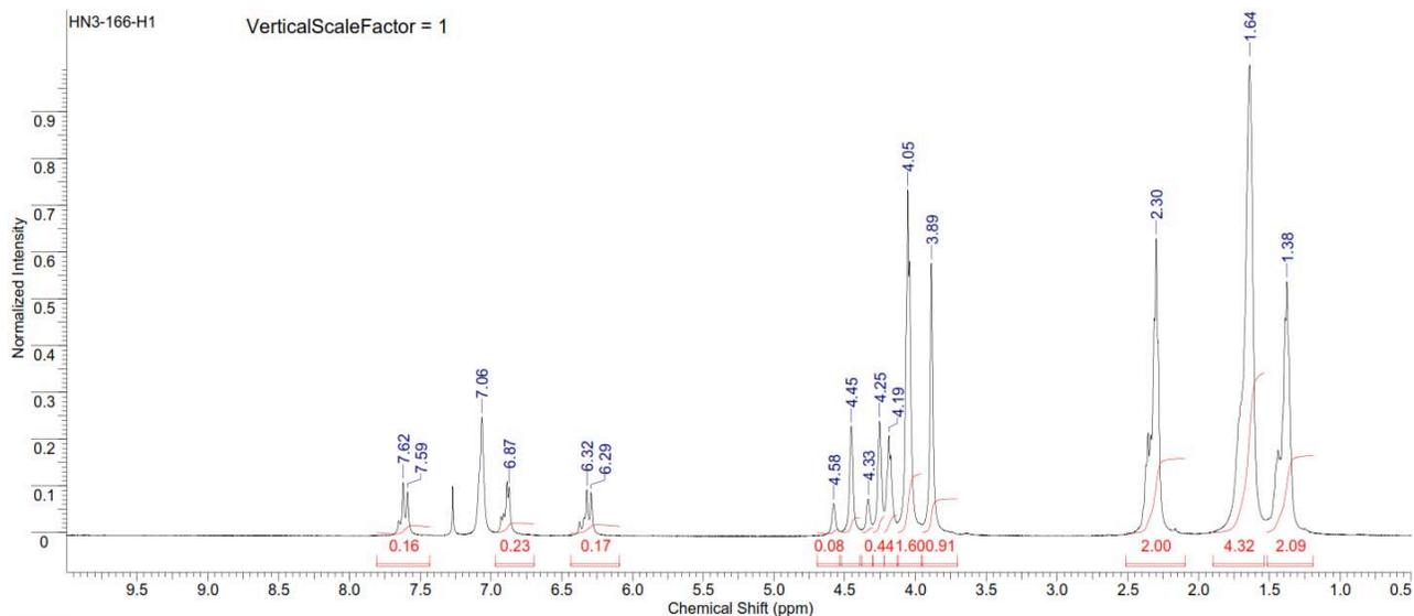
Figure S255. <sup>1</sup>H NMR spectrum of copoly(caprolactone/ hydroxyethylferulic acid) [80:20] (Table S2, entry 23).
