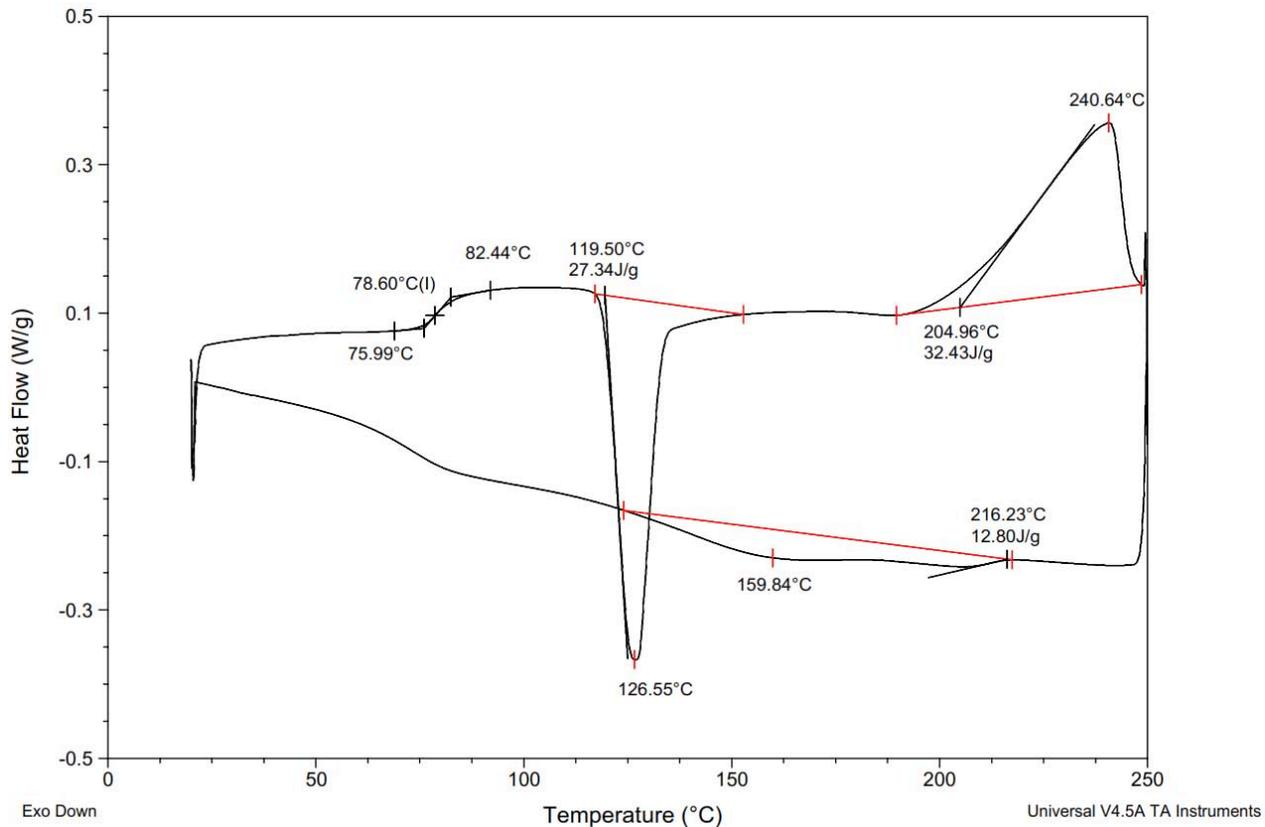
**Figure S129.** DSC Thermogram of copoly(L-lactide/ hydroxyethylvanillic acid) [20:80] (Table S3, entry 9).
