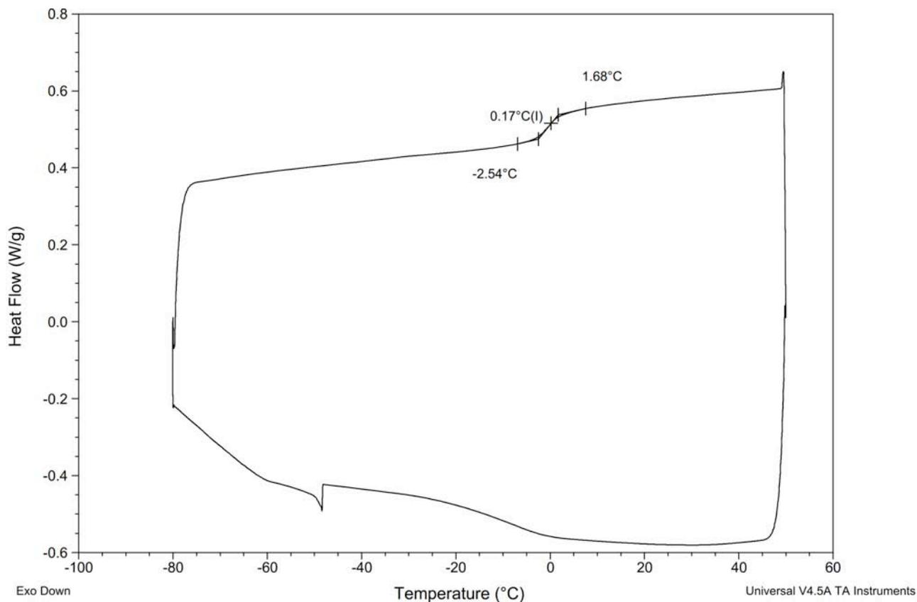
**Figure S148.** DSC Thermogram of copoly(caprolactone/ hydroxyethylsyngic acid) [50:50] at 3.5 hours (Table S4, entry 9).
