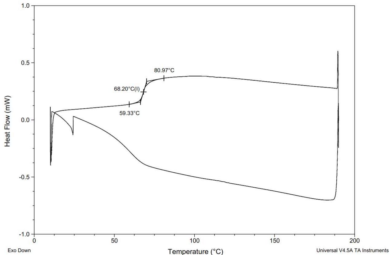
**Figure S123.** DSC Thermogram of copoly(L-lactide/ hydroxyethylsyringic acid) [60:40] (Table S3, entry 3).
