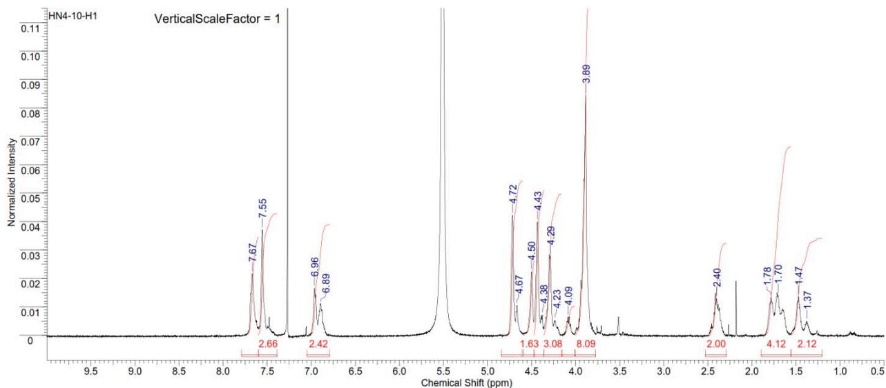
Figure S252. <sup>1</sup>H NMR spectrum of copoly(caprolactone/ hydroxyethylvanillic acid) [20:80] (Table S2, entry 19).
