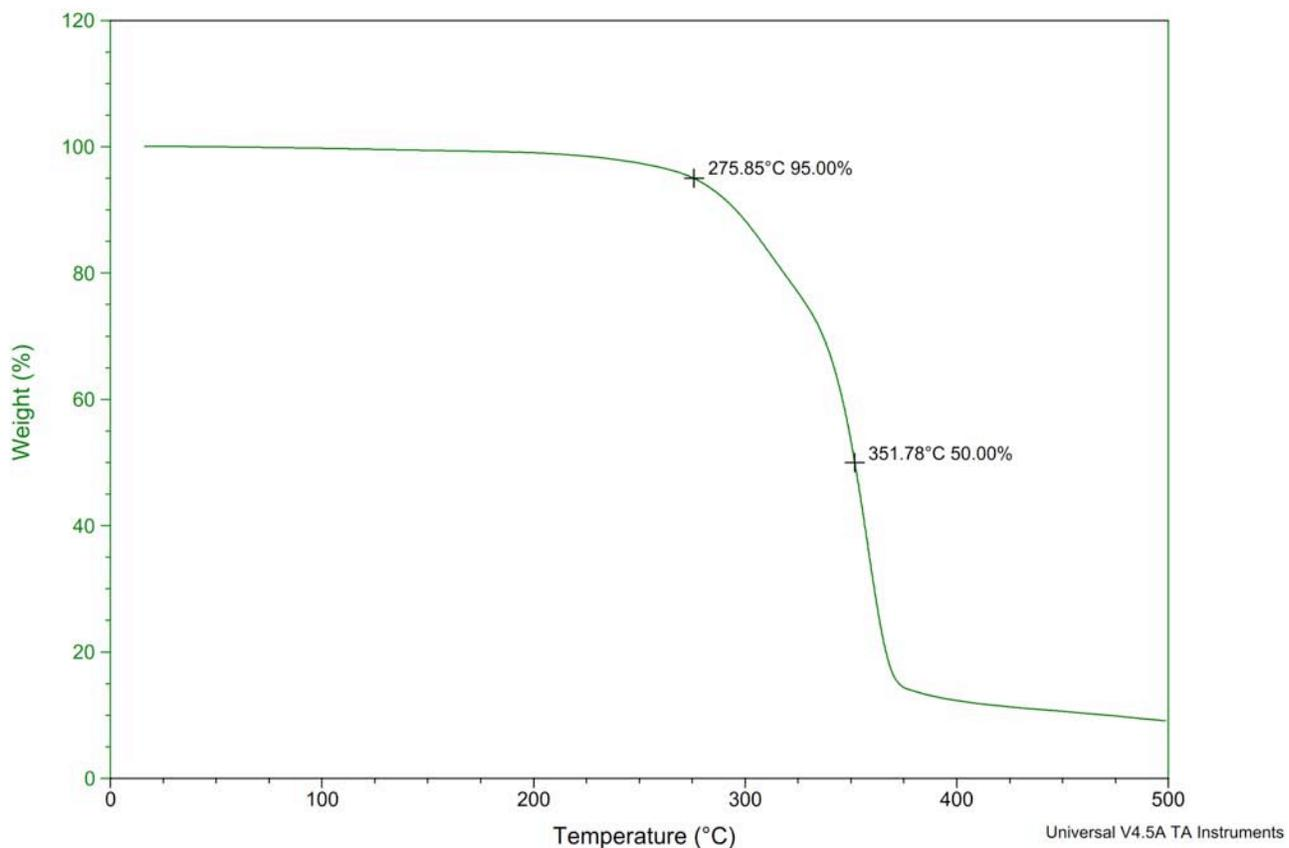
**Figure S223.** TGA Thermogram of copoly(caprolactone/ hydroxyethylsyringic acid) [50:50] at 5 hours (Table S4, entry 12).
