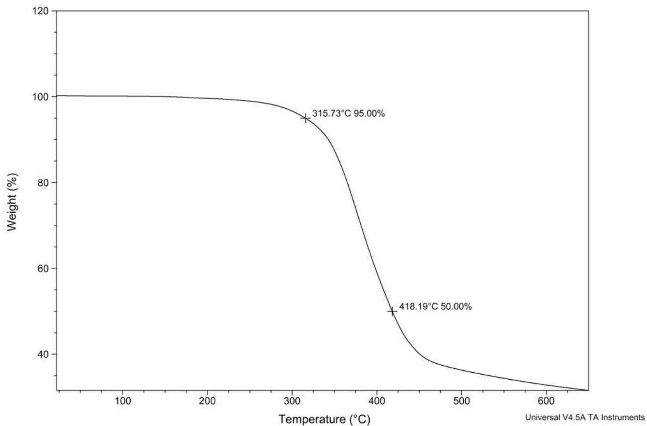
**Figure S211.** TGA Thermogram of copoly(L-lactide/ hydroxyethylcoumaric acid) [20:80] (Table S3, entry 22).
