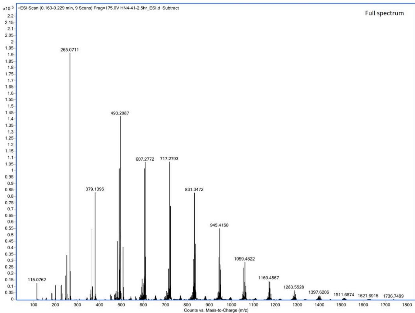
**Figure S386.** ESI spectra of copoly(caprolactone/hydroxyethylsyringic acid) [50:50] at 2.5 hours (Table S4, entry 7)
