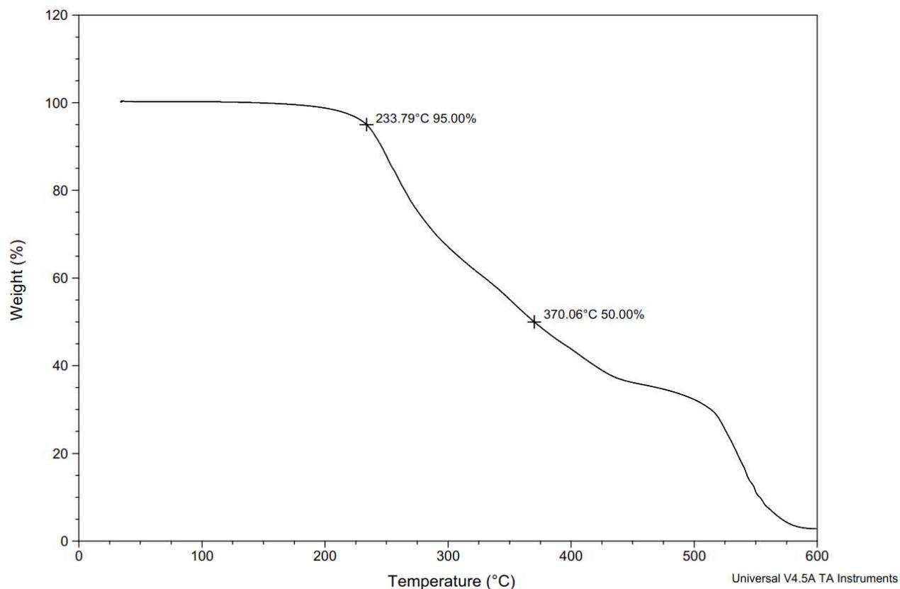
**Figure S208.** TGA Thermogram of copoly(L-lactide/ hydroxyethylcoumaric acid) [80:20] (Table S3, entry 19).
