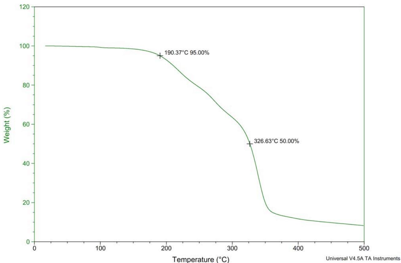
Figure S214. TGA Thermogram of copoly(caprolactone/ hydroxyethylsyngic acid) [50:50] at 30 min. (Table S4, entry 3).
