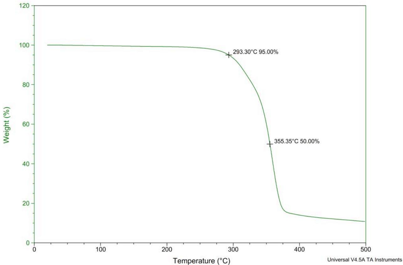
**Figure S224.** TGA Thermogram of copoly(caprolactone/ hydroxyethylsyngic acid) [50:50] at 6 hours (Table S4, entry 13).
