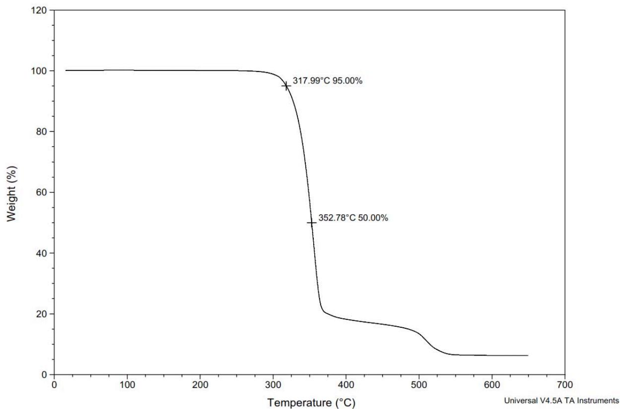
**Figure S177.** TGA Thermogram of copoly(caprolactone/ hydroxyethylvanillic acid) [10:90] (Table S2, entry 20).
