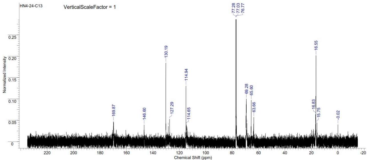
Figure S350. <sup>13</sup>C NMR spectrum of copoly(L-lactide/ hydroxyethylcoumaric acid) [90:10] (Table S3, entry 18).
