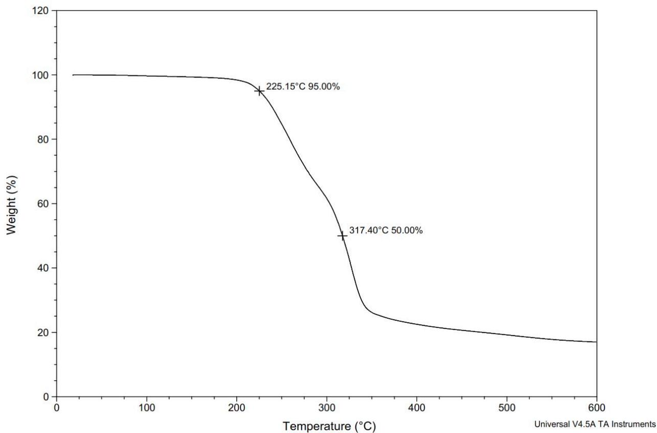
**Figure S194.** TGA Thermogram of copoly(L-lactide/ hydroxyethylsyringic acid) [80:20] (Table S3, entry 2).
