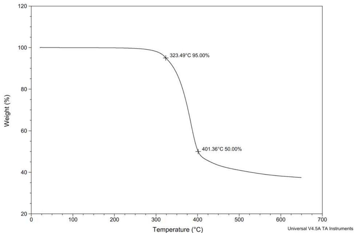
**Figure S206.** TGA Thermogram of copoly(L-lactide/ hydroxyethylferulic acid) [20:80] (Table S3, entry 16).
