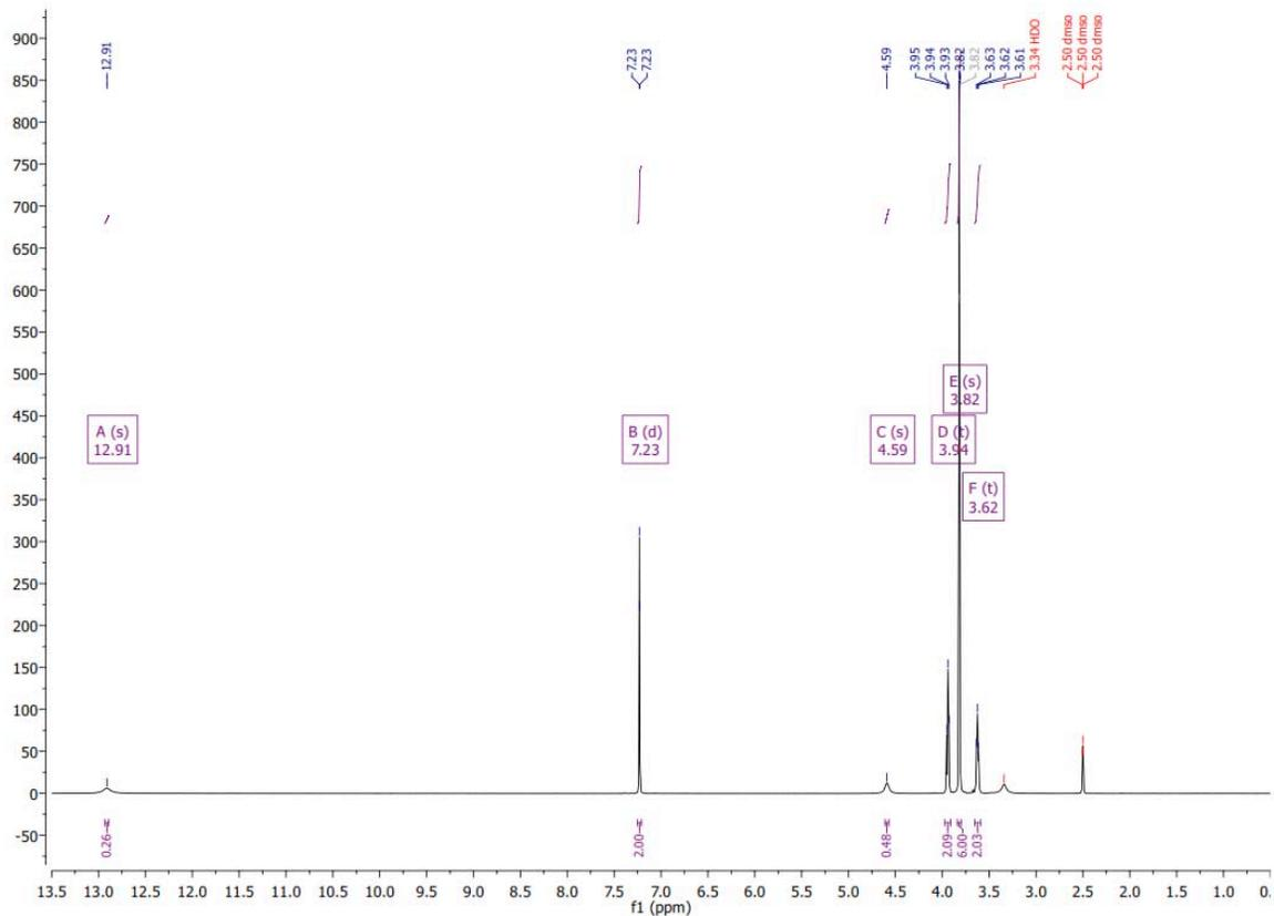
Figure S232. <sup>1</sup>H NMR spectrum of hydroxyethylsyringic acid.
