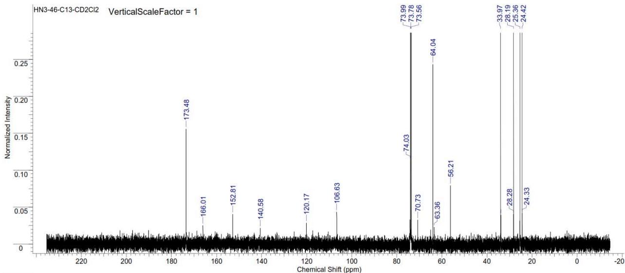
Figure S310. <sup>13</sup>C NMR spectrum of copoly(caprolactone/ hydroxyethylsyringic acid) [90:10] (Table S2, entry 2).
