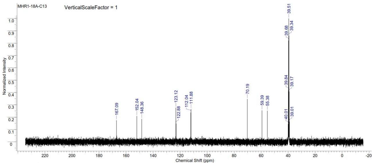
Figure S308.  $^{13}\text{C}$  NMR spectrum of hydroxyethylvanillic acid.
