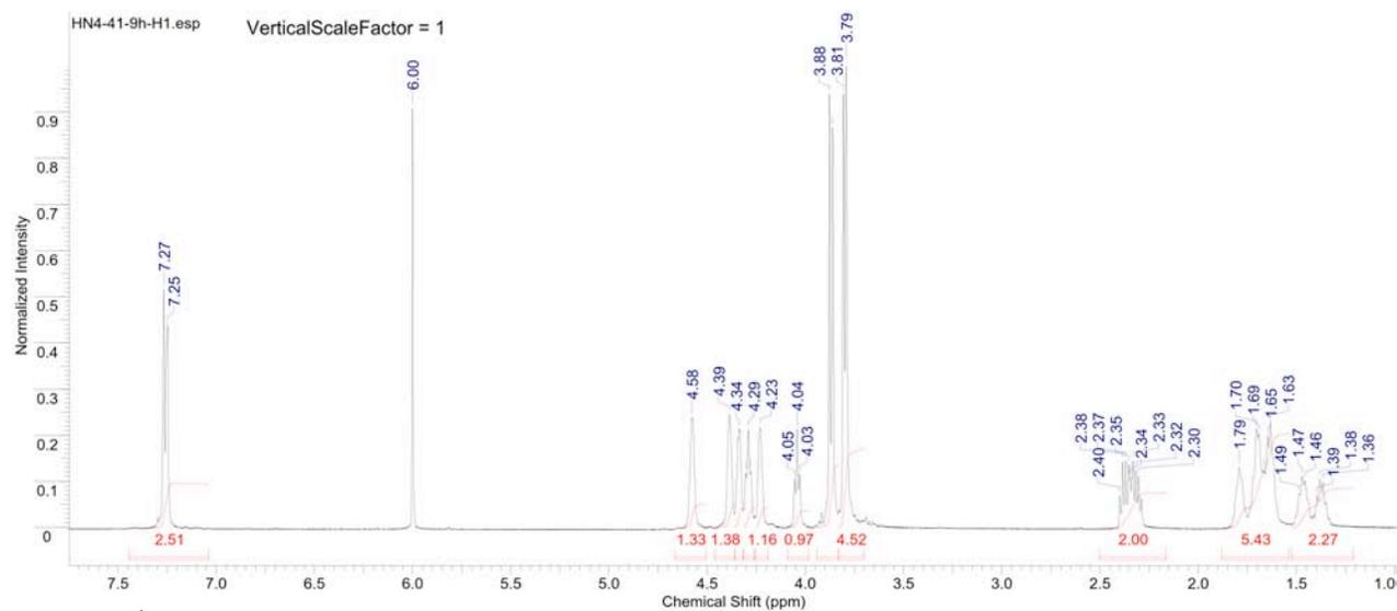
Figure S302. <sup>1</sup>H NMR spectrum of copoly(caprolactone/ hydroxyethylsyngic acid) [50:50] at 9 hours (Table S4, entry 16).
