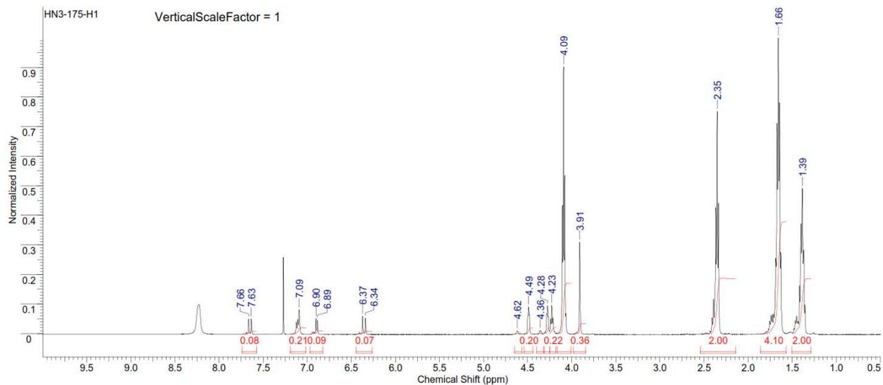
Figure S254. <sup>1</sup>H NMR spectrum of copoly(caprolactone/ hydroxyethylferulic acid) [90:10] (Table S2, entry 22).
