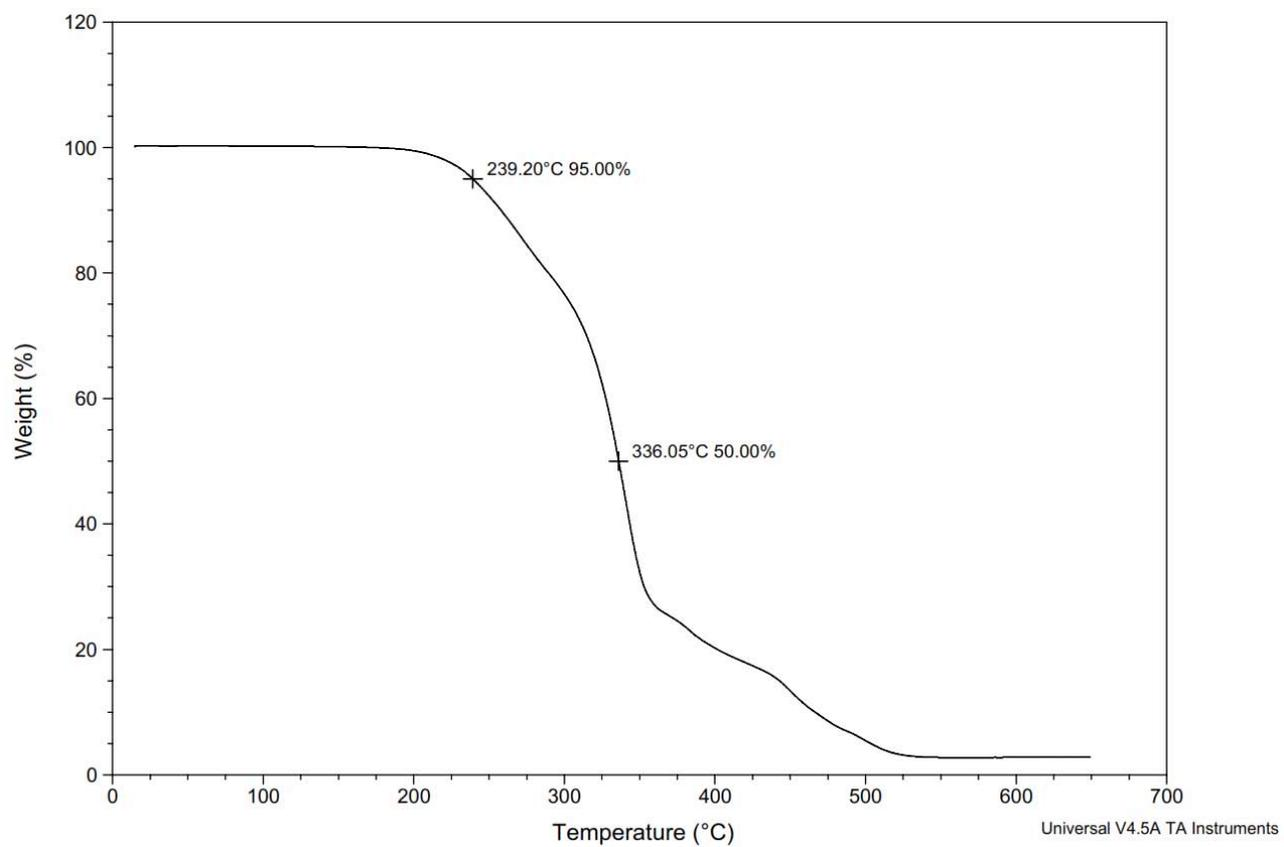
**Figure S195.** TGA Thermogram of copoly(L-lactide/ hydroxyethylsyringic acid) [60:40] (Table S3, entry 3).
