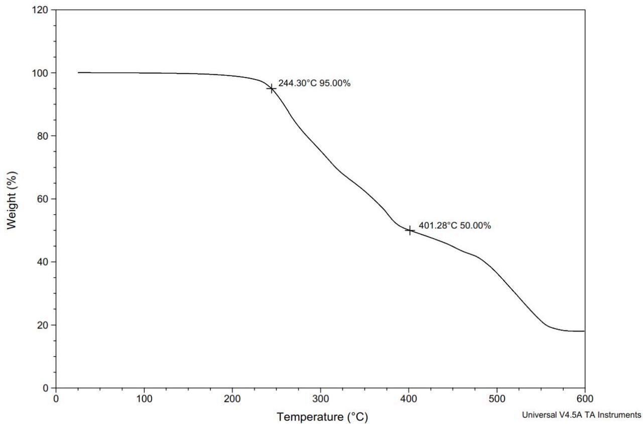
**Figure S204.** TGA Thermogram of copoly(L-lactide/ hydroxyethylferulic acid) [70:30] (Table S3, entry 14).
