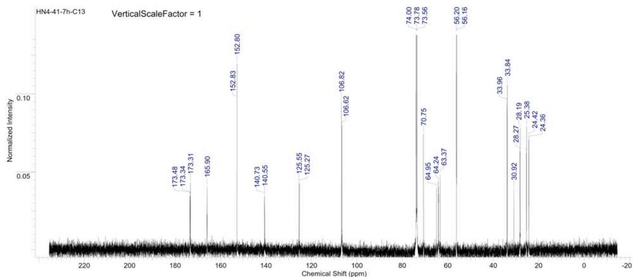
Figure S367.  $^{13}\text{C}$  NMR spectrum of copoly(caprolactone/ hydroxyethylsyringic acid) [50:50] at 7 hours (Table S4, entry 14).
