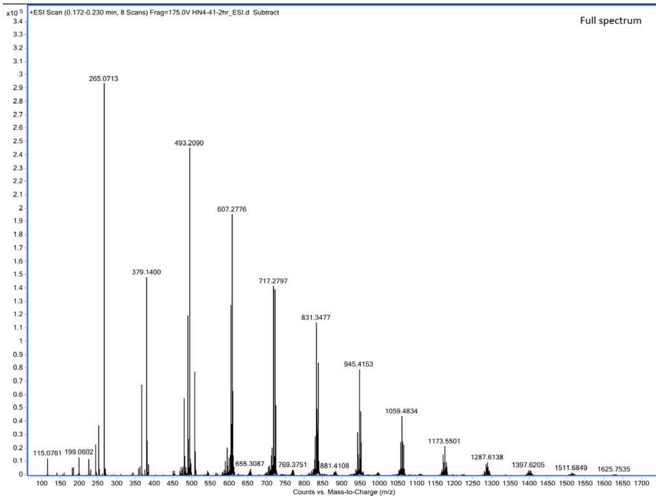
**Figure S385.** ESI spectra of copoly(caprolactone/hydroxyethylsyngic acid) [50:50] at 2 hours (Table S4, entry 6)
