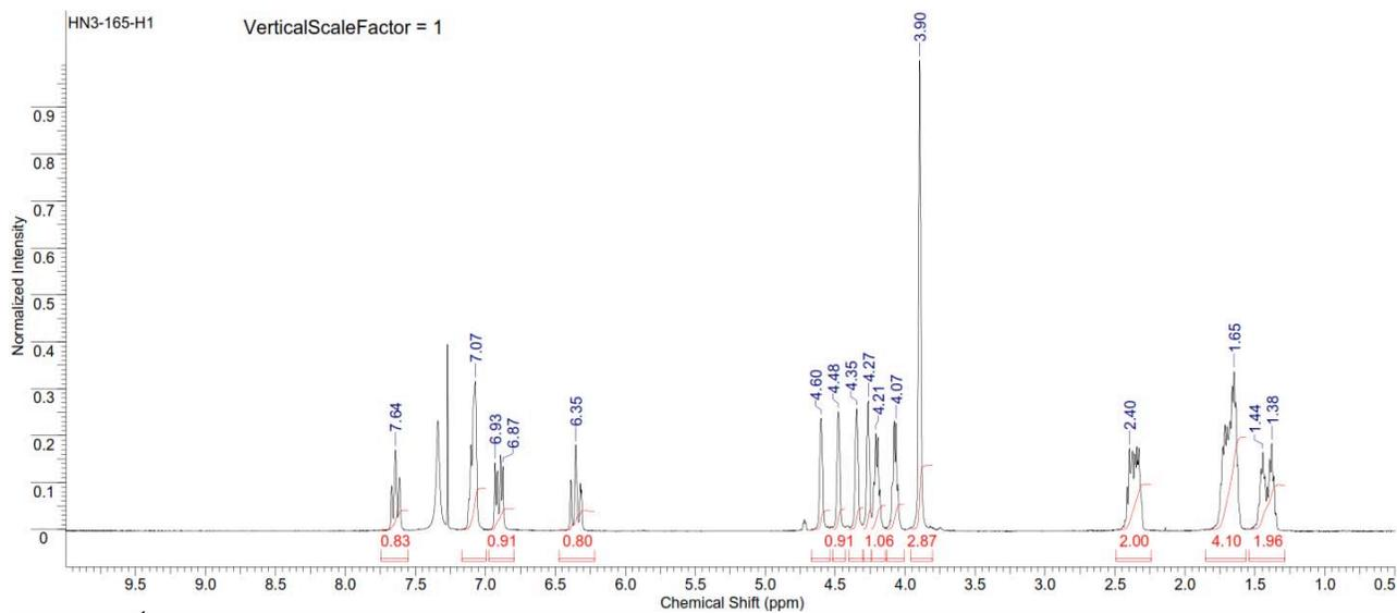
Figure S257. <sup>1</sup>H NMR spectrum of copoly(caprolactone/ hydroxyethylferulic acid) [60:40] (Table S2, entry 25).
