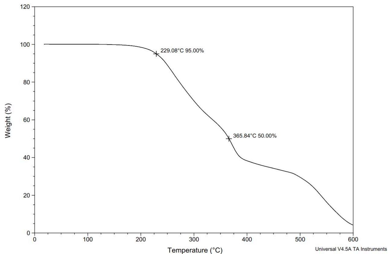
**Figure S203.** TGA Thermogram of copoly(L-lactide/ hydroxyethylferulic acid) [80:20] (Table S3, entry 13).
