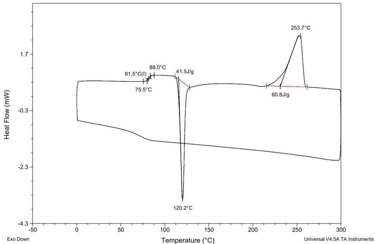
**Figure S106.** DSC Thermogram of polyethylene vanillate (Table S2, entry 21).
