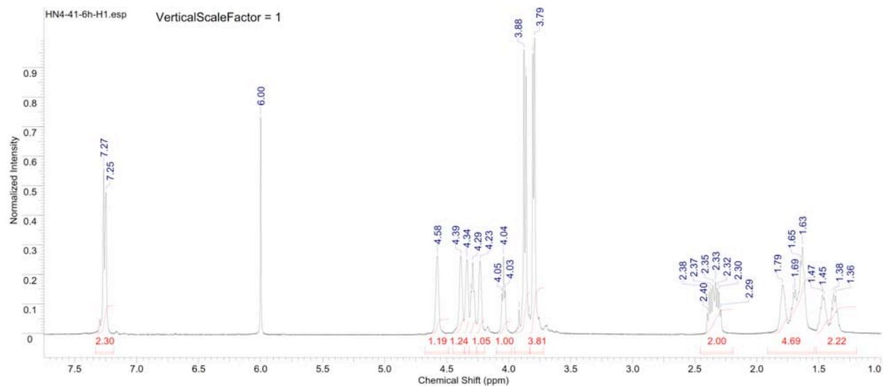
**Figure S299.** <sup>1</sup>H NMR spectrum of copoly(caprolactone/ hydroxyethylsyngic acid) [50:50] at 6 hours (Table S4, entry 13).
