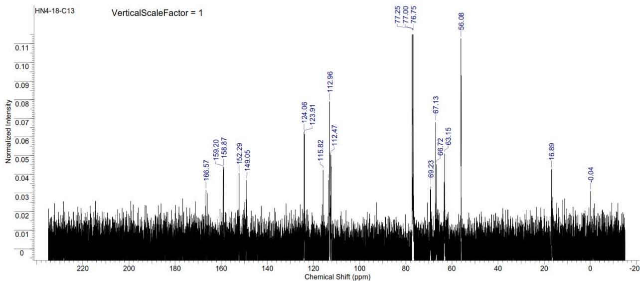
Figure S345. <sup>13</sup>C NMR spectrum of copoly(L-lactide/ hydroxyethylvanillic acid) [40:60] (Table S3, entry 9).
