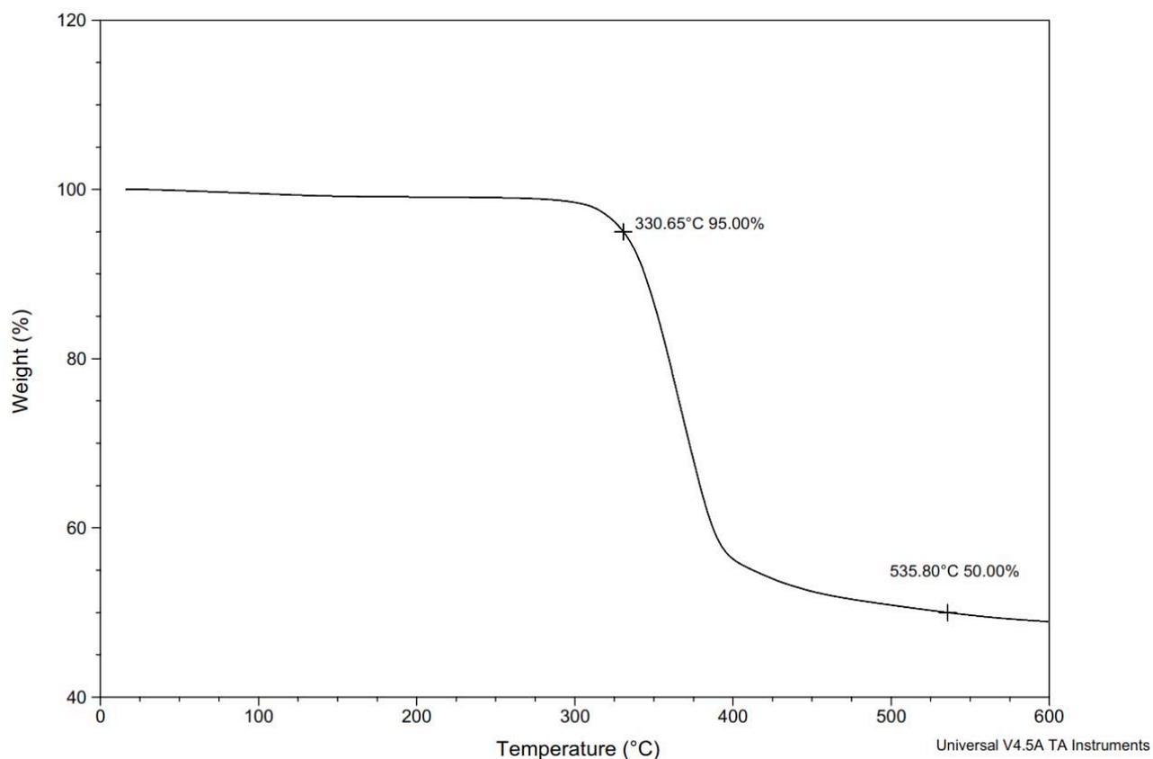
**Figure S188.** TGA Thermogram of polyethylene ferulate (Table S2, entry 31).
