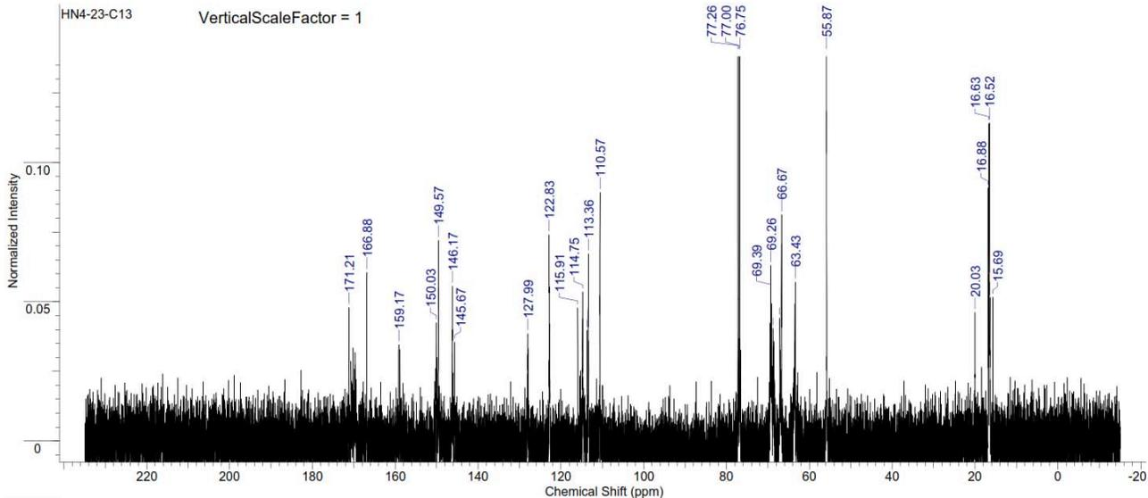
Figure S348. <sup>13</sup>C NMR spectrum of copoly(L-lactide/ hydroxyethylferulic acid) [70:30] (Table S3, entry 14).
