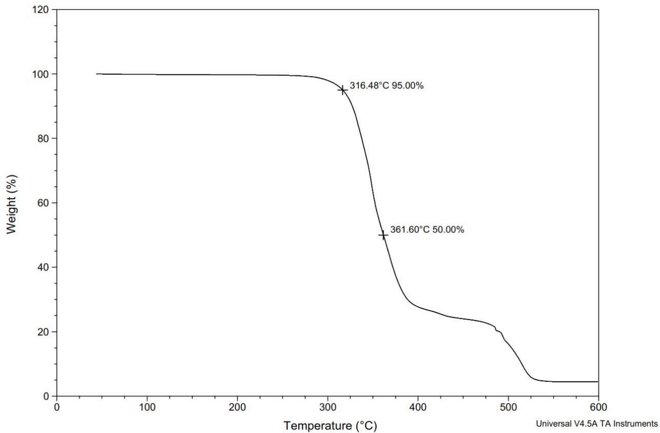
Figure S180. TGA Thermogram of copoly(caprolactone/ hydroxyethylferulic acid) [80:20] (Table S2, entry 23).
