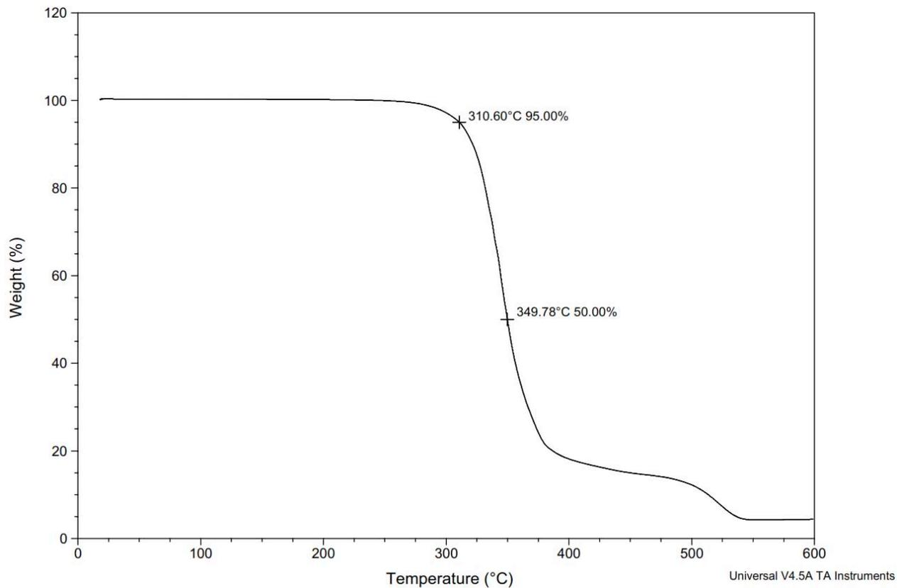
**Figure S179.** TGA Thermogram of copoly(caprolactone/ hydroxyethylferulic acid) [90:10] (Table S2, entry 22).
