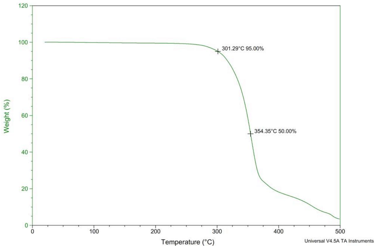
**Figure S225.** TGA Thermogram of copoly(caprolactone/ hydroxyethylsyngic acid) [50:50] at 7 hours (Table S4, entry 14).
