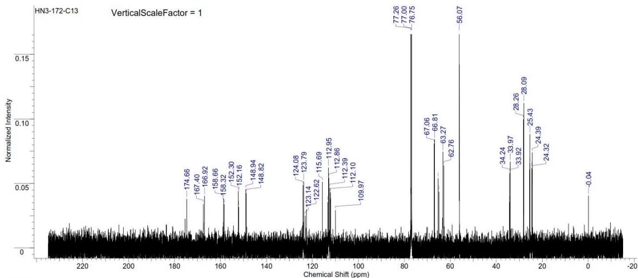
Figure S325.  $^{13}\text{C}$  NMR spectrum of copoly(caprolactone/ hydroxyethylvanillic acid) [40:60] (Table S2, entry 17).
