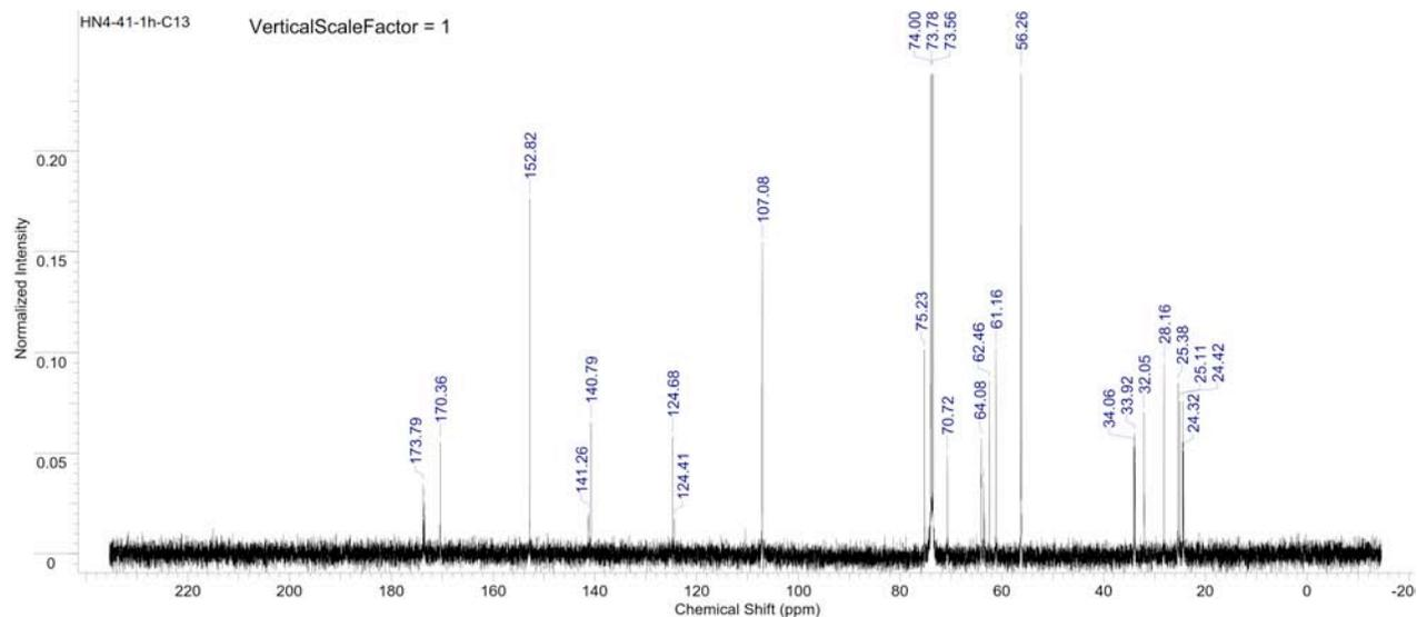
Figure S357.  $^{13}\text{C}$  NMR spectrum of copoly(caprolactone/ hydroxyethylsyringic acid) [50:50] at 1 hour (Table S4, entry 4).
