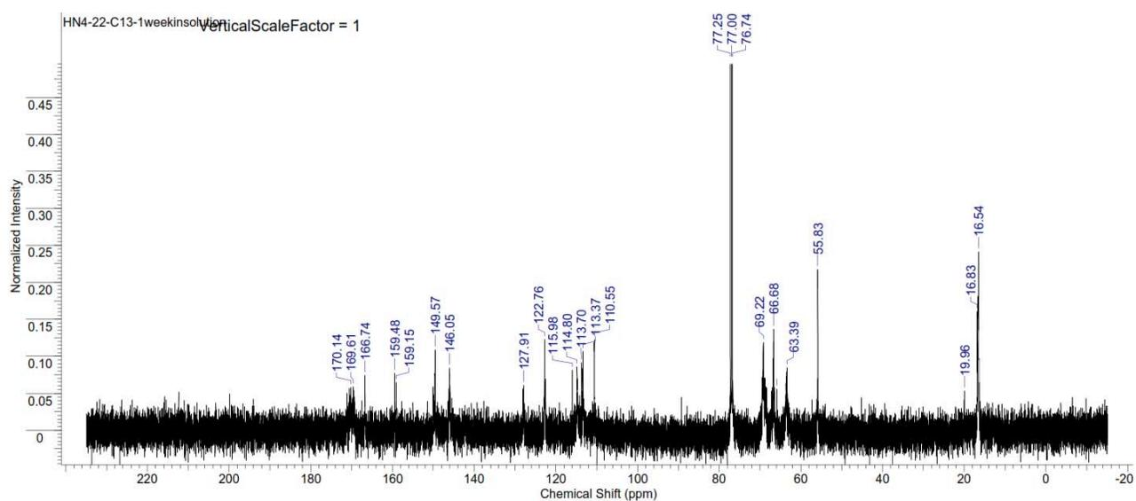
Figure S347. <sup>13</sup>C NMR spectrum of c copoly(L-lactide/ hydroxyethylferulic acid) [80:20] (Table S3, entry 13).
