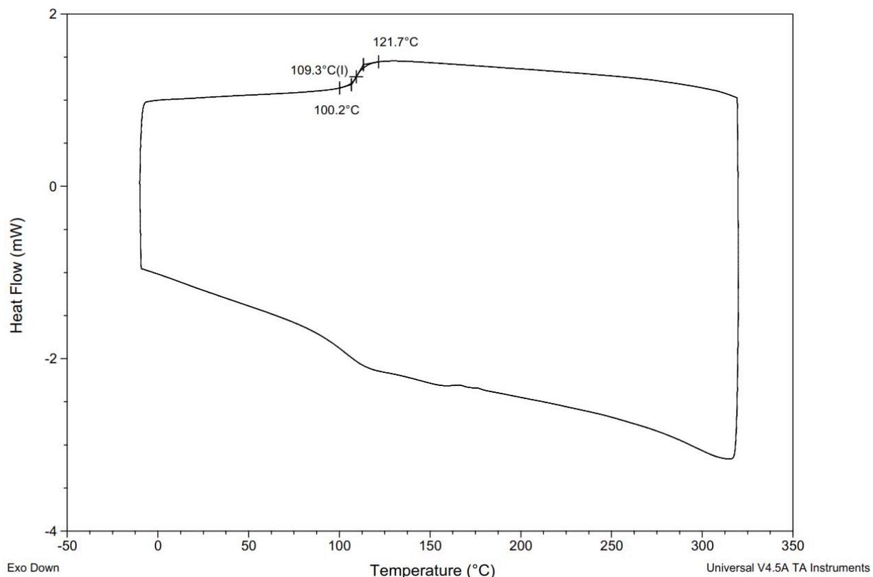
**Figure S120.** DSC Thermogram of polyethylene coumarate (Table S2, entry 35).
