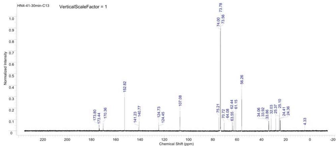
Figure S356.  $^{13}\text{C}$  NMR spectrum of copoly(caprolactone/ hydroxyethylsyringic acid) [50:50] at 30 min. (Table S4, entry 3).
