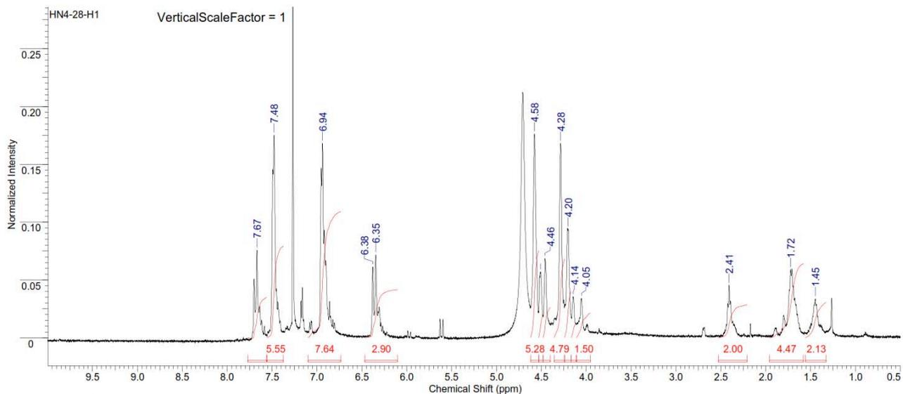
**Figure S266.**  $^1\text{H}$  NMR spectrum of copoly(caprolactone/ hydroxyethylcoumaric acid) [20:80] (Table S2, entry 34).
