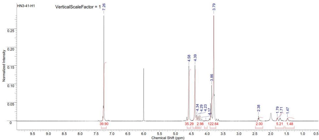
Figure S243. <sup>1</sup>H NMR spectrum of copoly(caprolactone/ hydroxyethylsyringic acid) [10:90] (Table S2, entry 10).
