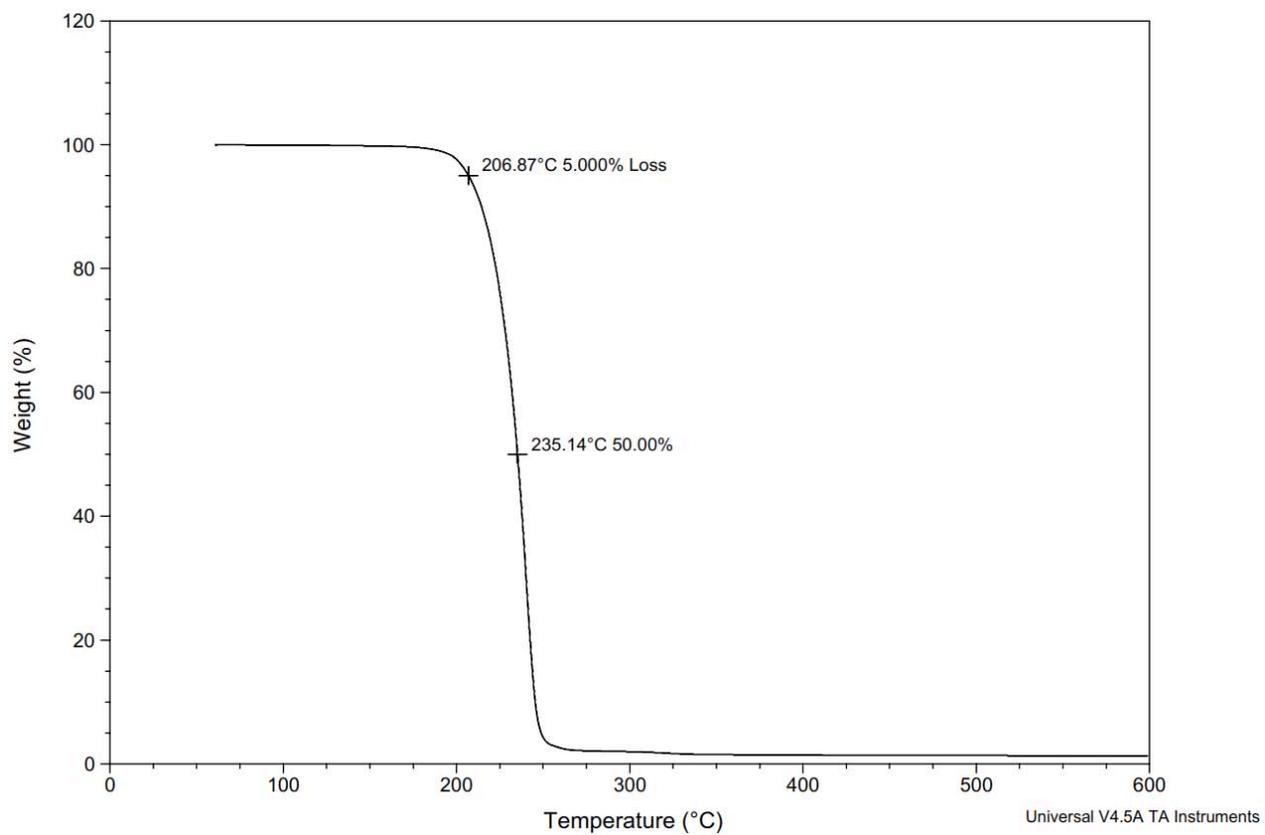
Figure S193. TGA Thermogram of polylactic acid (Table S3, entry 1).
