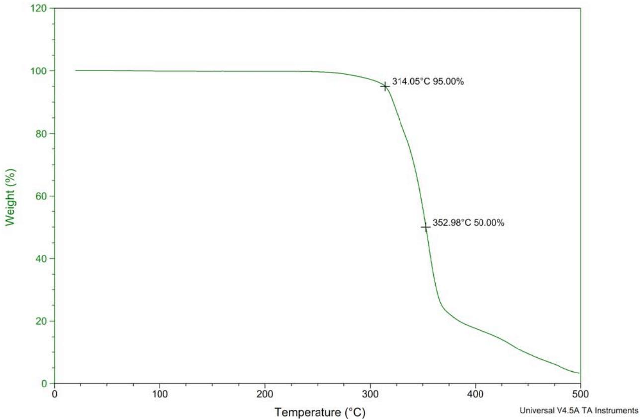
**Figure S228.** TGA Thermogram of copoly(caprolactone/ hydroxyethylsyngic acid) [50:50] at 10 hours (Table S4, entry 17).
