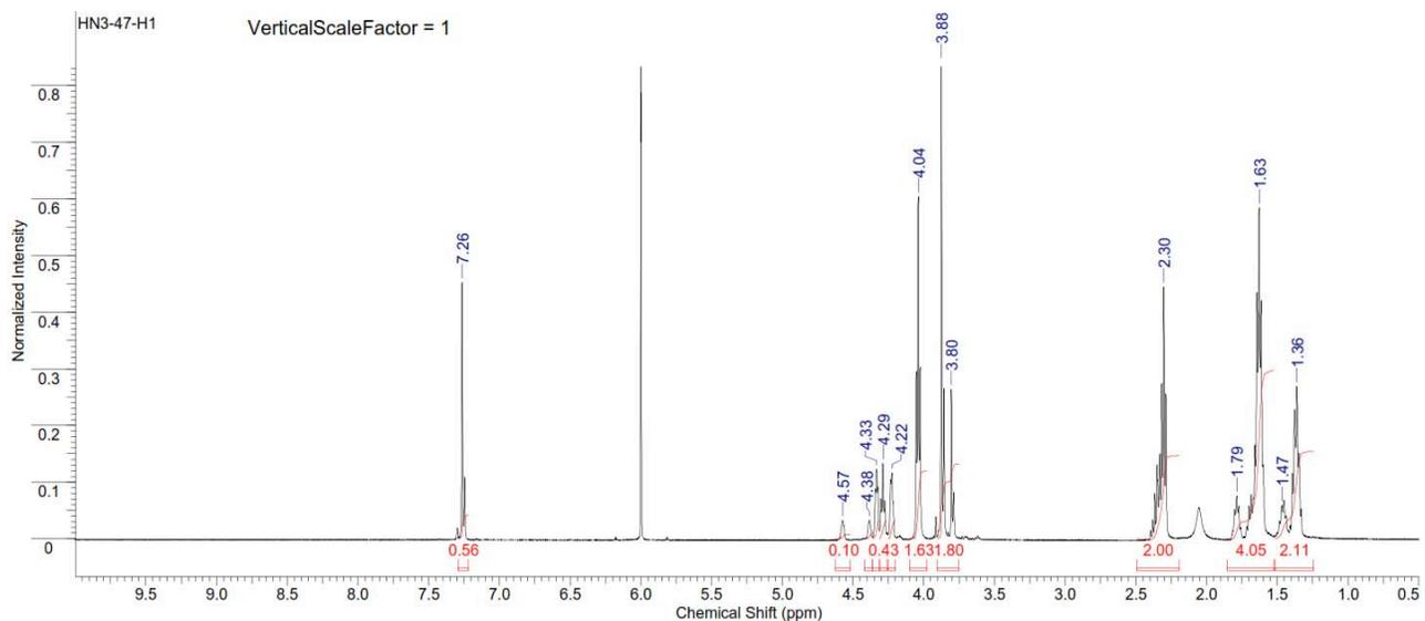
Figure S236. <sup>1</sup>H NMR spectrum of copoly(caprolactone/ hydroxyethylsyngic acid) [80:20] (Table S2, entry 3).
