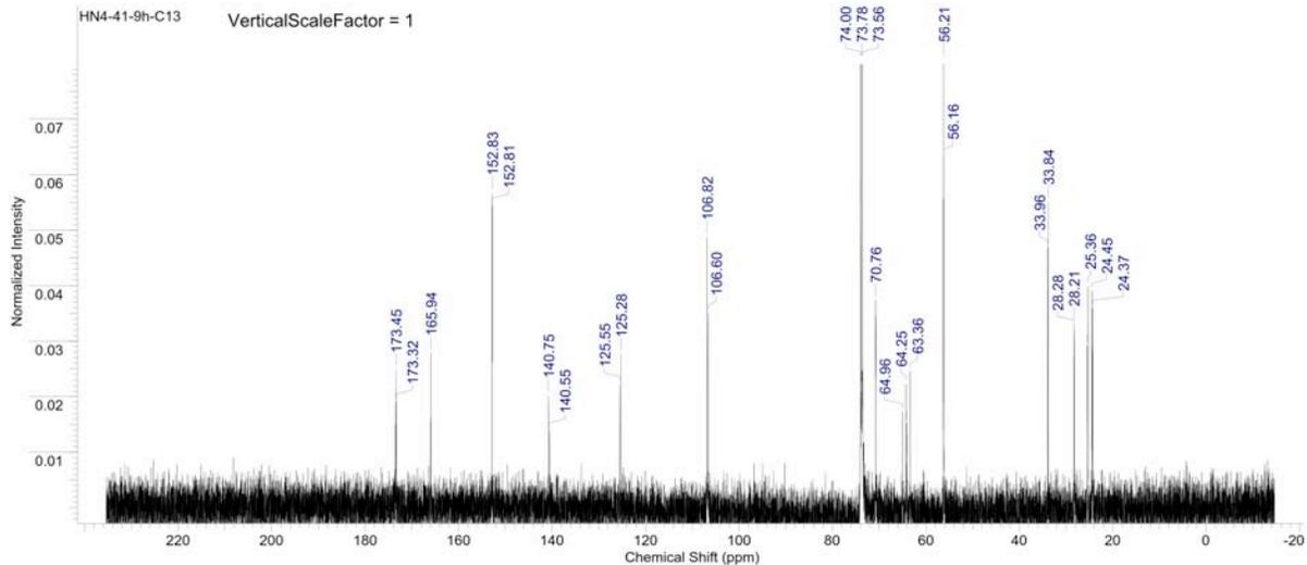
**Figure S369.**  $^{13}\text{C}$  NMR spectrum of copoly(caprolactone/ hydroxyethylsyringic acid) [50:50] at 9 hours (Table S4, entry 16).
