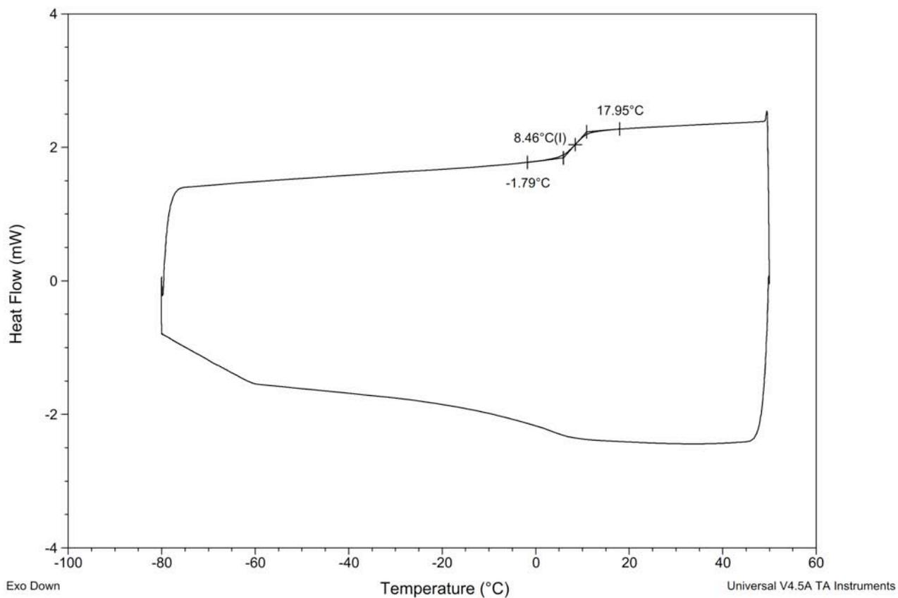
**Figure S150.** DSC Thermogram of copoly(caprolactone/ hydroxyethylsyngic acid) [50:50] at 4.5 hours (Table S4, entry 11).
