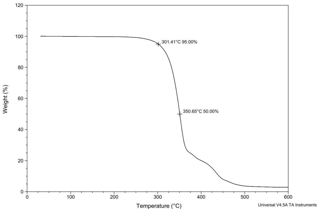
Figure S197. TGA Thermogram of copoly(L-lactide/ hydroxyethylsyngic acid) [20:80] (Table S3, entry 5).
