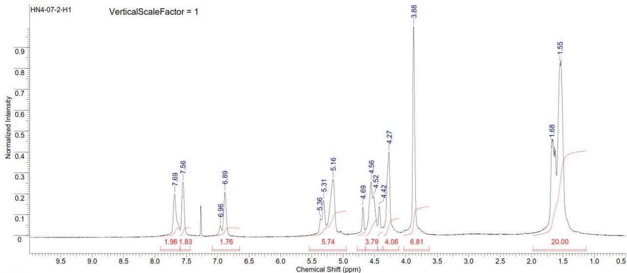
**Figure S273.**  $^1\text{H}$  NMR spectrum of copoly(L-lactide/ hydroxyethylvanillic acid) [80:20] (Table S3, entry 7).
