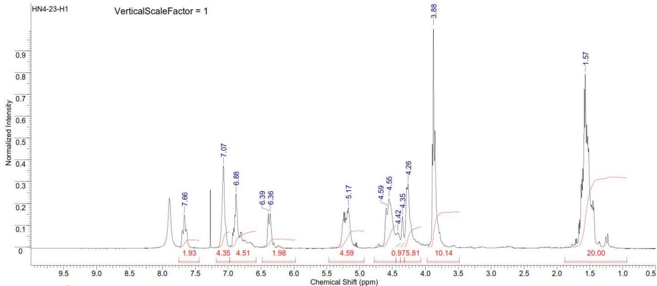
Figure S279. <sup>1</sup>H NMR spectrum of copoly(L-lactide/ hydroxyethylferulic acid) [70:30] (Table S3, entry 14).
