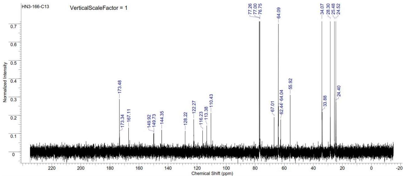
Figure S328. <sup>13</sup>C NMR spectrum of copoly(caprolactone/ hydroxyethylferulic acid) [80:20] (Table S2, entry 23).
