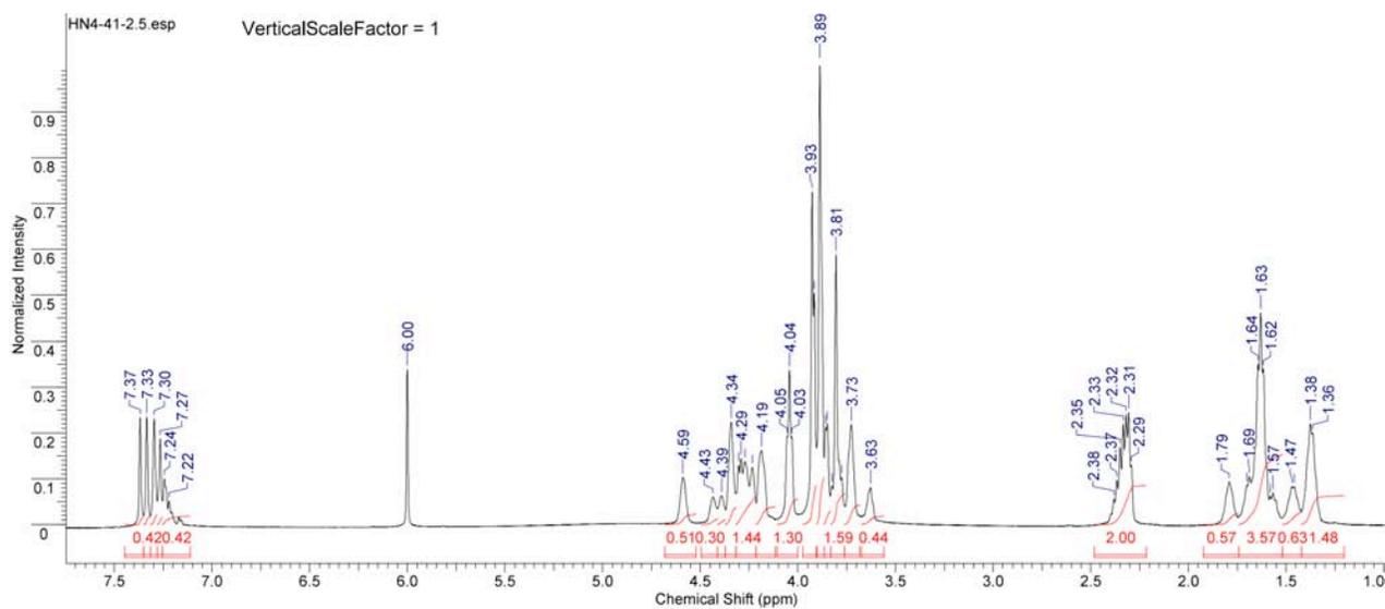
Figure S293. <sup>1</sup>H NMR spectrum of copoly(caprolactone/ hydroxyethylsyngic acid) [50:50] at 2.5 hours (Table S4, entry 7).
