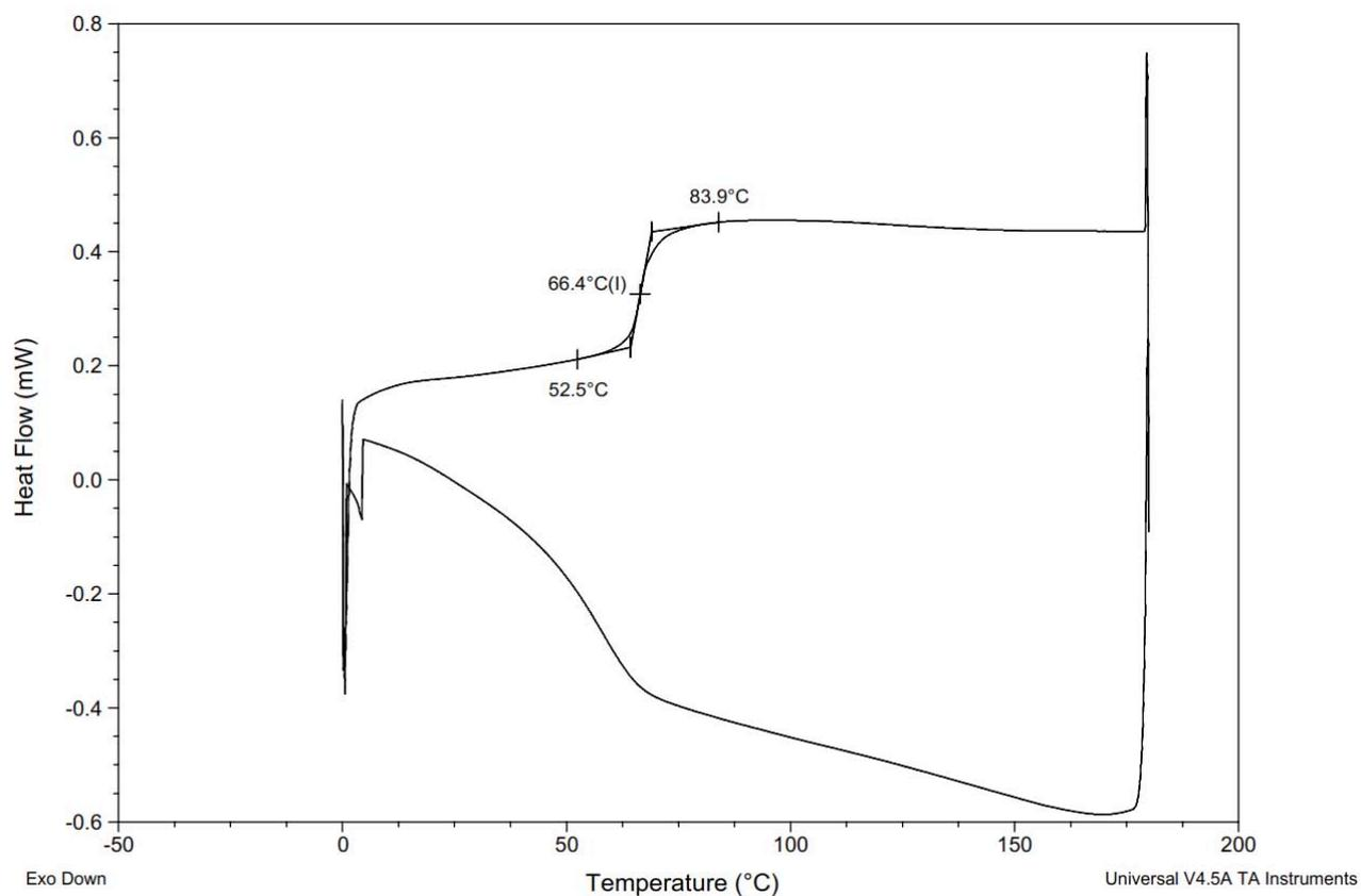
**Figure S126.** DSC Thermogram of copoly(L-lactide/ hydroxyethylvanillic acid) [80:20] (Table S3, entry 7).
