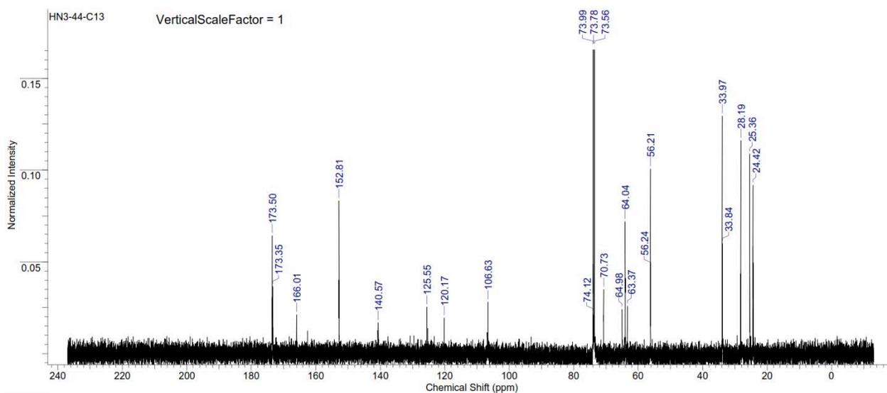
Figure S312. <sup>13</sup>C NMR spectrum of copoly(caprolactone/ hydroxyethylsyringic acid) [70:30] (Table S2, entry 4).
