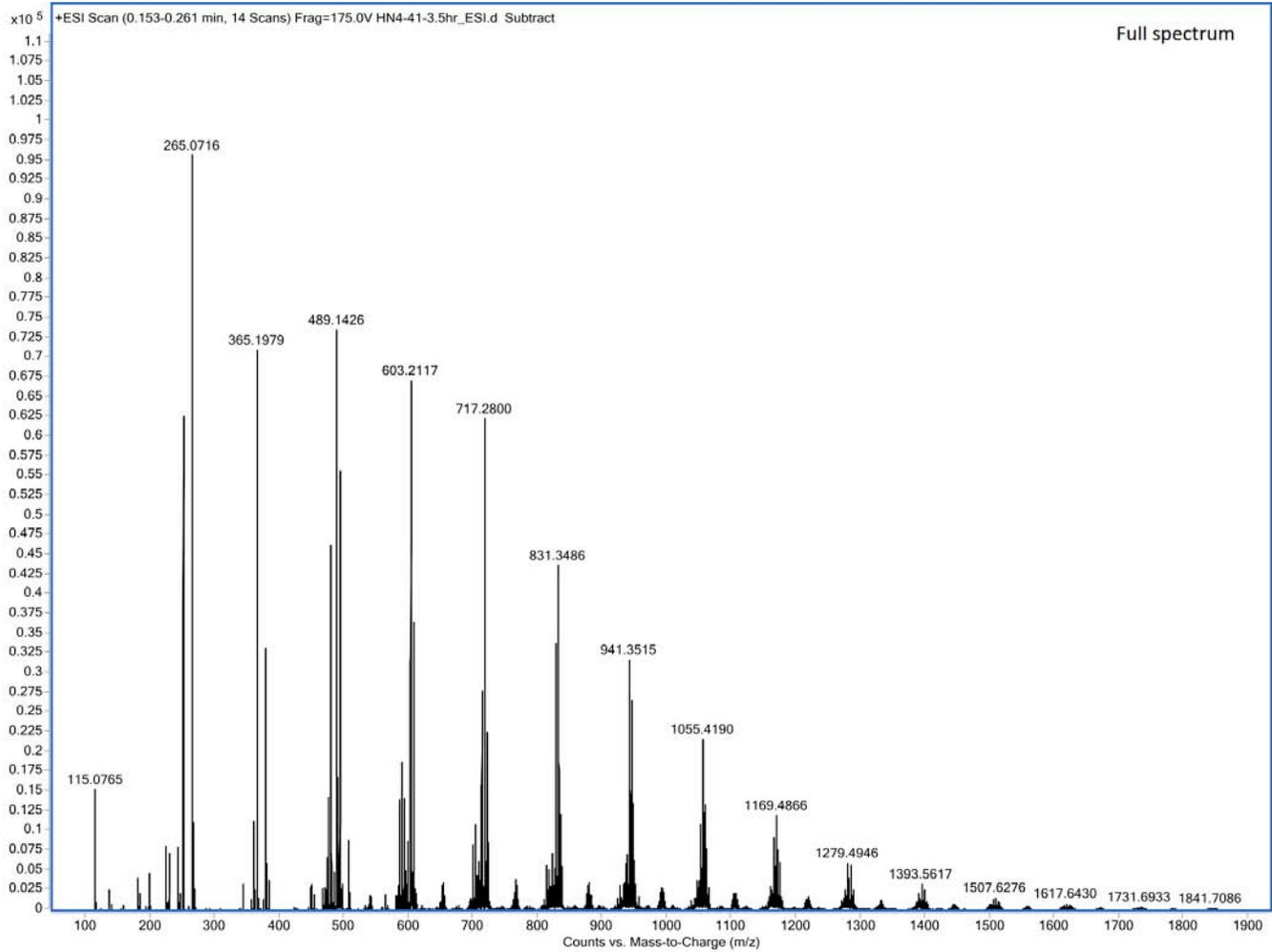
Figure S388. ESI spectra of copoly(caprolactone/hydroxyethylsyngic acid) [50:50] at 3.5 hours (Table S4, entry 9)
