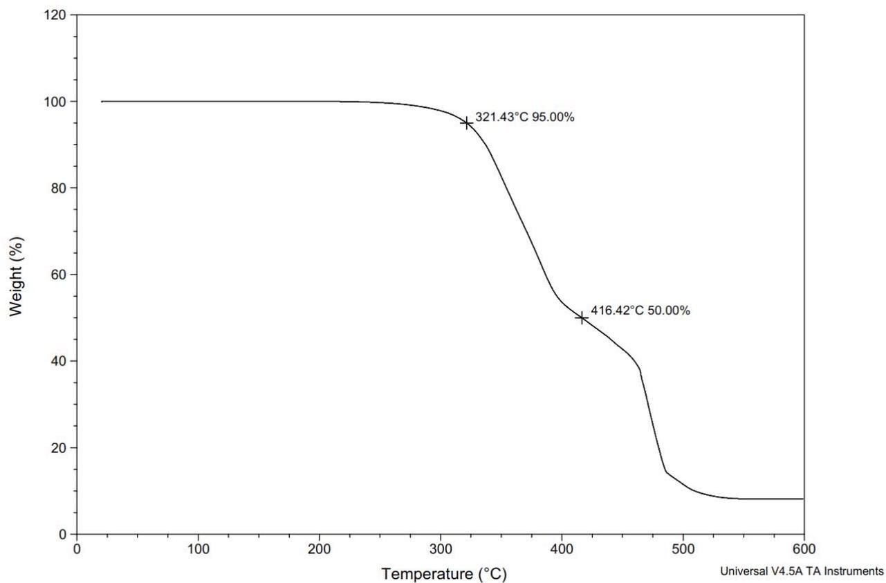
**Figure S186.** TGA Thermogram of copoly(caprolactone/ hydroxyethylferulic acid) [20:80] (Table S2, entry 29).
