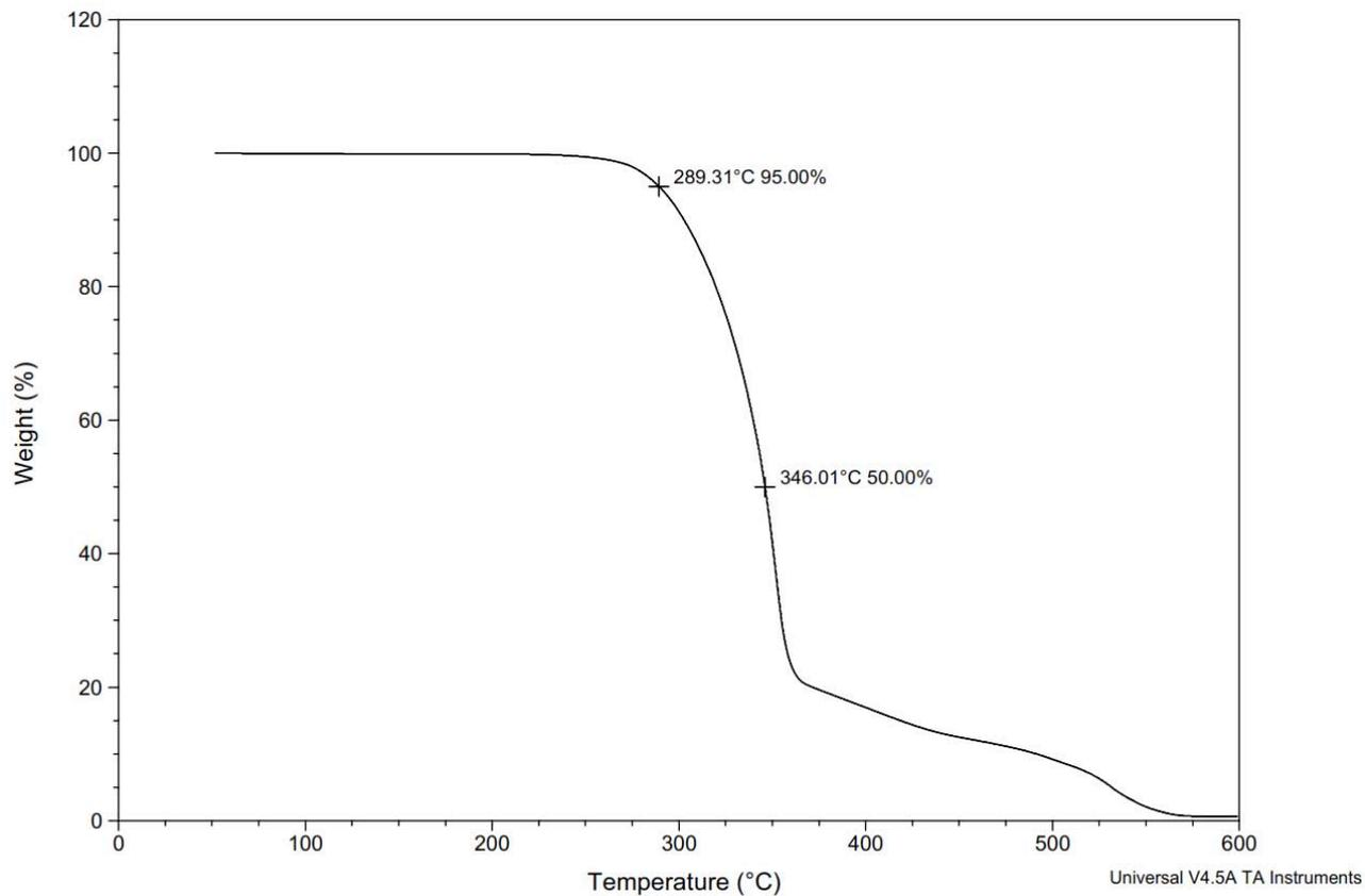
**Figure S160.** TGA Thermogram of copoly(caprolactone/ hydroxyethylsyngic acid) [80:20] (Table S2, entry 3).
