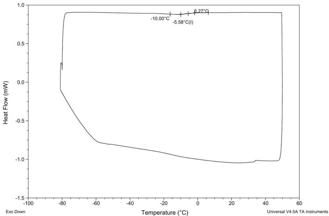
**Figure S147.** DSC Thermogram of copoly(caprolactone/ hydroxyethylsyngic acid) [50:50] at 3 hours (Table S4, entry 8).
