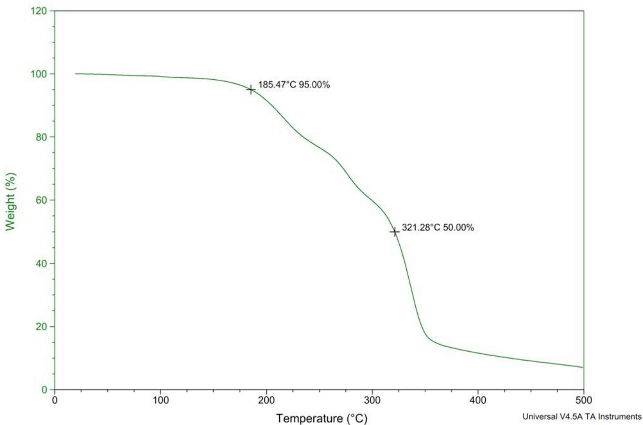
Figure S213. TGA Thermogram of copoly(caprolactone/ hydroxyethylsyngic acid) [50:50] at 20 min. (Table S4, entry 2).
