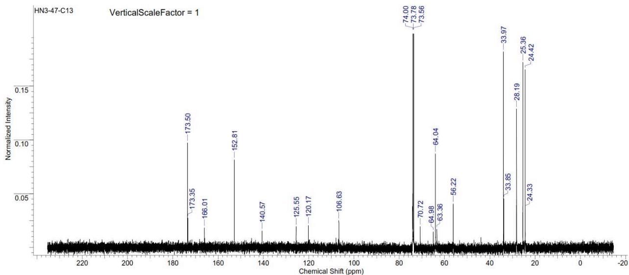
Figure S311. <sup>13</sup>C NMR spectrum of copoly(caprolactone/ hydroxyethylsyringic acid) [80:20] (Table S2, entry 3).
