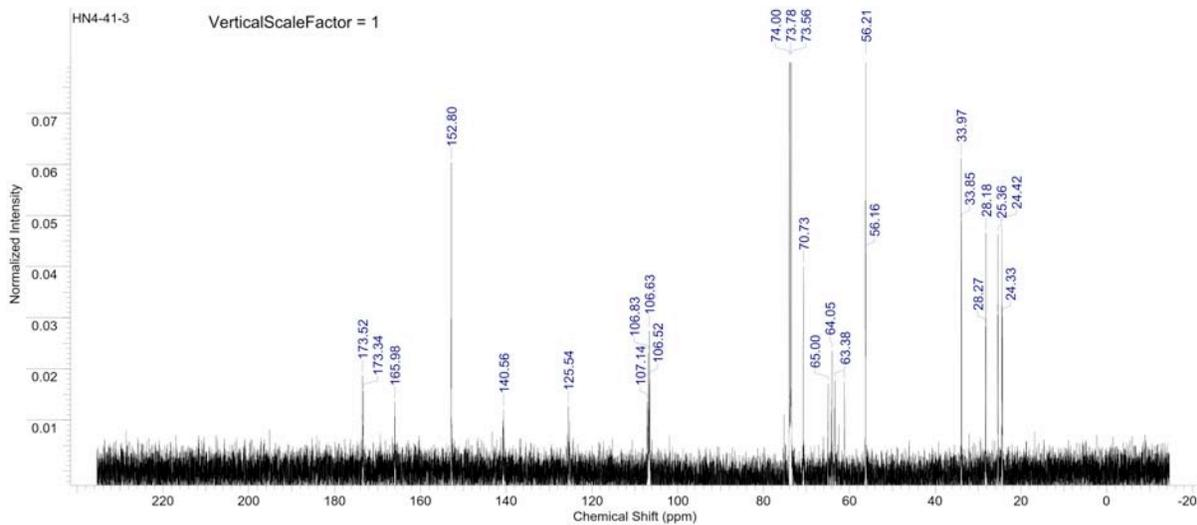
**Figure S362.**  $^{13}\text{C}$  NMR spectrum of copoly(caprolactone/ hydroxyethylsyringic acid) [50:50] at 3.5 hours (Table S4, entry 9).
