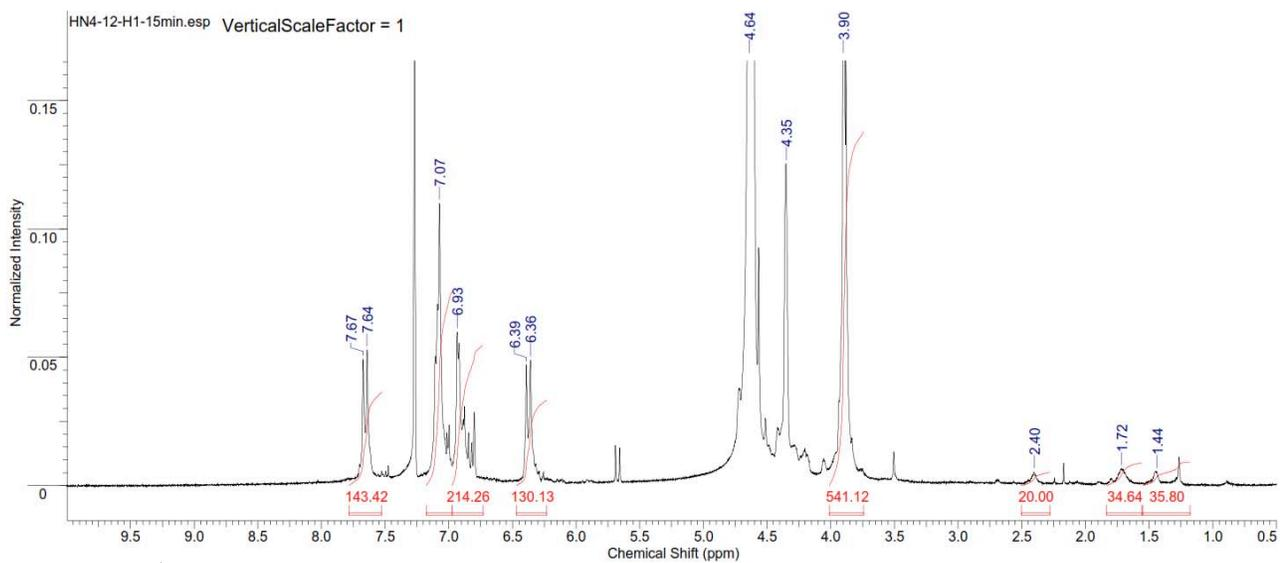
Figure S262. <sup>1</sup>H NMR spectrum of copoly(caprolactone/ hydroxyethylferulic acid) [10:90] (Table S2, entry 30).
