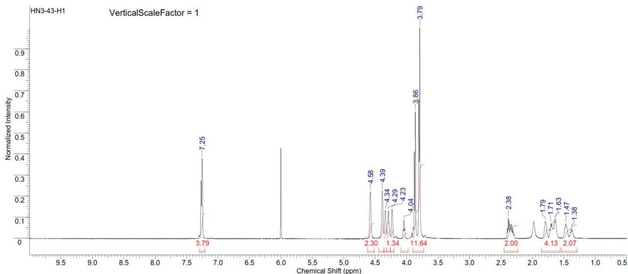
Figure S240. <sup>1</sup>H NMR spectrum of copoly(caprolactone/ hydroxyethylsyngic acid) [40:30] (Table S2, entry 7).
