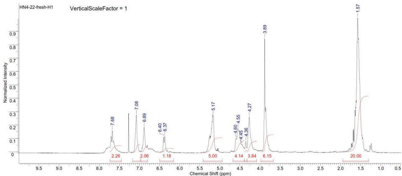
**Figure S278.**  $^1\text{H}$  NMR spectrum of copoly(L-lactide/ hydroxyethylferulic acid) [80:20] (Table S3, entry 13).
