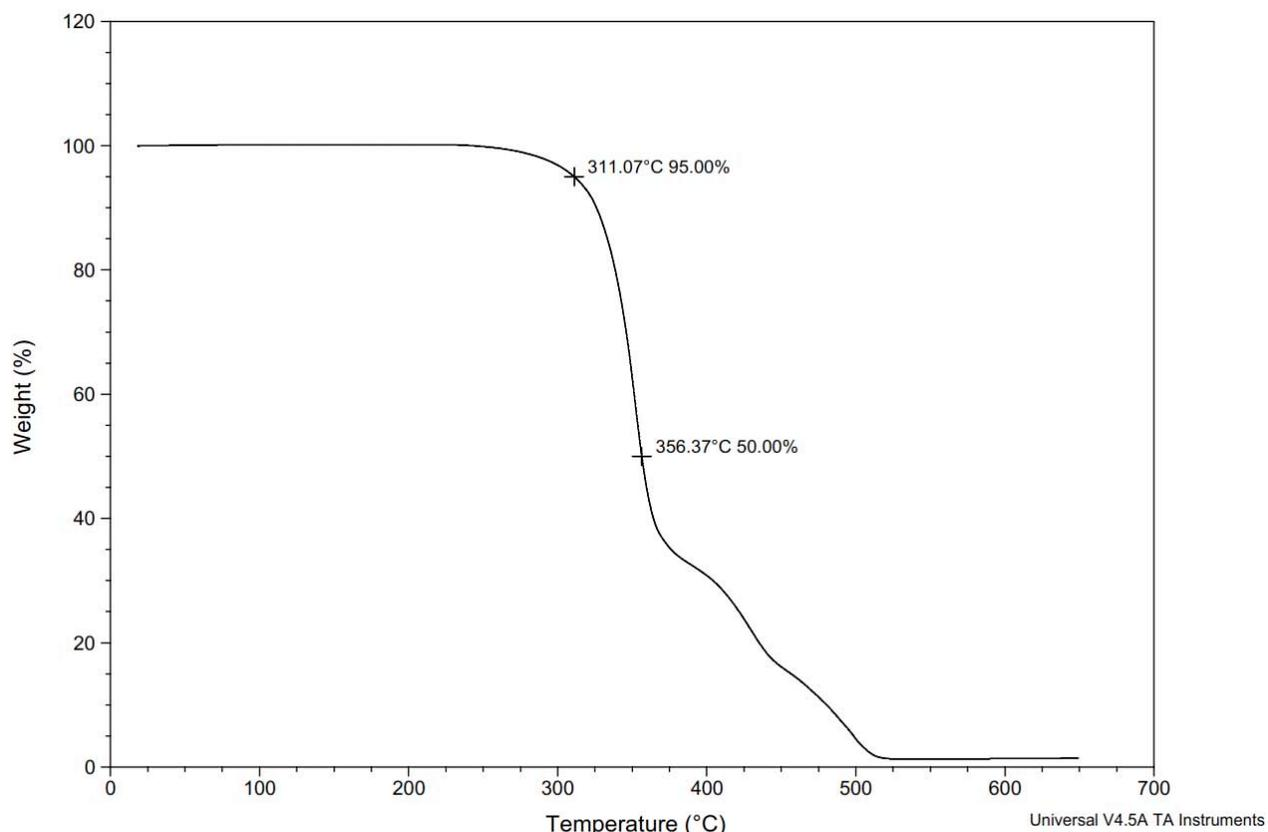
**Figure S178.** TGA Thermogram of polyethylene vanillate (Table S2, entry 21).
