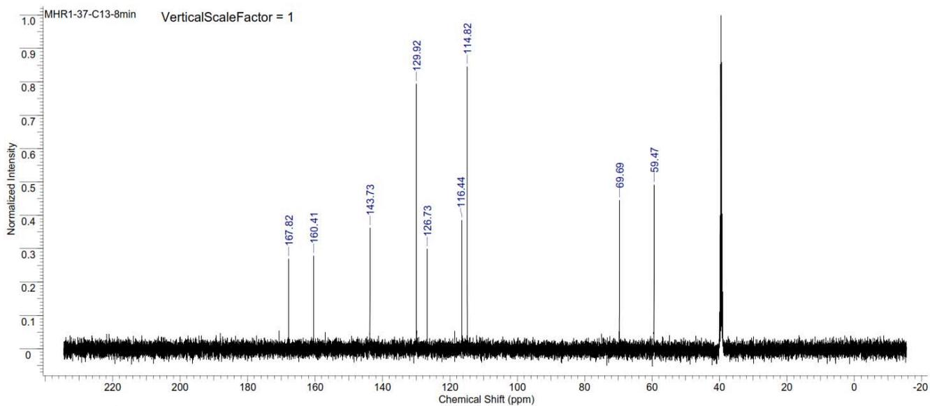
Figure S306. <sup>13</sup>C NMR spectrum of hydroxyethylcoumaric acid.
