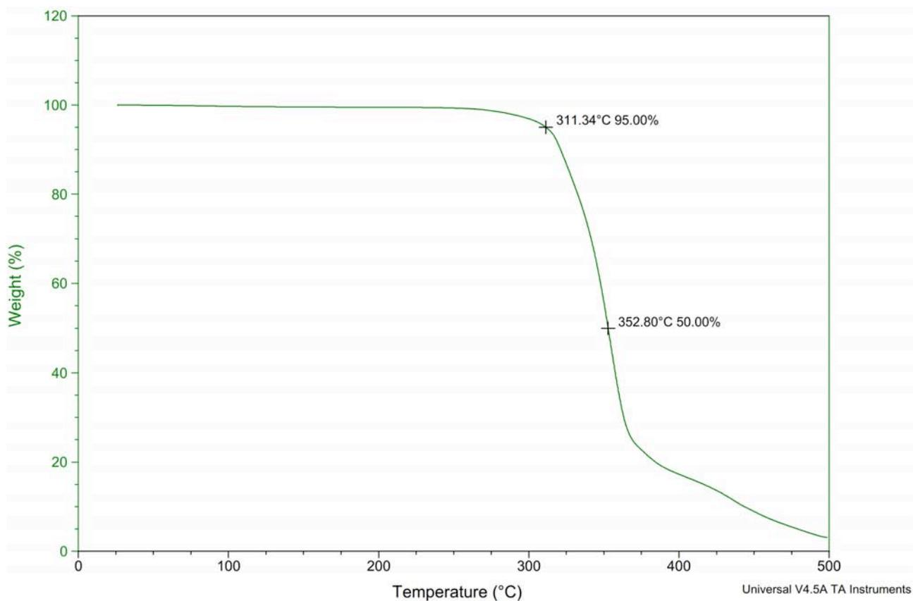
**Figure S227.** TGA Thermogram of copoly(caprolactone/ hydroxyethylsyngic acid) [50:50] at 9 hours (Table S4, entry 16).
