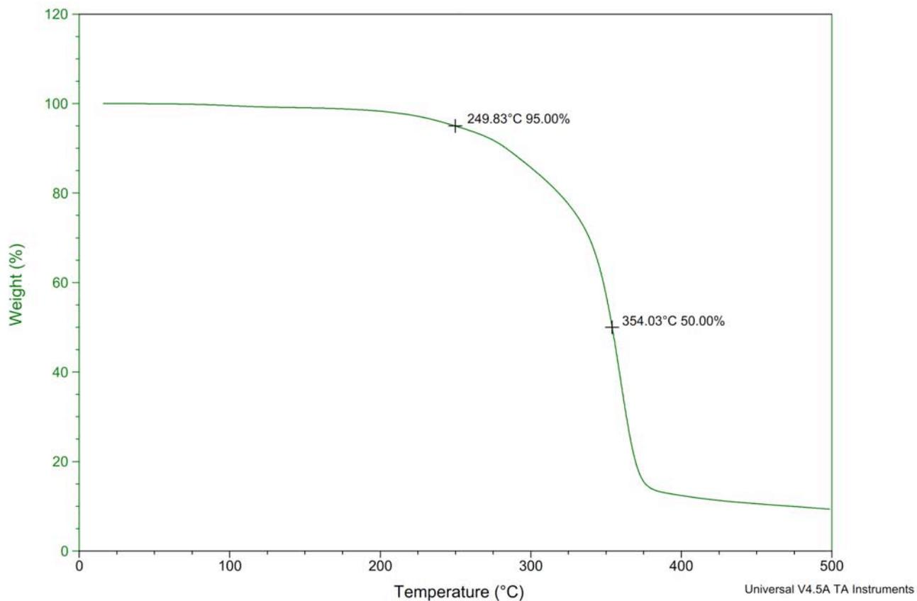
**Figure S220.** TGA Thermogram of copoly(caprolactone/ hydroxyethylsyngic acid) [50:50] at 3.5 hours (Table S4, entry 9).
