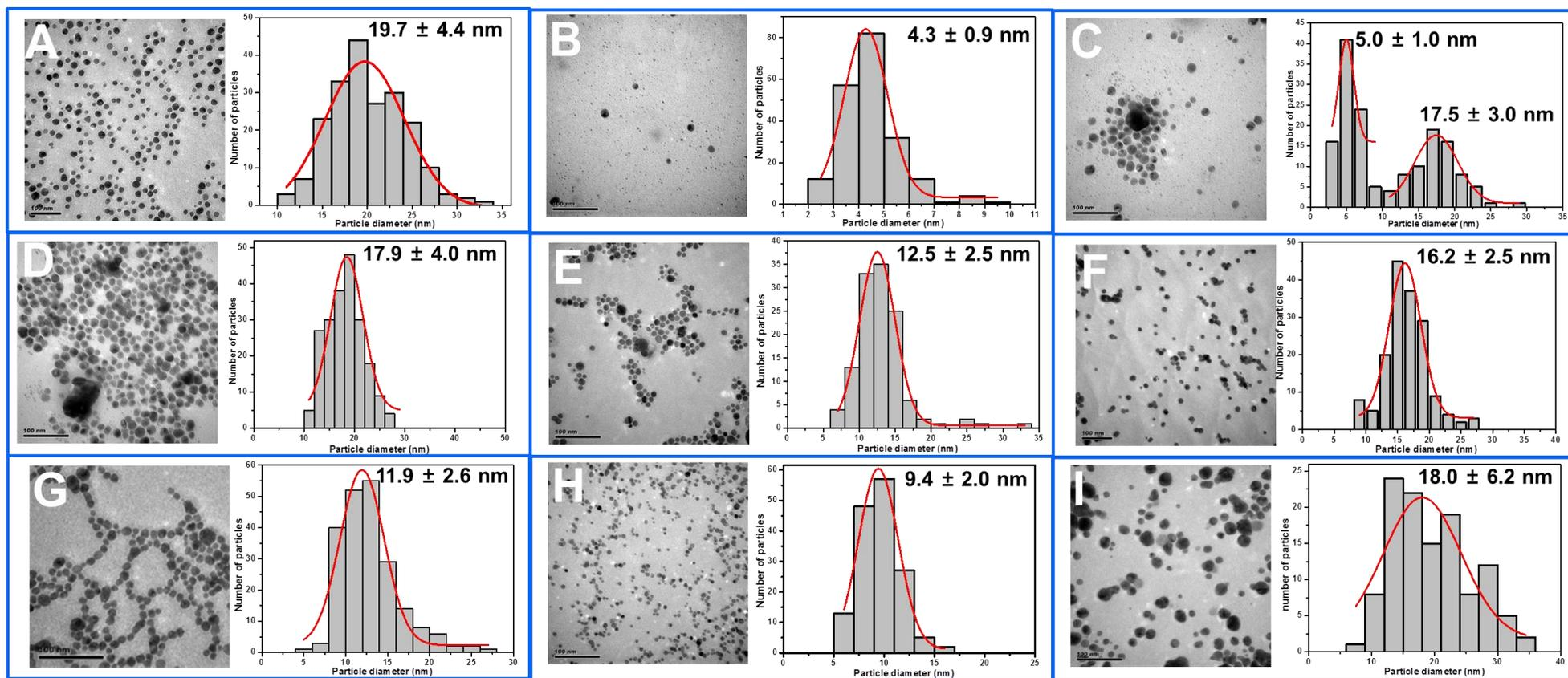
**Fig. S1** TEM characterization and size distribution of aged AgCNPs: commercial AgNPs with unknown coating (A); Ag<sub>2</sub>S NPs (B); Ag&Ag<sub>2</sub>S NPs (C); AgCl NPs (D); Citrate-AgNPs (E); GA-protected AgNPs (F); PVP-3.5-AgNPs (G); PVP-58-AgNPs (H); PVA-protected AgNPs (I).
