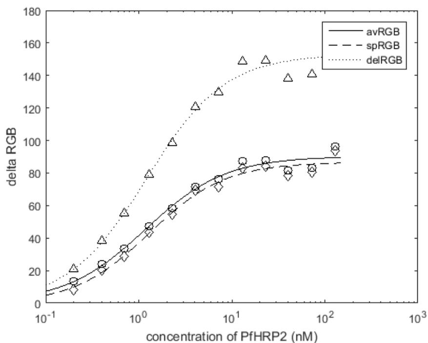
**Supplementary Figure S12:** Using three different methods to report the change in intensity in RGB color space for surfaces tested with ALP-BCIP/NBT, i) average intensity of the blue channel (spRGB), ii) average intensity of all three channels (avRGB), and iii) average intensity according to Murdock et al. (delRGB). The data points show the calculated values and the lines show the sigmoidal fits.
