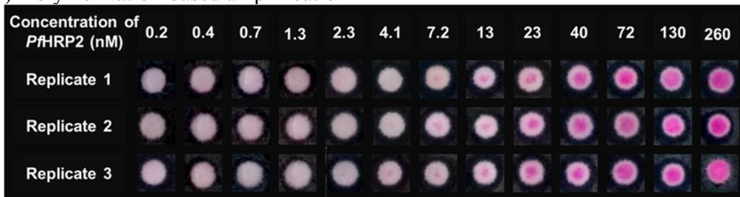
**Supplementary Figure S11:** Replicates of positive controls in the dilution series experiments across the full range of concentrations of *Pf*HRP2 that were tested, 0.2 nM – 260 nM for A) enzymatic amplification with HRP using DAB/H<sub>2</sub>O<sub>2</sub> solution as the substrate, B) enzymatic amplification with ALP using BCIP/NBT solution as substrate, C) using silver deposition, catalyzed by gold nanoparticles, and D) polymerization-based amplification.
