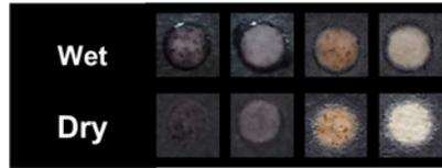
**Supplementary Figure S13:** The effect of surface condition on the appearance of color. Same surfaces were imaged while they were wet and when they became dry. The appearance of color on the surface is different for the two cases and also affects the absolute values of the red, green and blue channel intensities in the captured image.
