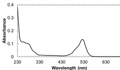
**Supplementary Figure S2:** UV-visible absorption spectrum of EITC conjugated to reporter antibody (7 EITC molecules per IgG molecule). For determining the average number of eosin molecules coupled to each IgG molecule, the following equation was used:
