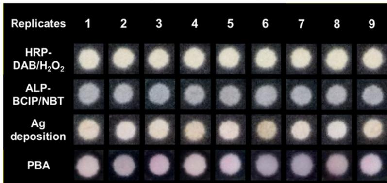
**Supplementary Figure S10:** Replicates of the negative controls in the dilution series experiments for the four different colorimetric methods show in Figure 2. All images were taken with Moto E2.
