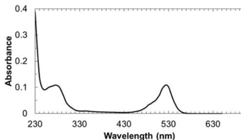
**Supplementary Figure S1:** UV-visible absorption spectrum of EITC conjugated to streptavidin (2.8 EITC molecules per streptavidin molecule). For determining the average number of eosin molecules coupled to each streptavidin molecule, the following equation was used:
