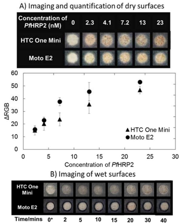
**Supplementary Figure S14:** Effect of device on images. (A) The images of the same dry surfaces obtained using HRP-DAB/H<sub>2</sub>O<sub>2</sub> taken with two different smartphones. On changing the device, the qualitative trend in images remains the same, but the absolute values of the red, green, and blue channels can be very different. (B) The wet negative control surfaces for HRP-DAB/H<sub>2</sub>O<sub>2</sub> taken with two different smartphones appear very different.
