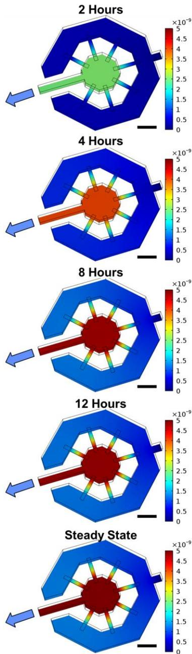
Supplemental Fig. 4. Simulations of the distribution of the concentration (mole/L) of the proteins secreted by cancer cell when 50 Pa was applied to the adherent port of the chamber (the flow condition right after media exchange) using COMSOL 5.1. We assume that one cell secretes 1000 proteins per second, 1 cancer cell is captured in the inner chamber, and the protein diffusion coefficient is  $1^{-10} \text{ m}^2/\text{s}$ .<sup>1-4</sup> (Scale bar: 100  $\mu\text{m}$ )
