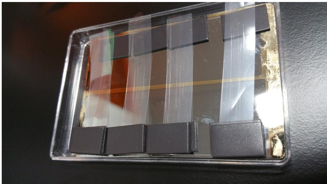
Fig. S4. Storage method for ultra-thin glass microchips.
