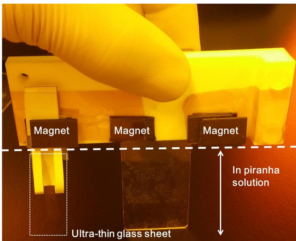
Fig. S2. Experimental jig for chemical cleaning of ultra-thin glass sheet.
