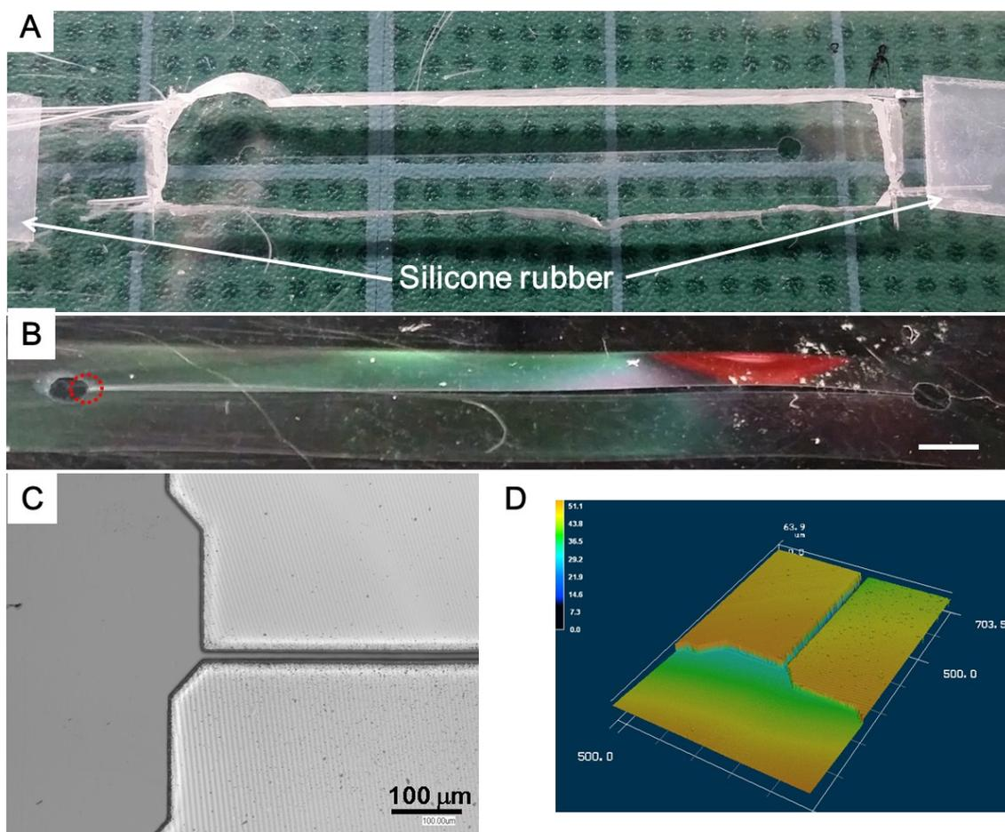
Fig. S1. Images of the fabricated layer 2 of the microchip.
