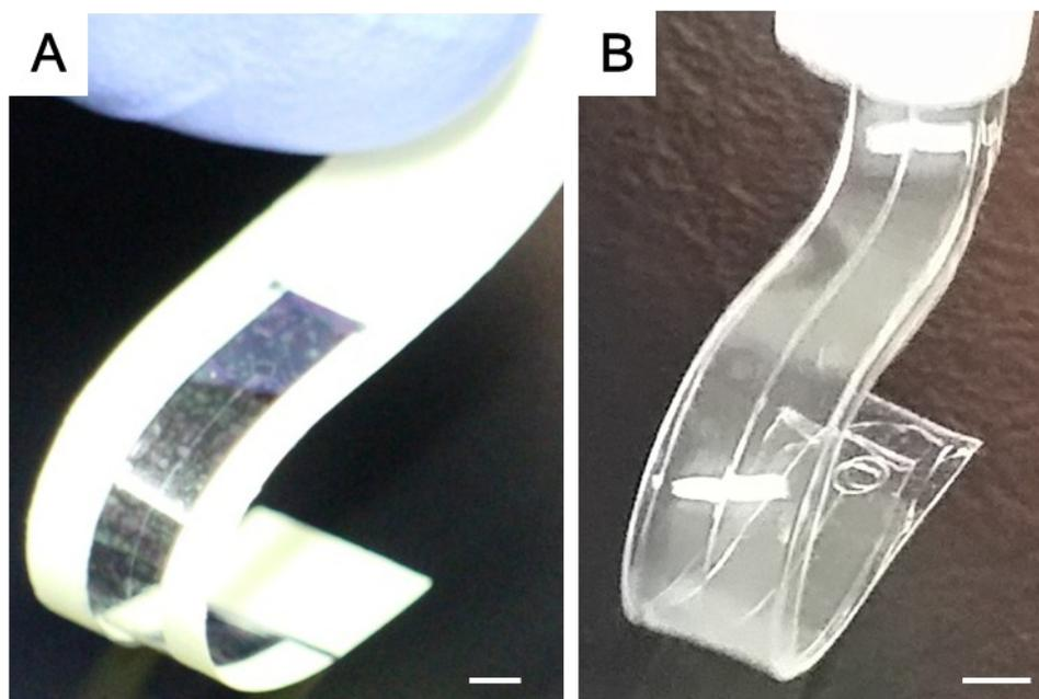
Fig. S6. Specimens for the flexibility experiment to evaluate fragility.
