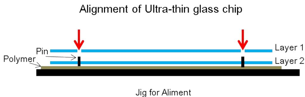
Fig. S3. The alignment jig for bonding of two layers.
