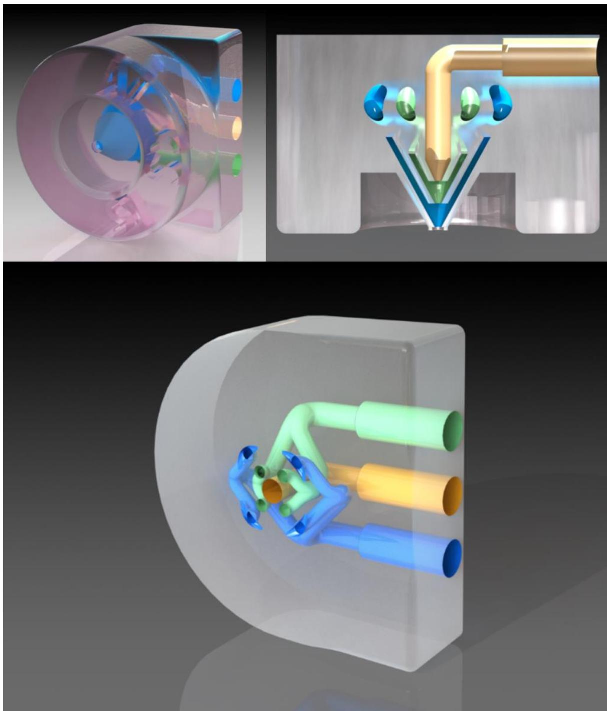
Supplementary Fig. 1: Internal structure of the co-extrusion device. In blue AL in green IS and in orange IS.
