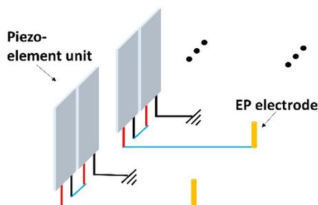
Figure S1: Electrical connections for biasing the EP electrodes using pairs of serially connected piezoelectric elements.
