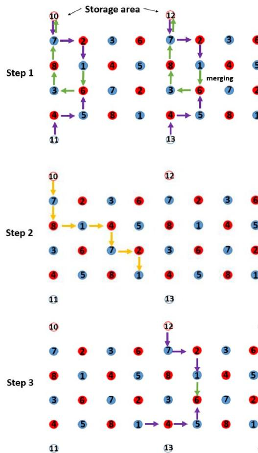
Figure S3: An example integration of storage sites and the base functional electrode matrices to process multiple droplets.
