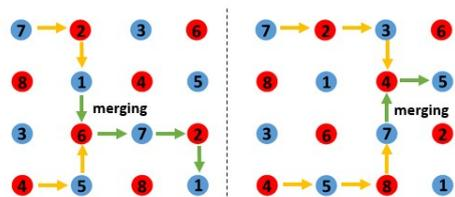
Figure S2: One possible implementation of the merging function using the base 4x4 electrode matrix.
