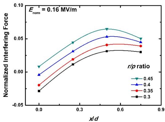
Figure S4: Predicted normalized interfering forces at different positions between two driving electrodes under different values of the ratio between the droplet radius and the electrode pitch,  $r/p$ .
