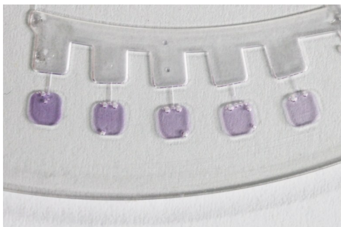
Fig. S2. Negative control experiments using a real sample spiked with non-pathogenic Escherichia coli K-12. No colour change was shown in the reaction chambers. This result proves the ability of this assay to distinguish bacteria sub-types within E. coli species.
