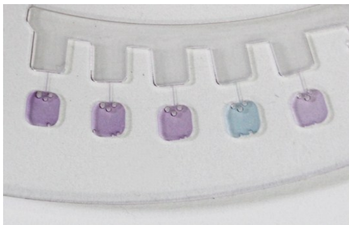
Fig. S1. Singleplex Listeria monocytogenes detection on the lab-on-a-disc. A real sample containing 10^4 cells of L. monocytogenes was used. Colour change was only observed in the reaction chamber #4, where the LAMP primer set targeting L. monocytogenes had been pre-stored, which confirmed specific detection of that bacteria species.
