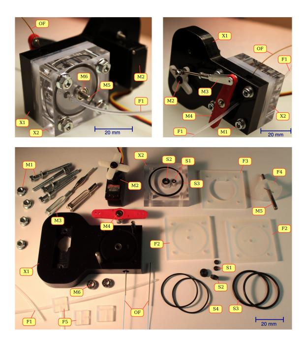
Mechanical parts and drive transmission: M1–mounting screws, M2–servo motor, M3–pusher rods, M4–rotary arm, M5–shaft, M6–ball bearing
