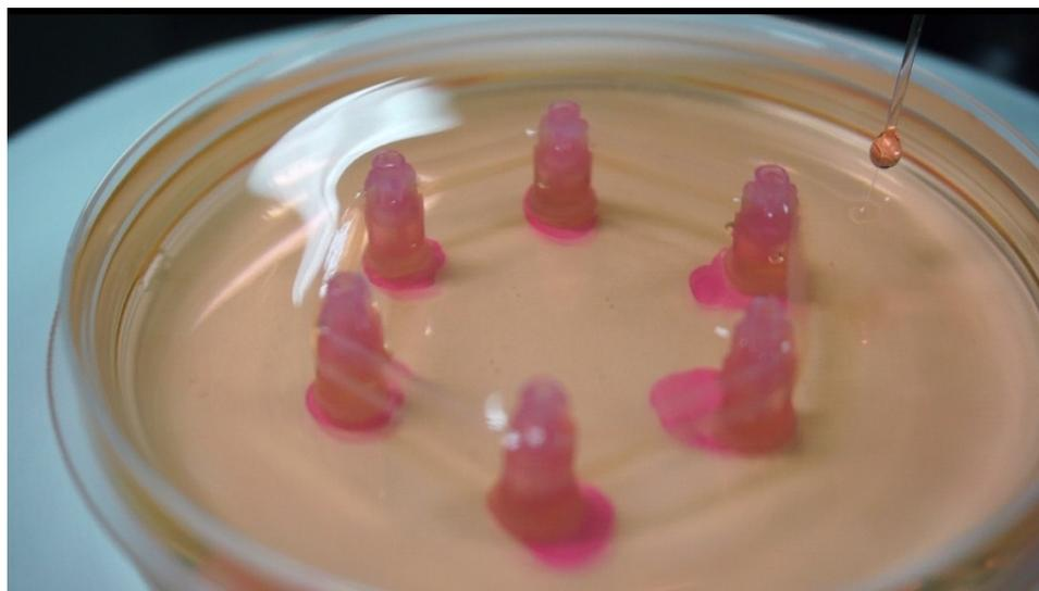
**Movie S1** Rotary collection process of hollow Ca-alginate microfibers from the coaxial microfluidic device.
