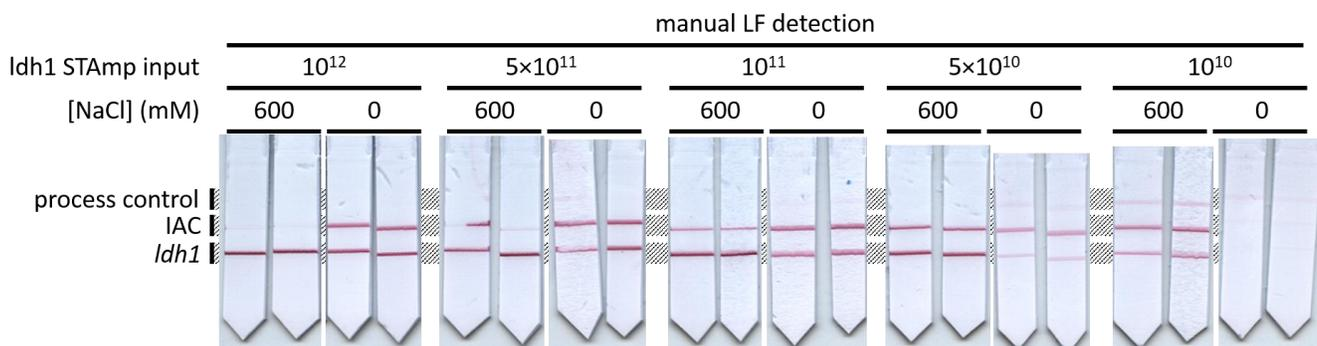
**Fig. S6** Detection results showing impact of salt condition on pDNA binding at ~20°C. A synthetic truncated amplicon (STAMP), which replicated the binding region of the amplicon output by the *ldh1* iSDA reaction, was mixed with detection reagents with and without 600 mM NaCl, and allowed to flow on LF strips. Limit of detection was worse in the no-salt condition.
