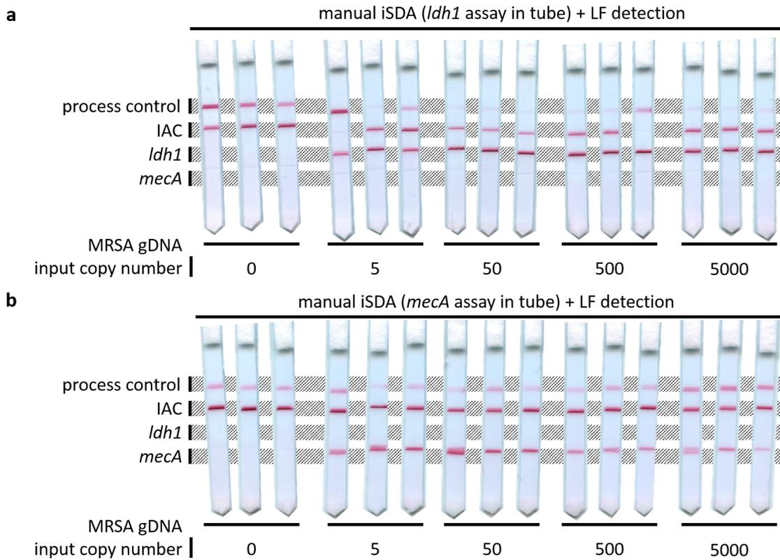
**Fig. S3** Manual iSDA and LF detection result for **(a)** *ldh1* and **(b)** *mecA* assays at low copy numbers of MRSA genomic DNA (gDNA) template. Amplifications were performed in tubes. The results were mixed to salt and Tween-20 to final concentrations of 600 mM and 1% w/v, respectively, then allowed to flow on LF strips. The assay showed robust detection down to at least five copies.
