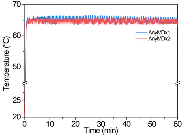
**Supplementary Figure 1.** The feedback-controlled reaction temperature profiles as a function of time. (blue curve: AnyMDx 1, red curve: AnyMDx 2)
