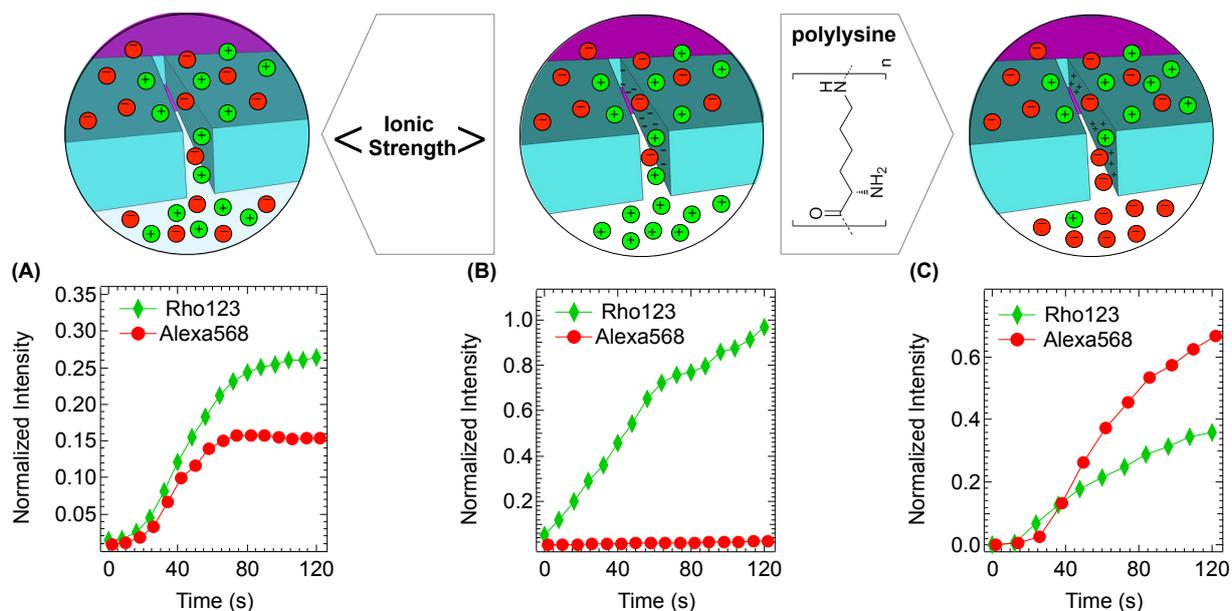
Figure 6: Comparison of permeation kinetics of rhodamine 123 and Alexa 568 in three different experimental conditions. (A) Permeation kinetics through negatively charged nanoslits at high ionic strength (0.5 M KCl). (B) Permeation kinetics through negatively charged nanoslits at low ionic strength. (C) Permeation kinetics through polylysine surface modified nanoslits at low ionic strength.
