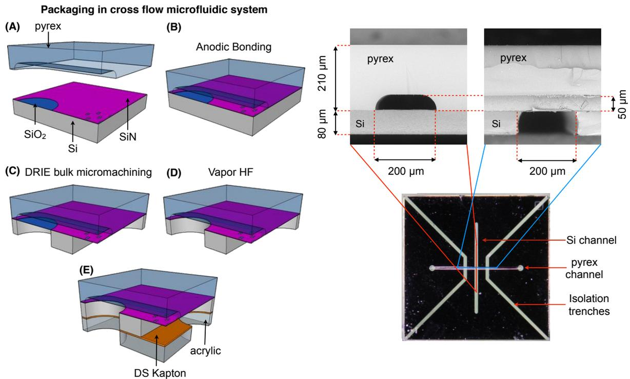
Figure 2: Packaging schematic. Chip top optical view and SEM views of chip cross section along Si and pyrex channel.
