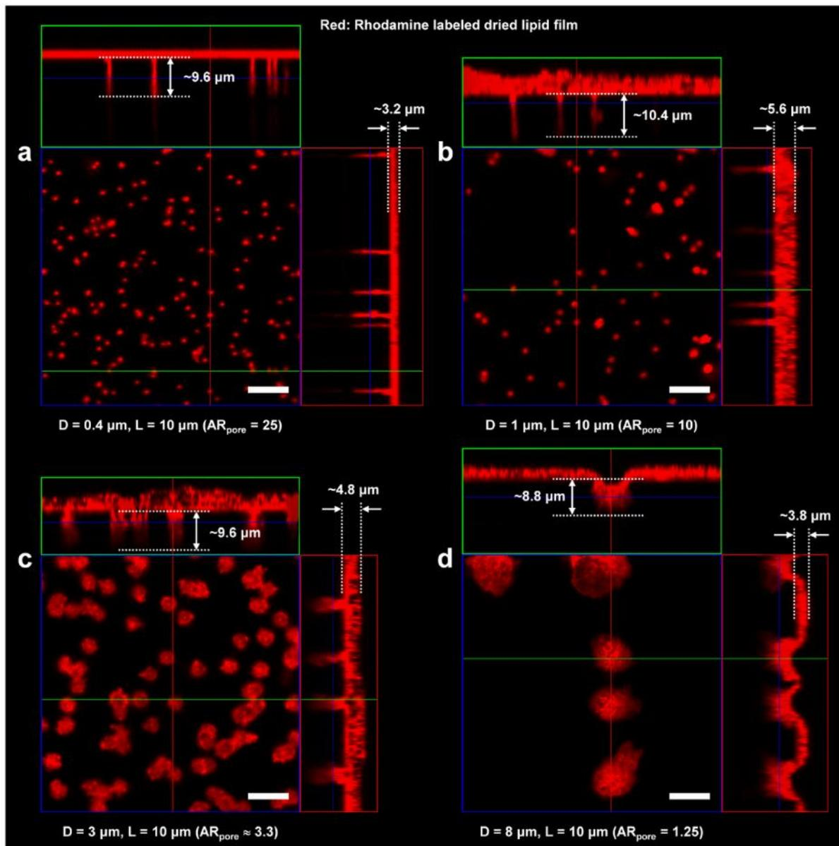
**Fig. S1** Cross-section images of fluorescently-labeled dried lipid films in each of porous membranes. Blue, green, and red box show top-view, X-Z section, and Y-Z section of dried lipid films, respectively. D and L indicate pore diameter and length, respectively. Scale bars, 20  $\mu\text{m}$ .
