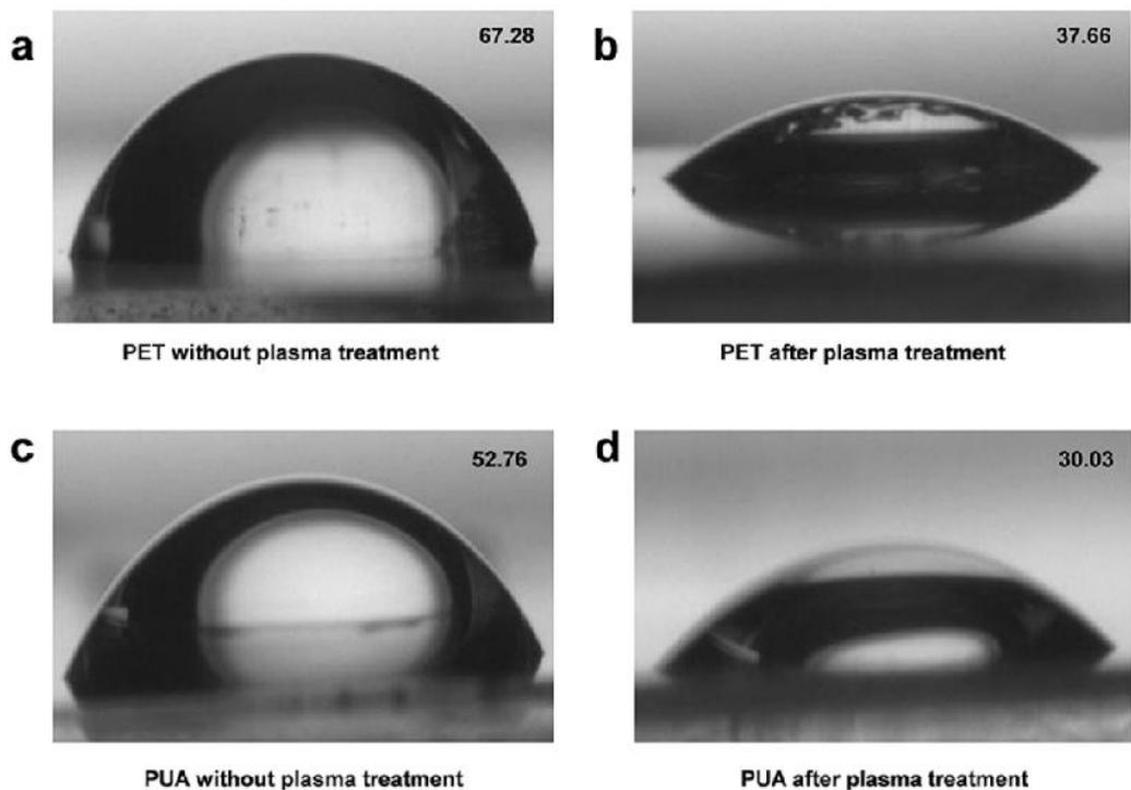
**Fig. S3** Images showing contact angle measurement of PET and PUA porous membranes before and after plasma treatment. After plasma treatment, the porous membranes changed to hydrophilic surface having contact angle of around 30-38 degree, which indicates there is no meaningful difference in surface property between the two kinds of porous membrane.
