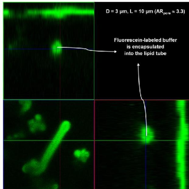
**Fig. S4.** X-Z and Y-Z cross-section images of a lipid tube in a 3- $\mu\text{m}$  transwell porous membrane. Z section is adjusted to the mid of lipid tube which shows the encapsulation of fluorescein-labeled buffer. Green color represents fluorescein.
