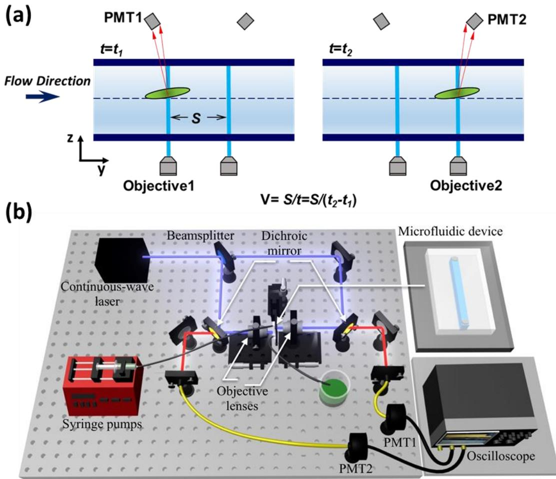
Figure S3 Laser-two-focus (L2F) system. (a) Schematic showing L2F principles. (b) Experimental setup of integrating the stepped microchannel with L2F for applications in flow cytometry.
