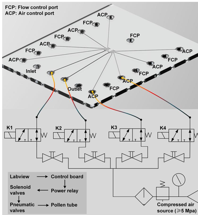
Fig. S1 Automatic pneumatic control system for microvalve pressurization. The inlet shows the schematic of pneumatic control.
