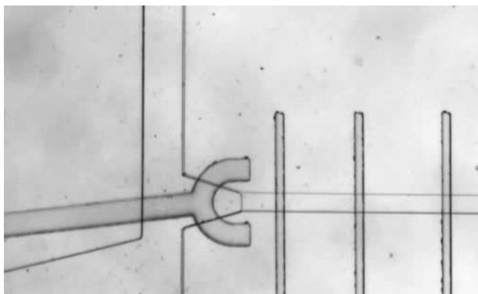
**Movie S1** Real time trapping of a lily pollen tube inside the LOC device. This video demonstrates the process of trapping a single pollen tube by reorientating the pollen tube by the flow inside the microchannel and fixing the pollen tube by a microvalve.
