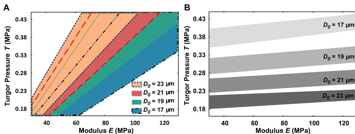
Fig. S4 Parameter space for stretch ratio and compressibility. (A) The subspaces of simulated tube properties that fall within the 95% confidence interval of the experimental  $\lambda$ . (B) Simulated tube property subspaces that fall within the 95% confidence interval of the experimental compressibility.
