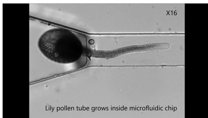
**Movie S2** Lily pollen tube grows inside the LOC device. This video demonstrates the pollen tube can grow well inside the microfluidic channel.
