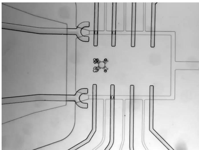
**Movie S3** Automatic pneumatic control of PDMS microvalves for trapping and indenting pollen tubes. This video demonstrates the independent control of PDMS microvalves by the automatic pneumatic control system. The applied pressure can also be regulated.
