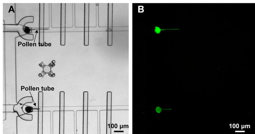
Fig. S2 Two pollen tubes are trapped simultaneously in the LOC device. (A) Bright field image and (B) Fluorescent image.
