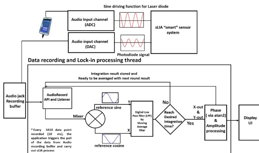
**Fig.S1** the SBLIA software algorithm
