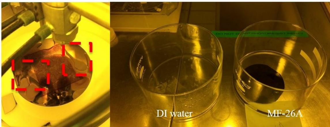
Figure S-4. (Left): partially covered wafer by the developer under the dispense arm of the automated track system. (Right): manual developing process where the wafer is immersed in the developer (MF-26A) after exposure.
