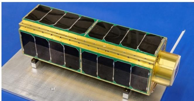
**Supplemental Figure 1. The fully assembled SporeSat nanosatellite is a 34 cm x 10 cm x 10 cm rectangular cuboid.**
