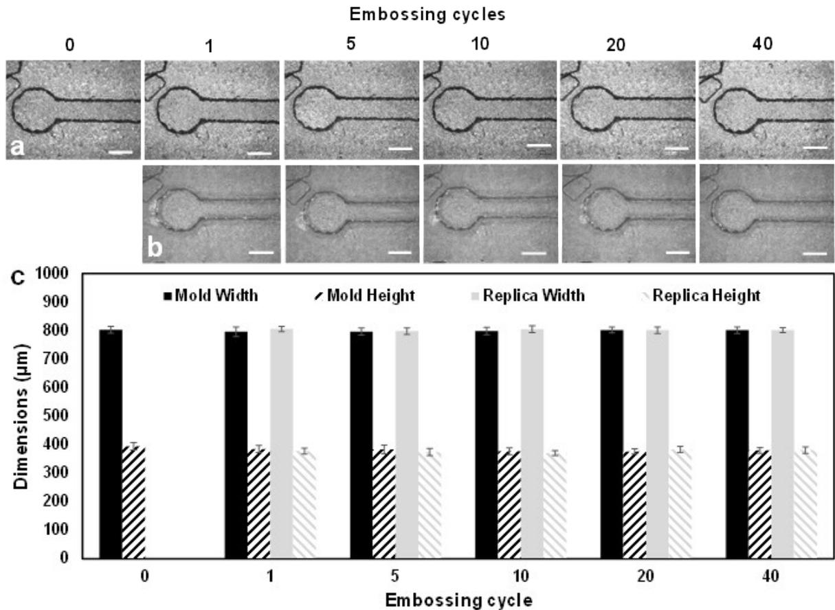
Figure S3: Reproducibility of 3D printed molds for multiple embossing cycles. Optical images of (a) the 3D printed mold and (b) PMMA replicas after 1, 5, 10, 20 and 40 embossing cycles. Scale bars, 1 mm. (c) Measurements of channel width (solid) and height (striped) for the mold (dark) and replicas (light) depicted in panels a and b. Bars represent the mean  $\pm$  SD of three separate measurements.
