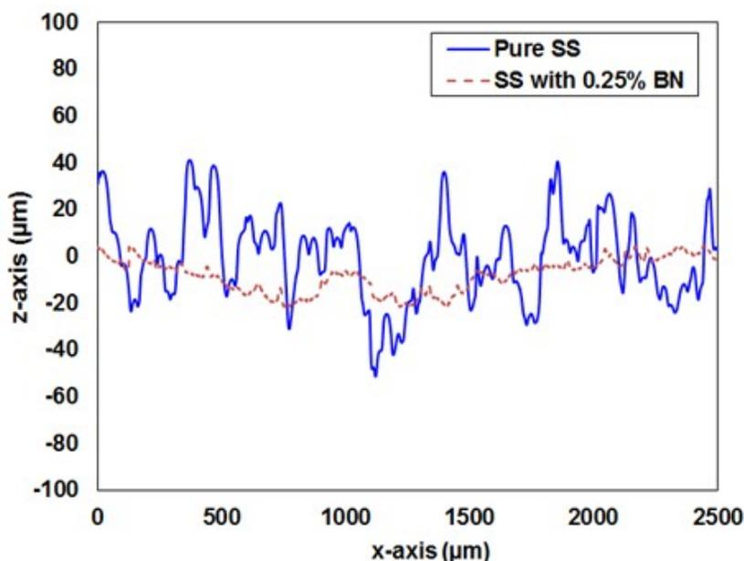
Figure S1: Surface profile scans of a pure SS mold (solid) and SS mold containing 0.25% wt. BN (dashed). Scans were generated using a NanoMap-500LS contact surface profilometer at a scan rate of 50 Hz.
