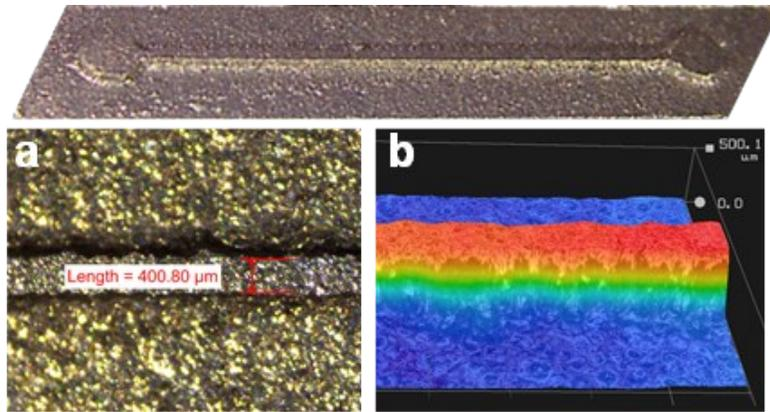
Figure S4: Optical image of the 3D printed mold containing 0.25% wt. BN with compensated dimensions. Results of the channel width (a) and height (b) measurements.
