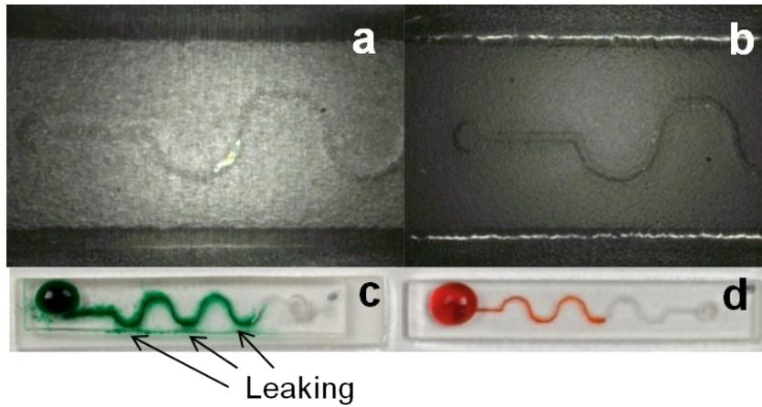
Figure S2: Influence of embossing parameters on the replication quality. Hot embossing performed at (a) 110°C with 0.5 tons, and (b) 120°C with 1 ton. Thermal bonding performed at (c) 60°C and (d) 80°C with 1 ton of force. Replicas were fabricated using the 3D printed mold containing 0.25% wt. BN.
