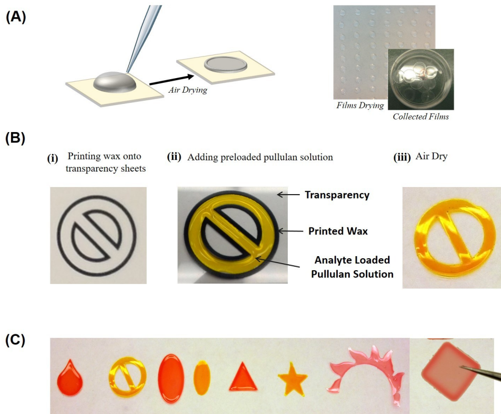
Fig S2. Schematic of how to make preloaded pullulan films in (A) a disc shape or (B) other desired shapes, with various dimensions, by pipetting the pullulan mixture on surface of a flexible transparency PET sheet followed by air drying. The desired patterns are created with PowerPoint and printing these on the PET sheet using a wax printer. (C) Examples of various shapes created using this method.
