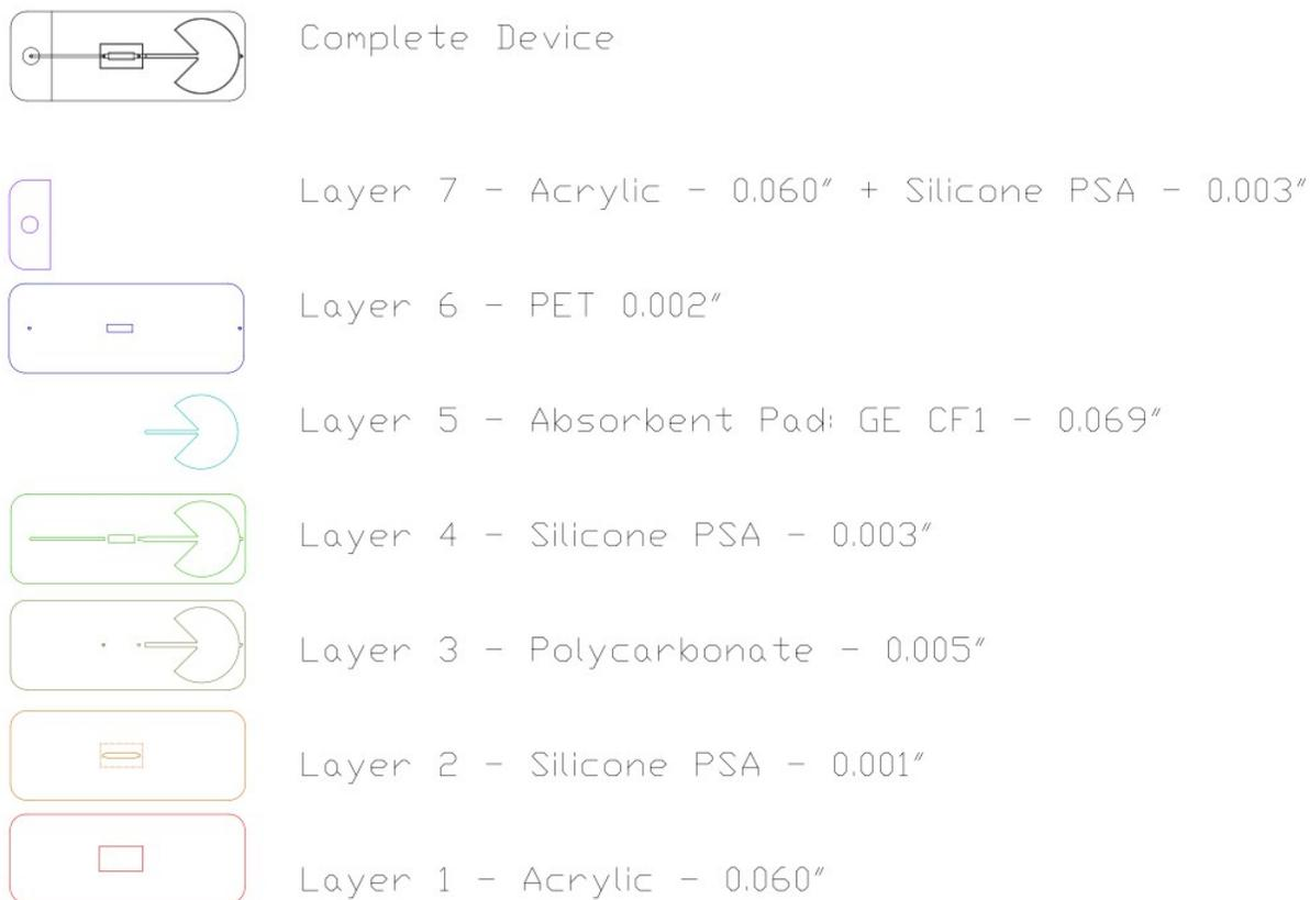
Figure 2. Cartridge design shows the 7 layers used to produce the device as well as the completed device at the top. The materials and thicknesses are labelled next to each layer.
