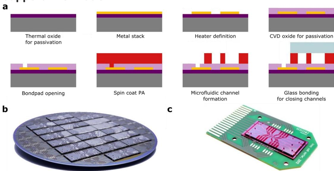
Figure S1. Cell sorter fabrication flow. (a) Fabrication steps of cell sorter chip with integrated fluidics and jet flow generator. (b) Photograph of 200 mm cell sorter wafer before dicing. Glass dies are attached to the cell sorter dies on wafer level. (c) Photograph of cell sorter chip packaged and wire-bonded to PCB.
