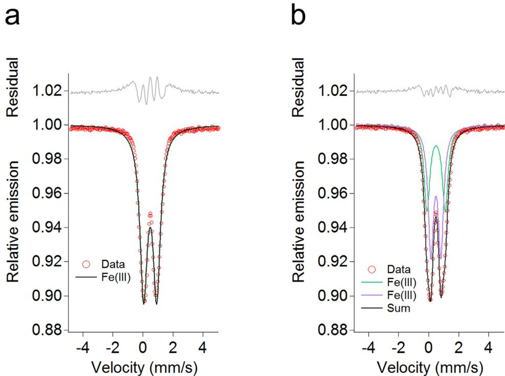
**Supplementary Figure 7.** Simulation of the Mössbauer spectrum of HuHF loaded with 50 Fe(II) per ferritin 24-mer 60 s after reaction with dioxygen. (a) Simulation of the spectrum using a model of one Fe(III) doublet, and (b) using a model of two Fe(III) doublets. The residual (grey lines) is the subtraction of experimental data (red circles) from the superposition of simulated subspectra (black line). Measurements were performed at 80 K.
