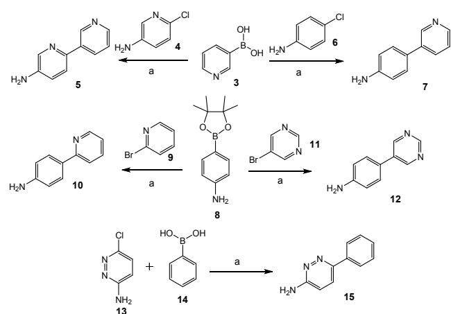
**Scheme 1** Synthesis of biphenyl amine compounds **5,7,12** and **15**. Reagents and conditions: (a)  $K_3PO_4$ ,  $Pd(dppf)Cl_2 \cdot CH_2Cl_2$ , 1,4-dioxane: $H_2O$ ,  $100^\circ C$ , 10-16 h.
