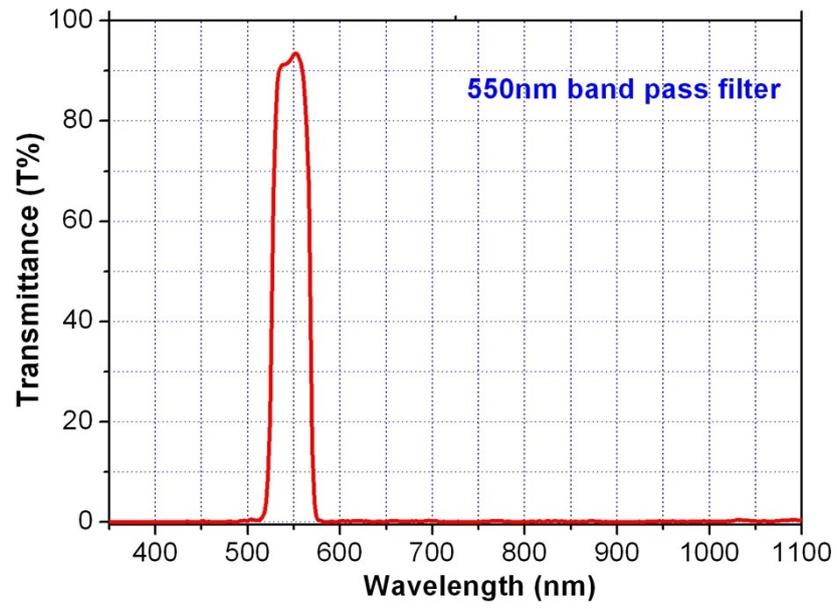
Figure S2. The transmittance spectra of the 550 nm band pass filter.
