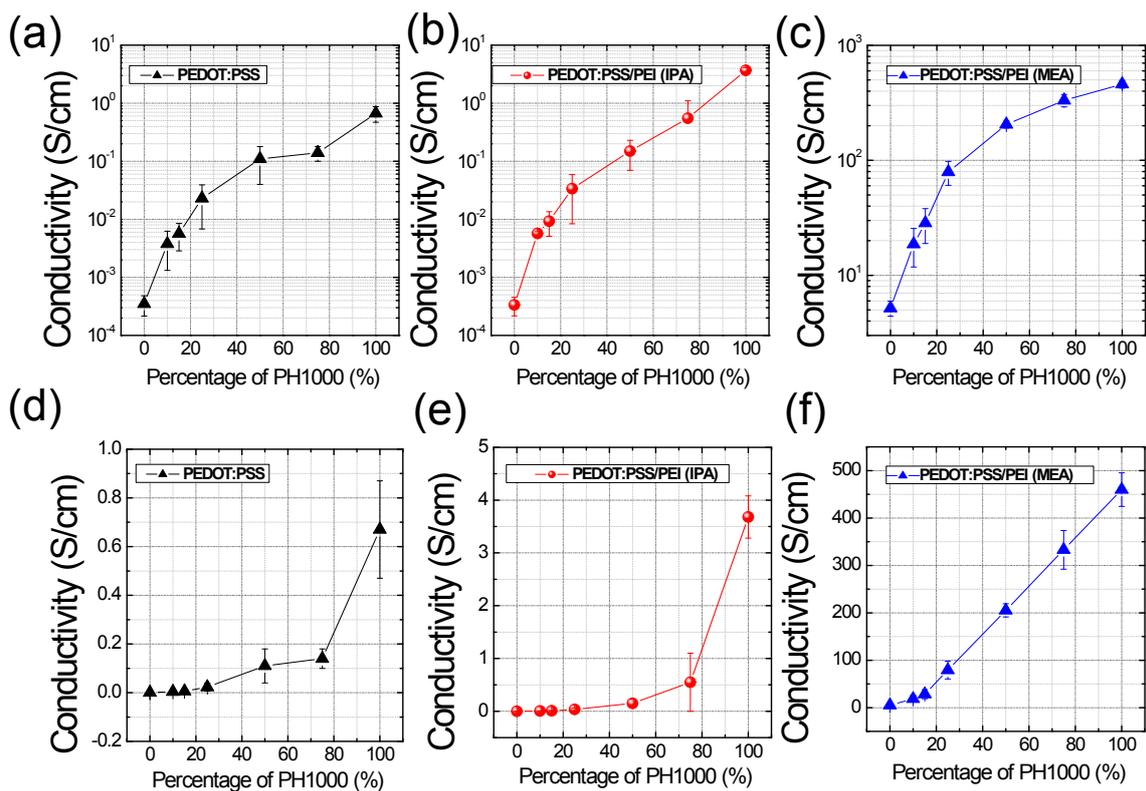
**Figure S4.** Conductivity of the PEDOT:PSS films (PH1000:AI 4083 mixture) with different percentages of PH1000 before and after PEI treatment: (a, d) Films of PH1000:AI 4083 mixture before PEI treatment in semi-log and linear scale; (b, e) Films PH1000:AI 4083 mixture/PEI in semi-log and linear scale where PEI is processed from 2-propanol solvent; (c, f) Films PH1000:AI 4083 mixture/PEI in semi-log and linear scale where PEI is processed from MEA solvent.
