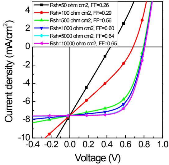
**Figure S1.** Fitted  $J$ - $V$  characteristics with different  $R_{sh}$  with the one-diode equivalent circuit model based on a fabricated device (glass/ITO/PEI/P3HT:ICBA/PEDOT-T,  $R_s = 8 \Omega \text{ cm}^2$ ).
