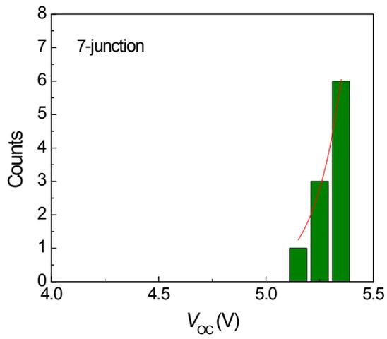
**Figure S9.**  $V_{OC}$  distributions of the all-solution-processed all-plastic 7-junction solar cells (10 devices)
