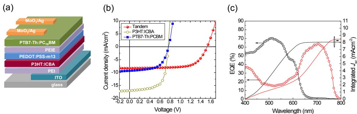
**Figure S7.** a) Device structure of the high-efficiency tandem solar cells with spectrally compensated active layers with ITO glass and MoO<sub>3</sub>/Ag electrodes (non-all plastic); b)  $J$ - $V$  characteristic of tandem and single-junction devices. c) EQE characteristics (the integrated current from the EQE curve is also displayed) of the reference tandem device with structure in (a).
