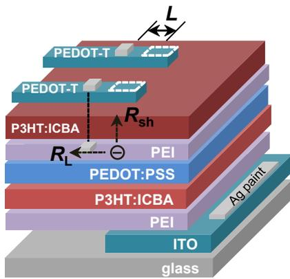
**Figure S2.** Schematic diagram of the possible lateral resistance of the charge recombination layer in the tandem solar cells.
