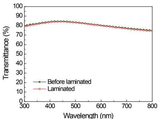
**Figure S5.** Transmittance of the top laminated electrode of PEDOT-T before and after the lamination.
