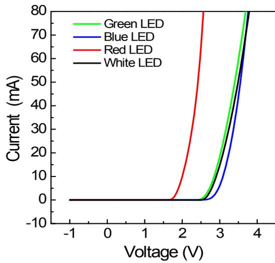
**Figure S10.**  $I$ - $V$  curves of the LEDs with different emission colors.
