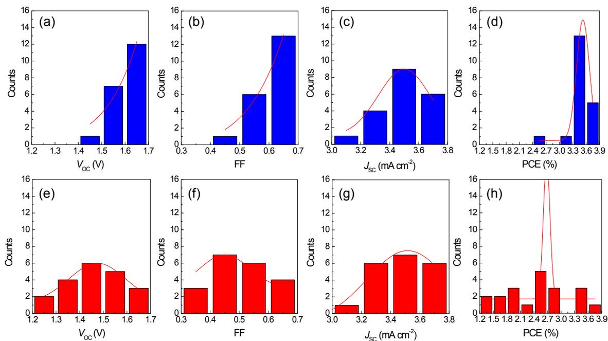
**Figure S6.** Performance distributions of the two-junction solar cells (device structures: glass/ITO/PEI/P3HT:ICBA/CRL/P3HT:ICBA/PEDOT-T) with different CRL: (a-d) with the CRL of PEDOT:PSS-m13/PEI (IPA); (e-h) with the CRL of the patterned PEDOT:PSS/PEI (MEA). (20 cells for each type)
