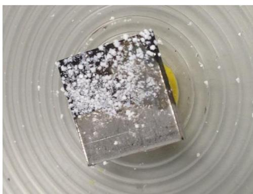
**Suppl. Fig. S1.4:** Most MOF crystallites will be localized at the PPy coated part of the stainless steel substrate after MOF synthesis in an autoclave.
