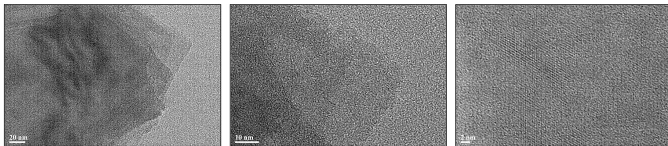
**Fig. S1.** Transmission electron microscopy of 2D MoS<sub>2</sub> recorded on JEOL 2100 equipped with a Gatan Orius charged-coupled device camera and Tridiem energy filter operating at 200 kV.
