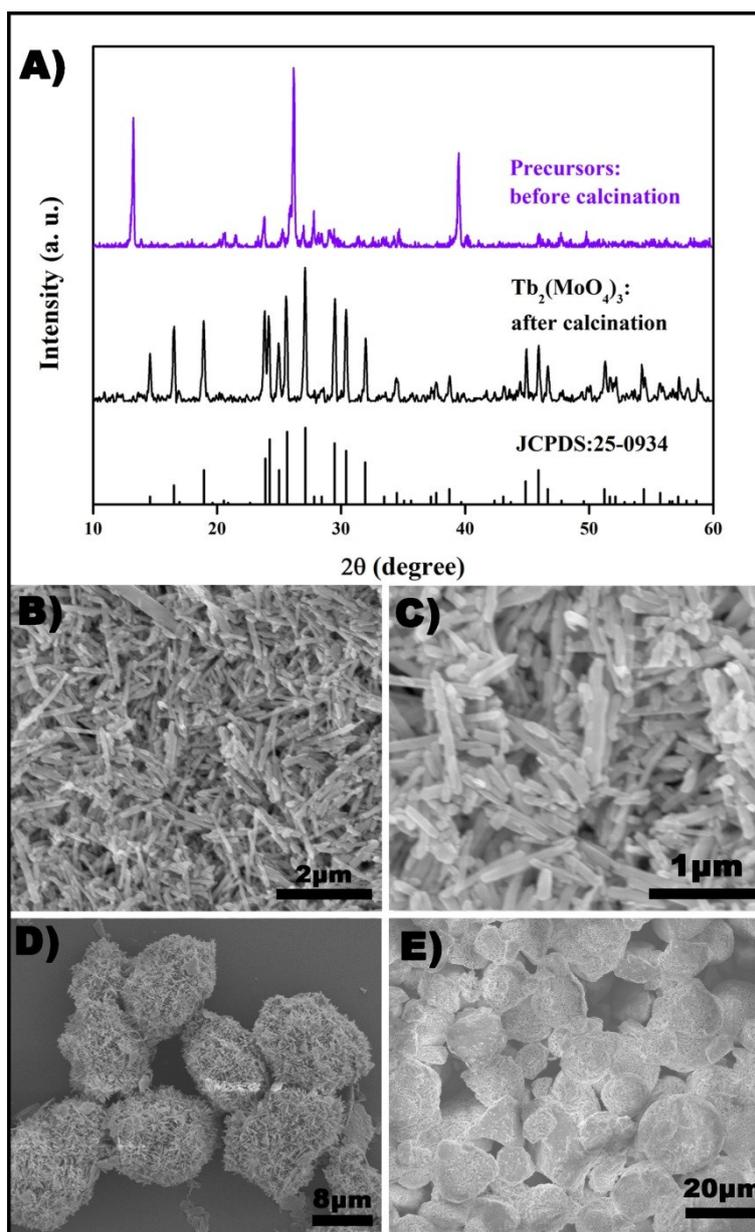
Fig. S2 (A) XRD patterns of the samples obtained before and after calcination (citric acid = 1.26g); (B) and (C) are microstructures of the samples obtained before and after calcination (citric acid = 0.42g); (D) and (E) are microstructures of the samples obtained before and after calcination (citric acid = 1.26g).
