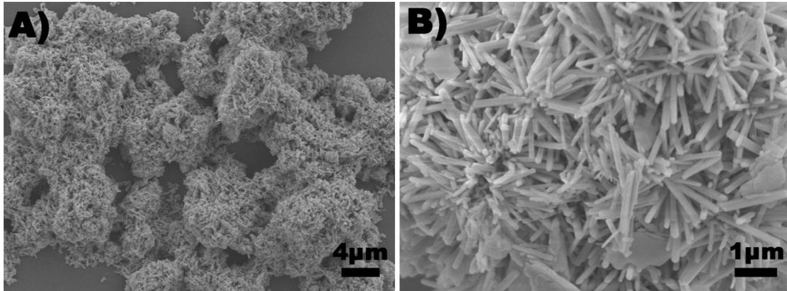
Fig. S1 (A) SEM image of  $\text{Tb}_2(\text{MoO}_4)_3$  precursors prepared with 0.84g citric acid; (B) Detailed surface information of image (A).
