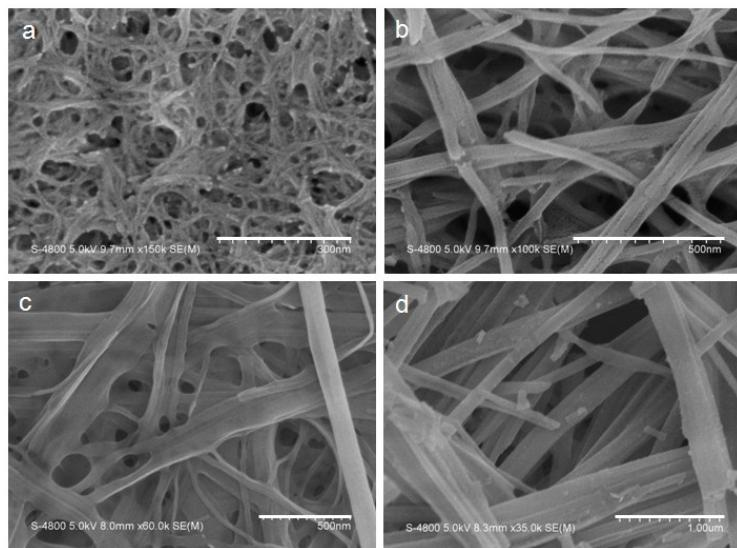
**Figure S4** SEM image of the Ag(I)-AMTD-MOG in different mixed solvent (v/v 1:1) (a)  $\text{CH}_3\text{CH}_2\text{OH}/\text{H}_2\text{O}$  (b)  $\text{C}_6\text{H}_6\text{O}/\text{H}_2\text{O}$  (c)  $\text{CH}_3\text{CN}/\text{H}_2\text{O}$  (d)  $\text{DMF}/\text{H}_2\text{O}$
