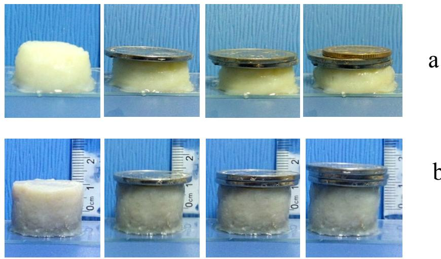
**Figure S1** Photographs showing the compression in the height of the gel prepared at different temperature (a) 40°C (b) 80°C after carrying coins to compare the mechanical strength of the gel.
