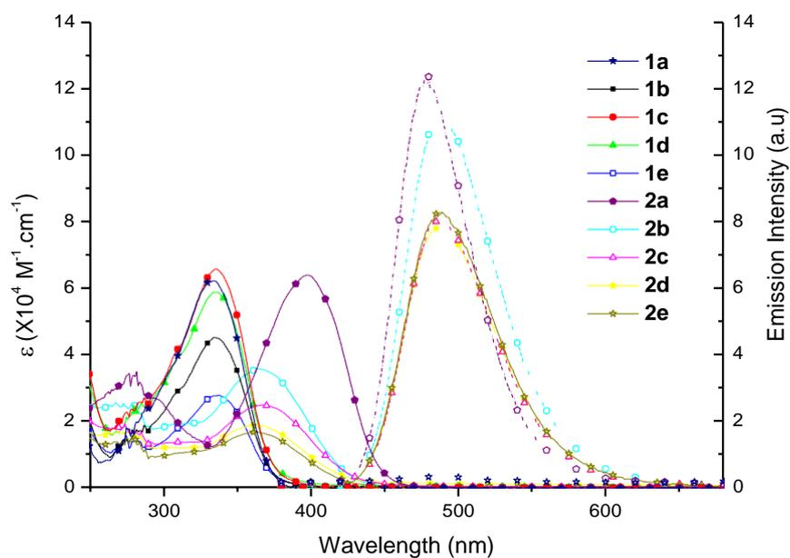
**Figure S25.** Absorption and emission spectra of chalcones **1a-e,2a-e** in THF solution (at *ca.*  $1.10^{-5}$  mol.L $^{-1}$ ). Excitation at 370 nm.
