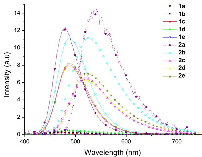
**Figure S27.** Photoluminescence spectra in solution (*ca.* 10<sup>-5</sup> mol.L<sup>-1</sup> in THF, solid lines) and solid state (dotted lines). The excitation wavelength was 365 nm.
